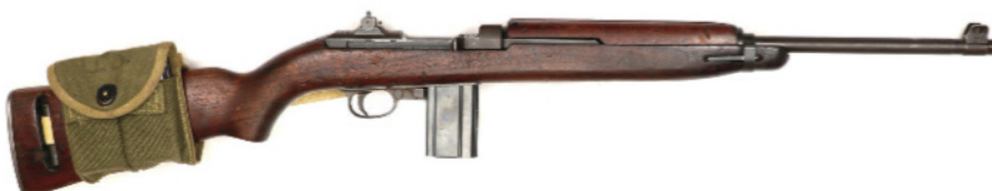
The M1 Carbine filled a niche between battle rifles and handguns, primarily a gun for officers and specialist troops. The early “high wood” stock is identified by the straight stock line covering half the operating rod.
