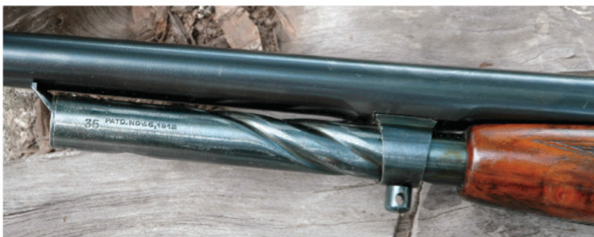
Spiral grooves in the wall of the tubular magazine cant cartridges to prevent bullet noses from resting against primers.
