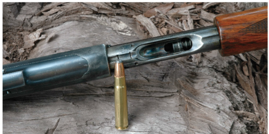
Cartridges are loaded in the magazine through a hinged gate at its bottom, and a spring-loaded follower feeds the action.
