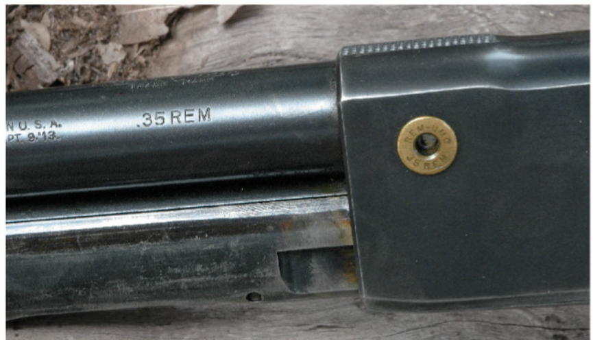
The facsimile of a brass cartridge head embedded in the receiver indicates chambering and includes a hole to vent gases in the event of a case rupture.
