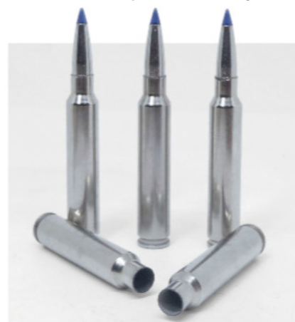
(From l.): .280 Ackley Improved, 7mm Backcountry, 7mm Rem. Mag., 7mm PRC. The Backcountry is the only one that manages 3,000 fps from a 20-inch barrel. (Below) The cartridge is loaded in nickel-plated Peak Alloy steel cases, which permit a much higher pressure than brass cases.
