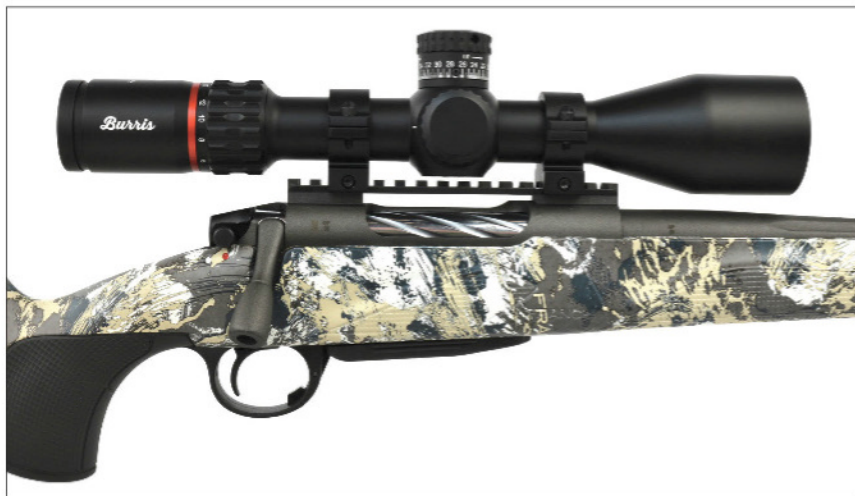
Momentum rifles feature a fat, fluted, tri-lug bolt with a 60-degree throw, and they ship with a Picatinny rail attached to the receiver for easy scope mounting.
