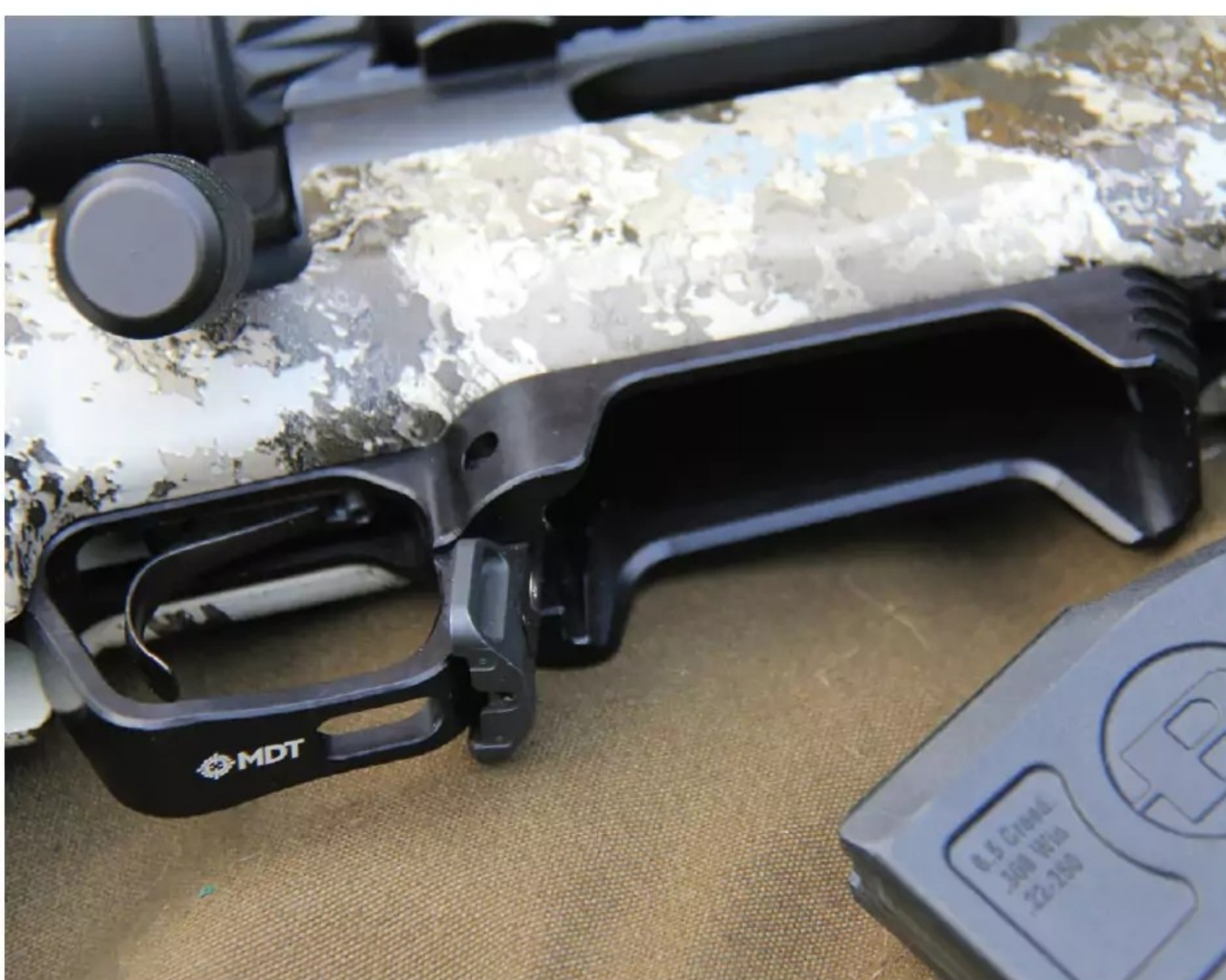
Above: MDT's Precision bottom metal with barricade stop and flared mag well
