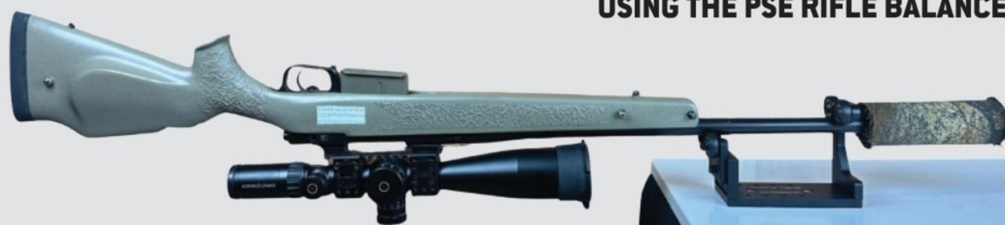
Unbalanced rifle - Centre of Gravity above the line of the bore
