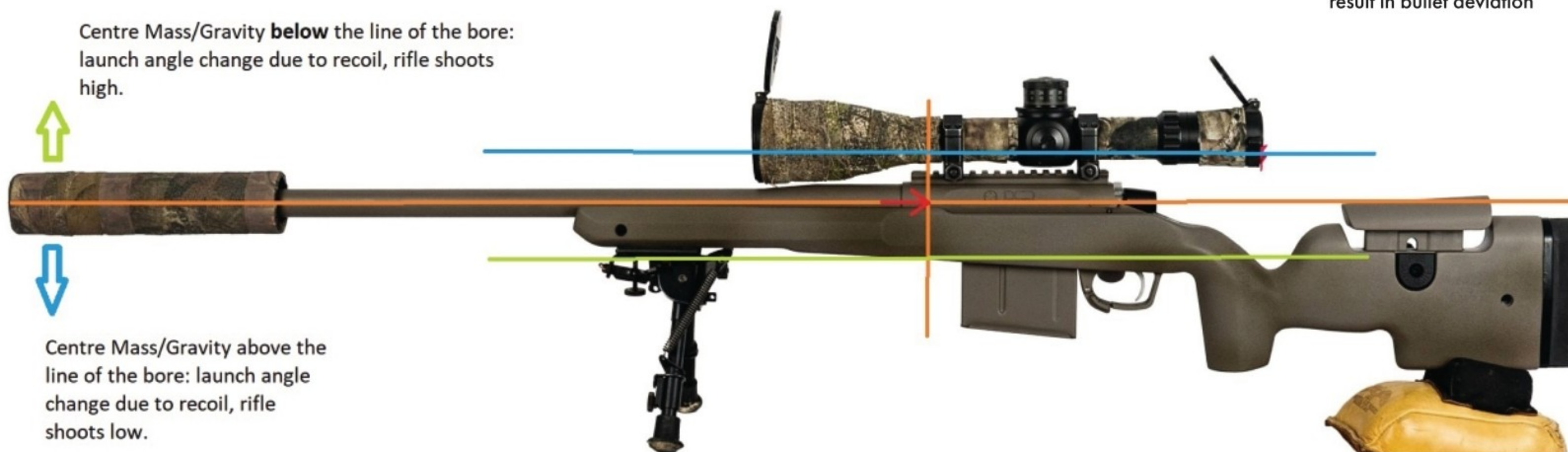
Below: How Centre/Mass Gravity in line with the rifle's bore will change the launch angle and result in bullet deviation
