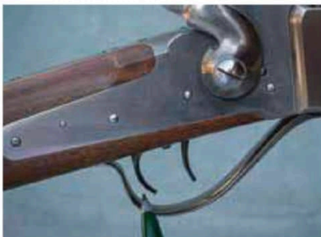
By pulling the rear set trigger, the front trigger pull is reduced to just 8 ounces.
