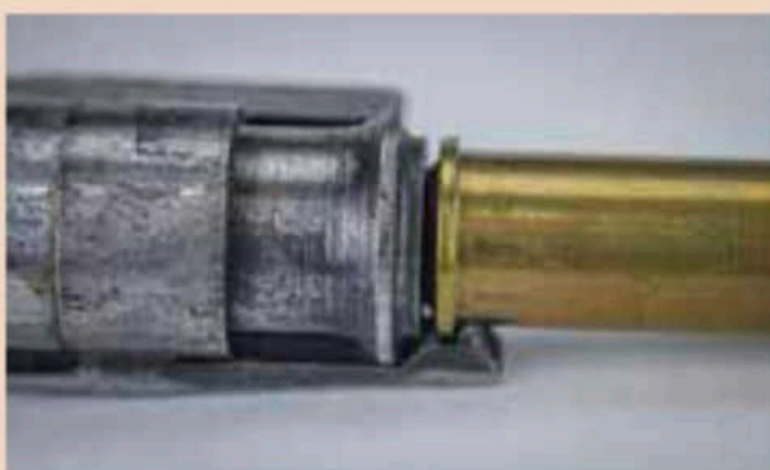
A raised center on the bolt face engages a raised center of the cartridge case head to aid fully chambering the cartridge...
