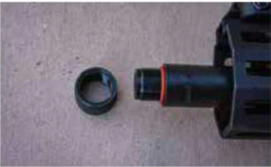
The 16.25-inch hammer-forged barrel is threaded .578x28 and comes standard with a protector.
