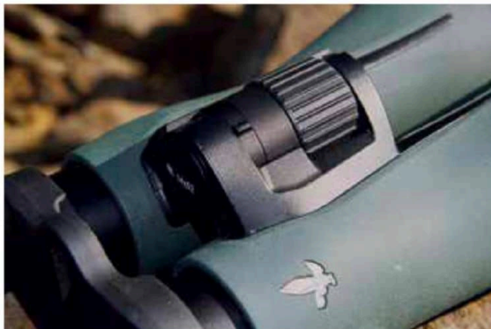
The diopter adjustment of the 14x52 NL Pure binoculars from Swarovski—allowing both eyes to obtain a sharp focus—is located on a rear ring with a raised tab. Hash marks and +4 to -4 indicators can be found on the inside of the binocular frame.
