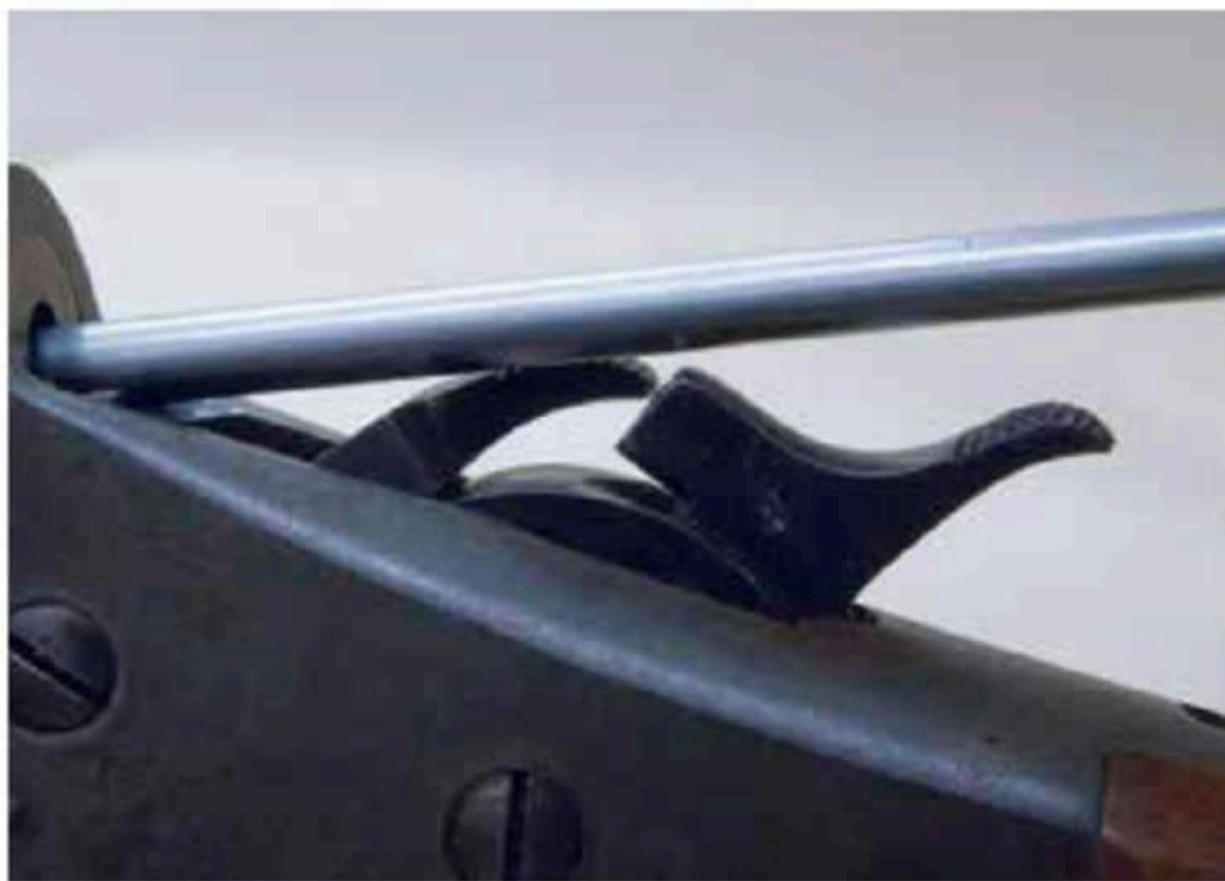
If no sear wear is present, the cleaning rod should miss the hammer nose by the amount shown.
