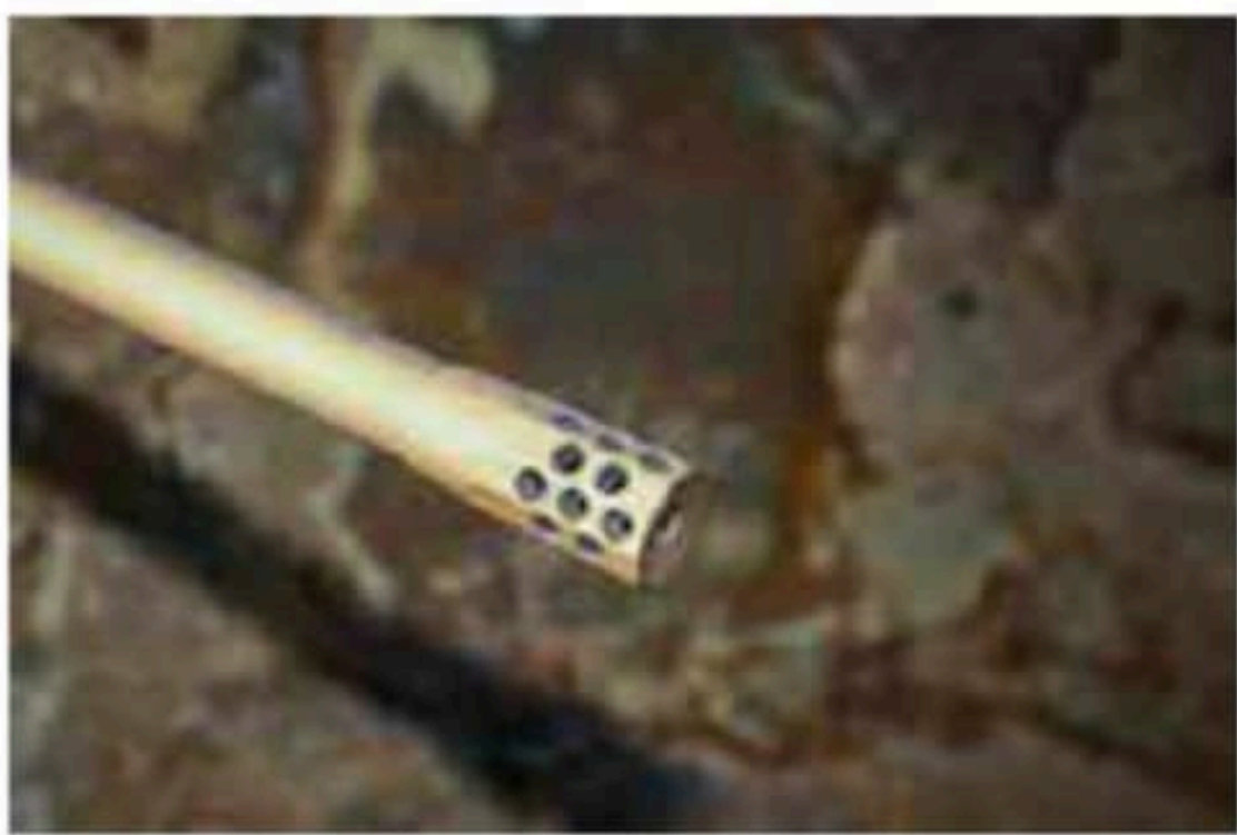
The Montana Rifle Company uses a straight-forward radial muzzle brake on its threaded sporter-weight barrel. The brake was effective at taming recoil and muzzle jump, but proved utterly obnoxious to the ears.
