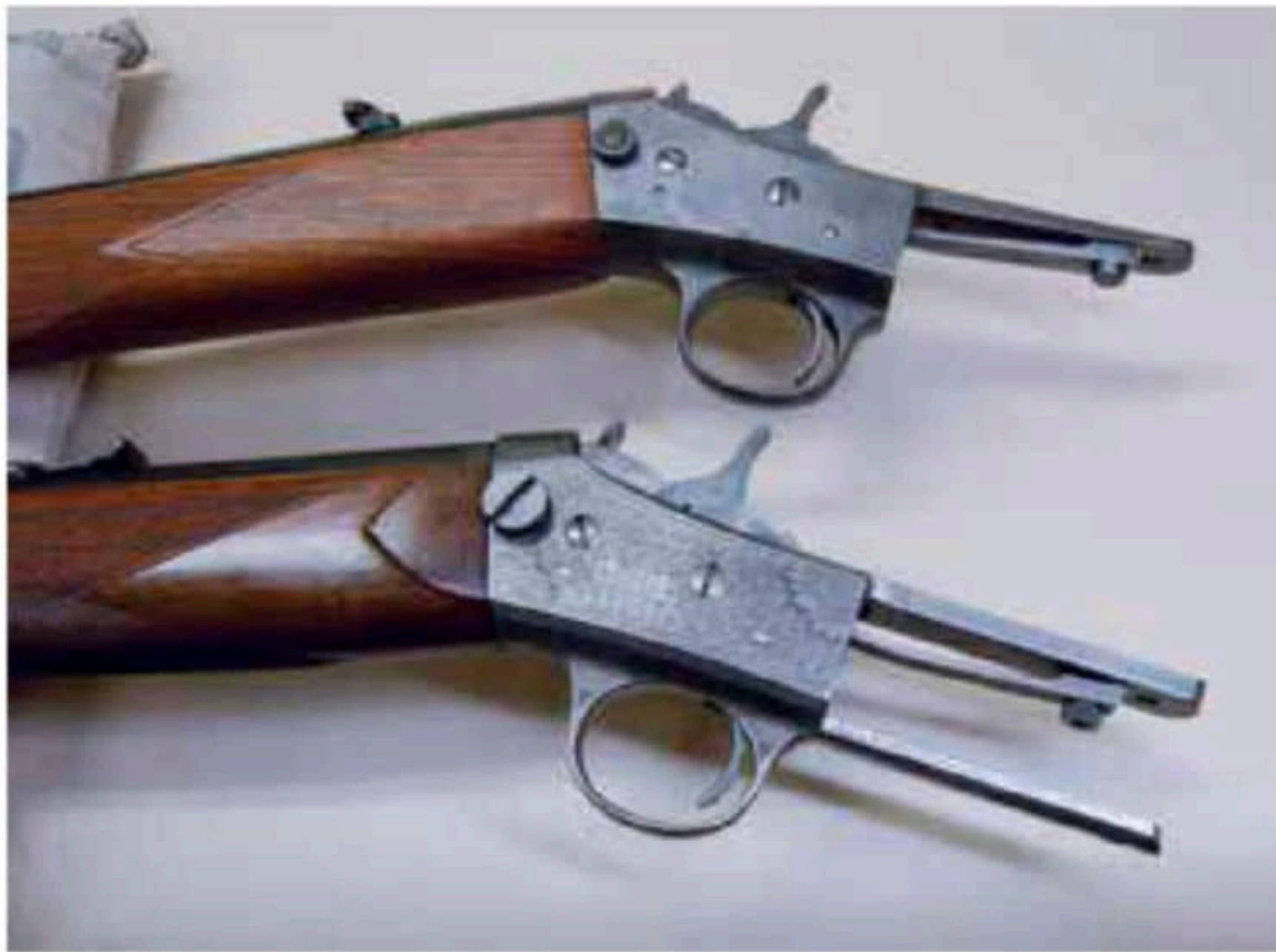
Unaltered Rem. No. 4 with no lower tang (top) and with added lower tang (bottom). Side view without stocks.
