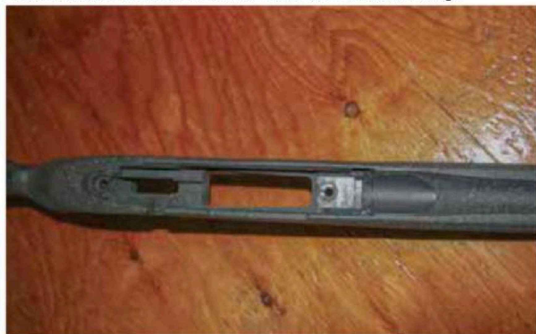
The MRC 2022 action of the Montana Rifle Company Highline rifle is bedded front and rear using high-compression-strength Devcon material. The stock also includes an embedded aluminum block behind the recoil lug.
