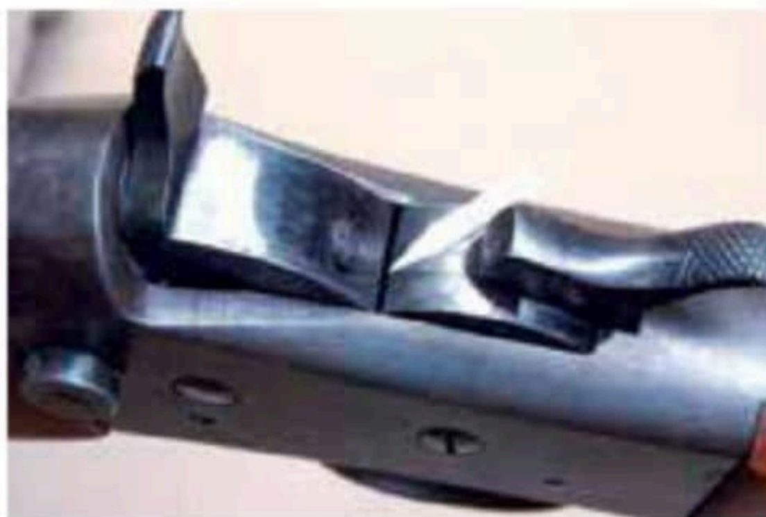
Gap (arrow) between the rear of the breechblock and front of the hammer when cocked indicates no sear wear.
