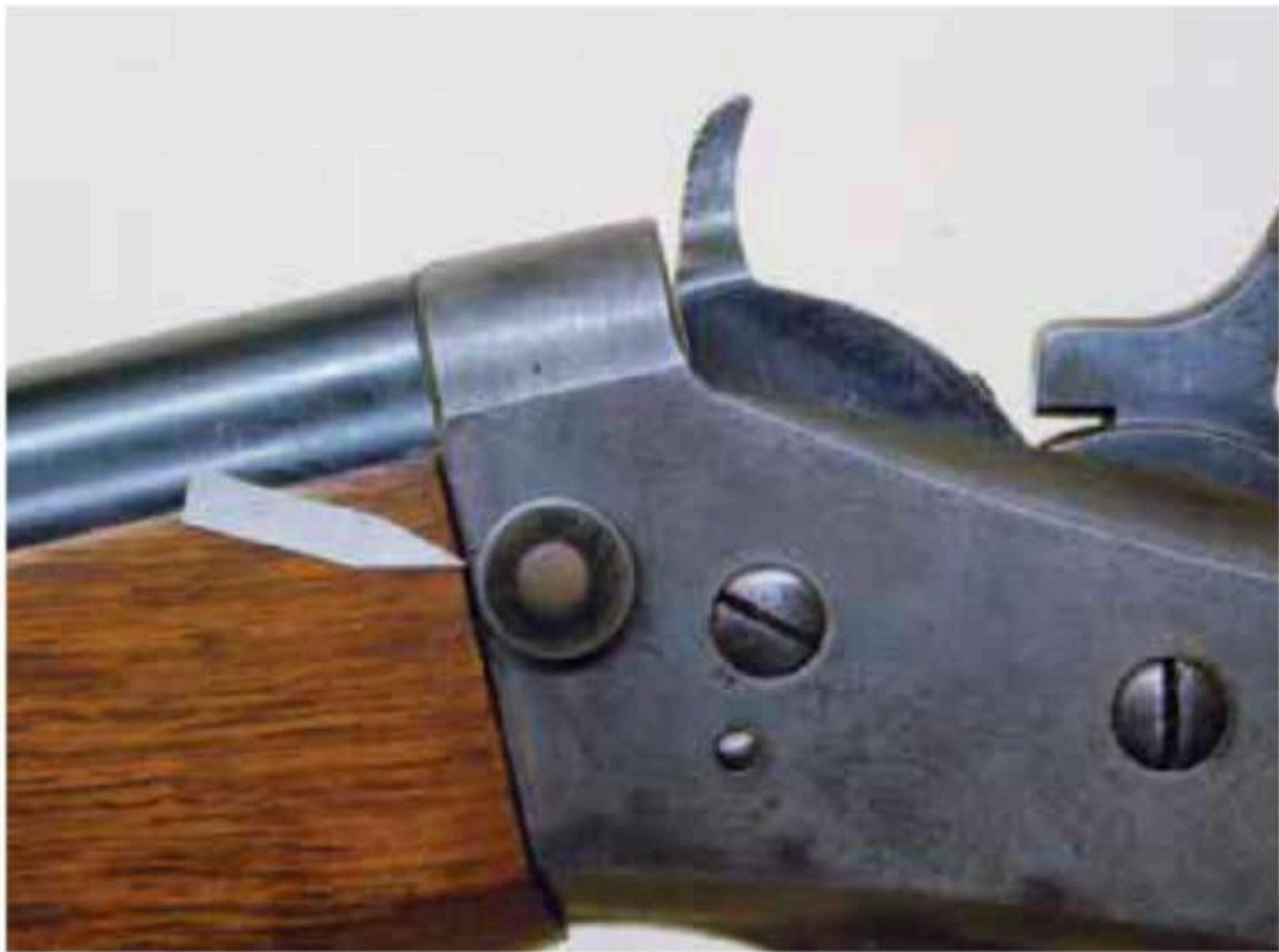
Opposite side of action showing round nut that pulls solid pin tight. It has a locking compound on it and won't come apart for the photo!
