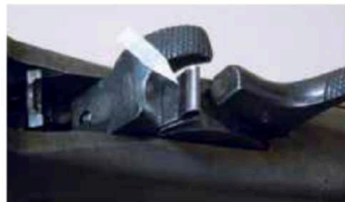
If the cleaning rod does rub the hammer nose a bit, a shim (arrow) between the breechblock and the hammer will push the hammer back far enough to miss the rod.
