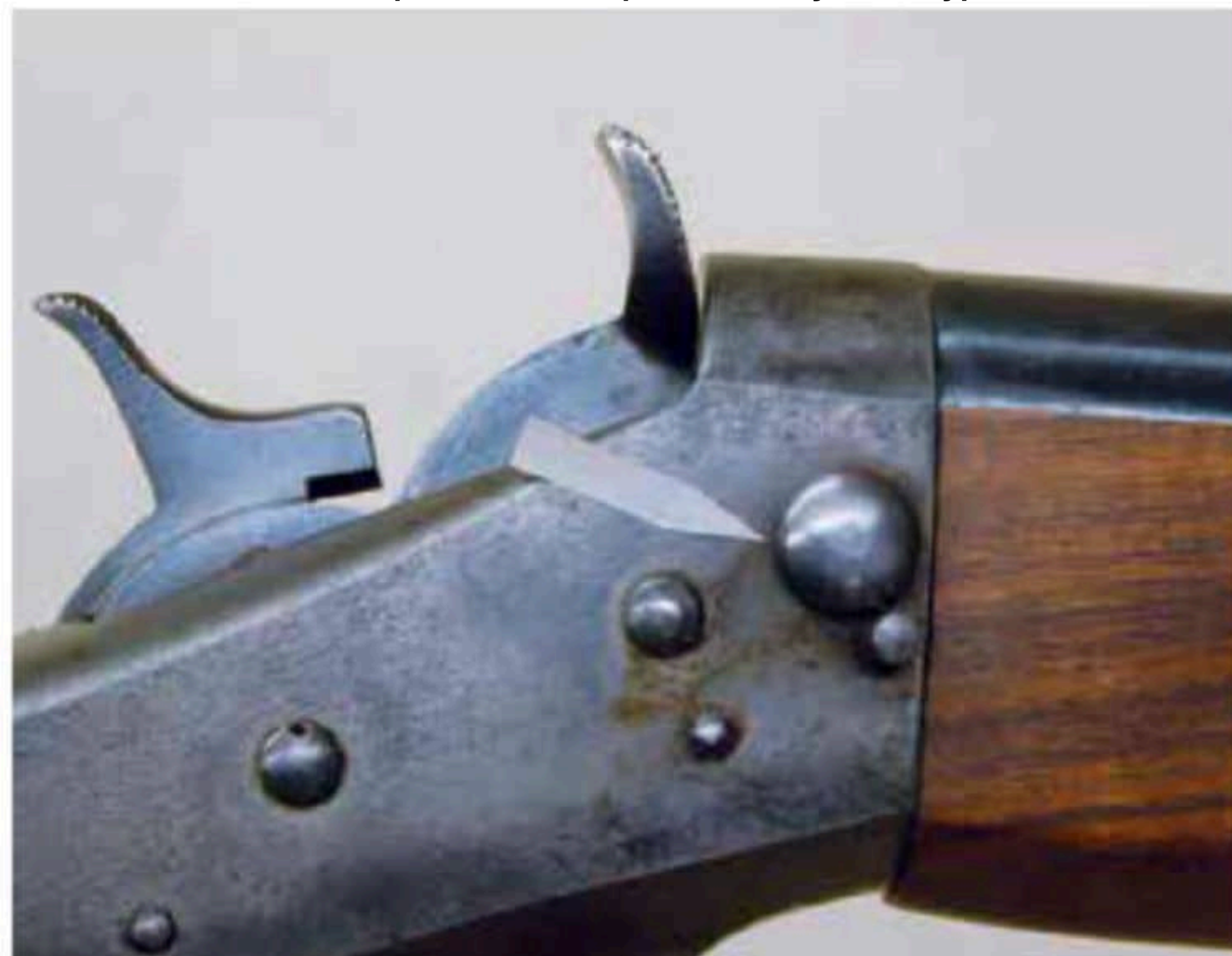
Head of solid takedown pin made to replace factory lever-type.
