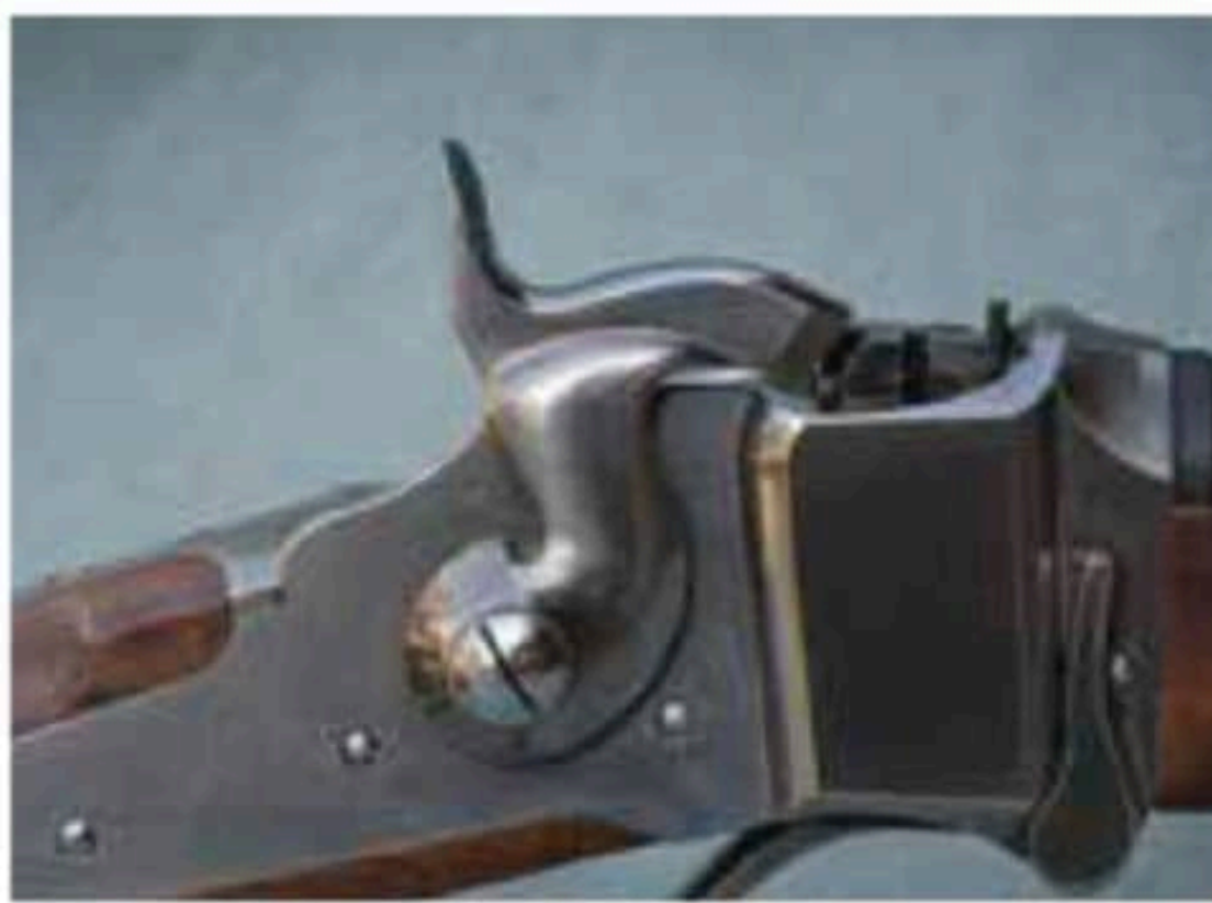
The hammer should be brought to the first click, or safety position, prior to opening the action to prevent damage to the firing pin.
