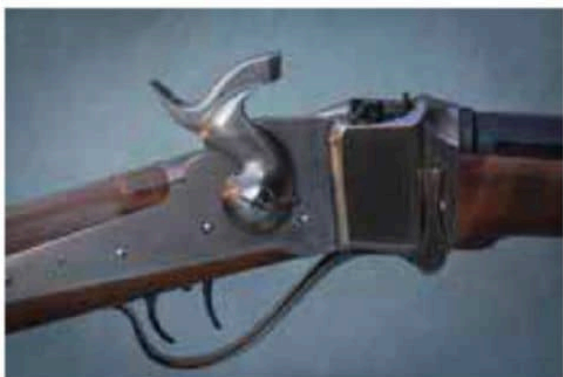
The hammer in the rear position is ready to fire. The rear set trigger should only be pulled once the hammer is cocked.
