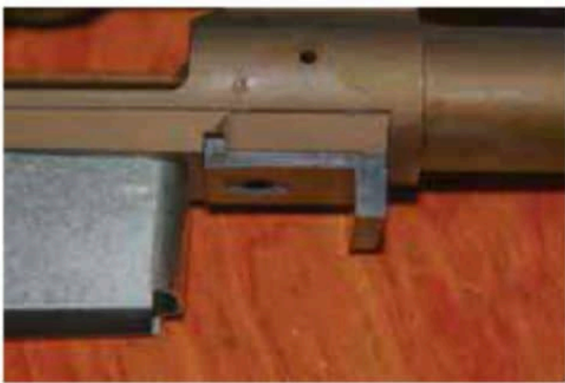
The MRC 2022 action's "Z-shaped" recoil lug fits into a slot in the action bottom, the front action bolt threading through the flat plate. This reduces material consumption and milling time, saving about $500 while proving effective.
