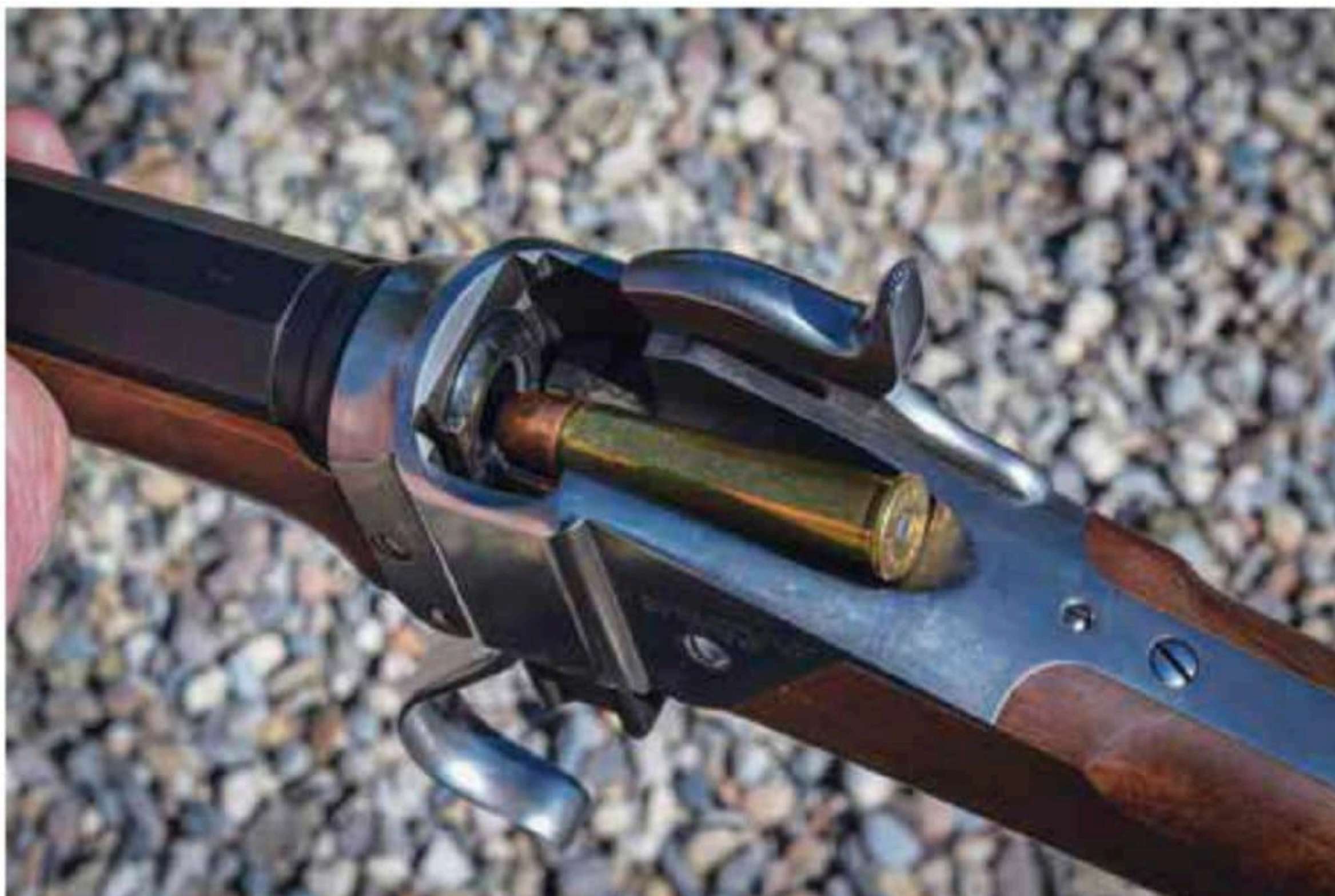
When loading the Model 1874, the hammer should be placed in the safety position to prevent damage to the firing pin.
