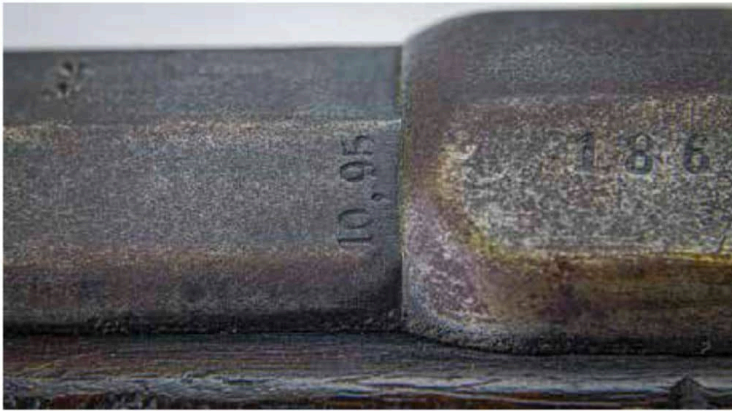
The "10,95" on the barrel indicates the bore diameter in millimeters across the lands (not groove diameter) at the time it was struck. The bore today measures 11.08mm.
