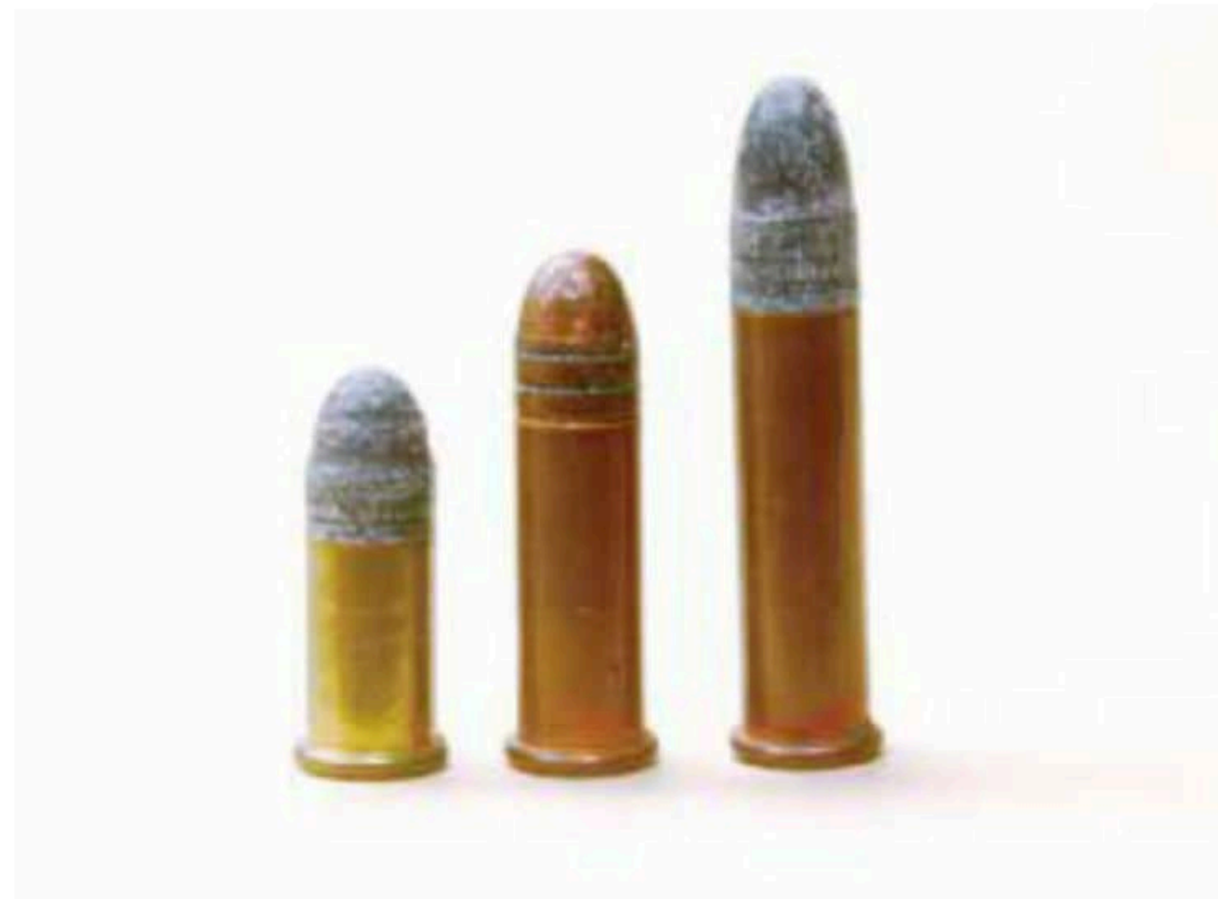
From left, Short, Long and Extra Long cartridges show why the shorter rounds didn't shoot well in an Extra Long chamber.
