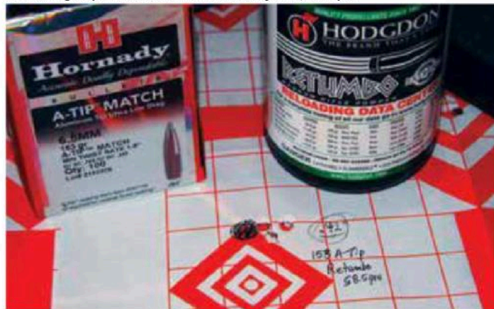
The best group of the entire test included a handloaded Hornady 153-grain A-Tip Match bullet seated over 58.5 grains of Hodgdon Retumbo. That .42-inch group included a muzzle velocity of 2,896 fps.
