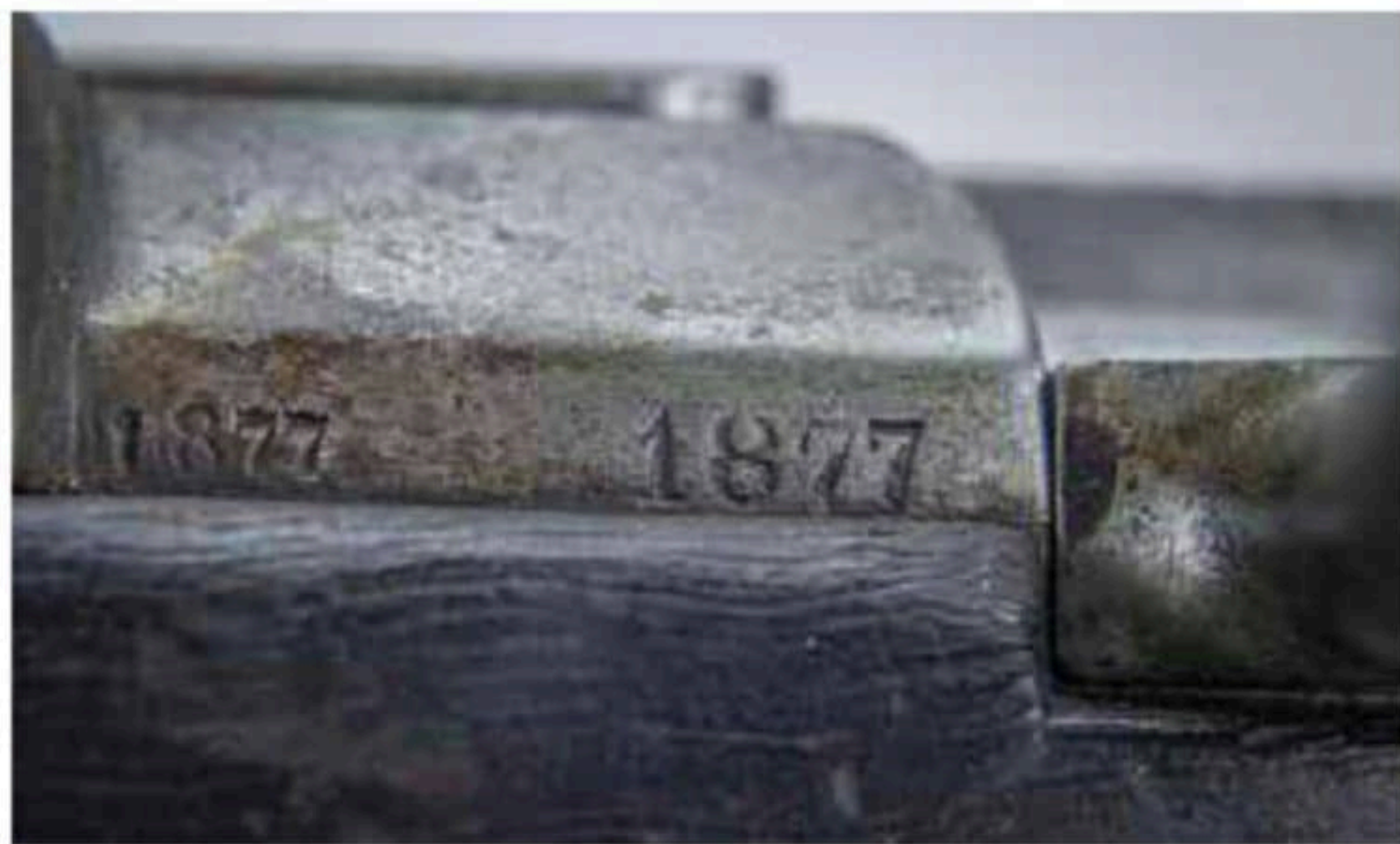
The manufacture date is "1887". Visible to the right, the bolt's only locking lug, the bolt guide, bears against the receiver.
