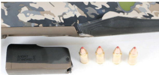
In standard cartridges, the X-Bolt 2's rotary polymer magazine holds four cartridges. In magnum cartridges capacity is reduced to three.
