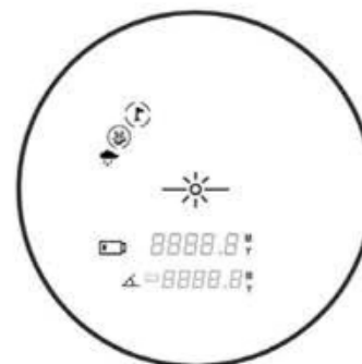
FIELD OF VIEW 104 meters at 914 meters LRF measuring range; 5 - 1800 meters
