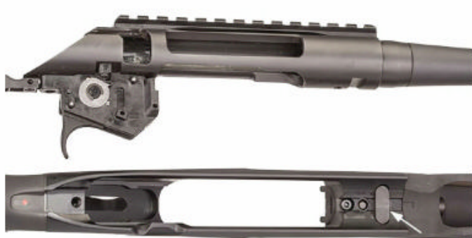
Multiple shim options between butt stock and lower receiver to customise fit
