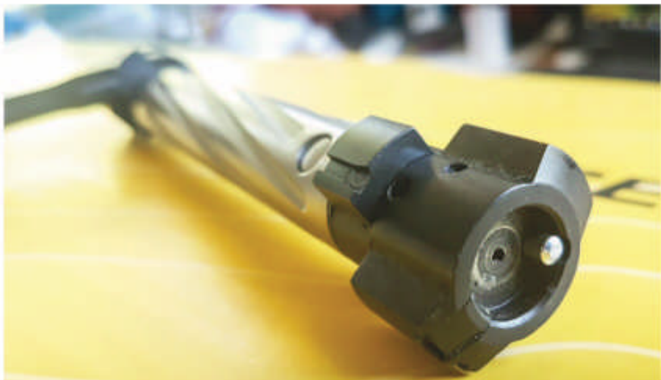
BOLT IN THE BATTERY POSITION WITH FRONT FIXED LUGS VERTICAL, SHOWING ROTATING DUMMY LUGS IN HORIZONTAL POSITION TO BLOCK THE LUG RACEWAYS IN THE RECIEVER IN THE ADVENT OF ESCAPING GAS.
