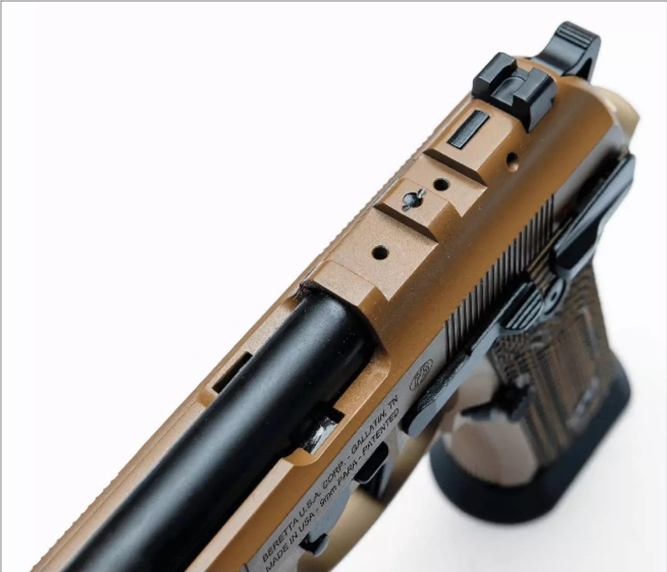
▲ Two slots are machined into the slide to allow for an optic plate. The plate is recessed to allow the firing pin catch to operate.
