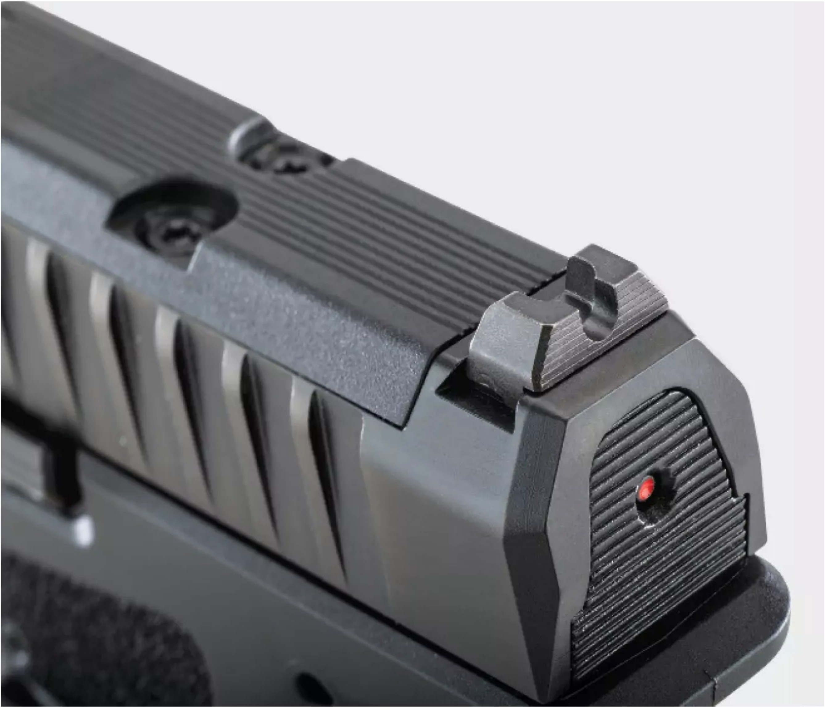
▲ The slide is cut for optics and ships with an RMR adapter plate. The rear sight is a serrated U-notch, and the slide plate and the top of the slide are grooved to reduce glare.
