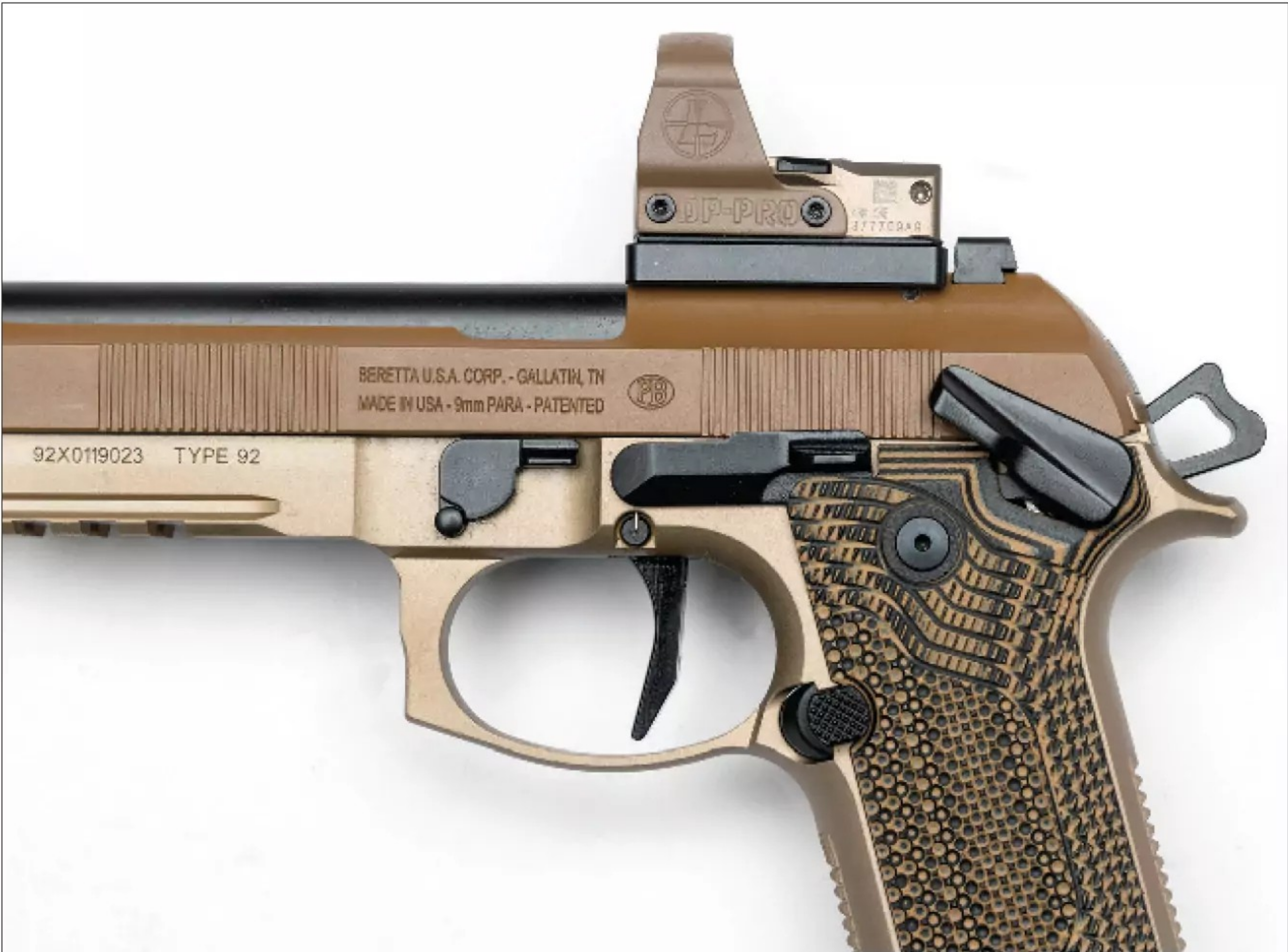
▲ The Sabbia is designed to be carried cocked and locked, and as such it features extended safety levers. The flat Xtreme-S trigger has a light pull and a short reset.
