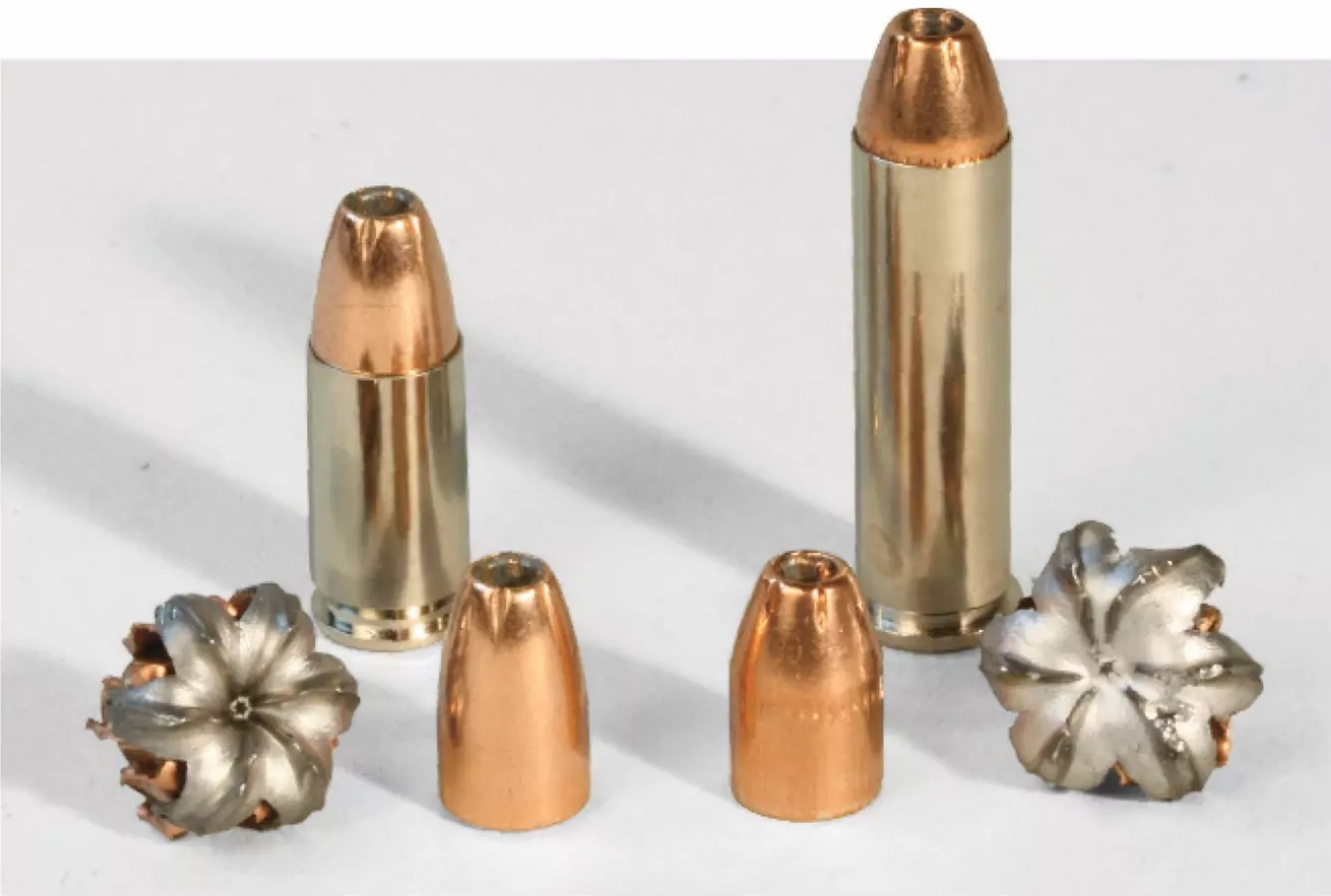
▲ Both the 9mm (l.) and .357 Magnum showed terrific terminal performance in synthetic gel blocks, with excellent penetration and mushroom expansion.
