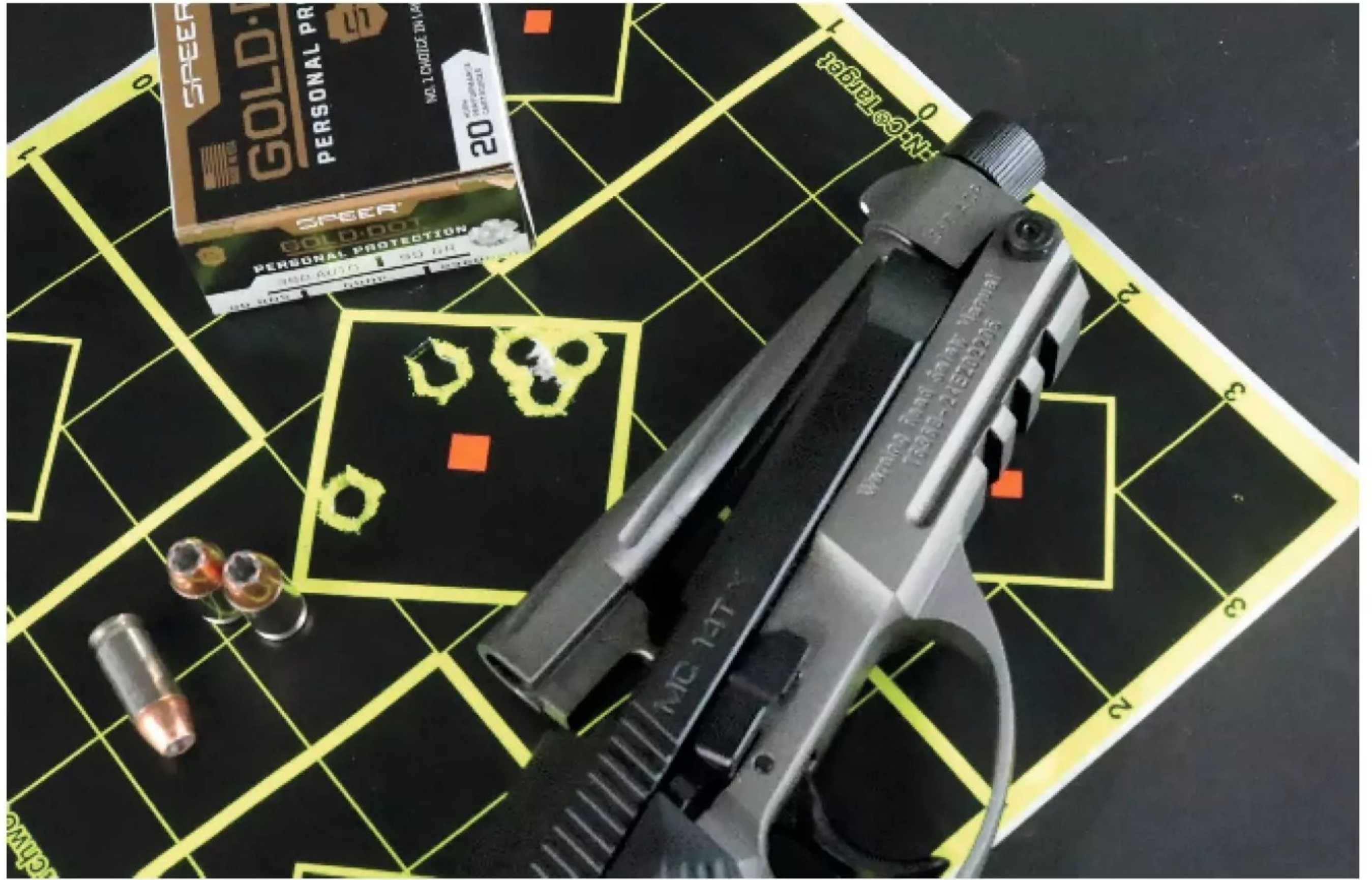
A The MC14T X Solution liked Speer's 90-grain Gold Dot Personal Protection load, placing five shots into 1.4 inches at 25 yards.
