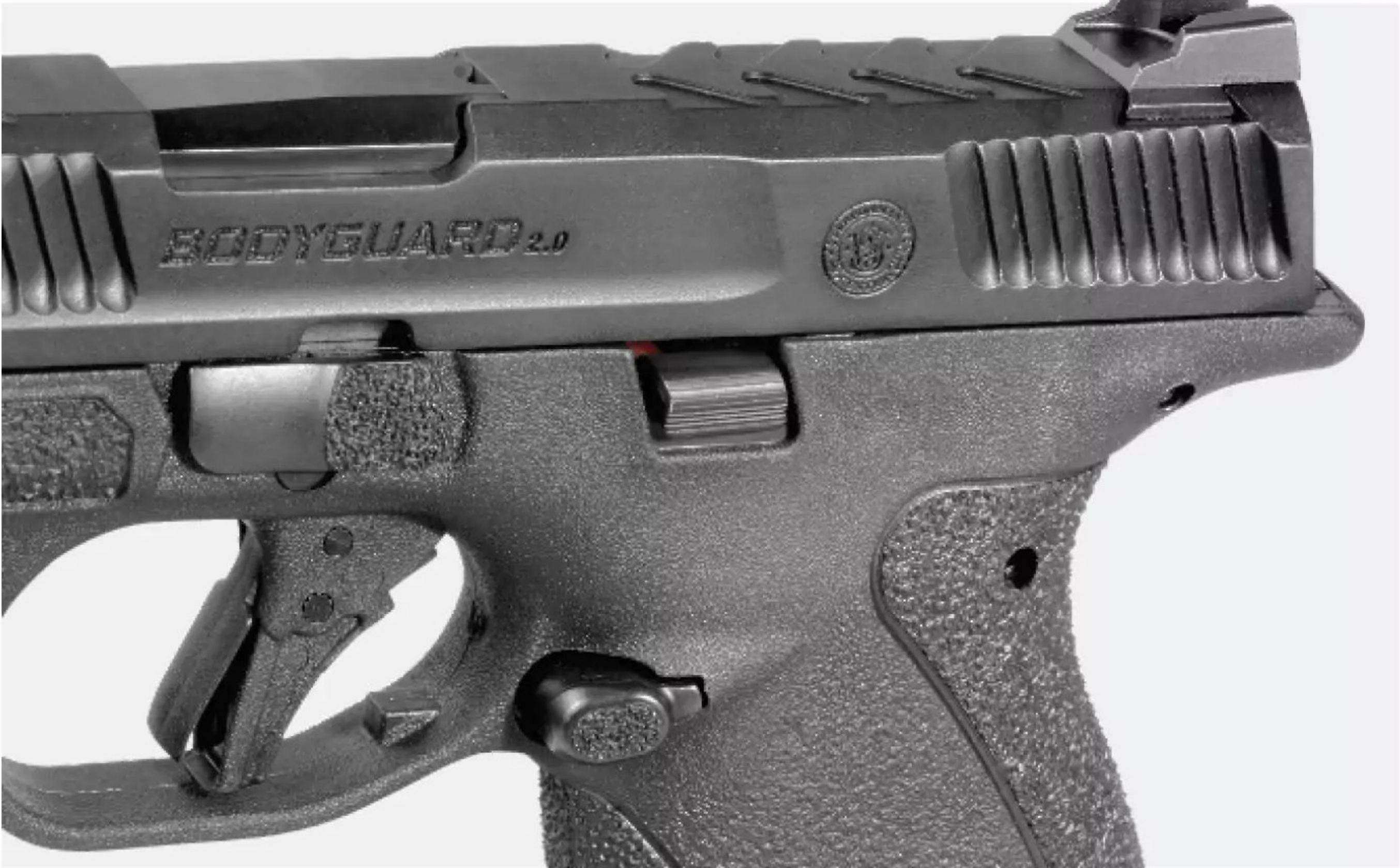
▲ The gun retains the excellent grip layout and striker-fired trigger found on the original 2.0, but the slide serrations and the flare at the rear of the slide make it easier to rack.
