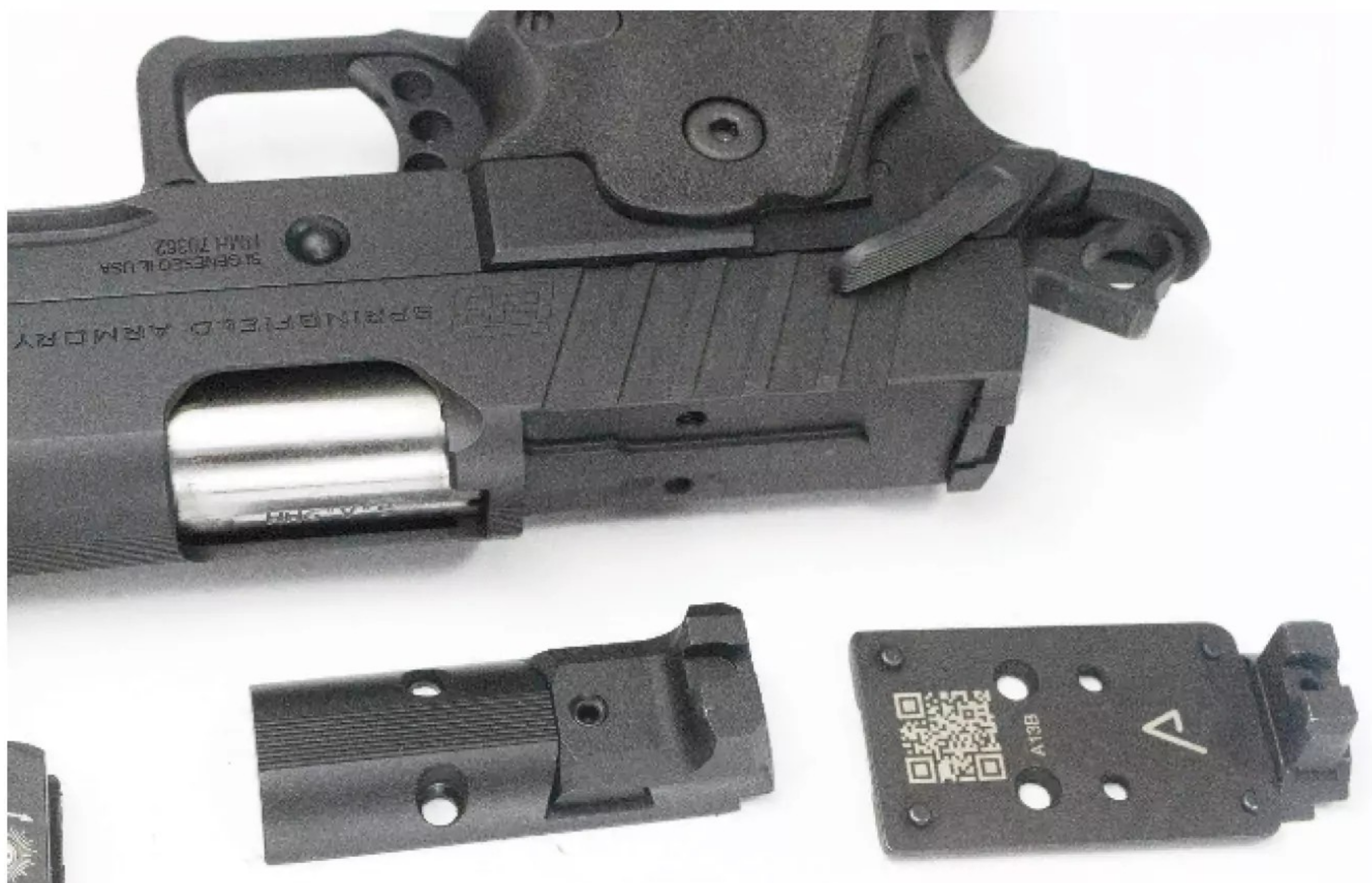
▲ The Fueled Prodigy 4.25 retains Springfield's AOS red-dot mounting system. Both the slide cover plate and dot adapter plate incorporate integral black rear sights.
