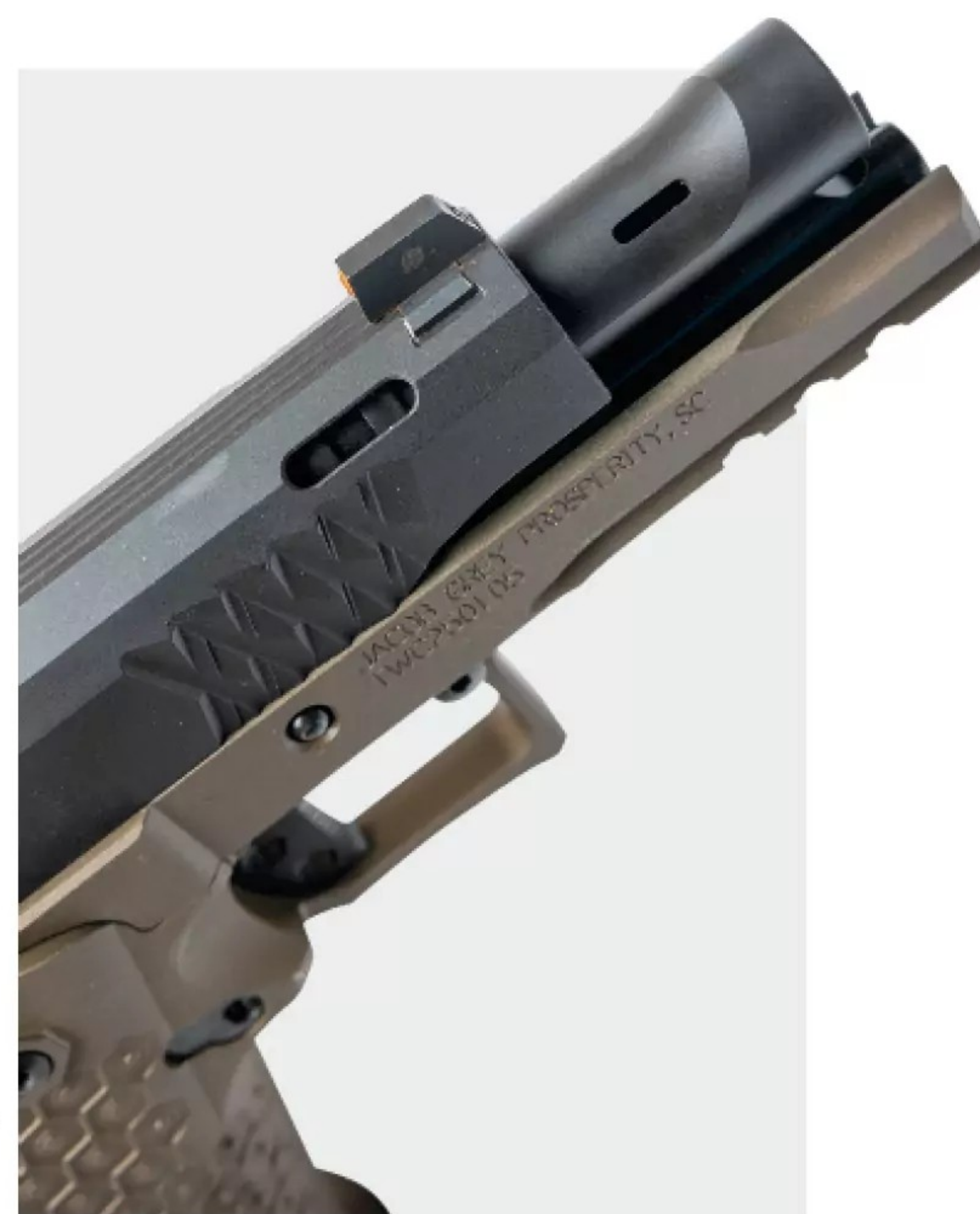
➤ Two longitudinal ports are cut into the barrel and the slide to divert propellant gases and reduce muzzle rise.
