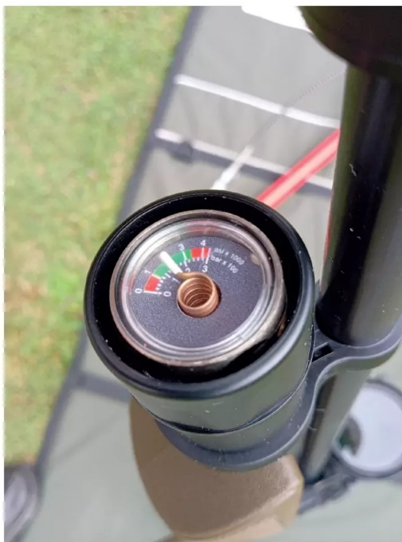
Detail of the well-marked manometer. You just need to work within the green area
