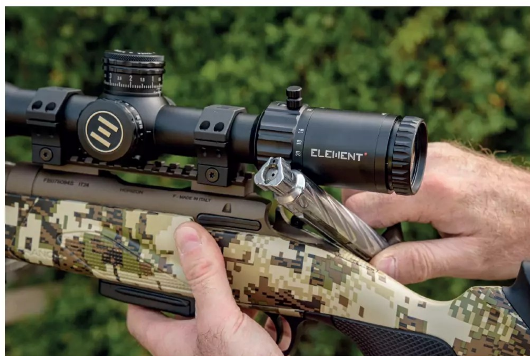
Here you can see the left-hand side bolt release catch and the three-lug bolt
