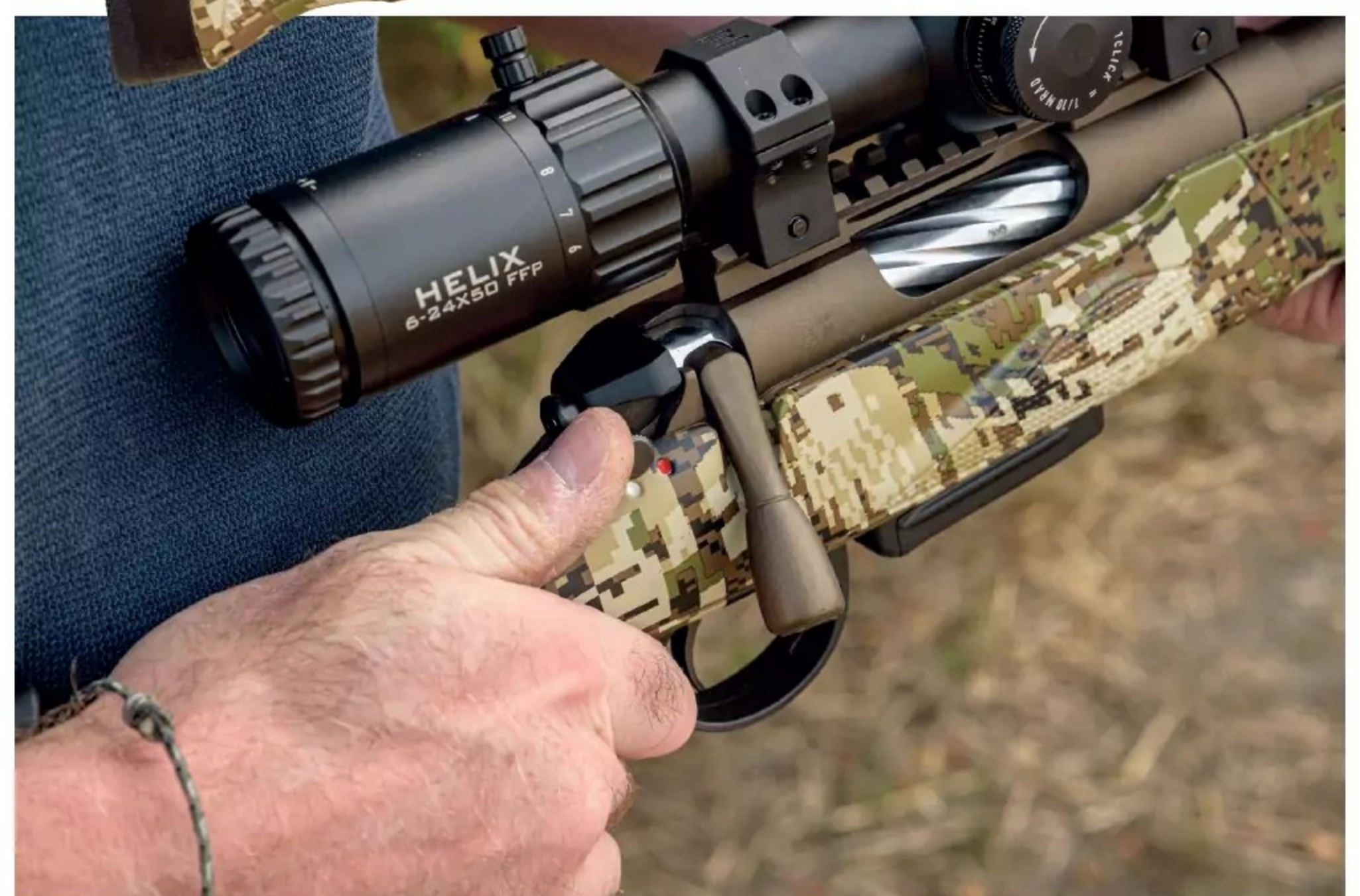
The safety can be operated silently. Note the fluted bolt shaft
