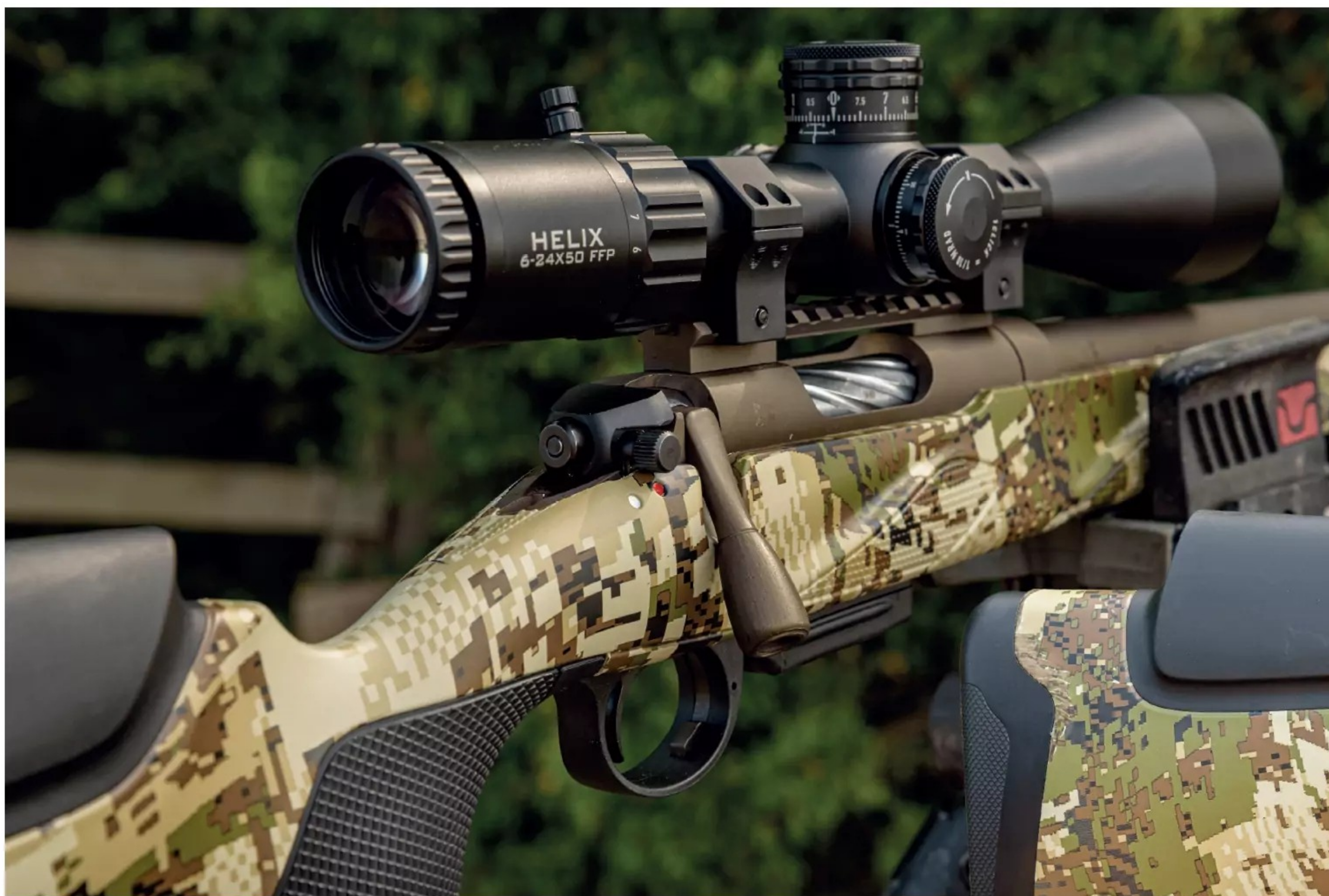
Detail of the bolt handle and the safety catch
