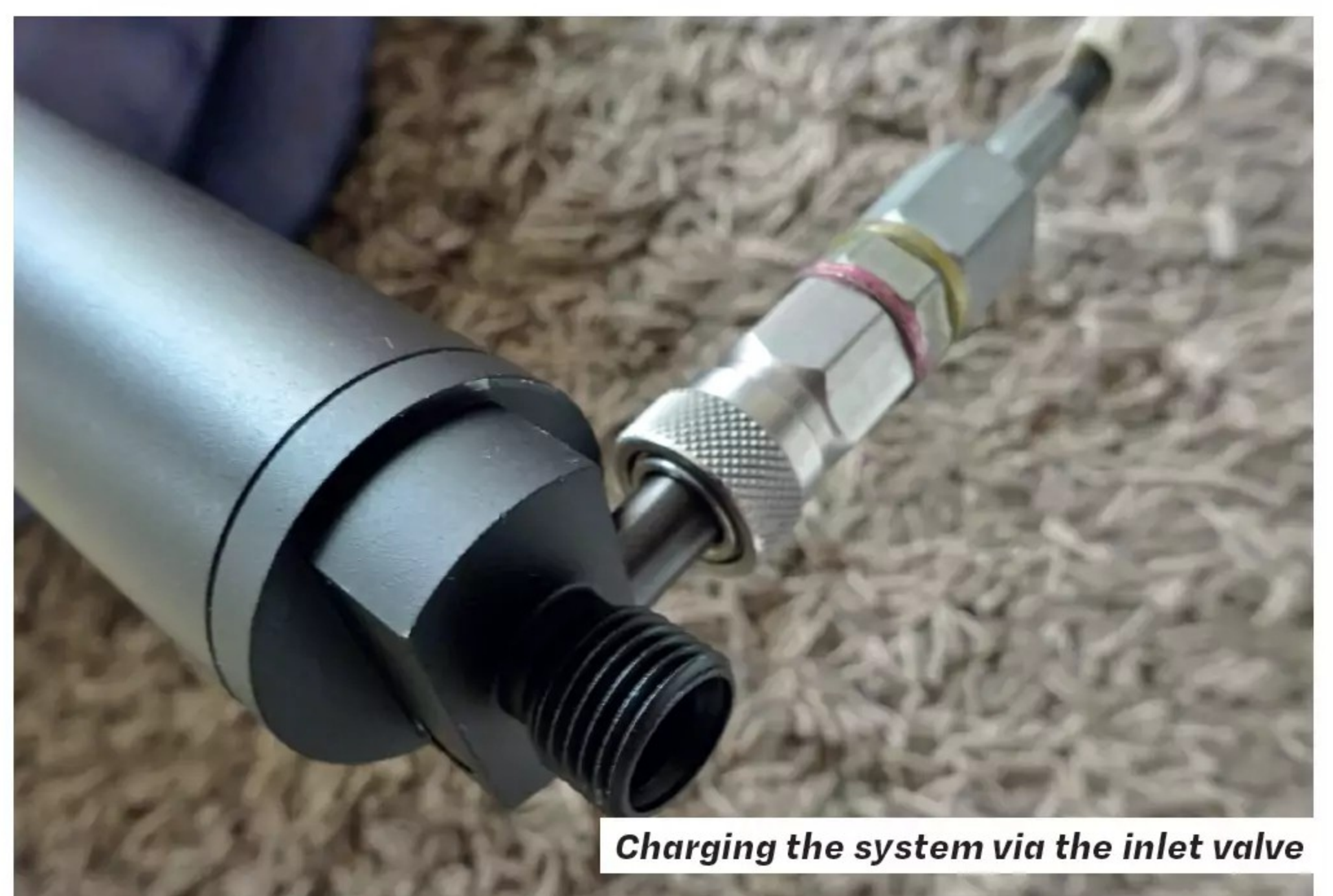
Under the muzzle cap, there's a 1/2" UNF thread and the inlet valve
