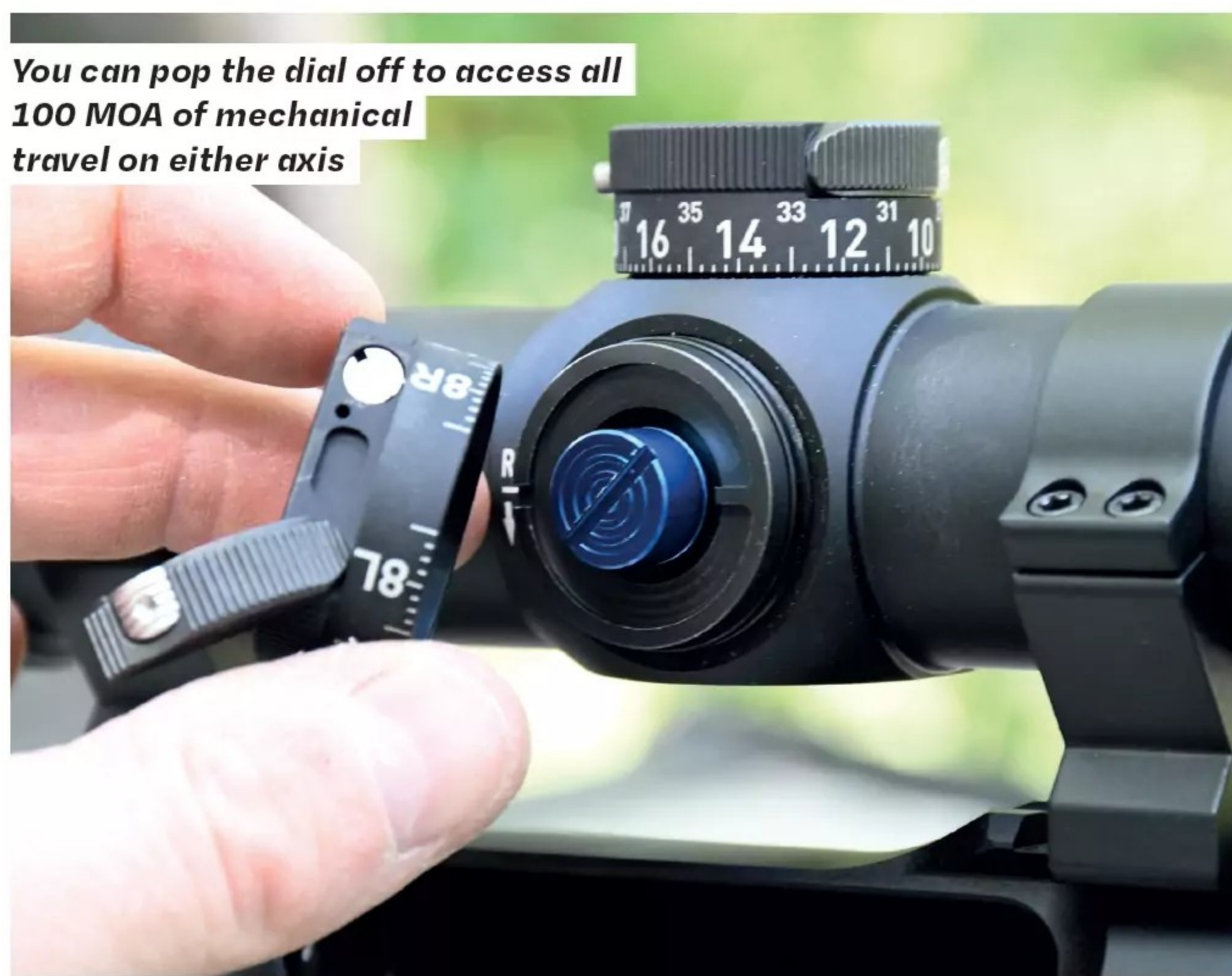
The windage is marked right and left of centre. Note the click values
