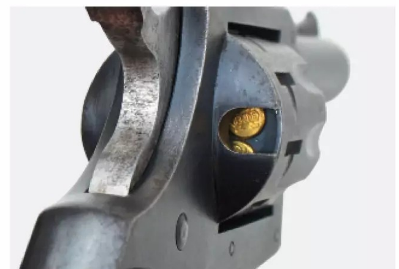
▲ The Model 900 had a combination base pin/ejector rod to simplify loading and reduce production costs. ▼ However, it retained the cutout in the right-side cylinder shield to permit single loading or unloading.
