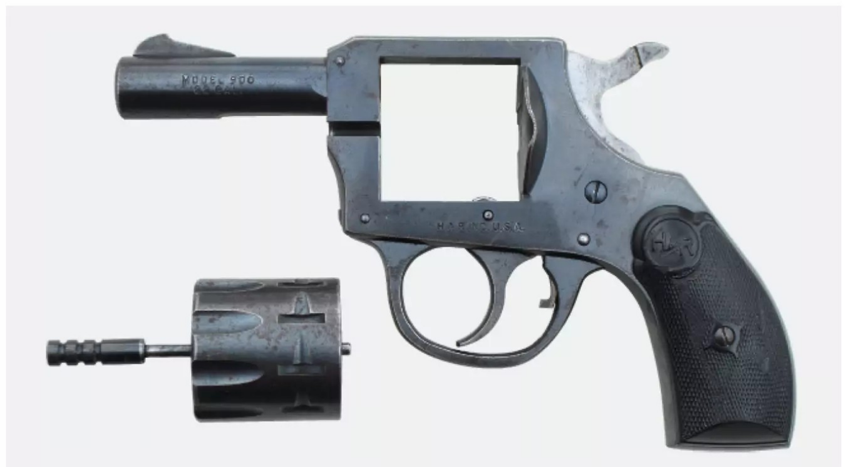
▲ The Model 900 had a combination base pin/ejector rod to simplify loading and reduce production costs. ▼ However, it retained the cutout in the right-side cylinder shield to permit single loading or unloading.
