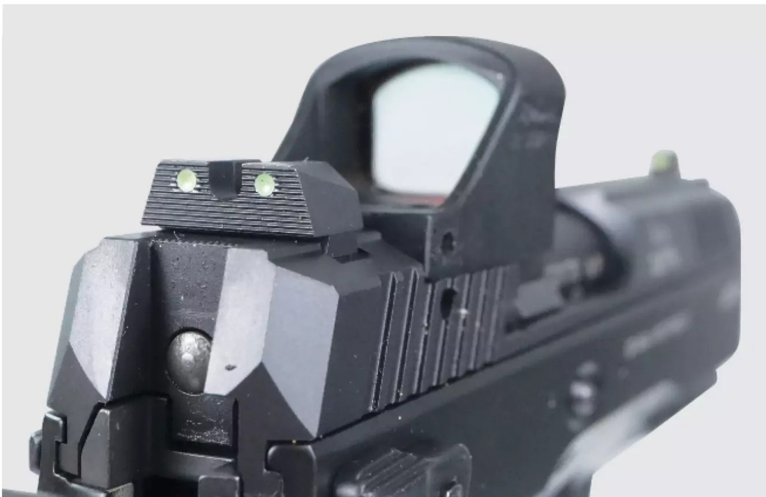
▲ The U-notch rear sight features anti-glare serrations and photoluminescent dots. It will co-witness with most red-dot sights built on the RMSc footprint.
