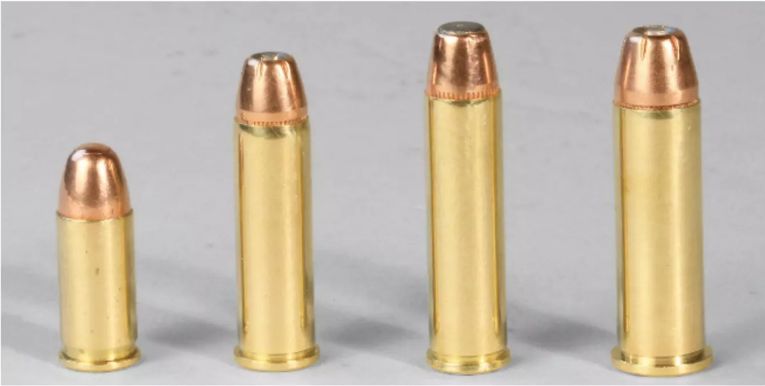
▲ (L.-r.): .32 ACP, .32 H&R Magnum, .327 Federal Magnum, .38 Special. The H&R round was the basis for the .327 Federal, and while less powerful it’s also more shootable than super-light snubbies in .327 or .38.
