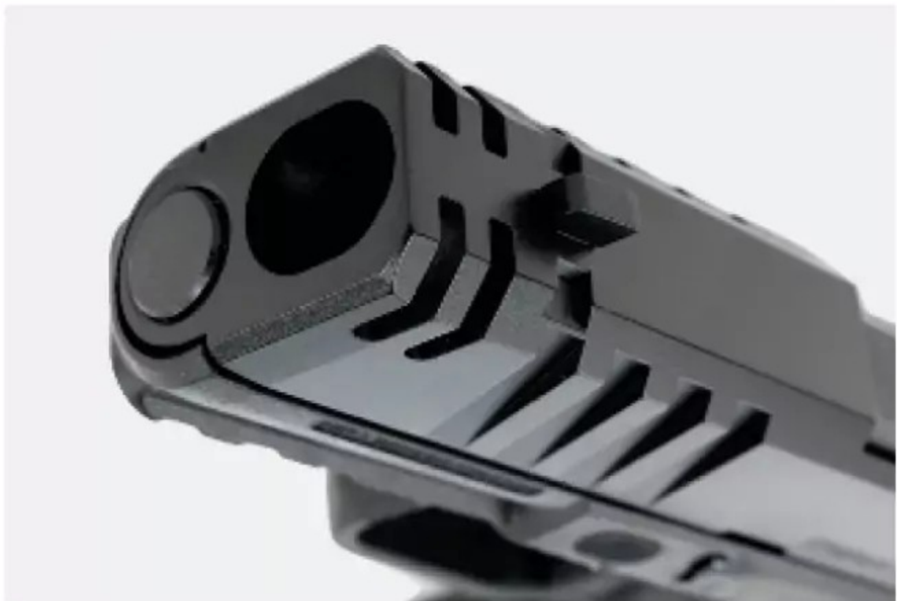
▲ The slide is ported at the front, and the barrel is recessed to direct gases upward to keep muzzle rise to a minimum.
