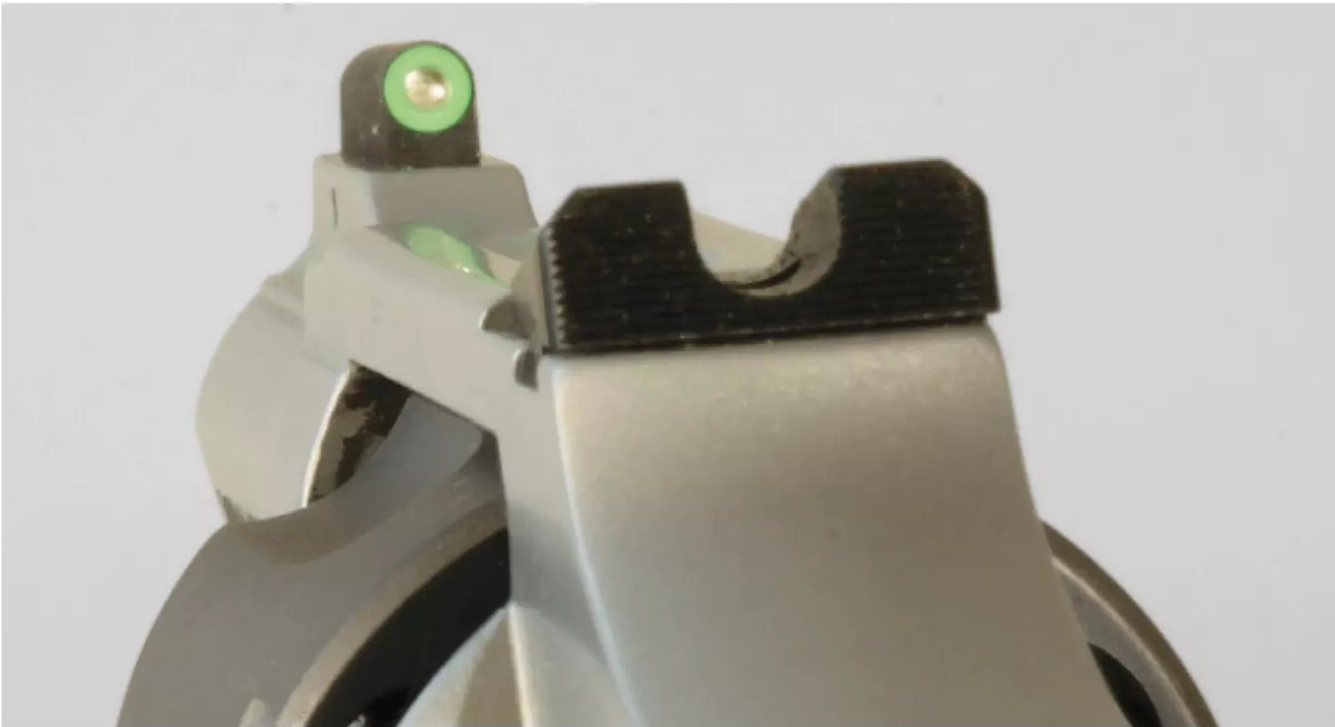
▲ Unlike a lot of snubbies, the 632 UC Ti has real sights: a drift-adjustable U-notch rear and an XS Sights tritium/green-ring front, which is visible in any lighting condition.
