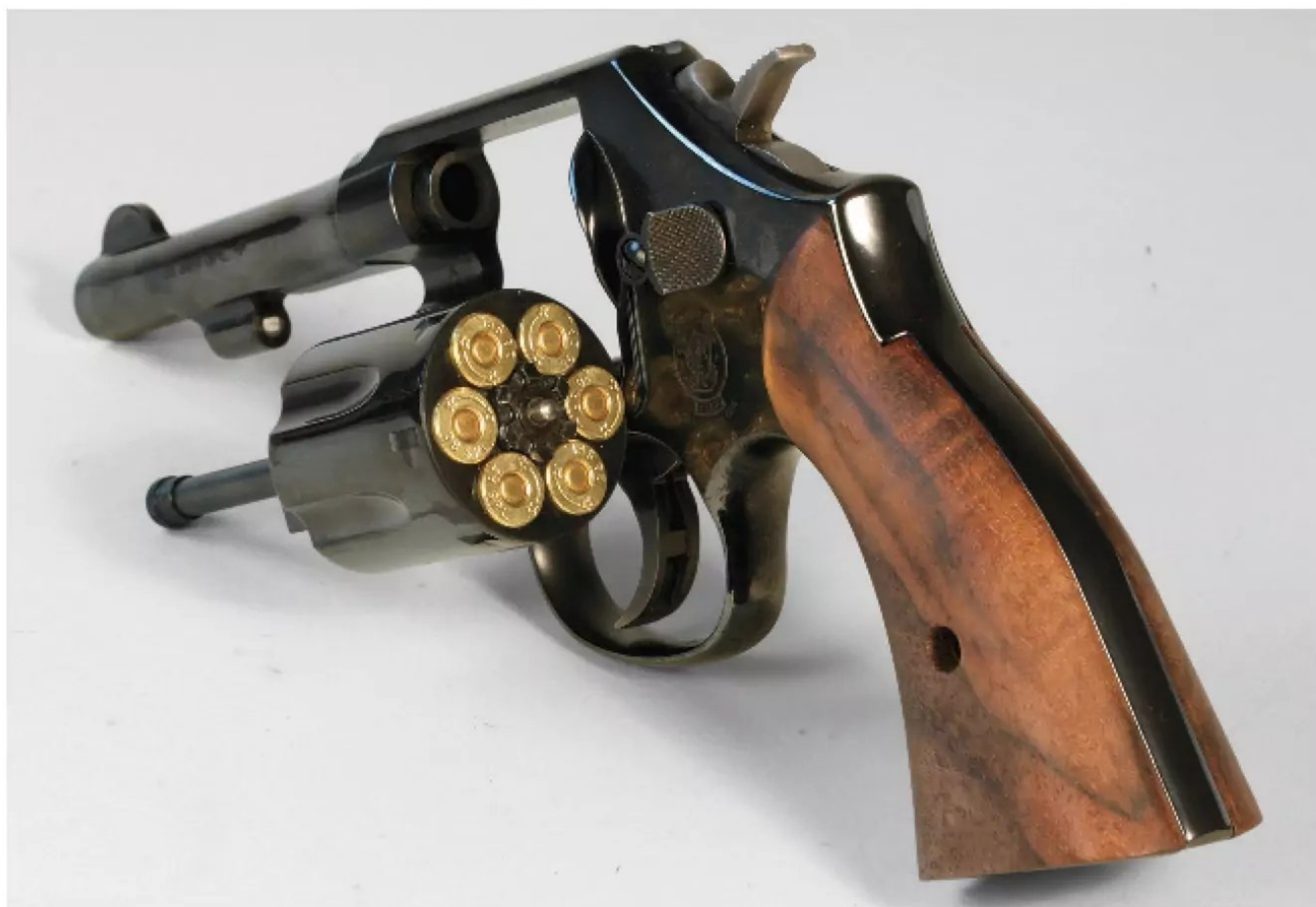
▲ The six-shot K-frame’s grips are of the Magna style, and like those on the “pre-Model 10” they’re unchecked and lack any sort of medallion.
