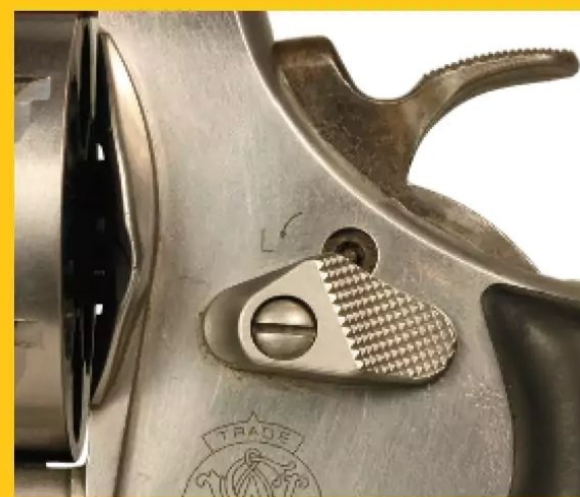
▲ Inserting the provided key into the hole and turning in the indicated direction blocks the hammer from moving.
