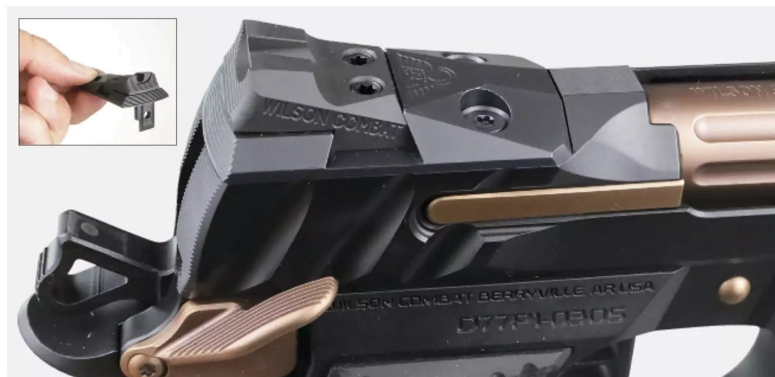
A The integral cover plate and rear sight are attached to the firing pin stop—a design that prevents changes in zero when the sight is removed and replaced. Underneath lies Wilson's pin system for mounting red dots.
