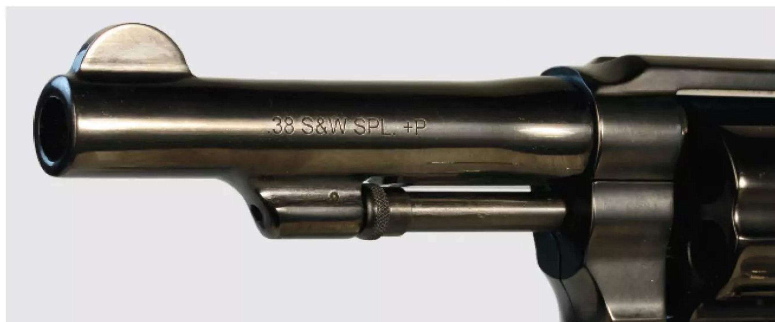
▲ The four-inch barrel is tapered, a throwback to earlier Model 10s, and the round-blade front sight is reminiscent of postwar .38 M&P revolvers.
