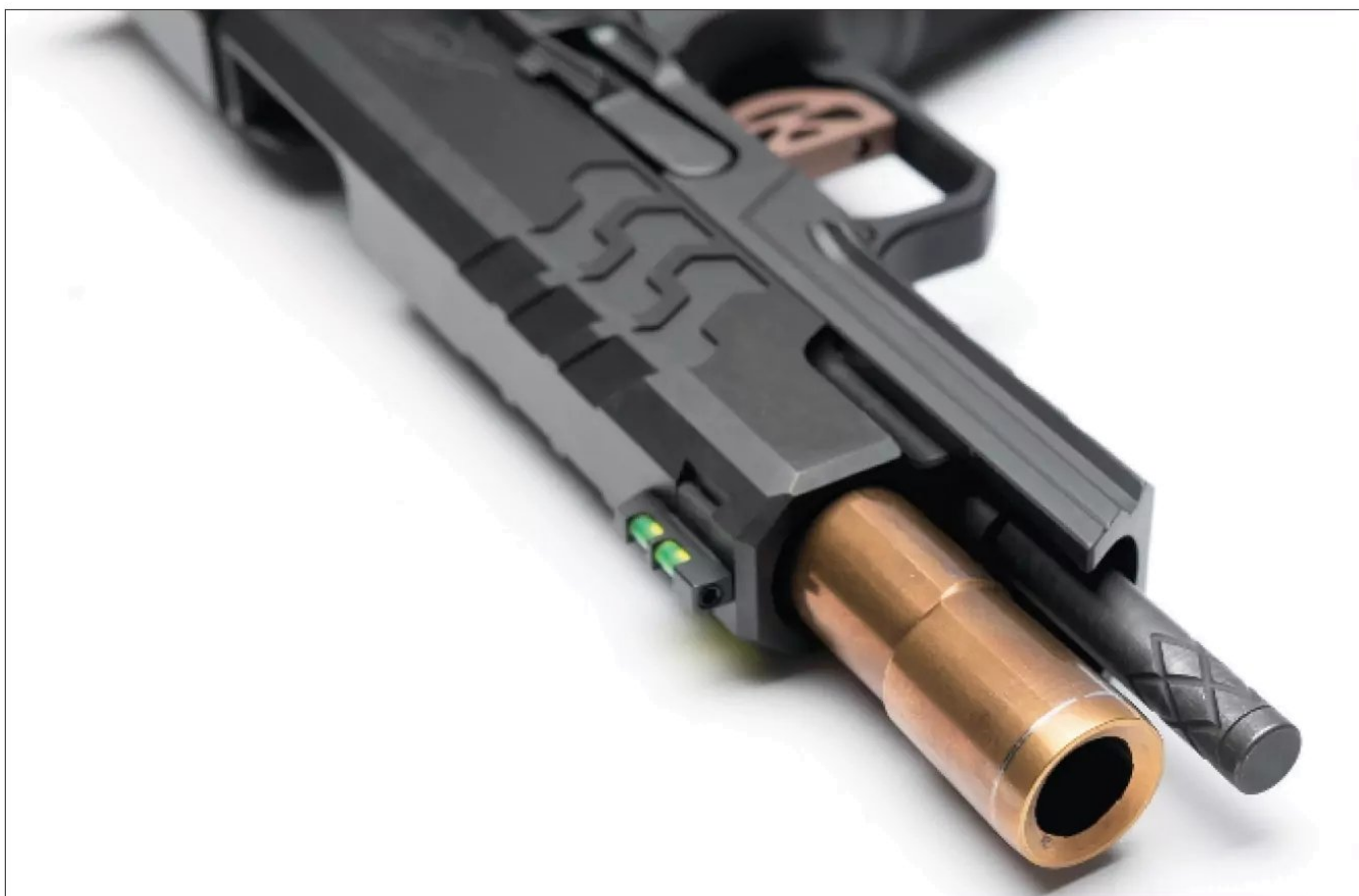
▲ Twisting the full-length, two-piece guide rod locks it in a compressed position for easy removal. The barrel's enlarged muzzle diameter locks into the slide recess without a bushing.
