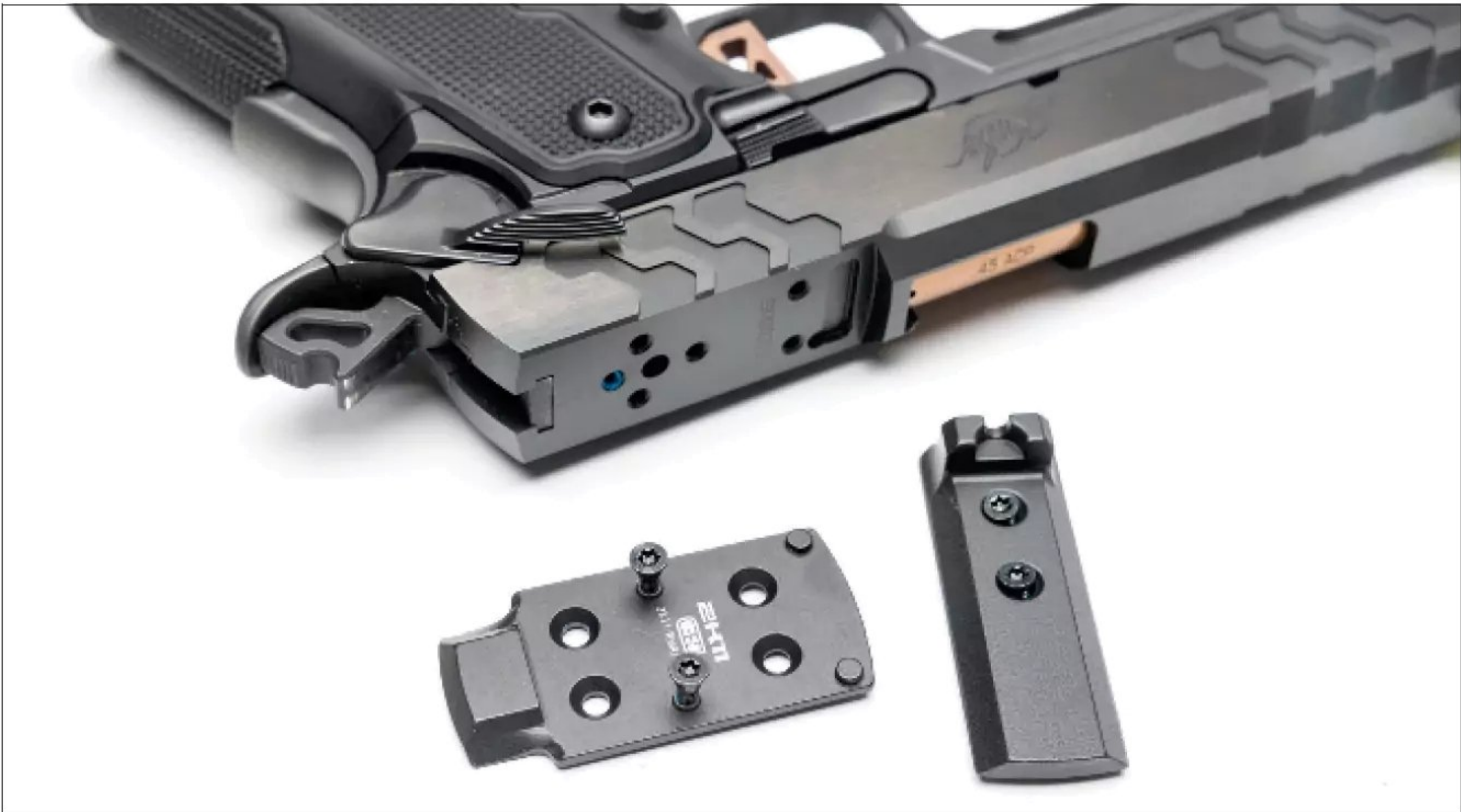
A The optic-ready 2K11 uses an adapter plate (l., not included) to mount a red-dot sight, and plates are available from Kimber. The rear sight is part of the slide cover plate (r.) and is not adjustable.
