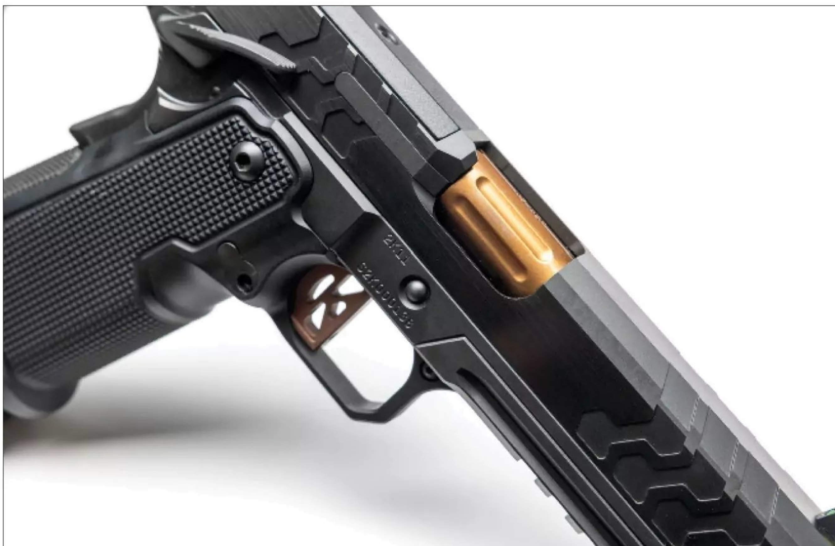
▲ The ejection port is generously cut and flared, and it shows off the fluted exterior of the barrel's chamber. The slide stop hole is treated to an HRT cut on the right side.
