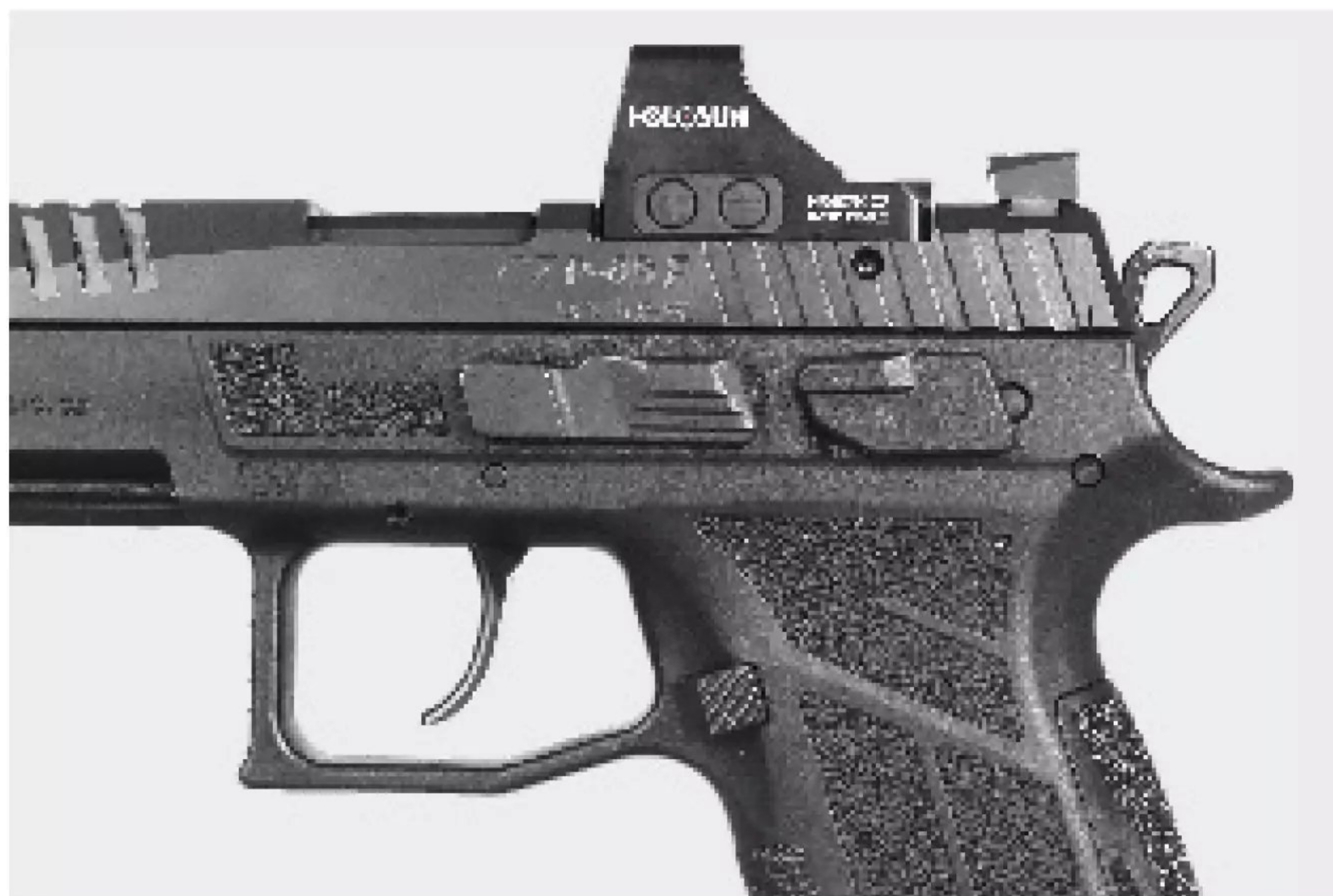
▲ The CZ's controls are easy to use and much improved over earlier models. The slide stop and decocker are wider at the top and offer better purchase.
