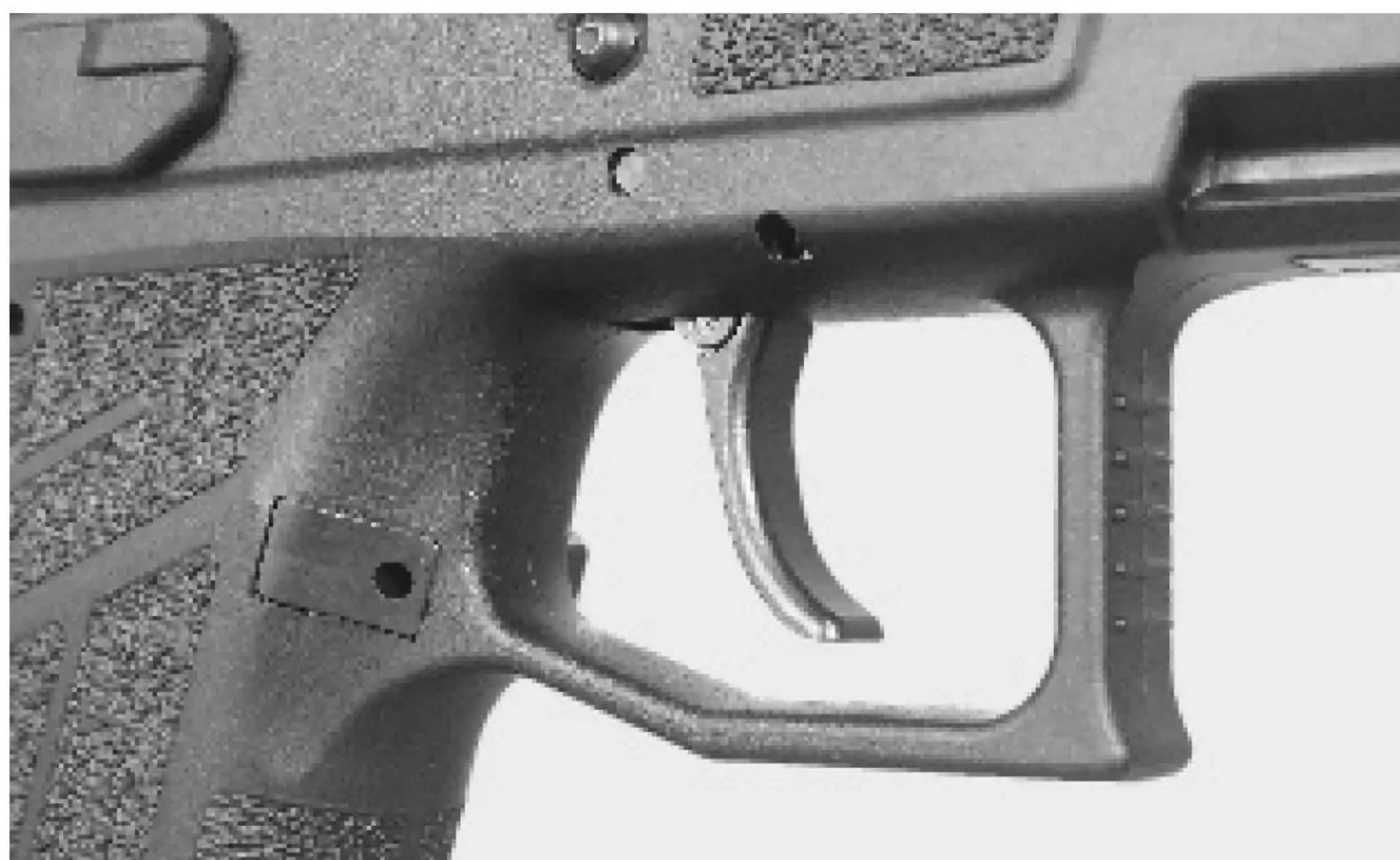
▲ The DA/SA Omega trigger system has a heavy double-action pull of about 11 pounds, but the single-action pull is a more manageable four pounds.
