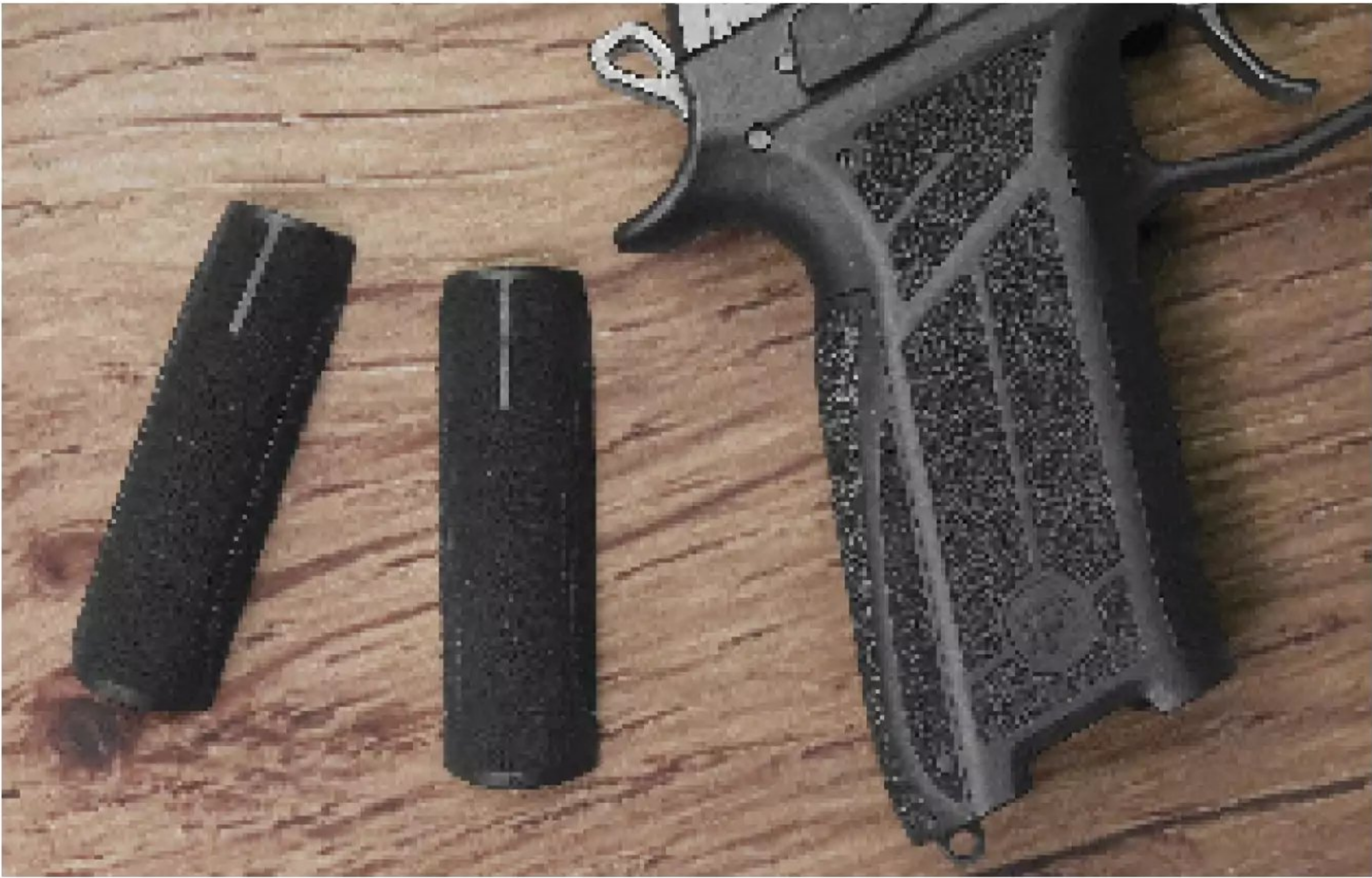
▲ Three backstraps are included, but because you must remove the mainspring and mainspring plug to swap them, the manual suggests you have a gunsmith do the job.
