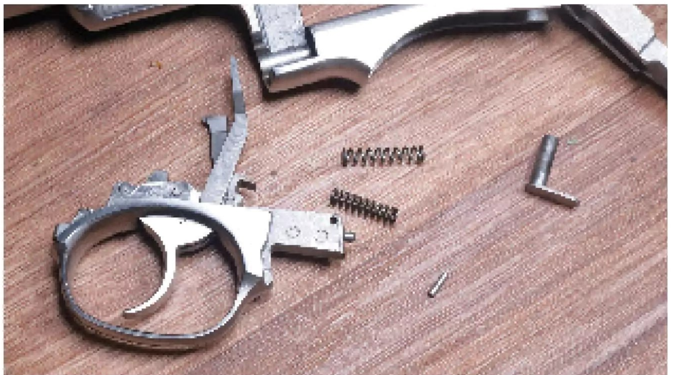
▲ The trigger return spring is behind the trigger and is secured inside the trigger housing. The 15-pound factory trigger is below while the replacement 10-pound Wilson Combat trigger is above. Note the tiny spring retaining pin.
