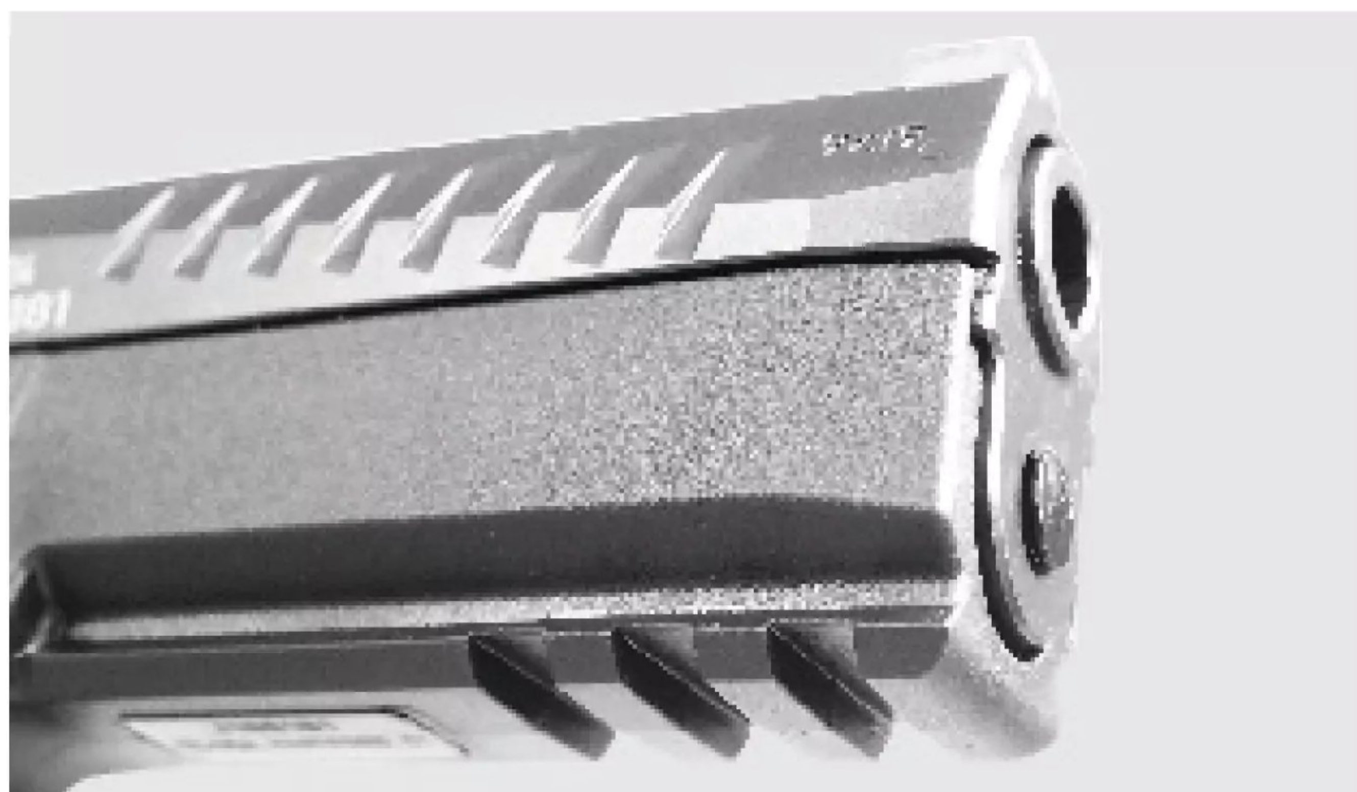
▲ The CZ design puts the pistol's slide rails inside the frame, which reduces bore height and can improve accuracy, although it presents less real estate to grab hold of.
