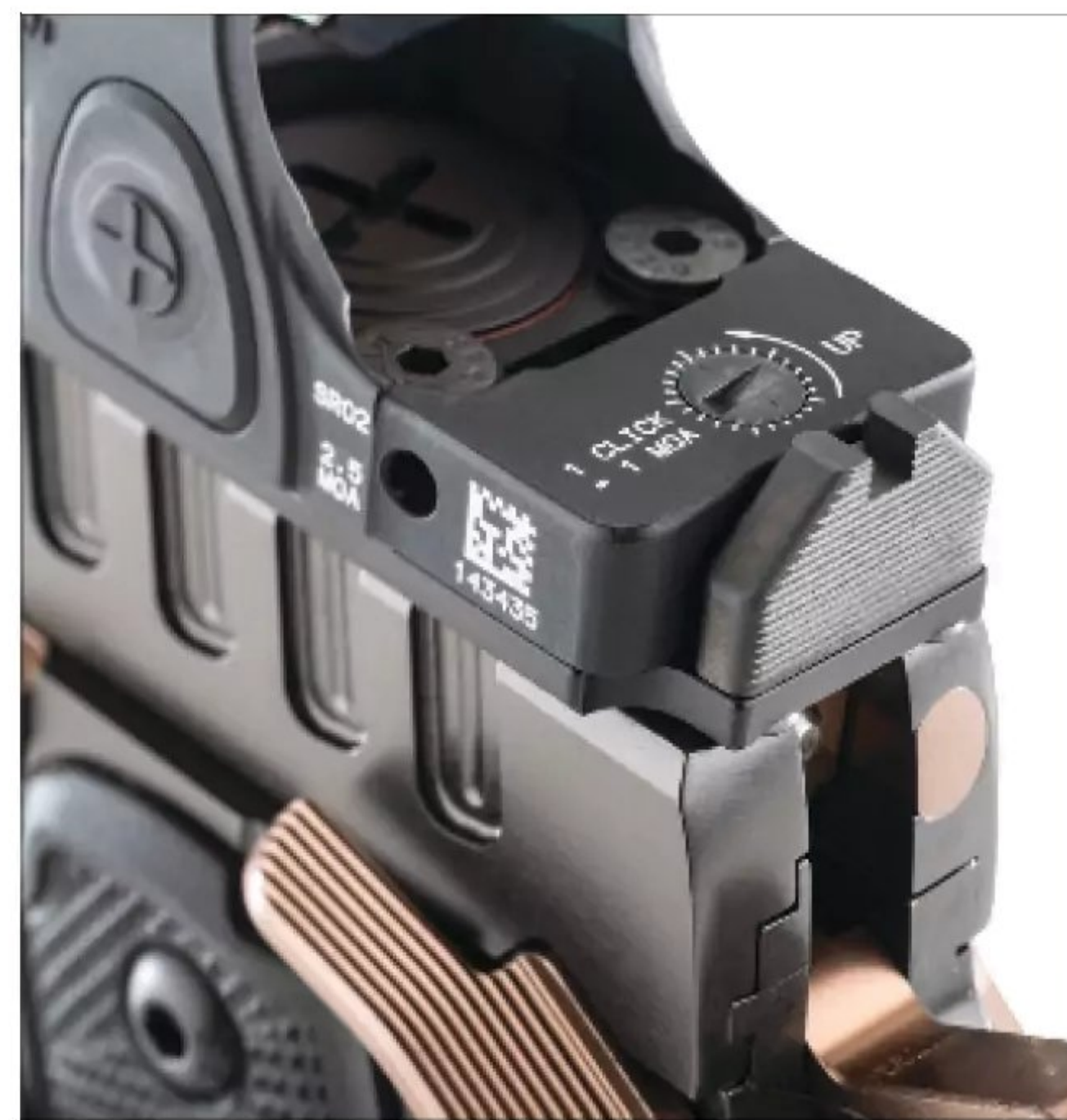
A The Apache's sights are suppressor height and co-witness with this Trijicon red dot—and likely will with many others. The face of the rear is serrated to reduce glare.
