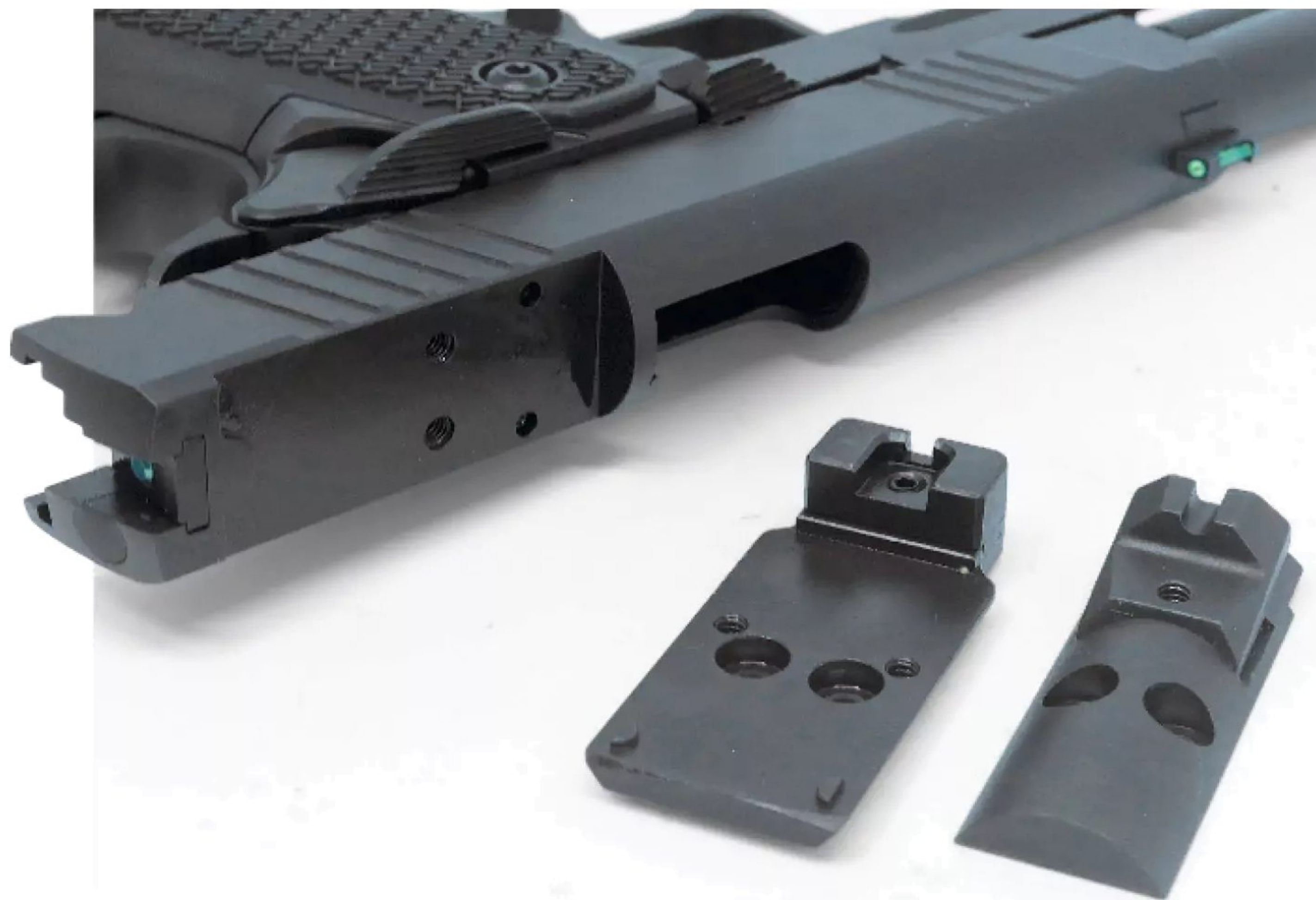
▲ The gun comes with a slide plate that accepts RMR-footprint red dots (l.) and incorporates a rear sight (r.) as well as a cover plate complete with dovetailed U-notch sight.
