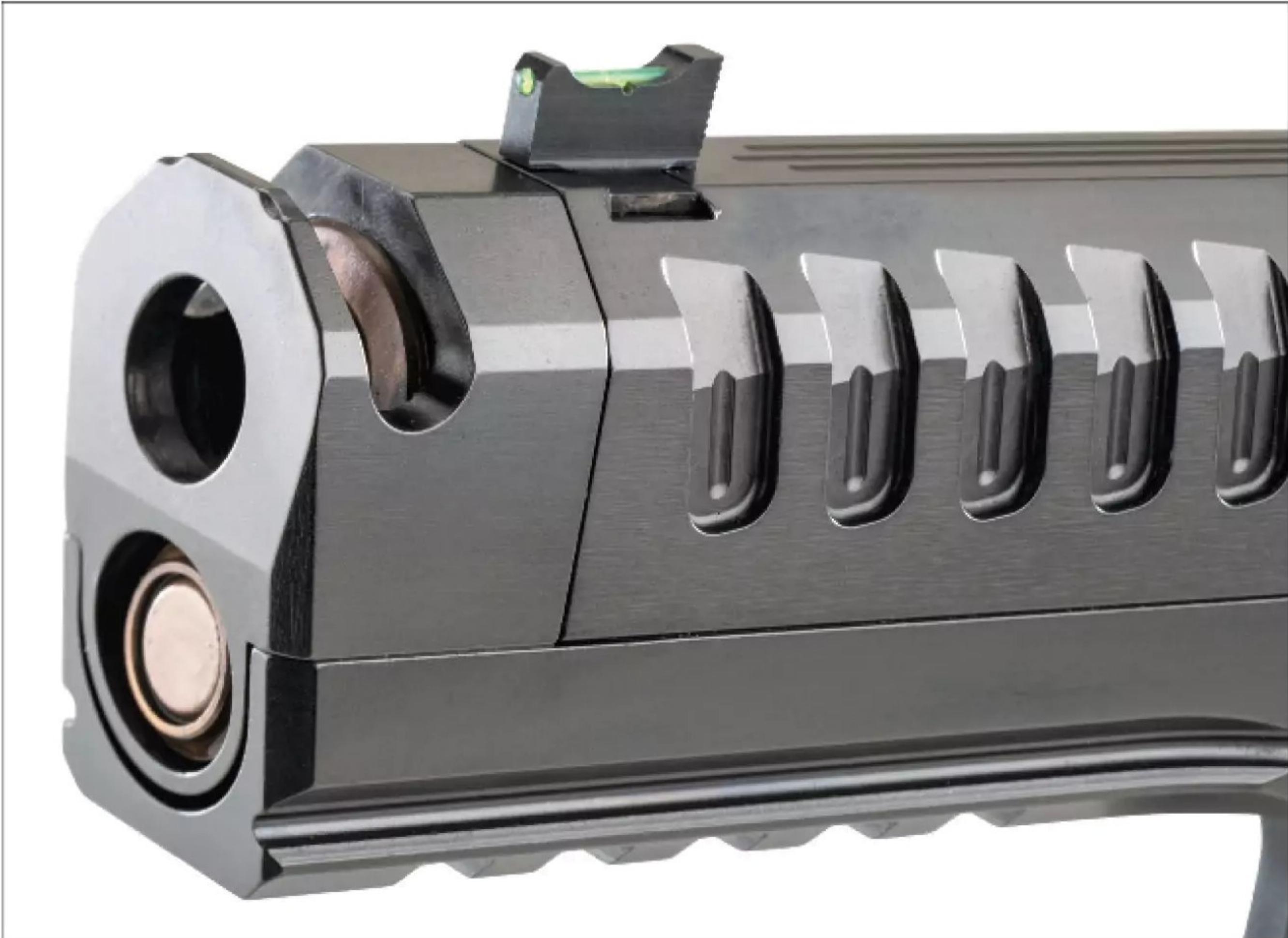
▲ The integral compensator reduces muzzle flip, and the deep slide serrations provide ample texture. The tri-top slide is serrated on top to reduce glare, and the sights are suppressor height.
