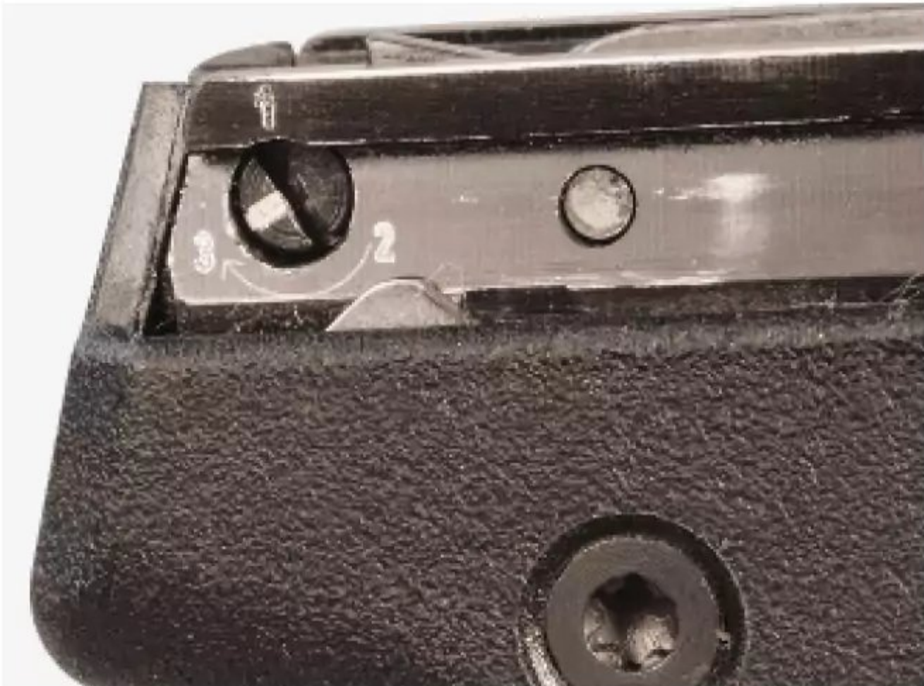
▲ A safety selector allows shooters to customize the gun. Position 1, the factory setting, activates the grip and magazine safeties. Position 2 deactivates both, while 3 keeps the grip safety but disables the mag disconnect.
