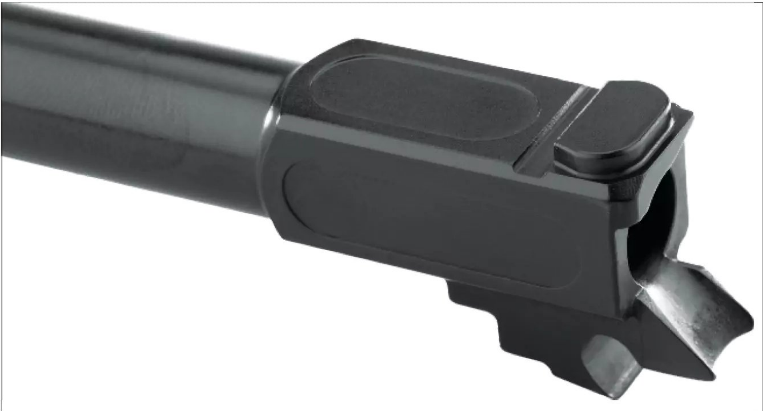
▲ The Bubits-style action locks at the rear of the barrel, resulting in less barrel tilt than standard designs as well as a lower bore axis.
