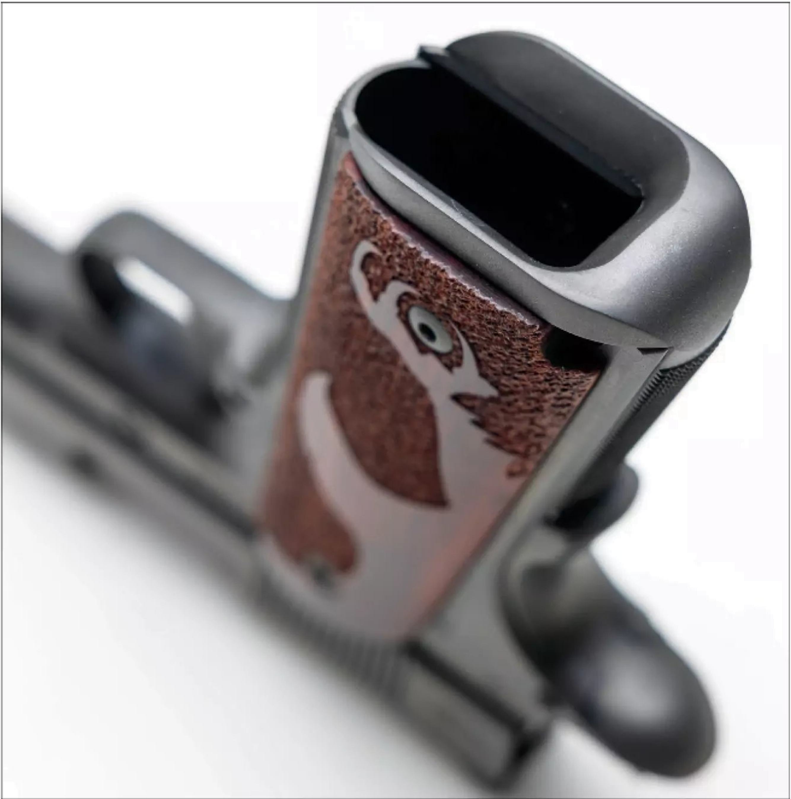
▲ An oversize Nighthawk Custom Falcon mag well was installed, and the frame was contoured to match the bevel.
