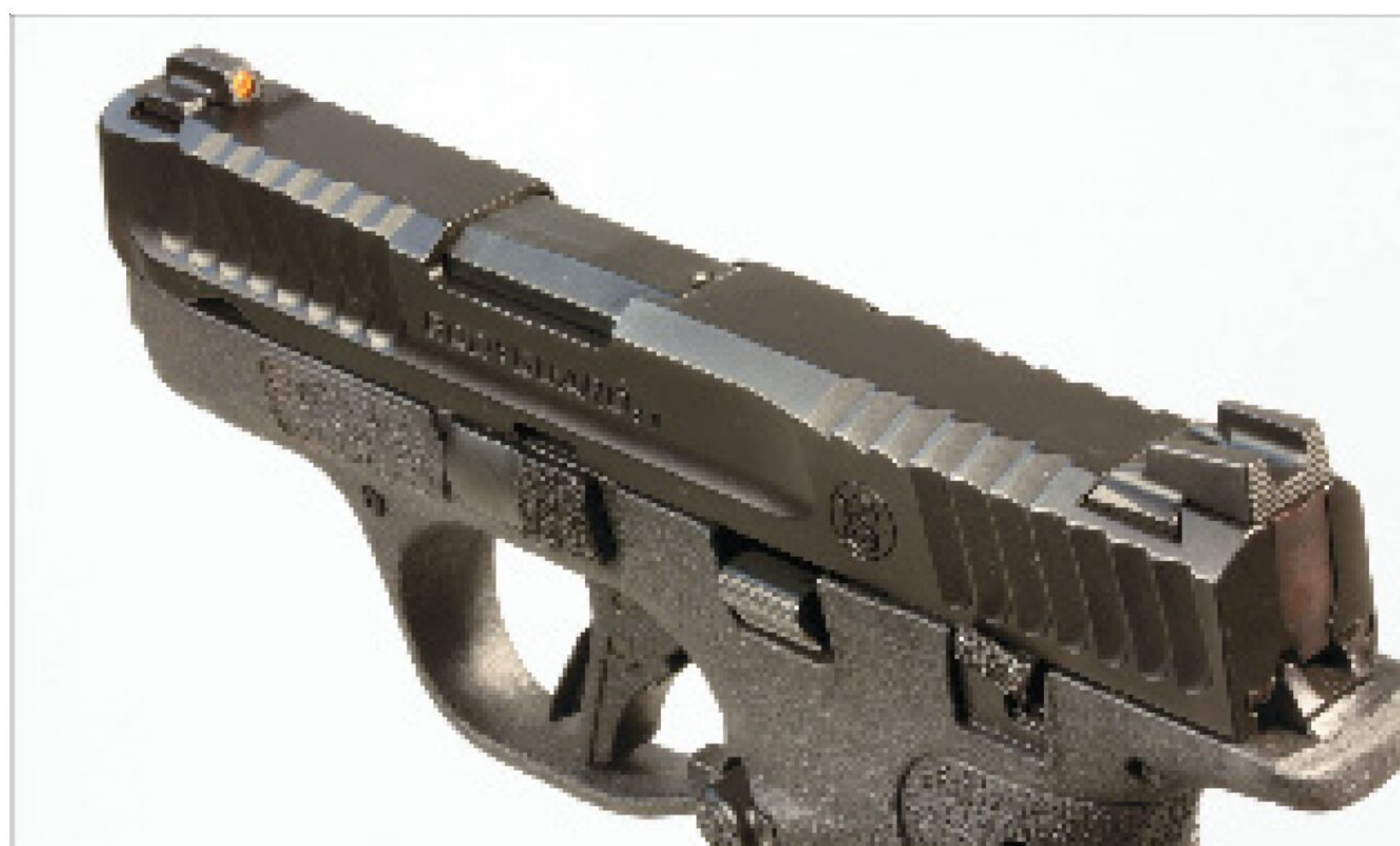
A The slide serrations extend across the transition bevel to the top of the slide for excellent purchase. The day/night front sight sports a big orange dot surrounding a tritium vial.
