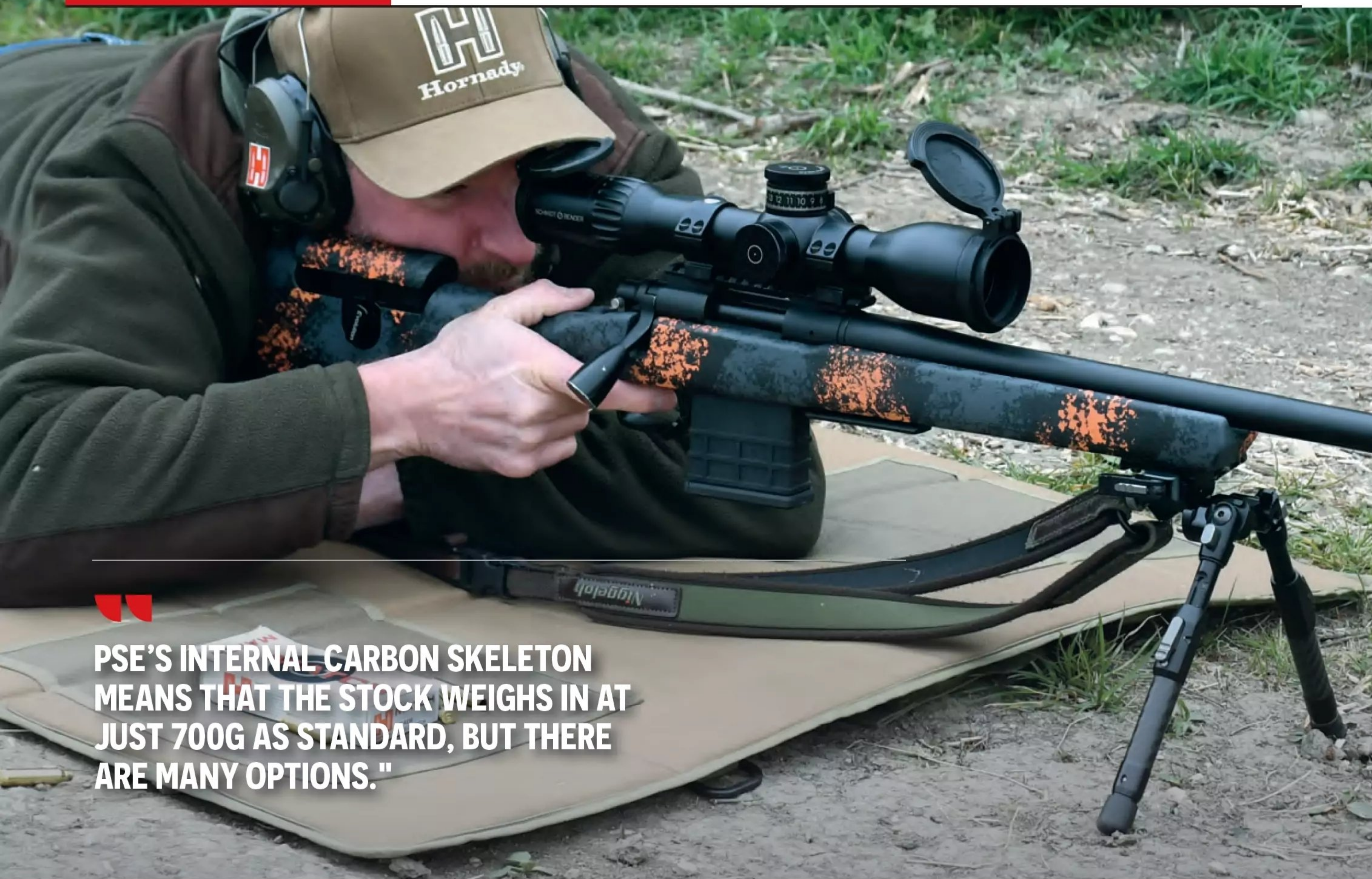
The PSE Evolution carbon-fibre rifle stock
