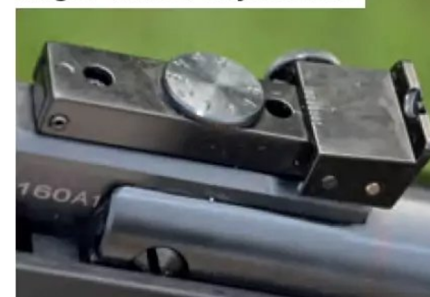
The rear sight is robust and finger-wheel-adjustable
