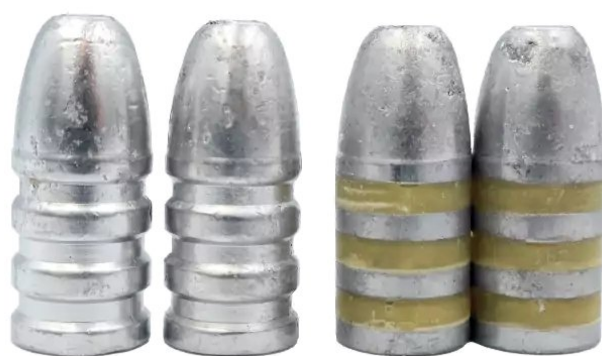
As-cast bullets on the left need resizing and lubricating like those on the right
