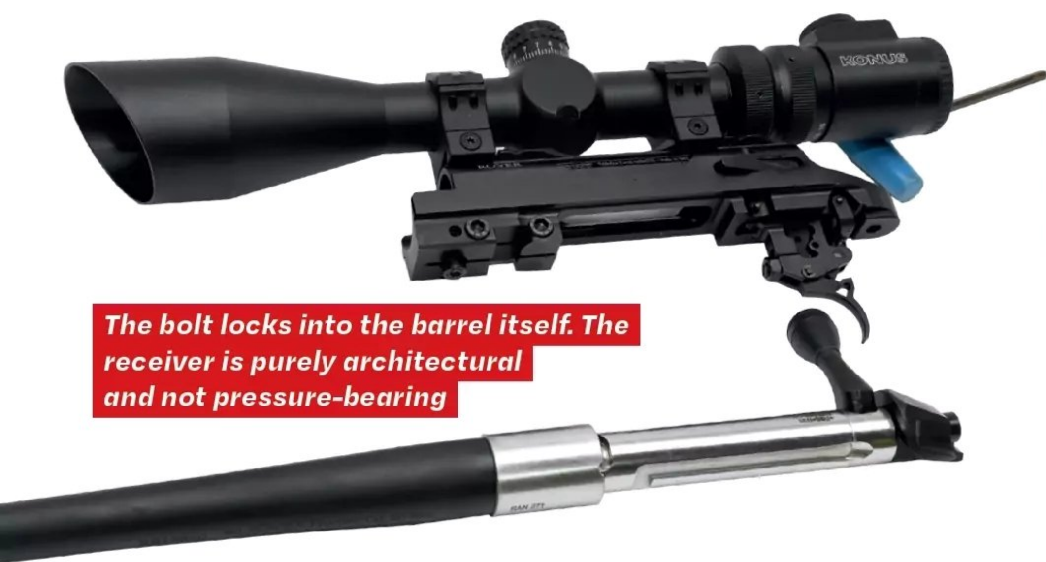
Once disassembled, you can see the flat-bottomed action and precise stock inlet
