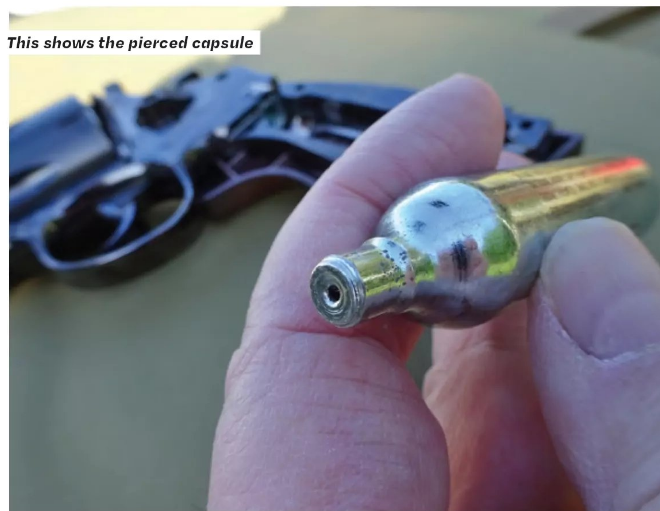
Use the integral Allen tool in the grip to pierce the capsule
