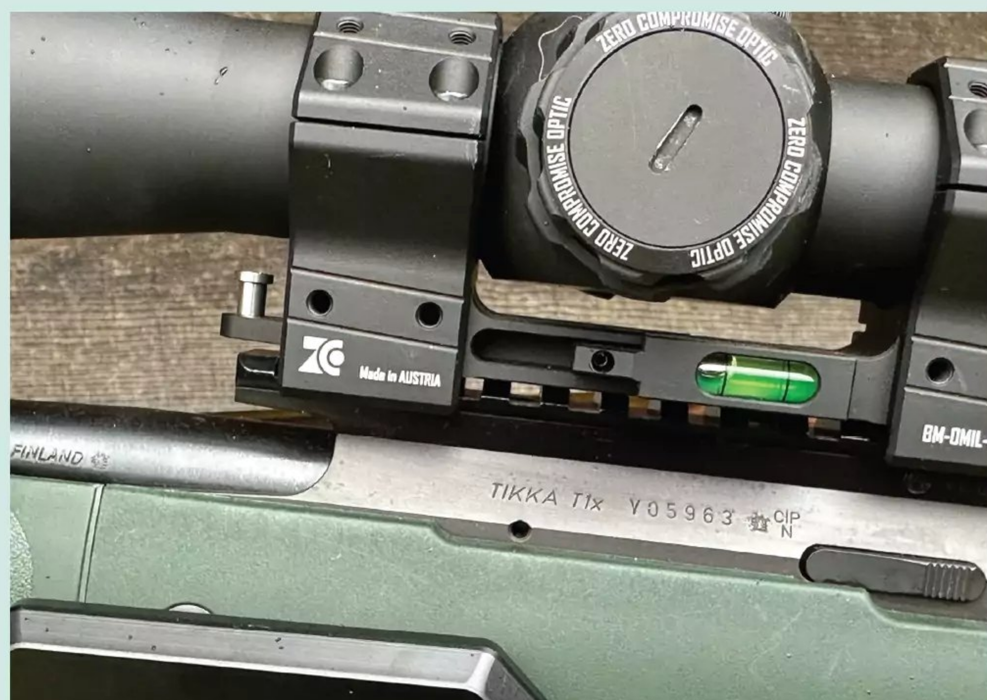
ZCO's mount is an impressive design that comes complete with a mirage-band stud and a swing-out bubble-level
