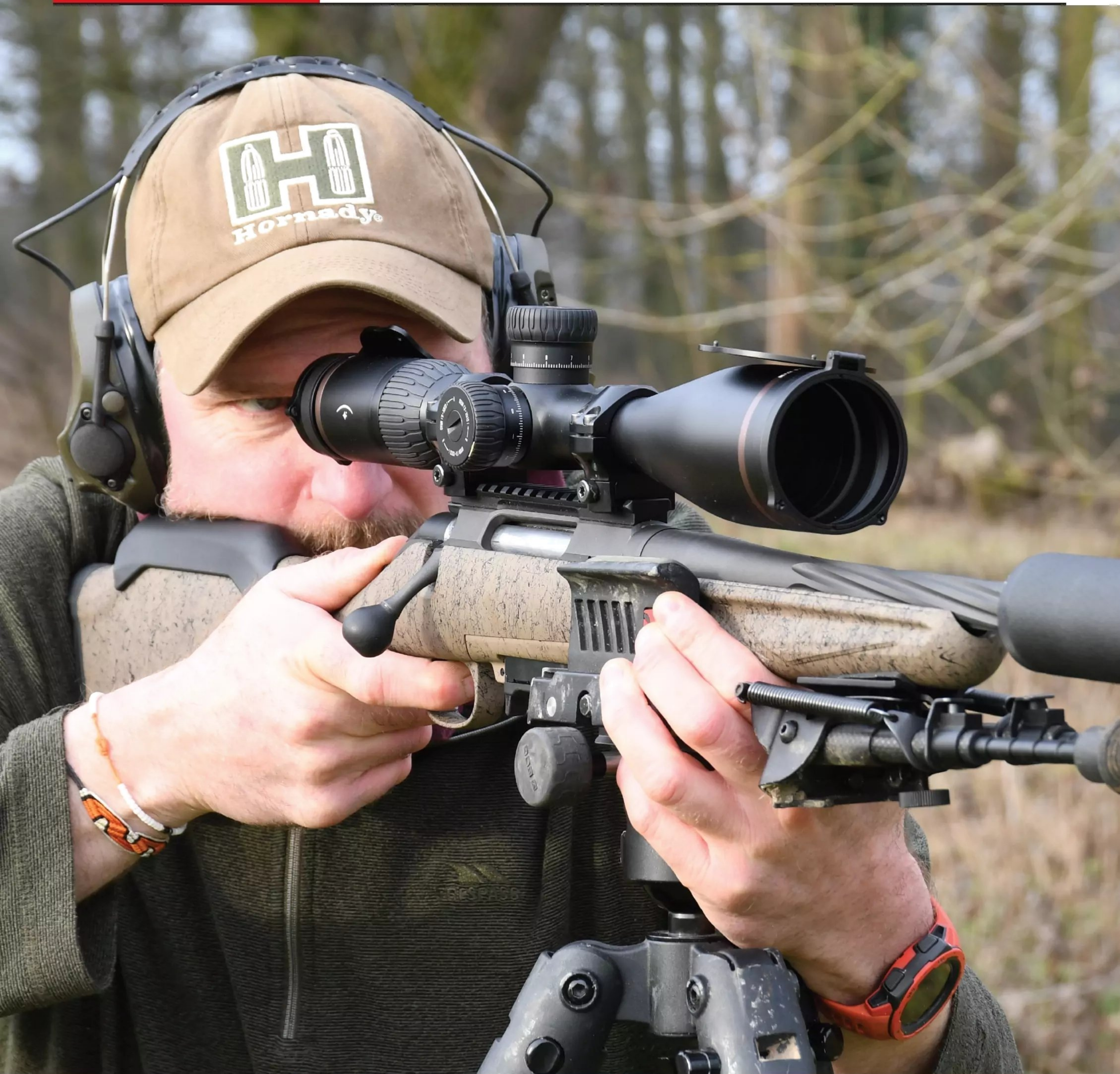
Here you can see the free-floating, fluted barrel
