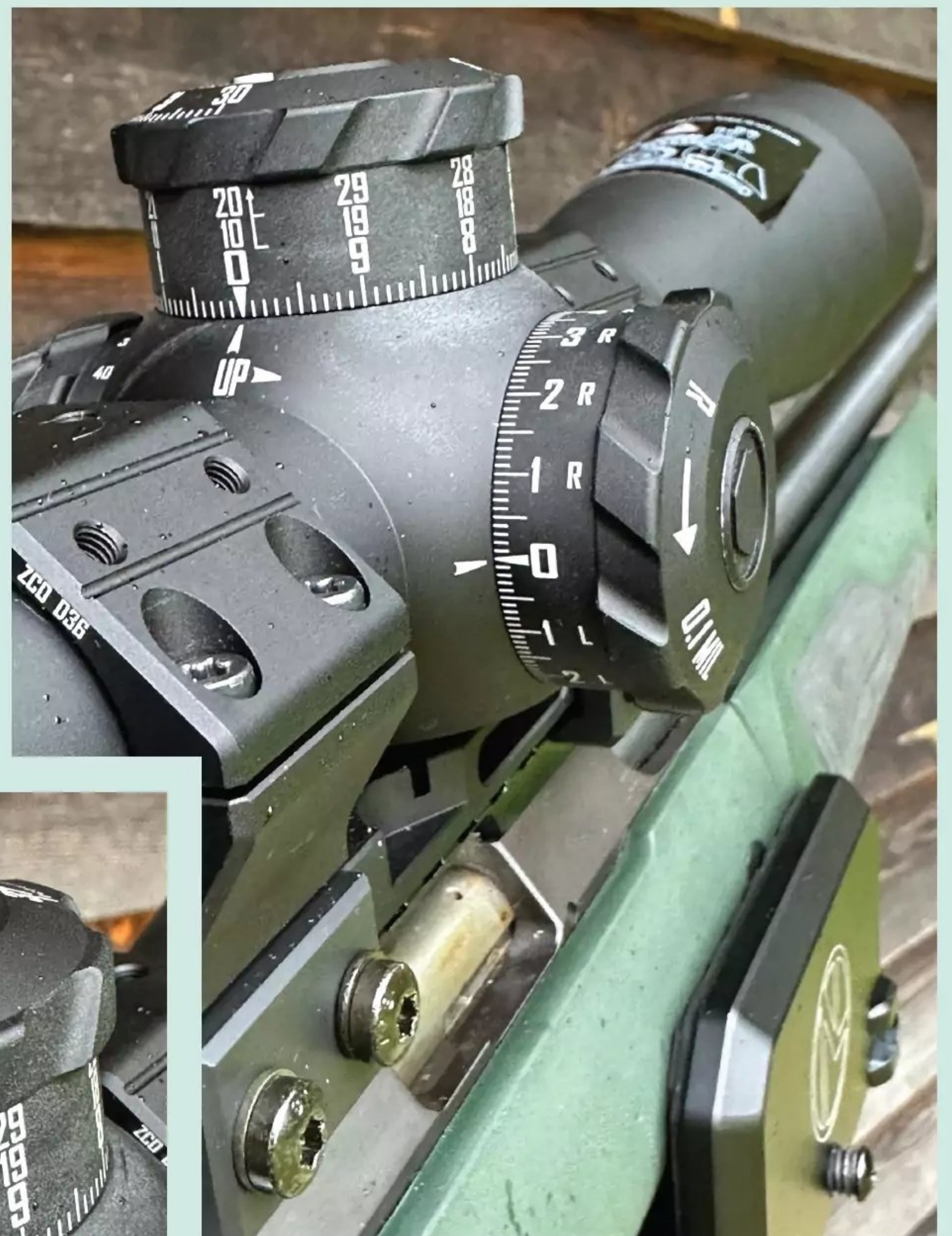
The turrets are well marked and offer audible and tactile 0.1 MRAD clicks
