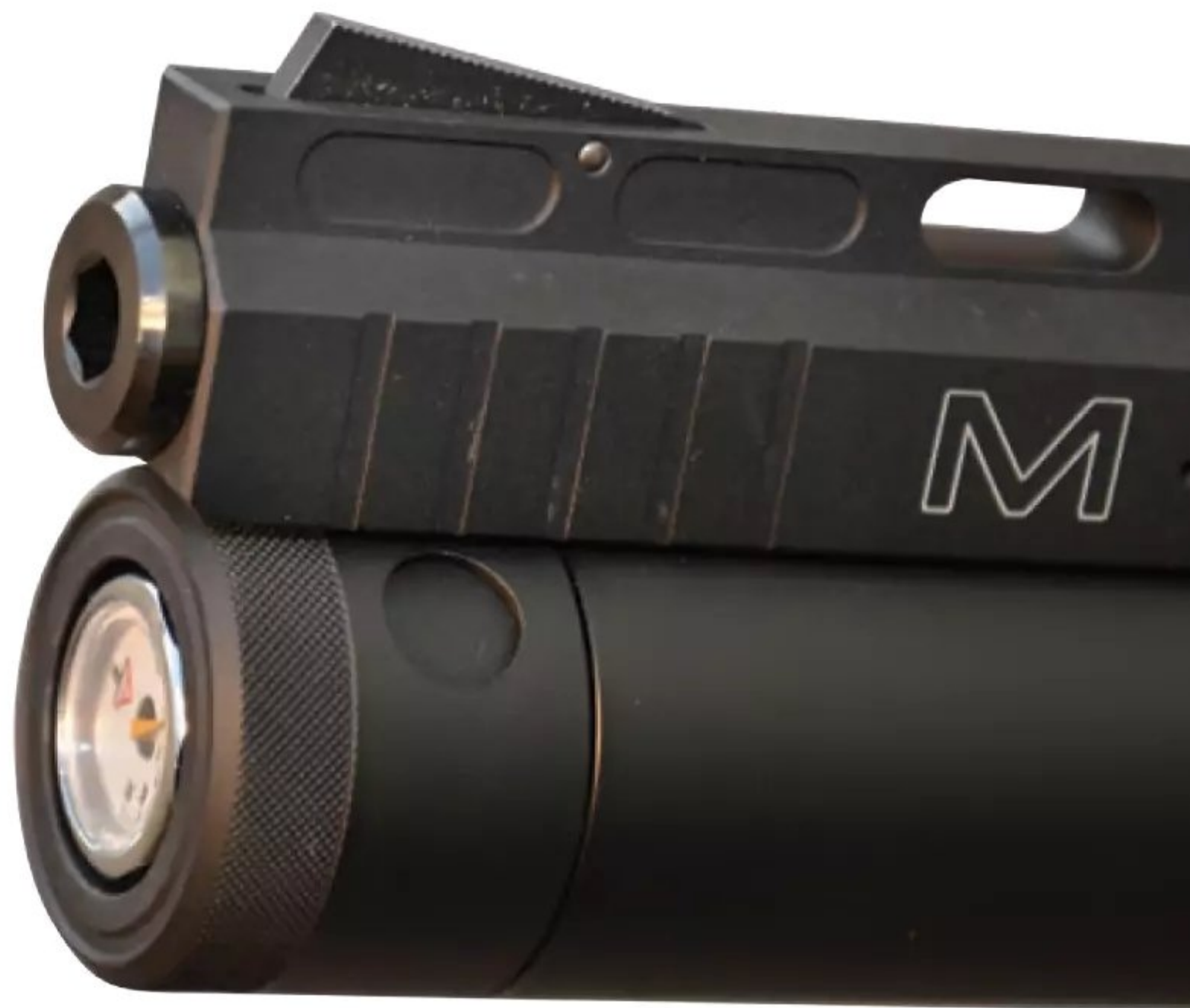
Here you can see the adjustable foresight and the rotating valve cover
