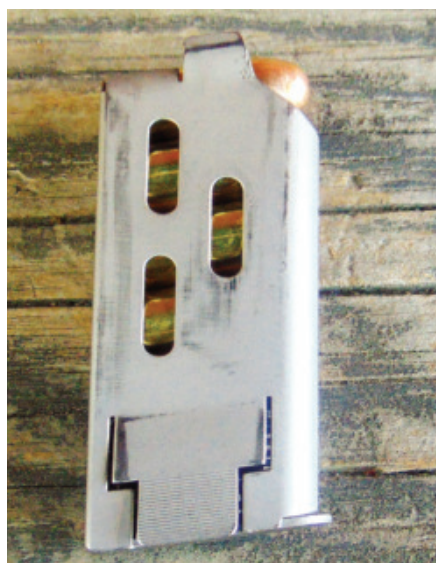
The magazine is removed by pinching both sides at the base and pulling down. Speed reloads are pretty much out of the question! Magazine capacity is four rounds of .45 ACP hardball.
