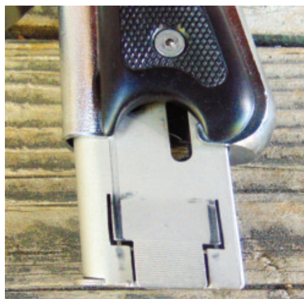
The magazine is removed by pinching both sides at the base and pulling down. Speed reloads are pretty much out of the question! Magazine capacity is four rounds of .45 ACP hardball.
