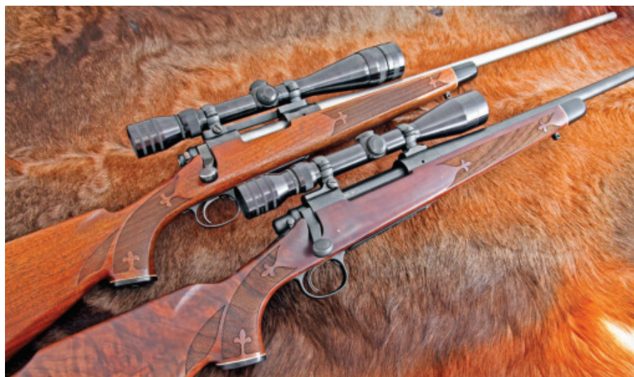
Top is a stainless steel Remington 700 from the mid-1960s re-barreled in .243 Win. Scope is a Redfield 6-18 variable. Beneath it is a 50th anniversary model in 7mm Rem Mag. with Redfield 3-9x40 scope.
