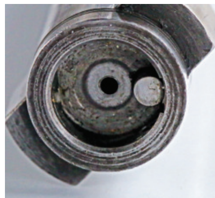
Bolt face of the Remington 700 rifle showing twin locking lugs and spring-loaded ejector. The extractor is a spring clip in the bolt face so there are no cuts in the ring of steel surrounding the case head.
