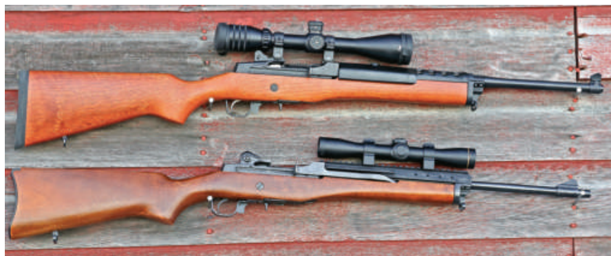
Semi-auto .223 rifles are workhorses around a farm or ranch. This older Ruger Mini-14 (bottom) has a 1-10 twist while the current Ranch rifle (top) has a 1-9 twist.
