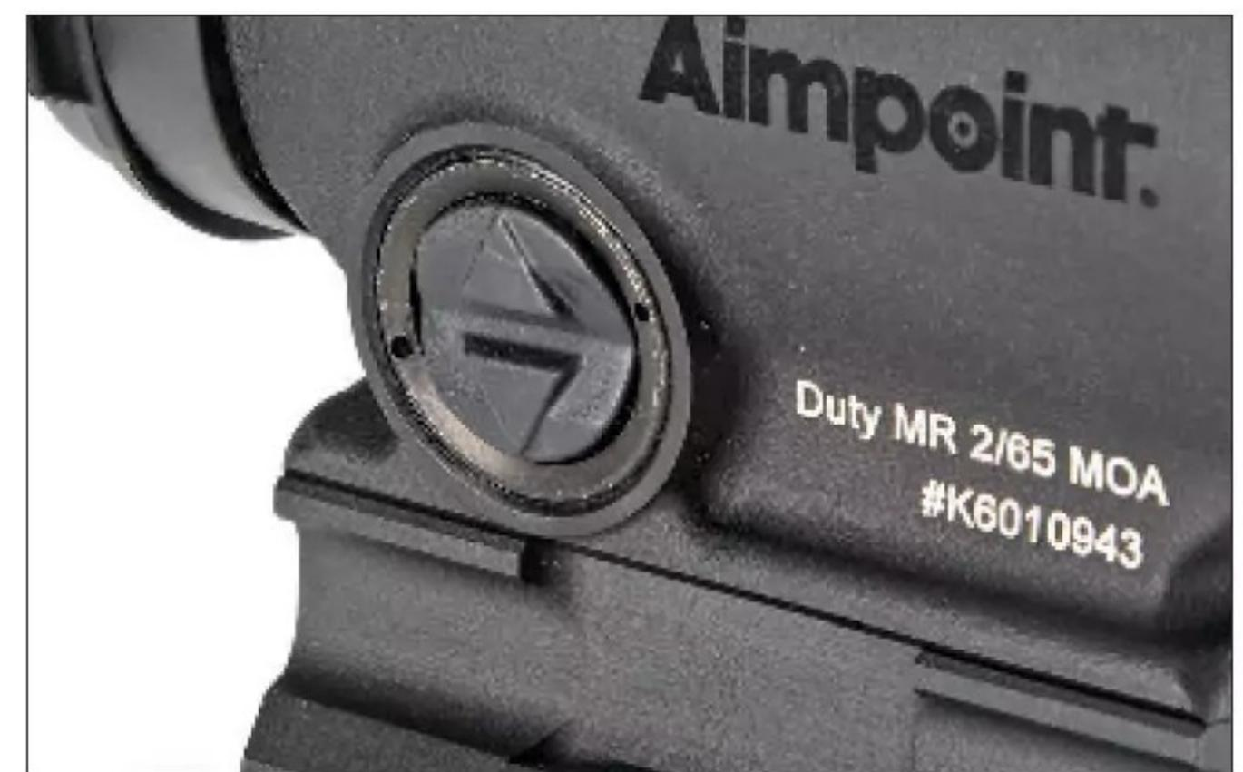
Using the provided tool, the process of zeroing windage and elevation are aided by intuitive "U" and "R" markings with arrows to indicate the direction to push bullets downrange. The reticle brightness adjustment is a tactile control pad on the left side.
