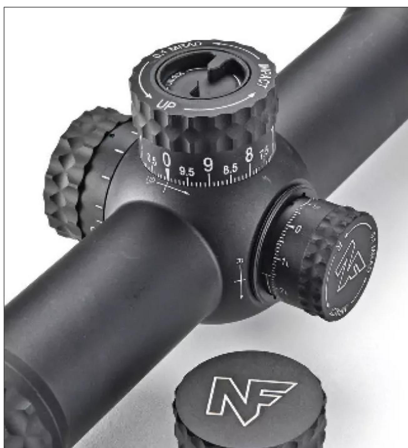
Some NX6 models feature an exposed elevation turret for shooters who prefer to dial elevation adjustments in the field. Returning to zero is quick and aided by a zero stop. Windage turrets are capped.
