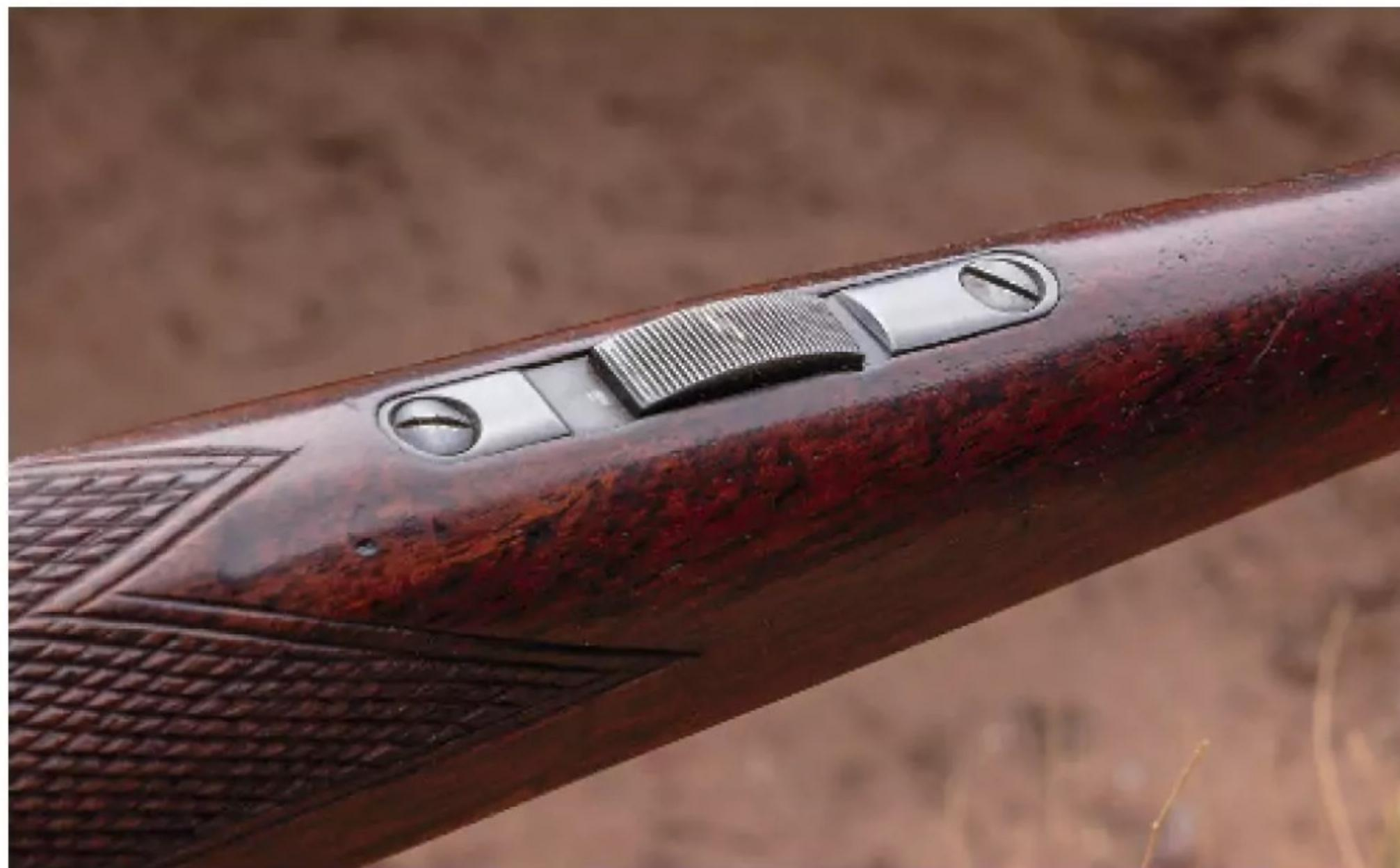
Ahead of the diamond checkering under the forend is a two-position serrated switch. Thumbing it down unlocks the forend and allows it to be separated from the barrel assembly.
