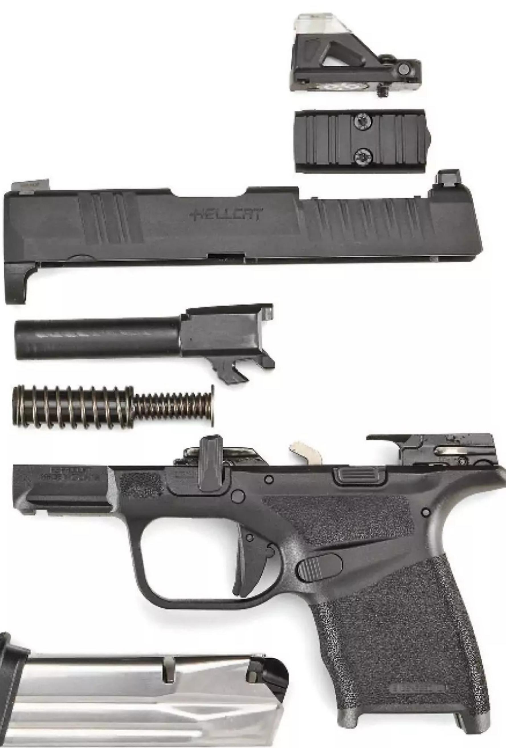
Disassembly of the Hellcat .380 is identical to the 9mm. To remove the slide assembly, rotate the takedown lever 90-degrees up with the slide locked to the rear.
