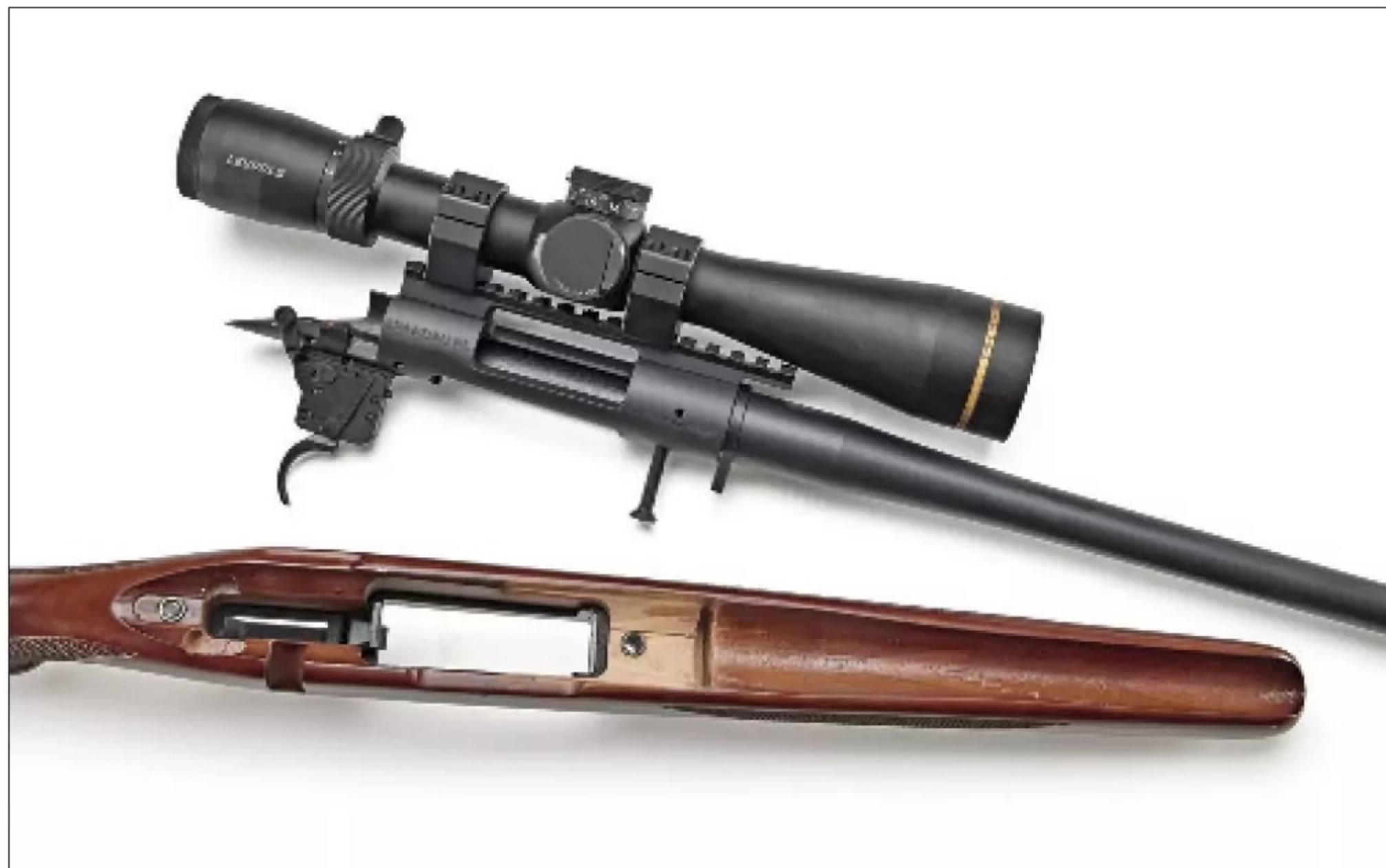
The Spandau RL is based on a standard M700-pattern short action and stock. It isn't bedded, but the action screws are sleeved and front lug stress relieved. The barrel does not contact the stock.
