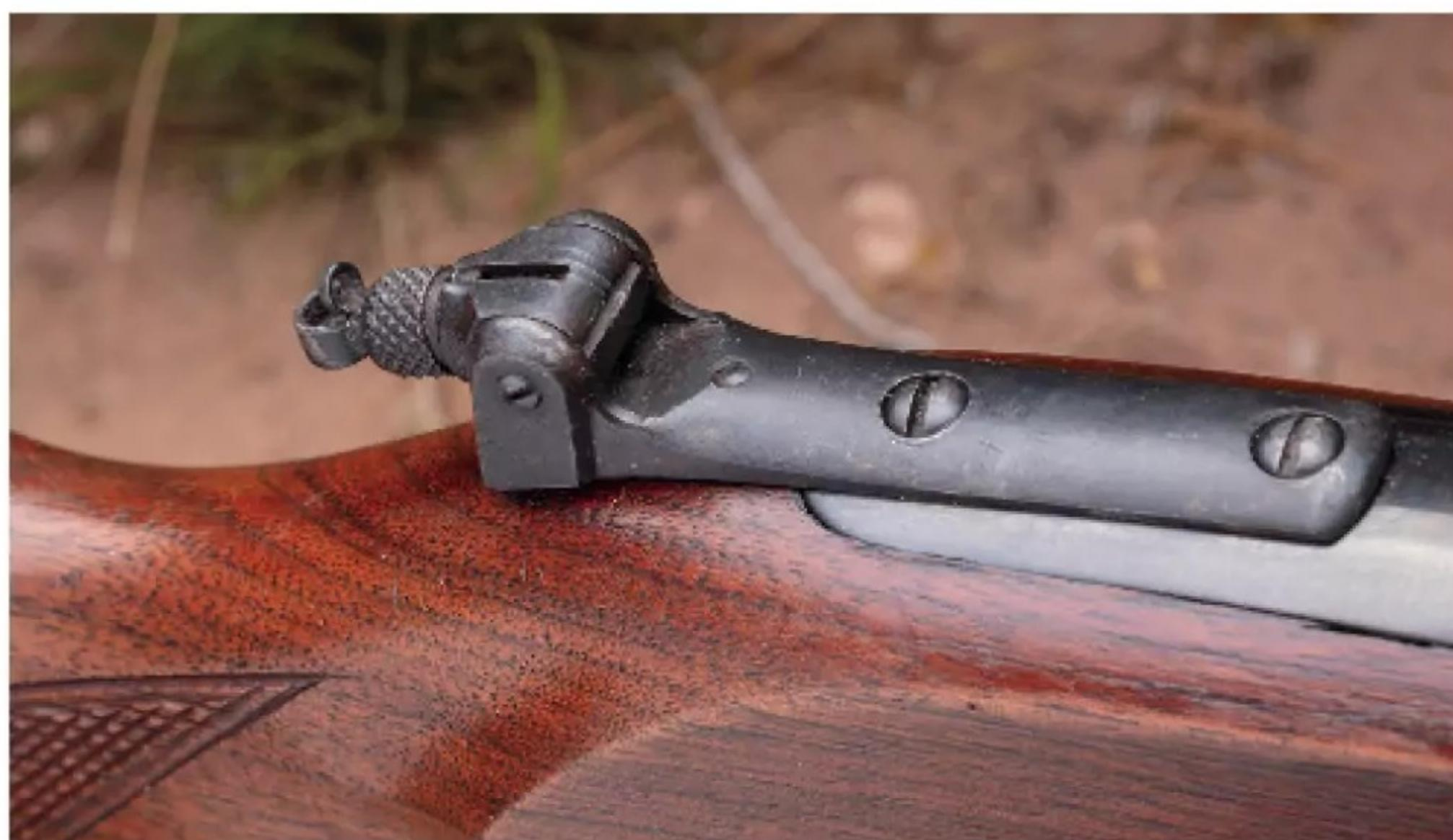
One of the popular upgrades of the era was the addition of a tang sight. A Lyman combination folding sight with two-aperture system was mounted to G&A's Model 1899 test rifle.
