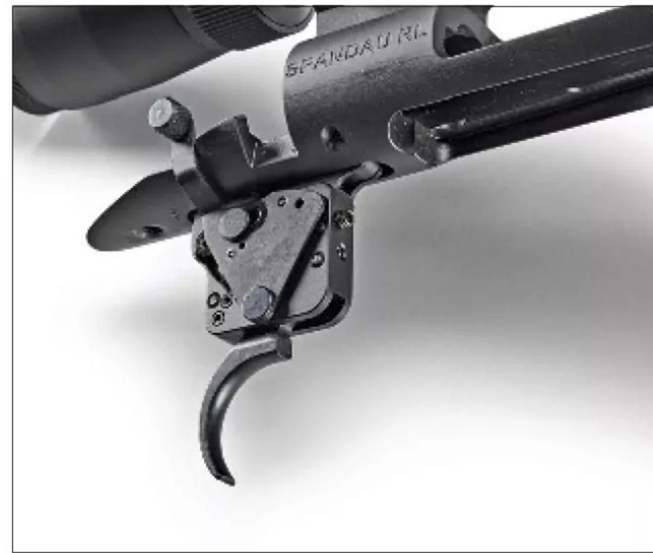
The trigger is patterned off of the M700, meaning that it can be replaced with an aftermarket unit. The factory trigger averaged at just less than 3 pounds.
