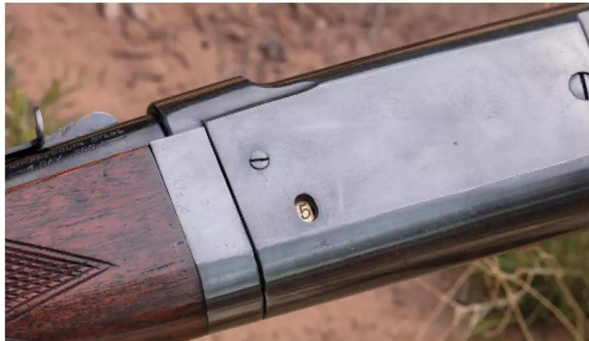
For decades, the Model 1899 and 99 offered a distinctive brass cartridge counter that indicated the number of rounds available in the rifle's internal magazine.
