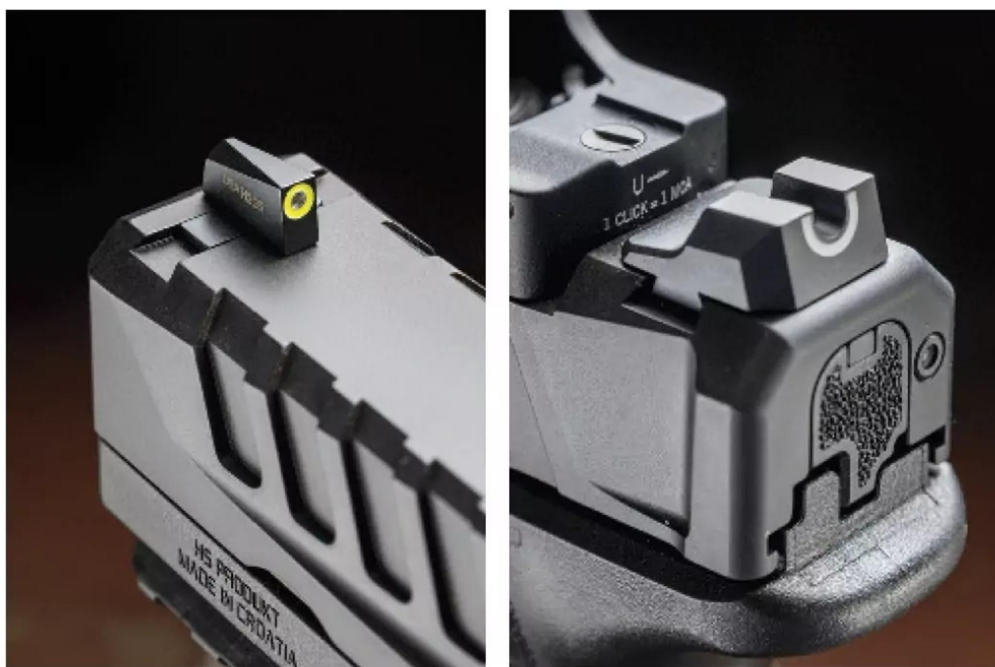
The sights are dovetailed to the slide. The front features a bright yellow ring with a tritium dot in the center. The rear is a U-notch rear sight with white outline. The sights co-witness with most red dots.
