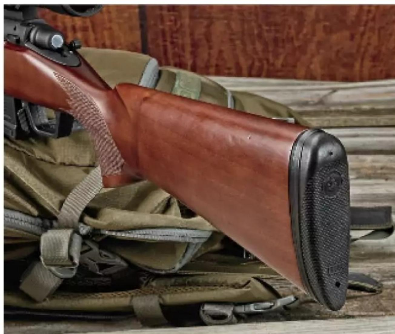
Total weight including scope and suppressor measured 9.66 pounds. The rubber recoil pad effectively reduces what remains of the felt recoil from the .308 Winchester.
