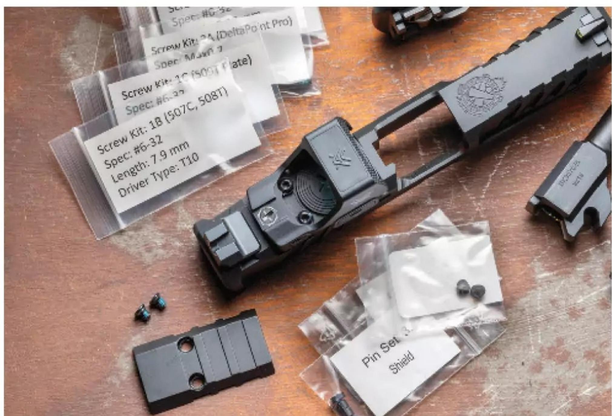
The Echelon 4.0FC features the Springfield Armory Variable Interface System, which includes optic mounting plates and fasteners making the pistol compatible with more than 30 red-dot sights.
