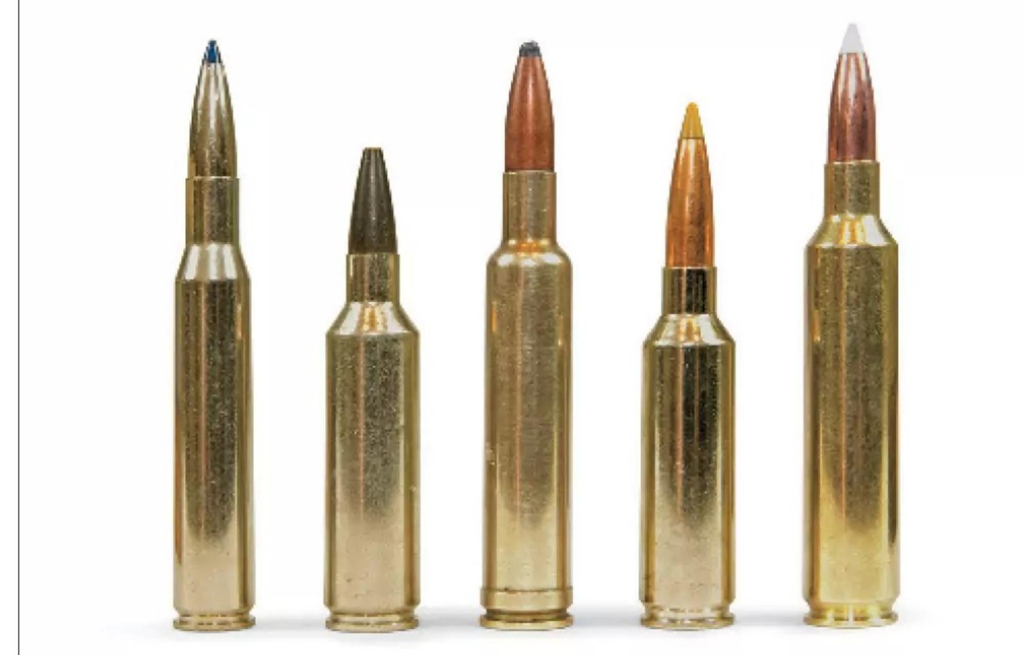
The ".270" hunting cartridges include (above left to right): .270 Winchester, .270 WSM, .270 Wby. Mag., 6.8 Western and .27 Nosler. With a 1-in-10-inch twist, the first three are limited to 150-grain bullets, maximum. Specified for faster twists, the 6.8 Western and .27 Nosler allow use of longer, heavier low-drag bullets.
