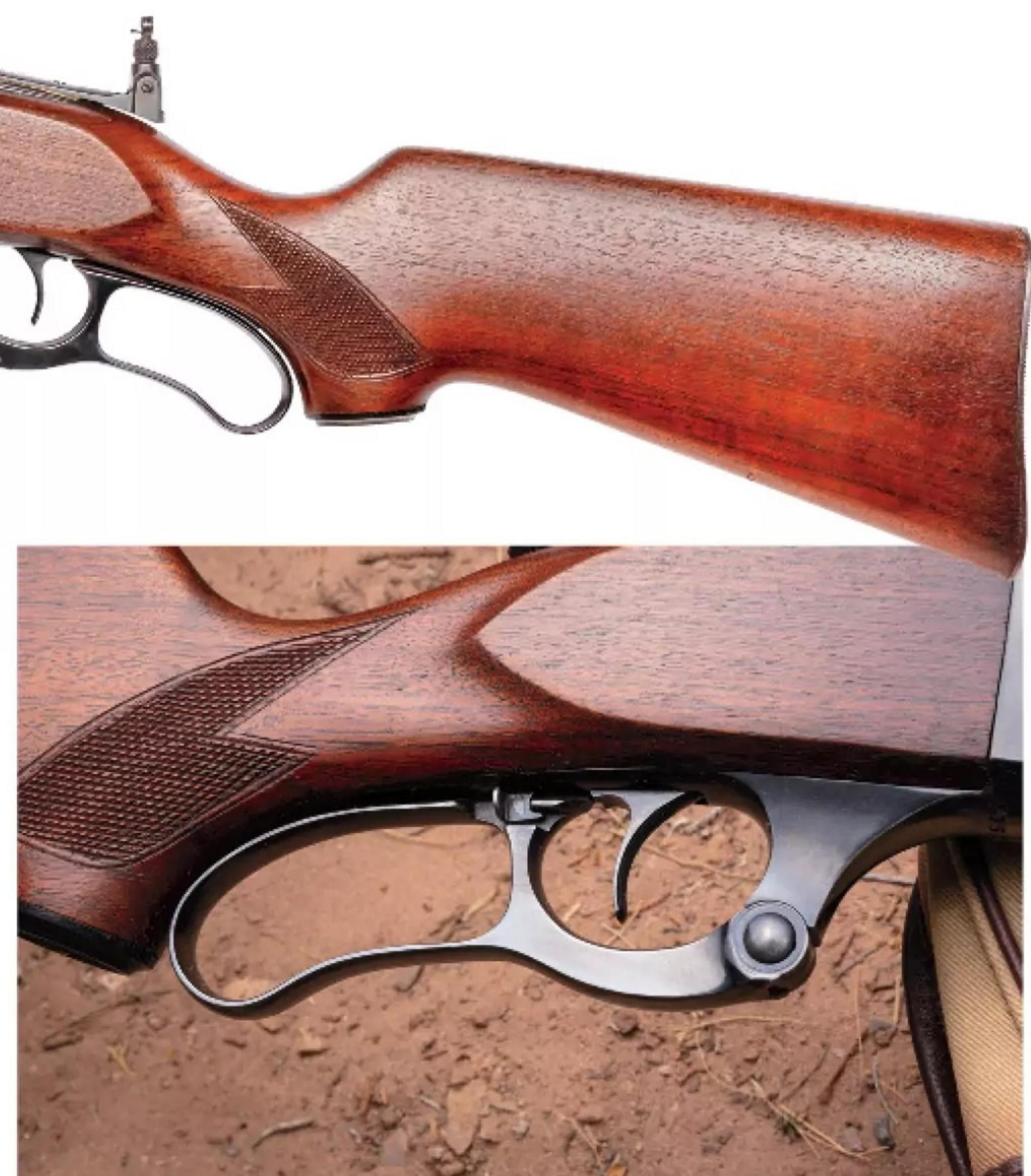
Behind the trigger is a safety latch used to lock the lever in its closed position. A shotgun-style tang safety was introduced in 1960, but some later 99 models retained the sliding safety.
