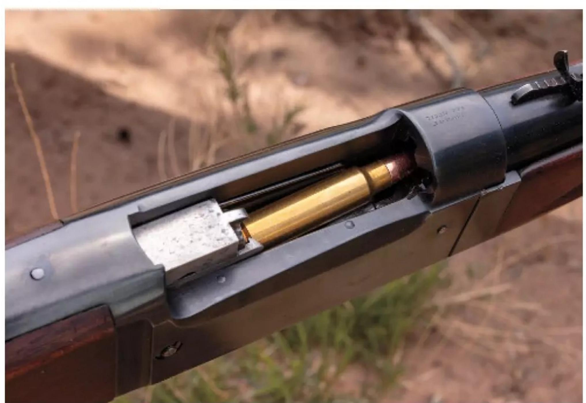
The Savage Model 1899 incorporated an internal rotary magazine that organized up to five rounds, plus one in the chamber. The elevator guided and centered each round to the feed ramp.
