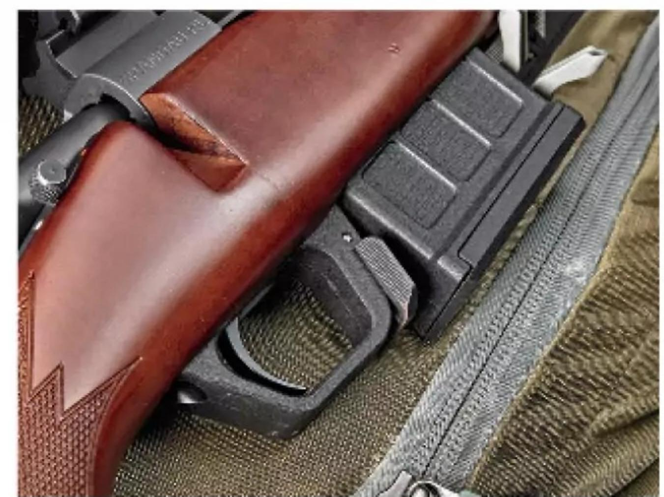
A bilateral push-forward-to-release lever drops mags free from the action. The Spandau RL also utilizes a molded polymer triggerguard.
