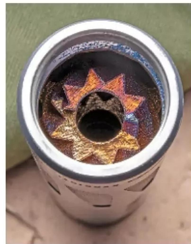
The first Triskelion is a 3D-printed blast baffle. It features three interlocking spirals, hence the name.
