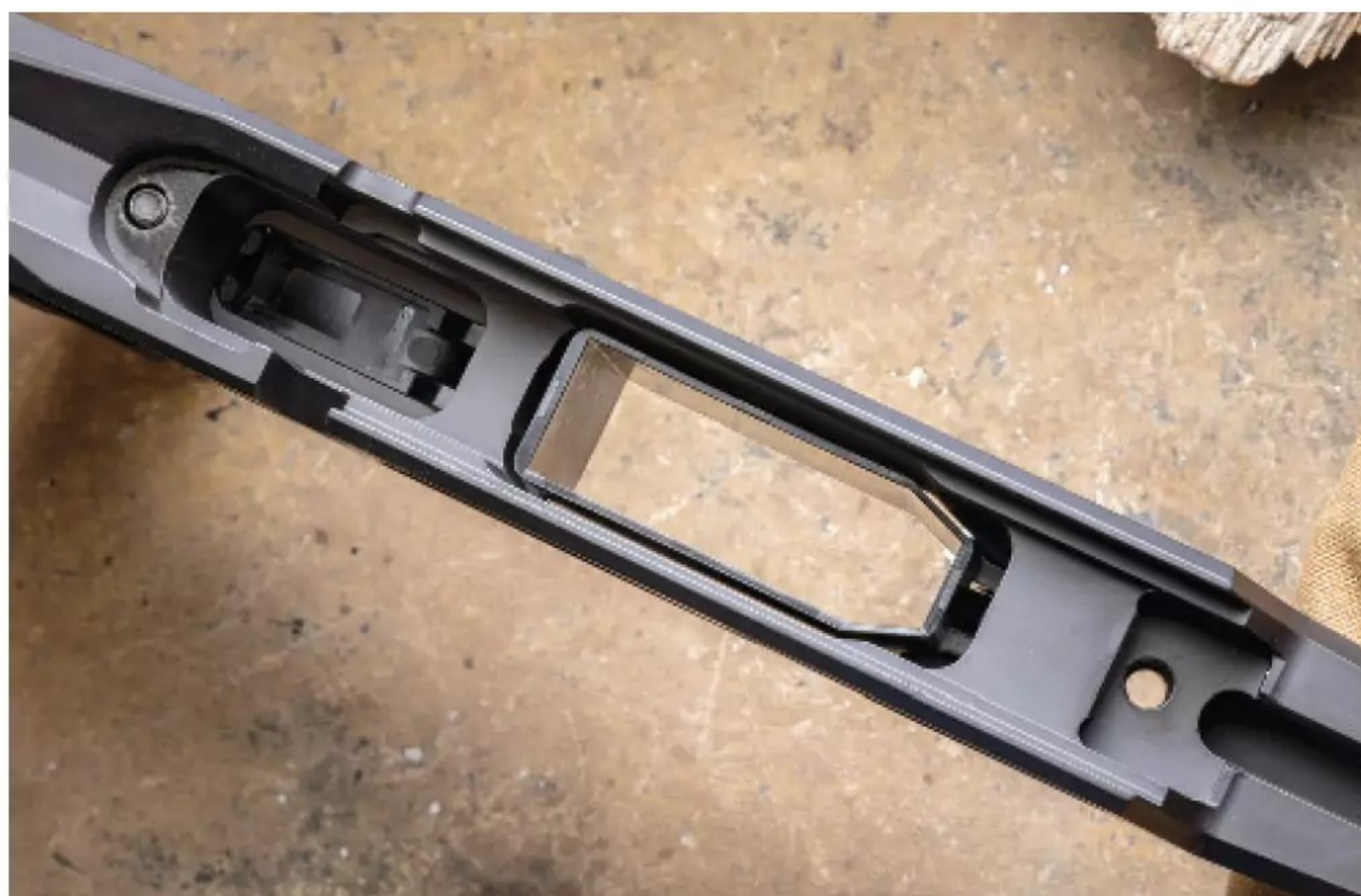
Note the recoil lug and flat mating surfaces between the action (above, top) and the chassis (above, bottom). The large surface area supports and immobilizes the barreled receiver for accuracy.
