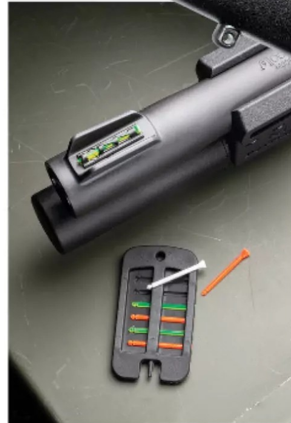
Protected by wings, the SPX front sight accepts interchangeable fiber-optic or solid white and orange rods.
