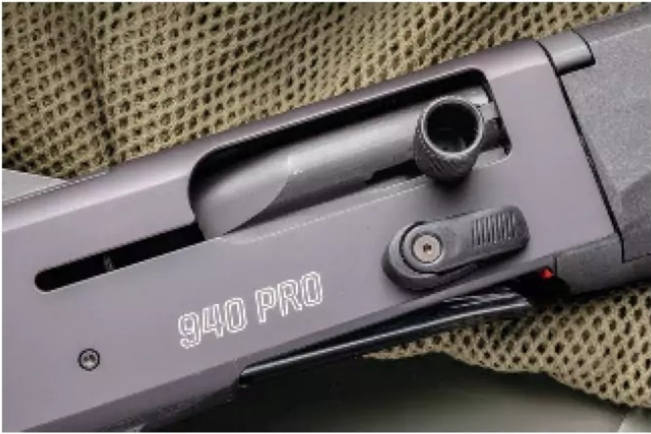
The knurled charging handle and bolt release are large. A small fence protects the bolt release from unintended activation.
