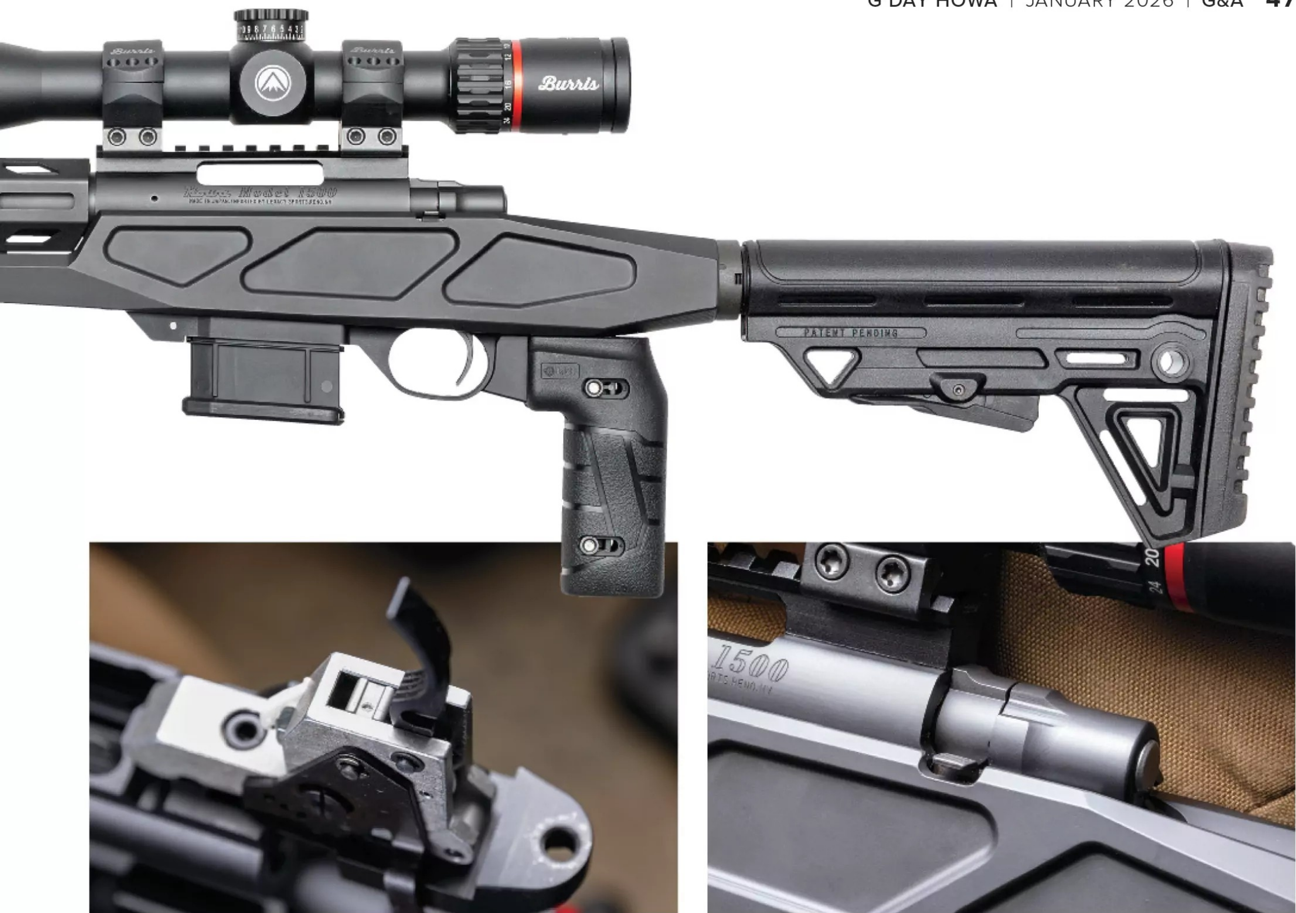
Removing a single screw allows easy separation of the two-stage trigger from the receiver. Trigger maintenance is convenient. It was tested at 2 pounds, 13 ounces.
