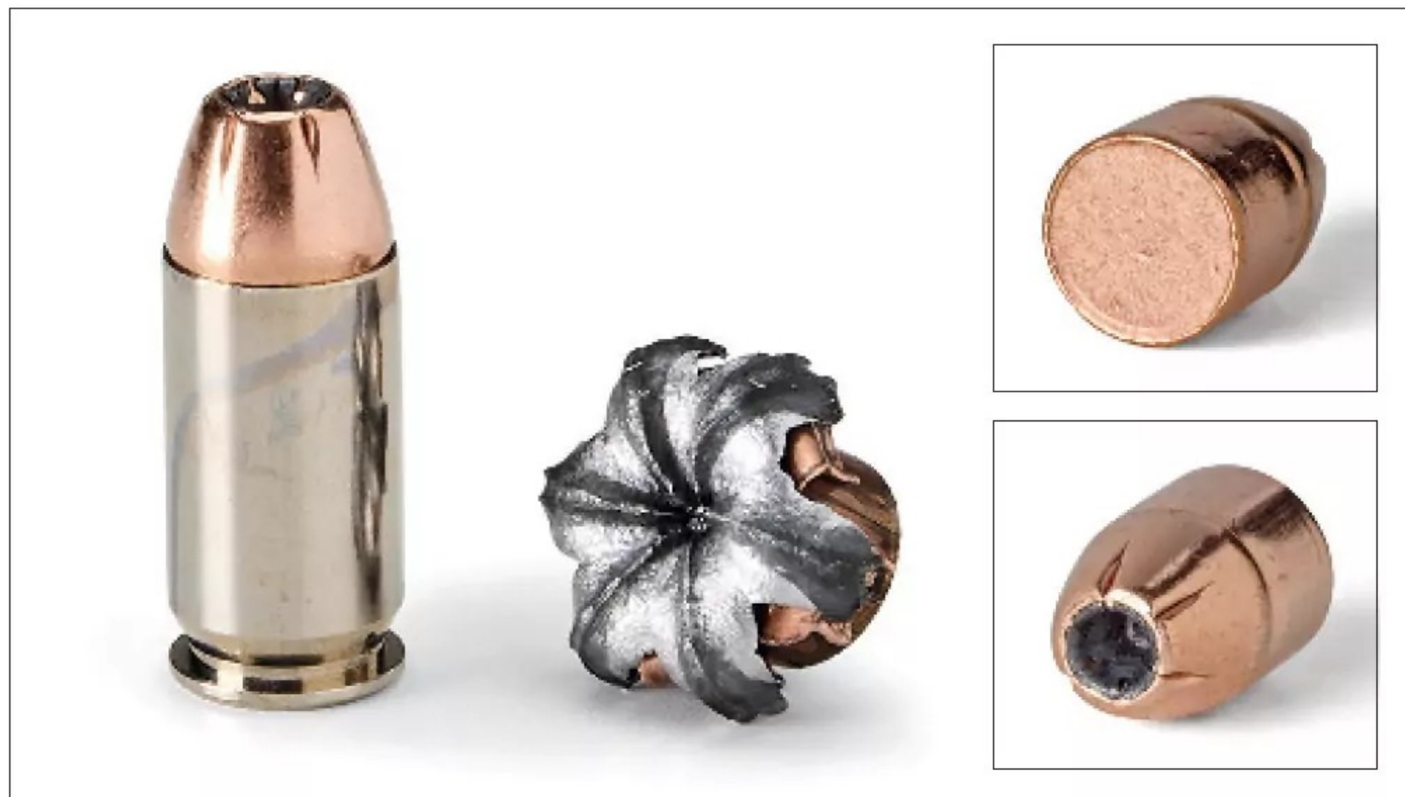
Fiocchi CovertX ammunition features a flat-base JHP bullet with a lead-alloy core given a skived jacket. The case is nicked brass.
