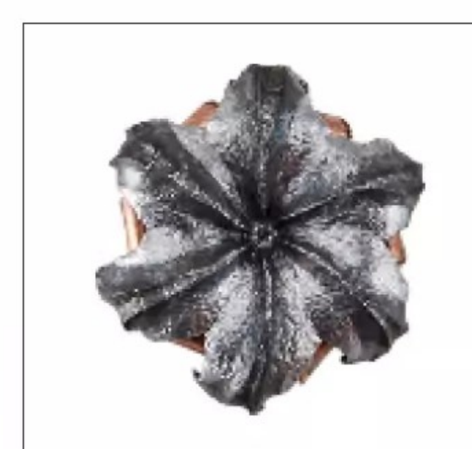
Fiocchi CovertX load for the .45 Auto features a 230-grain JHP that averaged 875 fps from a 4.25-inch barrel. Penetration in bare 10-percent clear gel was measured at 13.25 inches. The projectile expanded to .77 inch.
