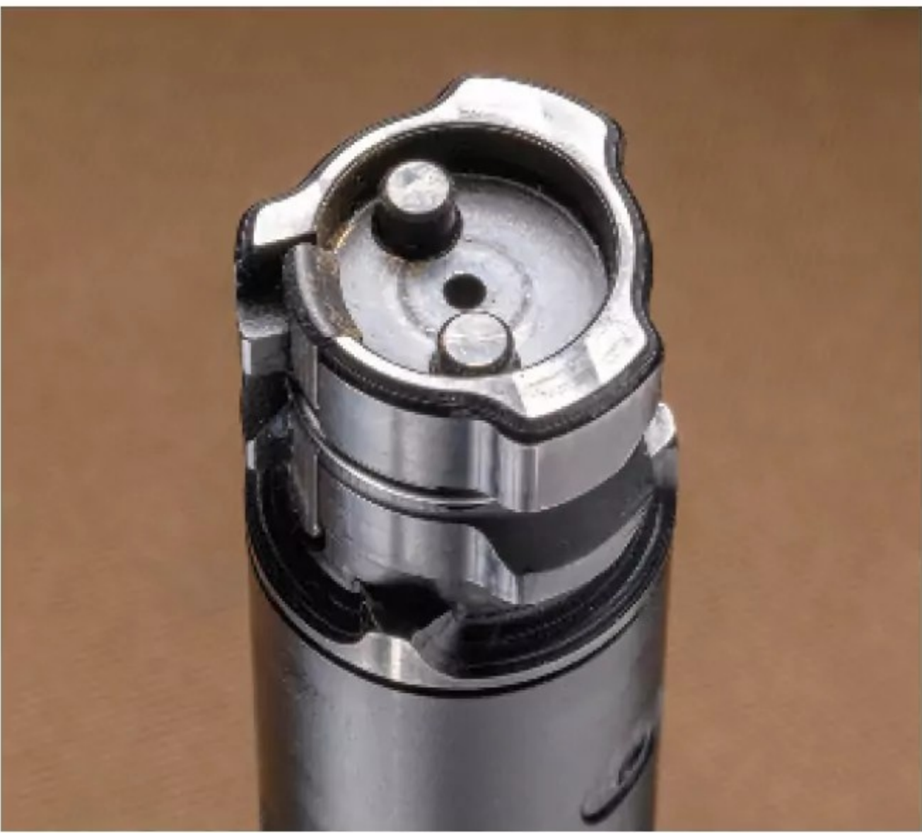
Count them! There are six lugs on the bolt head to contain magnum cartridge pressures. The bolt has a unique 65-degree lift.
