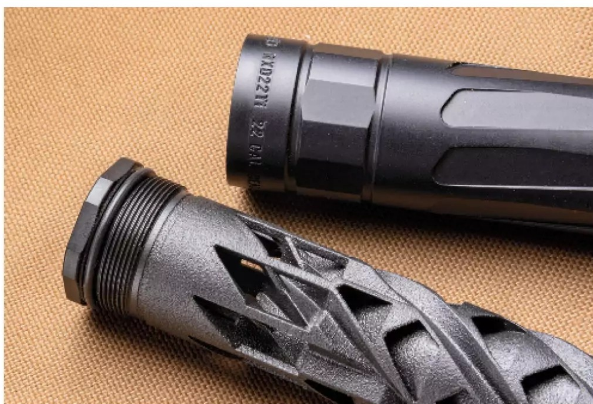
The Ruger RXD22Ti is a rimfire suppressor with a monocoque baffle assembly. It is light weight and short at 5.6 ounces and 5.66 inches.
