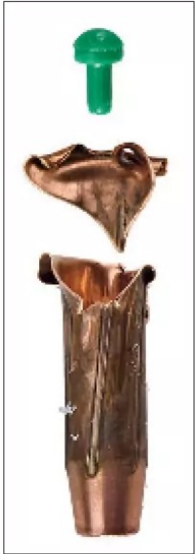
The .300 Blackout load exits an 8.5-inch barrel at 1,080 fps with 570 ft.-lbs. of energy, leaves a 10.5-inch barrel at 1,111 fps with 603 ft.-lbs., and a 16-inch barrel at 1,126 fps with 619 ft.-lbs. of energy. The 220-grain projectile penetrated 15 inches and fragmented in clear gel.
