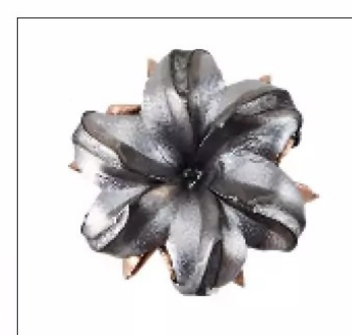
Fiocchi CovertX load for the 9mm features a 124-grain JHP bullet that averaged 1,145 fps from a 3.8-inch barrel. Penetration in bare 10-percent clear gel was measured at 14 inches. The projectile expanded to .58 inch.
