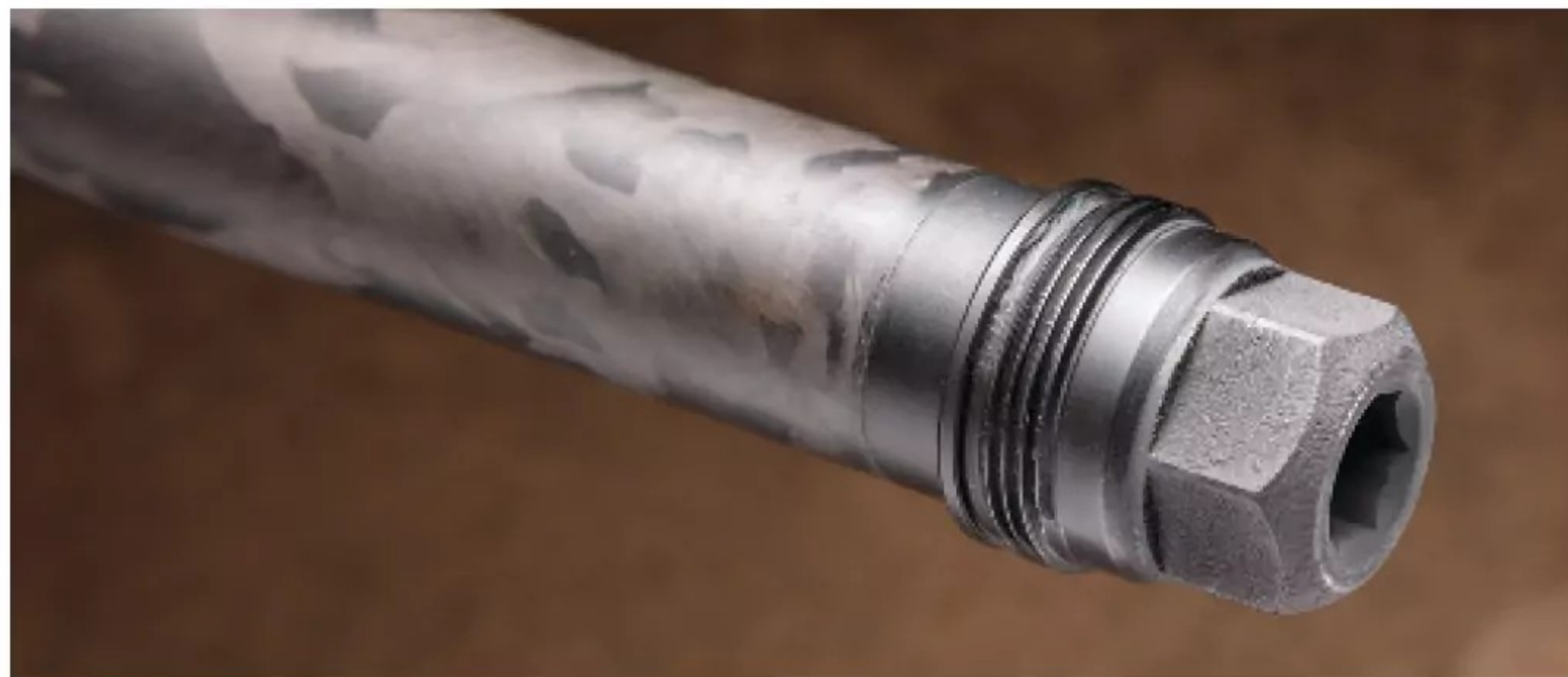
The carbon-fiber-wrapped barrel is standard with 5/8x24 threads. Underneath is a nut tightened to secure the threaded ring against the wrapped, stainless-steel barrel. A brake is also available.
