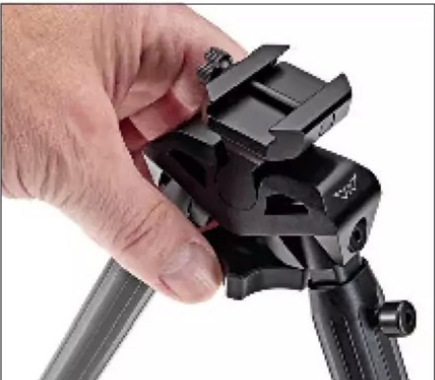
Loosening the tension knob underneath the Vapor bipod unlocks 50 degrees of cant. Unscrewing it completely allows the mount to change between Picatinny to M-Lok.
