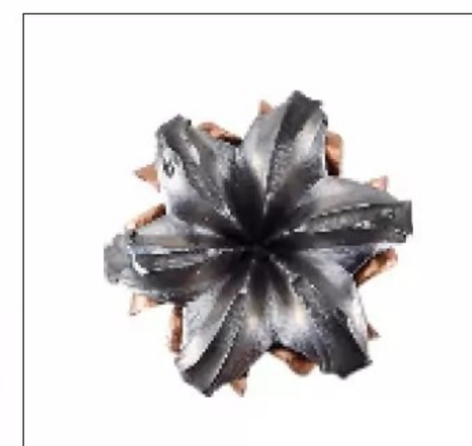
Fiocchi CovertX load for the .380 Auto features a 95-grain jacketed hollowpoint (JHP) that averaged 994 fps from a 3.25-inch barrel. Penetration in bare 10-percent clear gel was measured at 11 inches. The projectile expanded to .57 inch.
