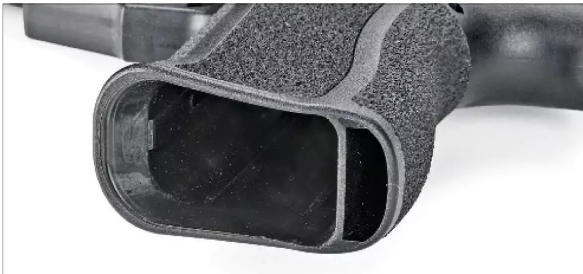
The magazine well isn't as aggressively flared as other modern handguns, but the inner-contour does help funnel magazines.
