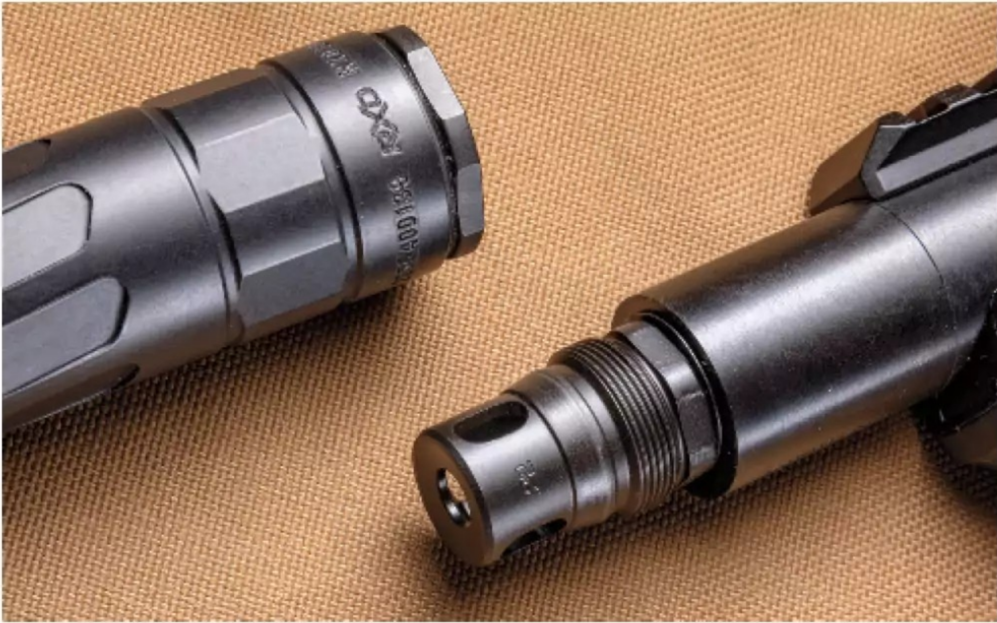
Rimfires are notoriously dirty to shoot. The XRF muzzlebrake helps to prevent lead build-up farther down the suppressor.
