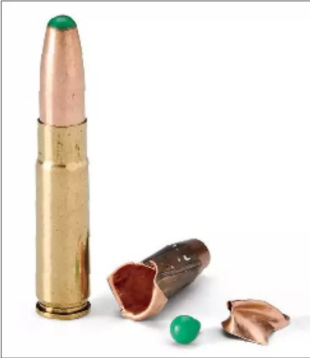
The .300 Blackout load exits an 8.5-inch barrel at 1,080 fps with 570 ft.-lbs. of energy, leaves a 10.5-inch barrel at 1,111 fps with 603 ft.-lbs., and a 16-inch barrel at 1,126 fps with 619 ft.-lbs. of energy. The 220-grain projectile penetrated 15 inches and fragmented in clear gel.
