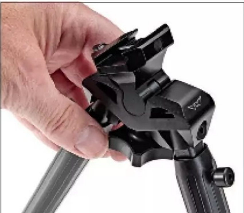
Loosening the tension knob underneath the Vapor bipod unlocks 50 degrees of cant. Unscrewing it completely allows the mount to change between Picatinny to M-Lok.
