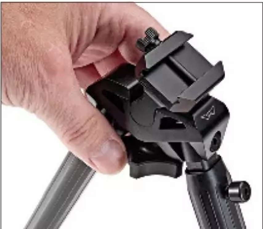
Loosening the tension knob underneath the Vapor bipod unlocks 50 degrees of cant. Unscrewing it completely allows the mount to change between Picatinny to M-Lok.
