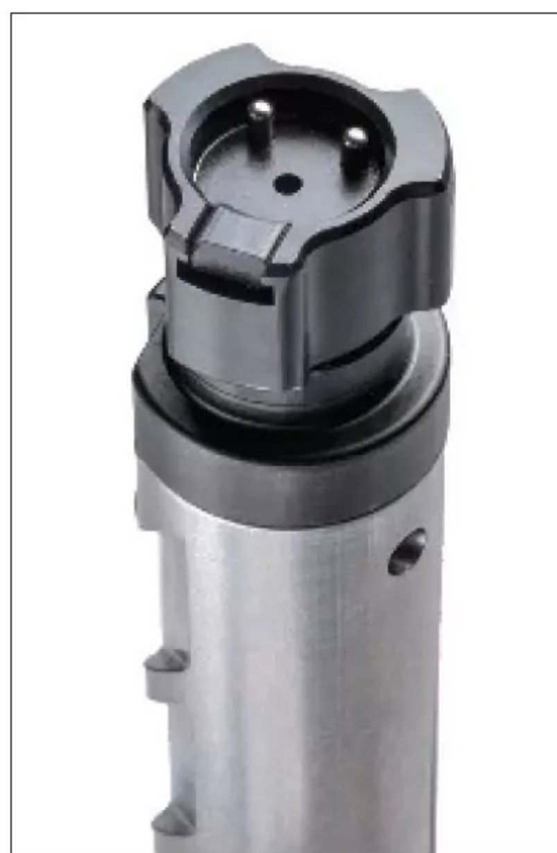
The three-lug bolt enables the short 60-degree lift. The bolt includes dual ejectors, extractor, and small-diameter firing pin.
