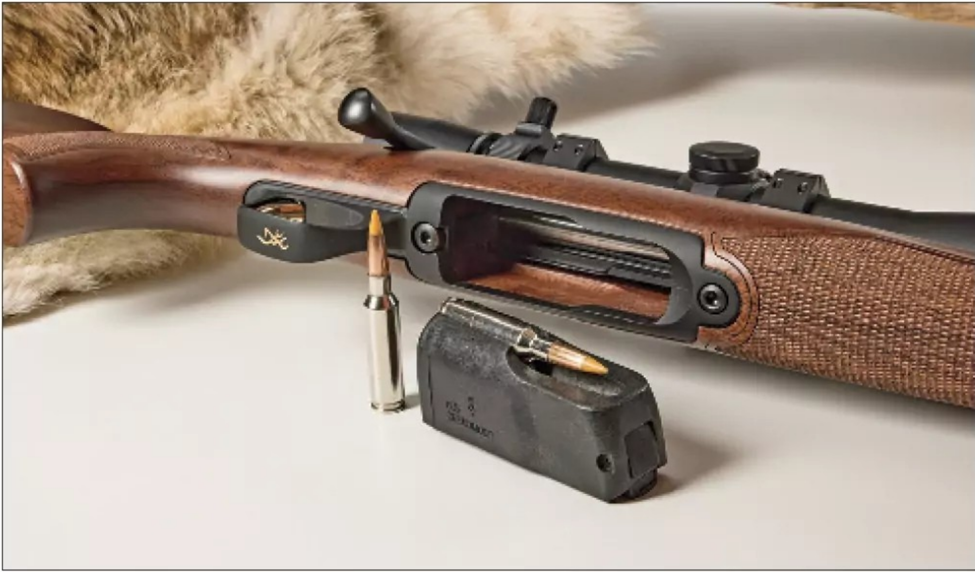
The triggerguard and magazine well are aluminum and secured to the action by two screws. The polymer center-feed magazine is a rotary design, cartridge specific and reliable. $63
