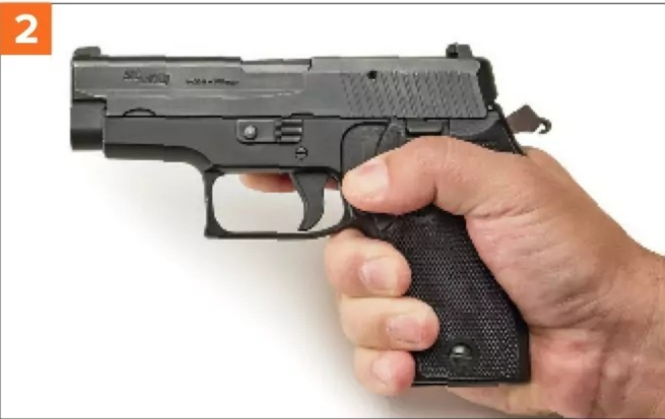
SIG Sauer’s P-Series featured a serrated thumb-operated decocking lever in front of the slide-stop lever and above the magazine release button. With the hammer cocked (1), press down on the lever with the thumb (2). The hammer safely falls forward, even when loaded (3).
