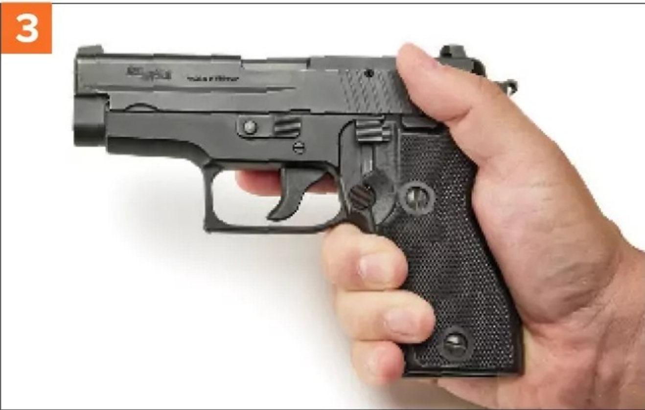
SIG Sauer’s P-Series featured a serrated thumb-operated decocking lever in front of the slide-stop lever and above the magazine release button. With the hammer cocked (1), press down on the lever with the thumb (2). The hammer safely falls forward, even when loaded (3).
