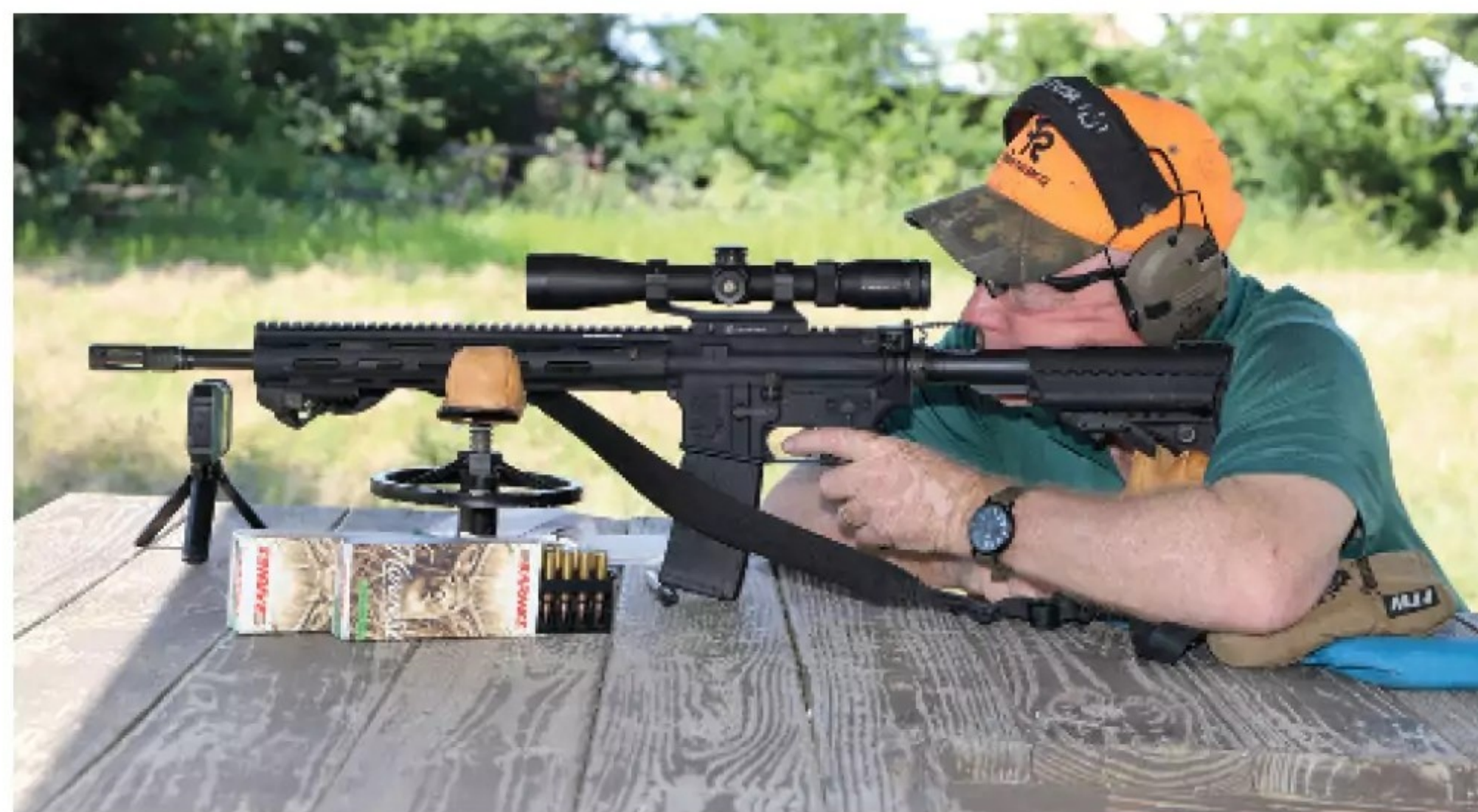
Harvest Collection's .223 Remington load with 69-grain TGK was grouped using a S&W M&P15. Naturally, the 16.1-inch barrel resulted in significant velocity loss, but it was consistent and produced small extreme spread (ES) and low standard deviation (SD).
