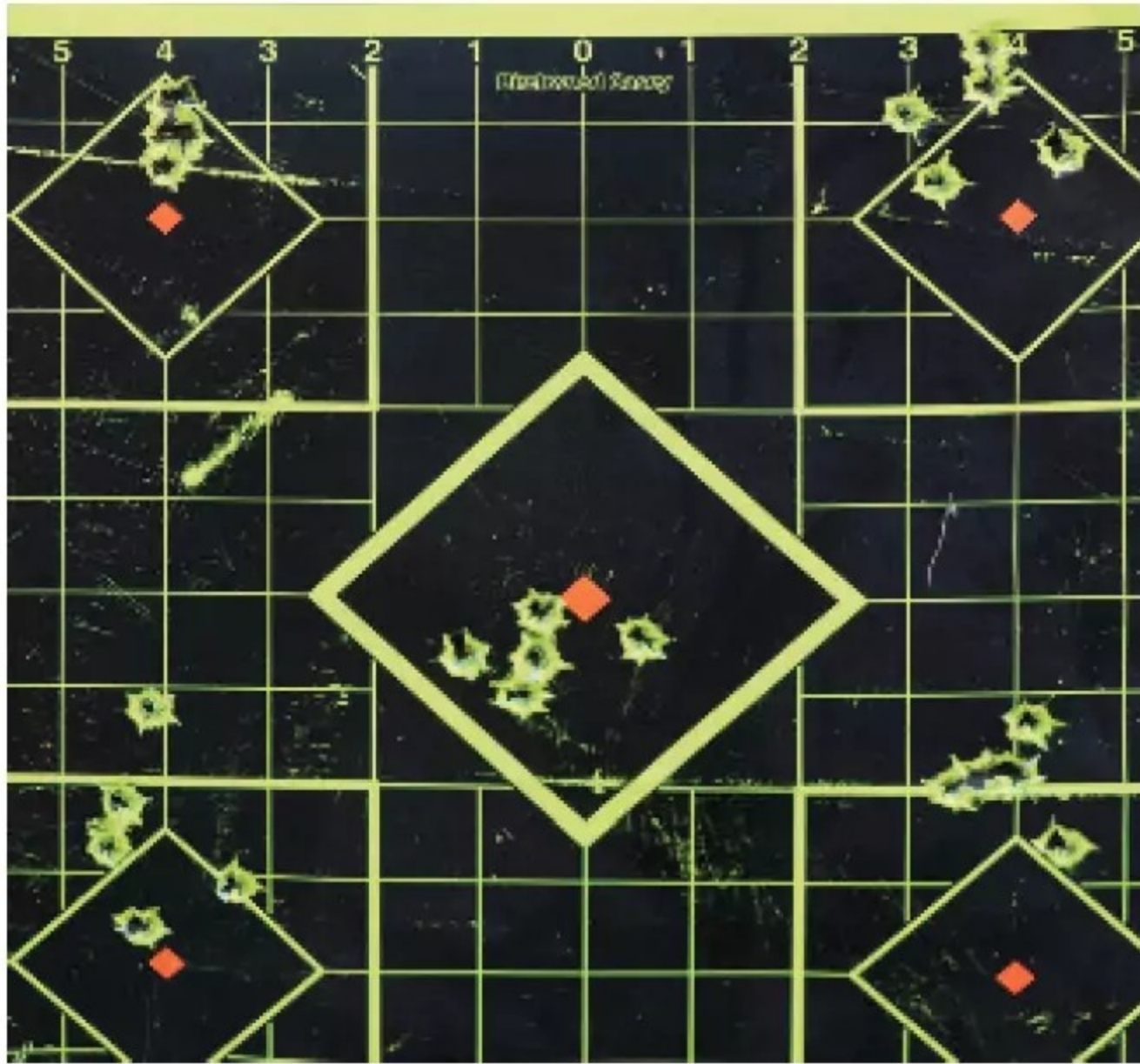
The Harvest Collection's 165-grain TKG load for the .308 Win. was also tested in a Browning X-Bolt 2 Speed. The average group size measured 1.514 inches. The chrono reported excellent consistency.
