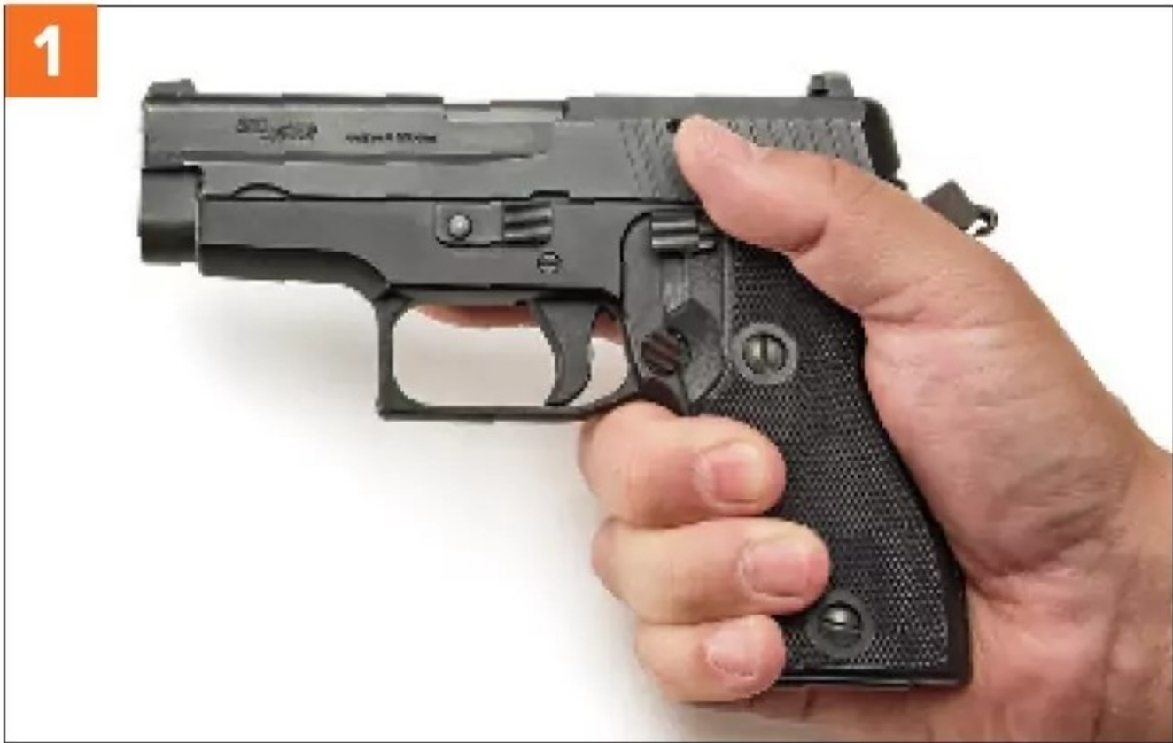
SIG Sauer’s P-Series featured a serrated thumb-operated decocking lever in front of the slide-stop lever and above the magazine release button. With the hammer cocked (1), press down on the lever with the thumb (2). The hammer safely falls forward, even when loaded (3).
