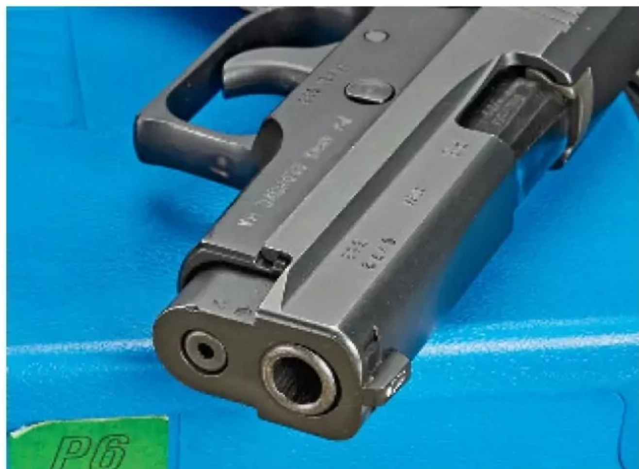
The distinctive lines of the slide are an artifact of the slide-manufacturing process, giving the SIG Sauer P6 its distinctive look.
