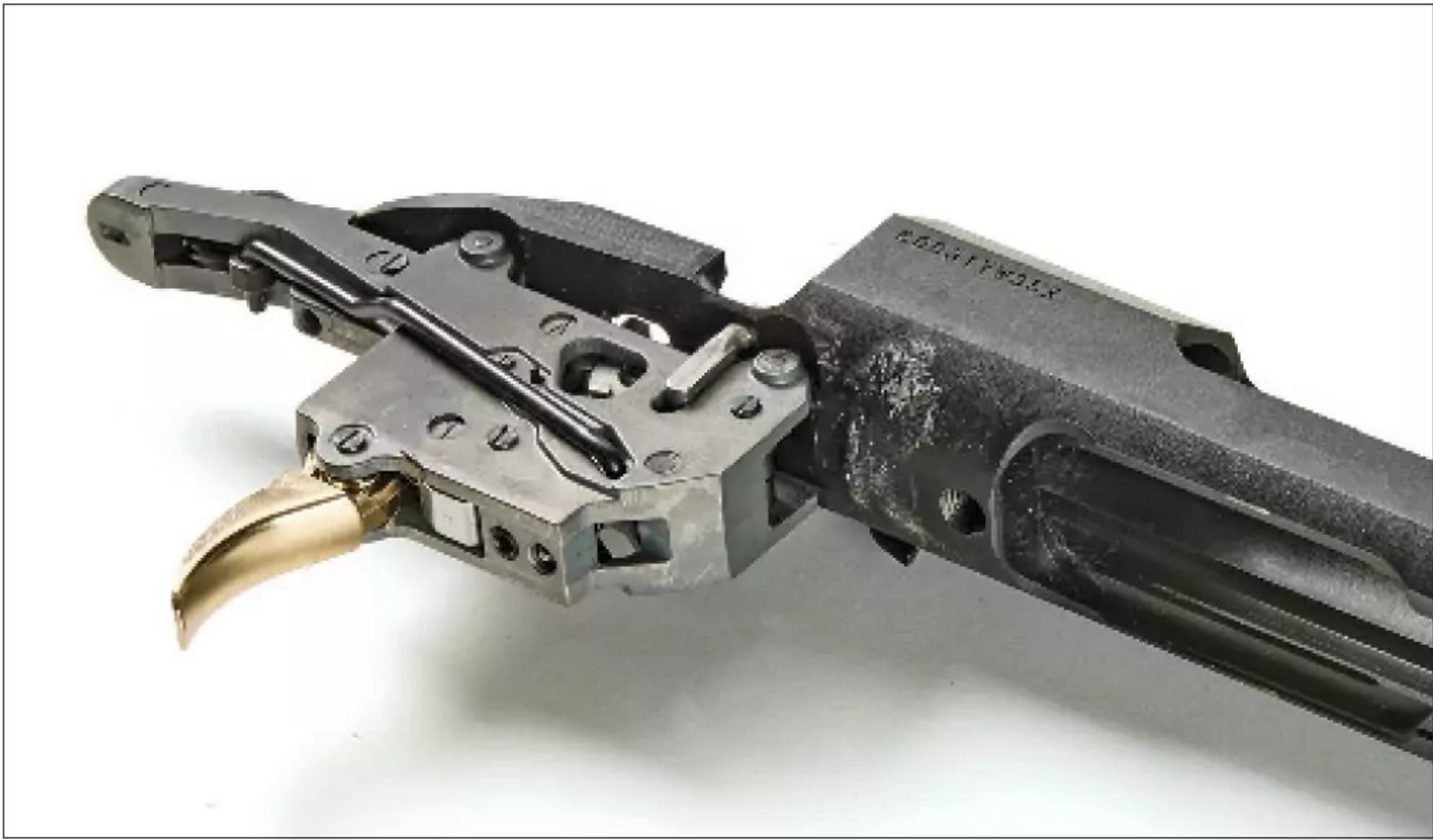
The Browning DLX trigger is a refined design that retains the familiar “gold” appearance. Factory set at 3½ pounds, it can be adjusted to the SAAMI minimum of just 3 pounds.
