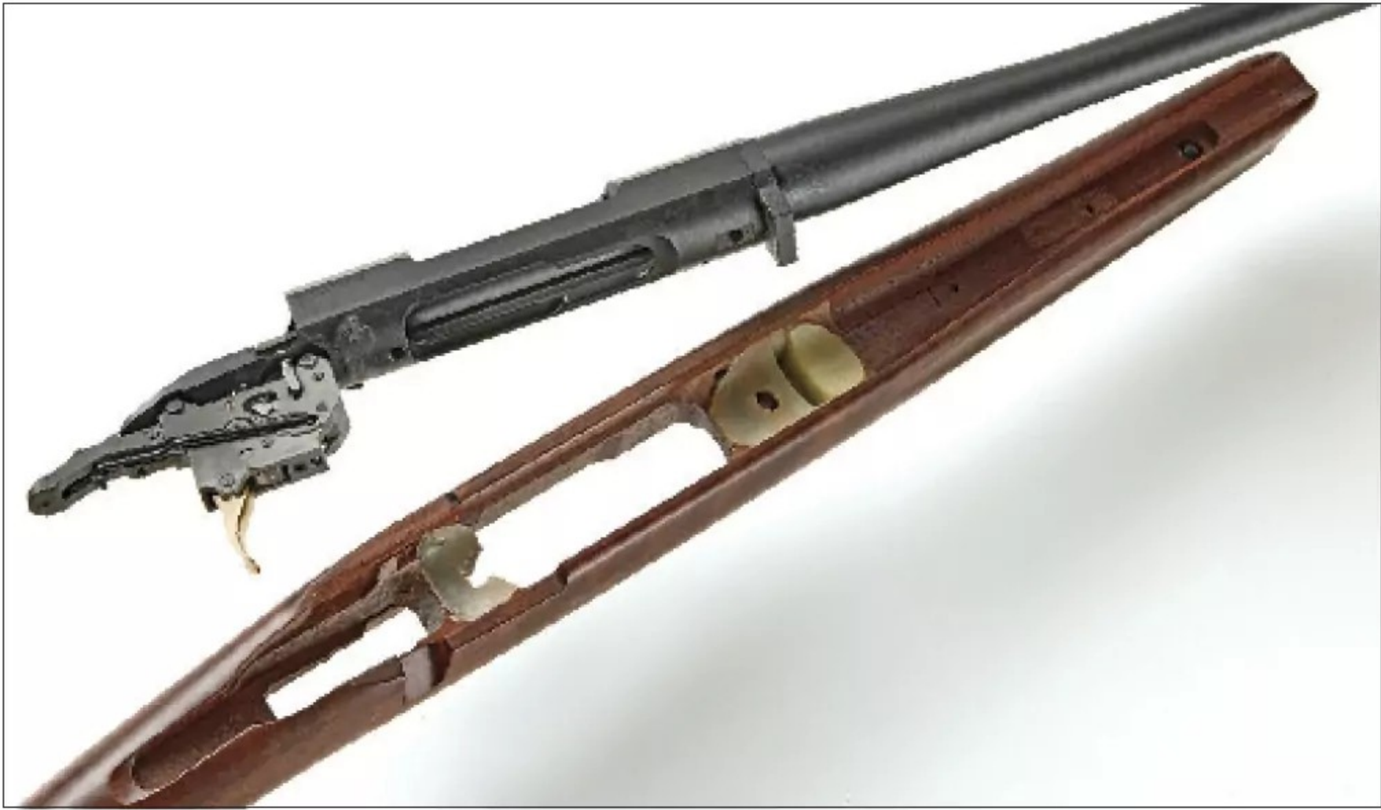
A single recoil lug is bedded to the walnut stock, and the forend is inletted to free-float the barrel for increased accuracy potential. The front and rear action screws are also factory bedded.
