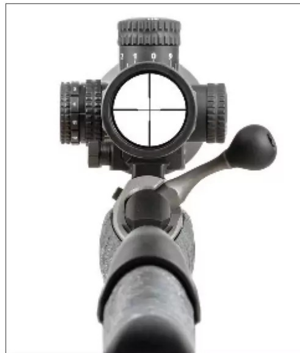
A Ruger American has a 75-degree bolt lift. It clears most ocular housings, but it may not clear magnification throw levers.
