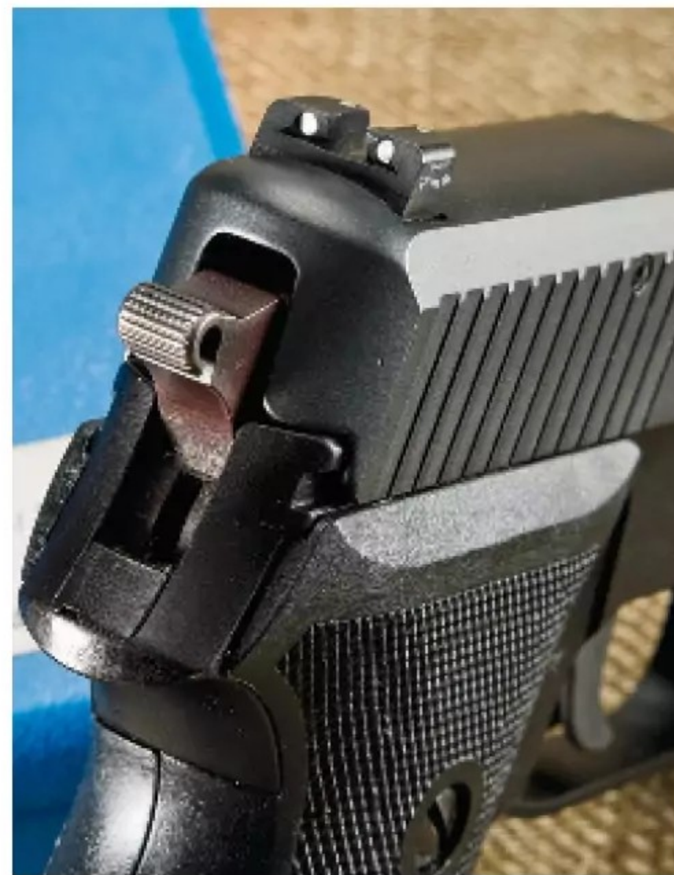
German police-issued pistols featured three white-dot dovetailed sights. The P225s imported into the U.S. were upgraded with tritium sights. Aftermarket SIG Sauer replacement sights fit, also.
