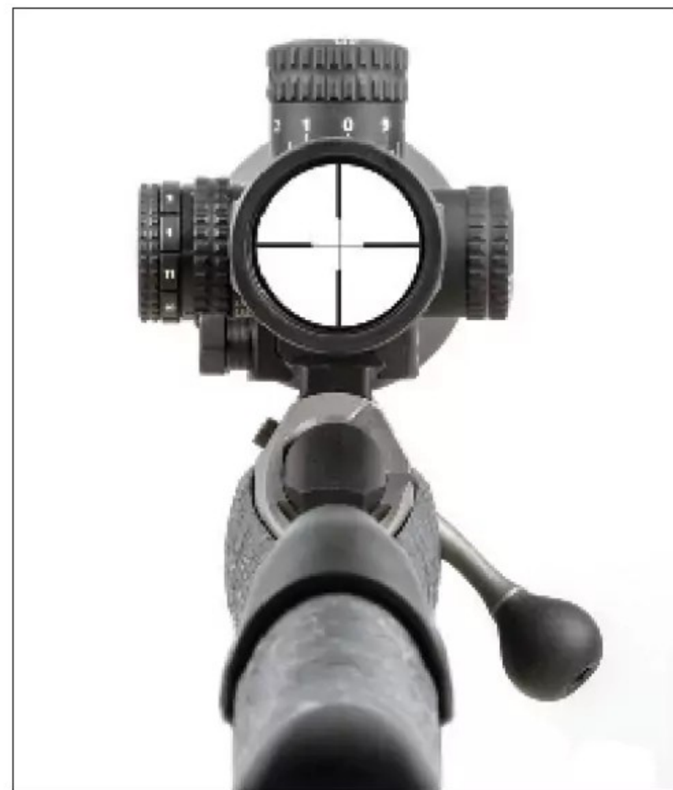
A Ruger American has a 75-degree bolt lift. It clears most ocular housings, but it may not clear magnification throw levers.
