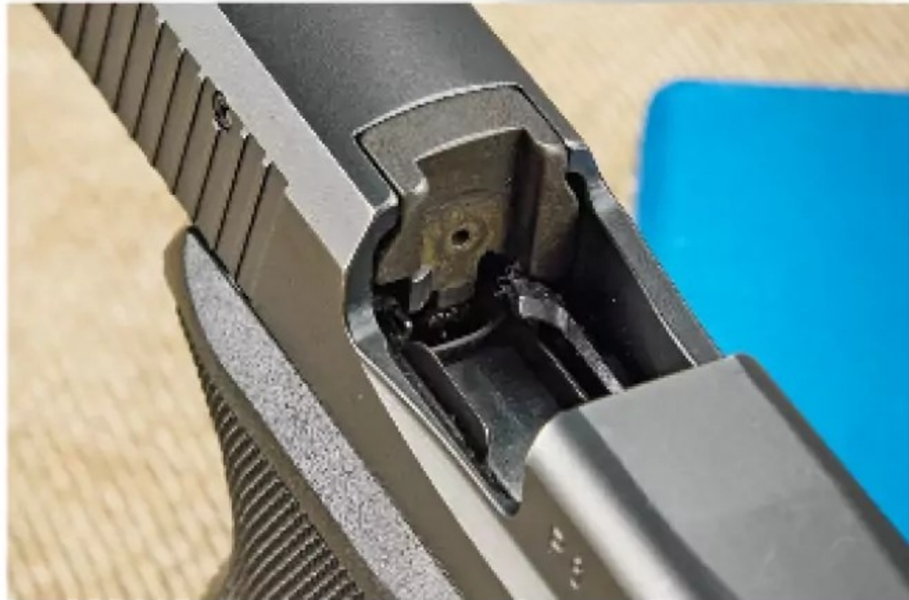
The breechblock of the P6 was not machined with the slide. It is a separate component held in place by a stout roll pin.
