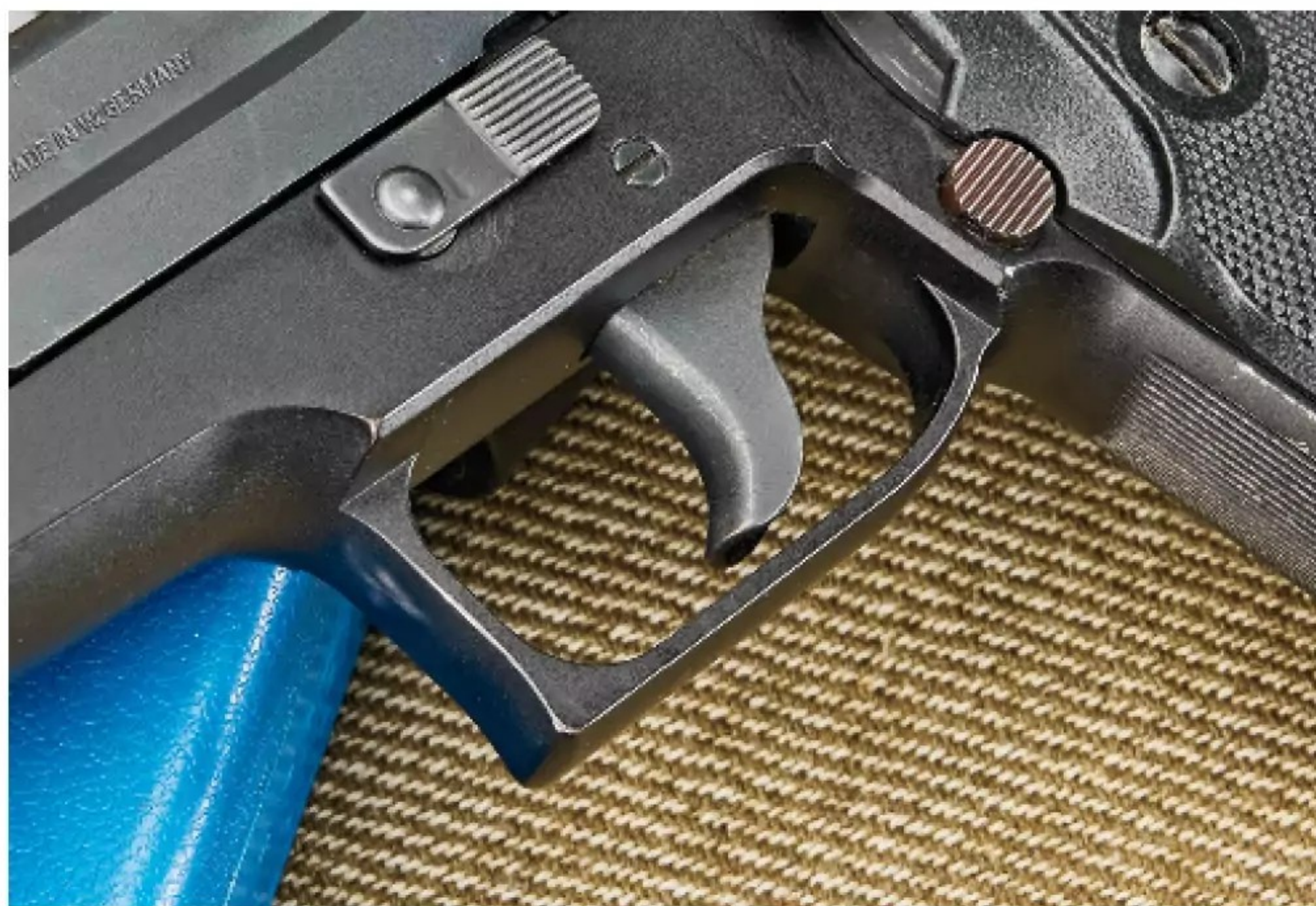
The triggerguard is square and slightly hooked. Integral to the frame is a high-grip junction atop the frontstrap. The stamped-metal trigger is curved and without texture.
