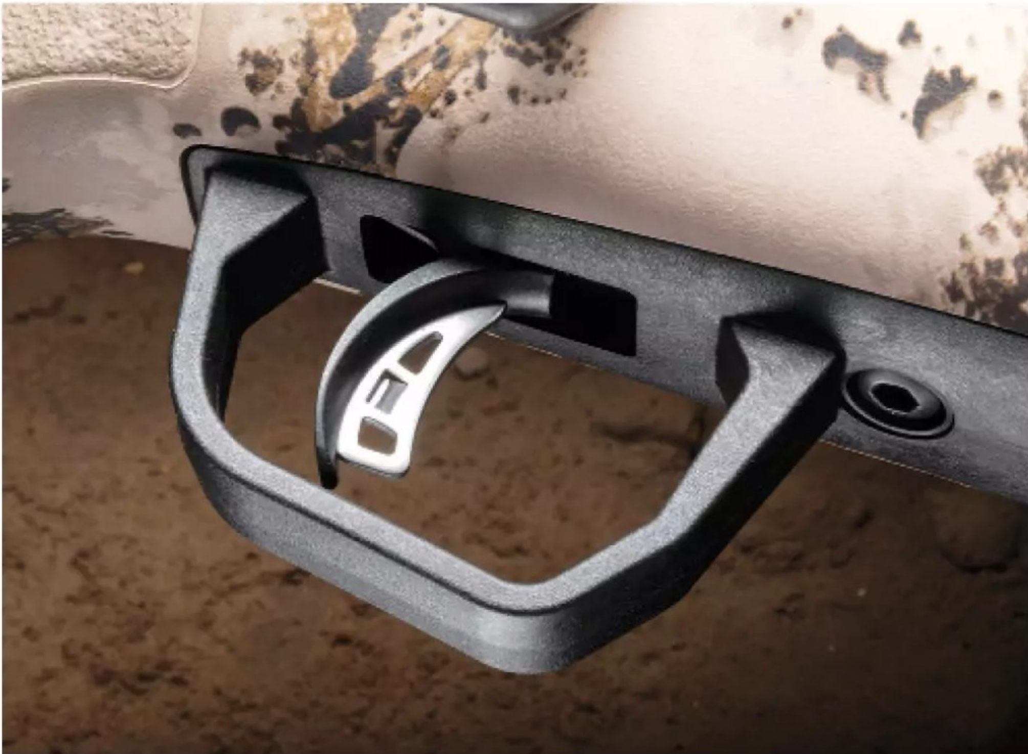
The AccuTrigger is user-adjustable, featuring a safety lever in the center that must be depressed before the trigger can be operated. The triggerguard and “bottom metal” are molded polymer.
