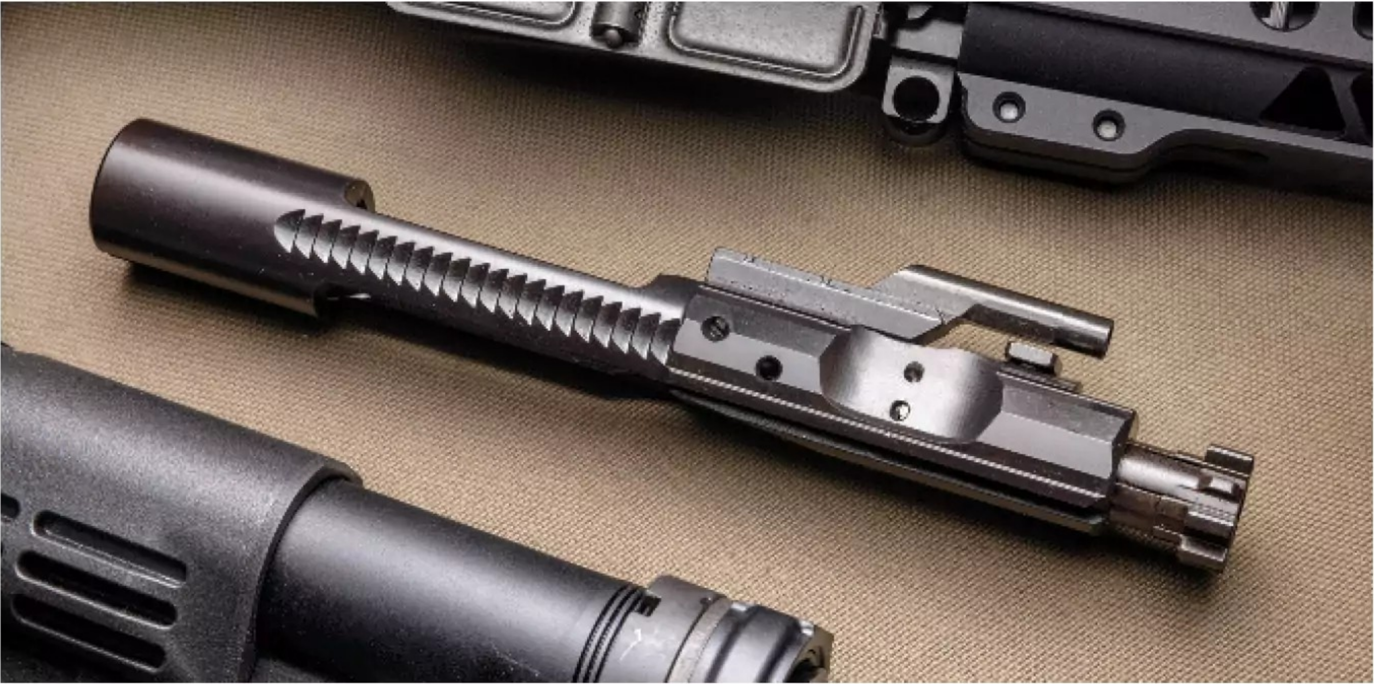
The bolt carrier group features a nitride finish. Note the mil-spec notches along the right sight for the forward assist to press against. The gas key, bolt and cam are standard items.
