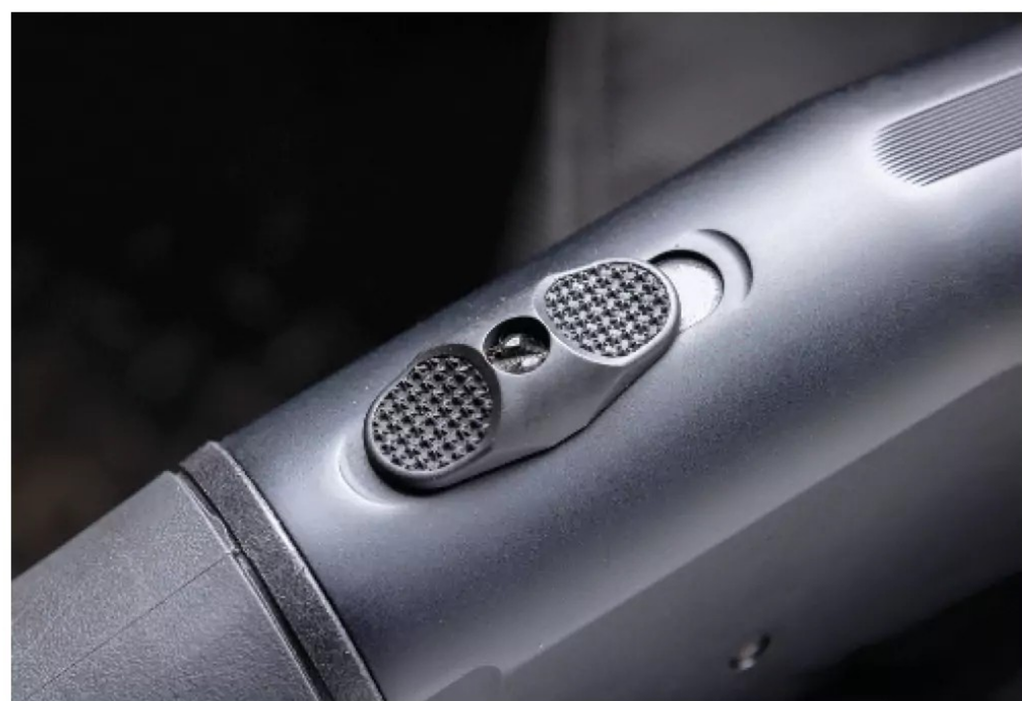
The 990 AfterShock features Mossberg’s new receiver-mounted safety. It’s oversized, featuring aggressive knurling for sure activation. Press the switch forward to fire, and thumb it back for safe.
