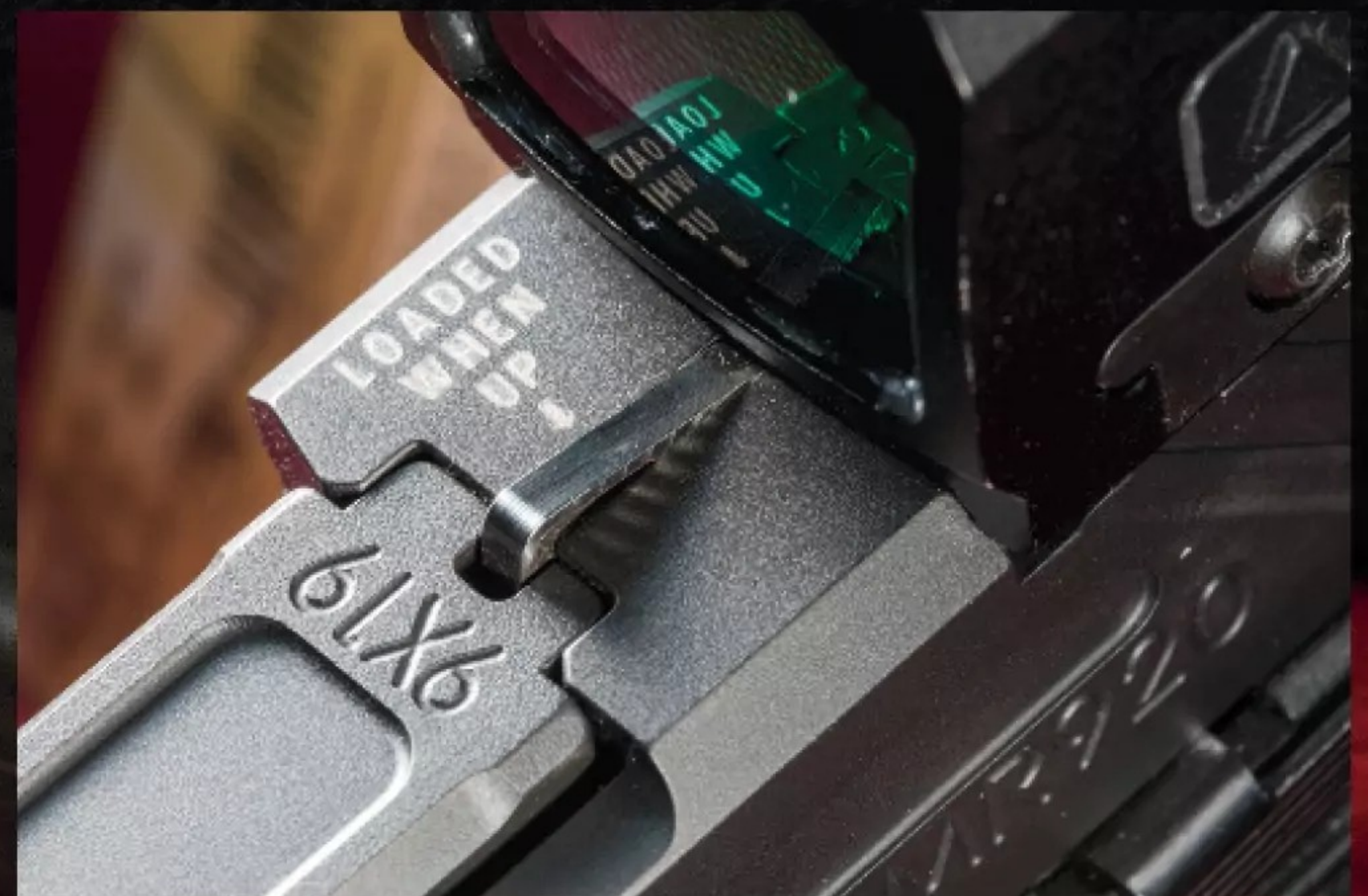
The loaded chamber indicator (LCI) is necessary for California compliance but must clear a mounted optic.
