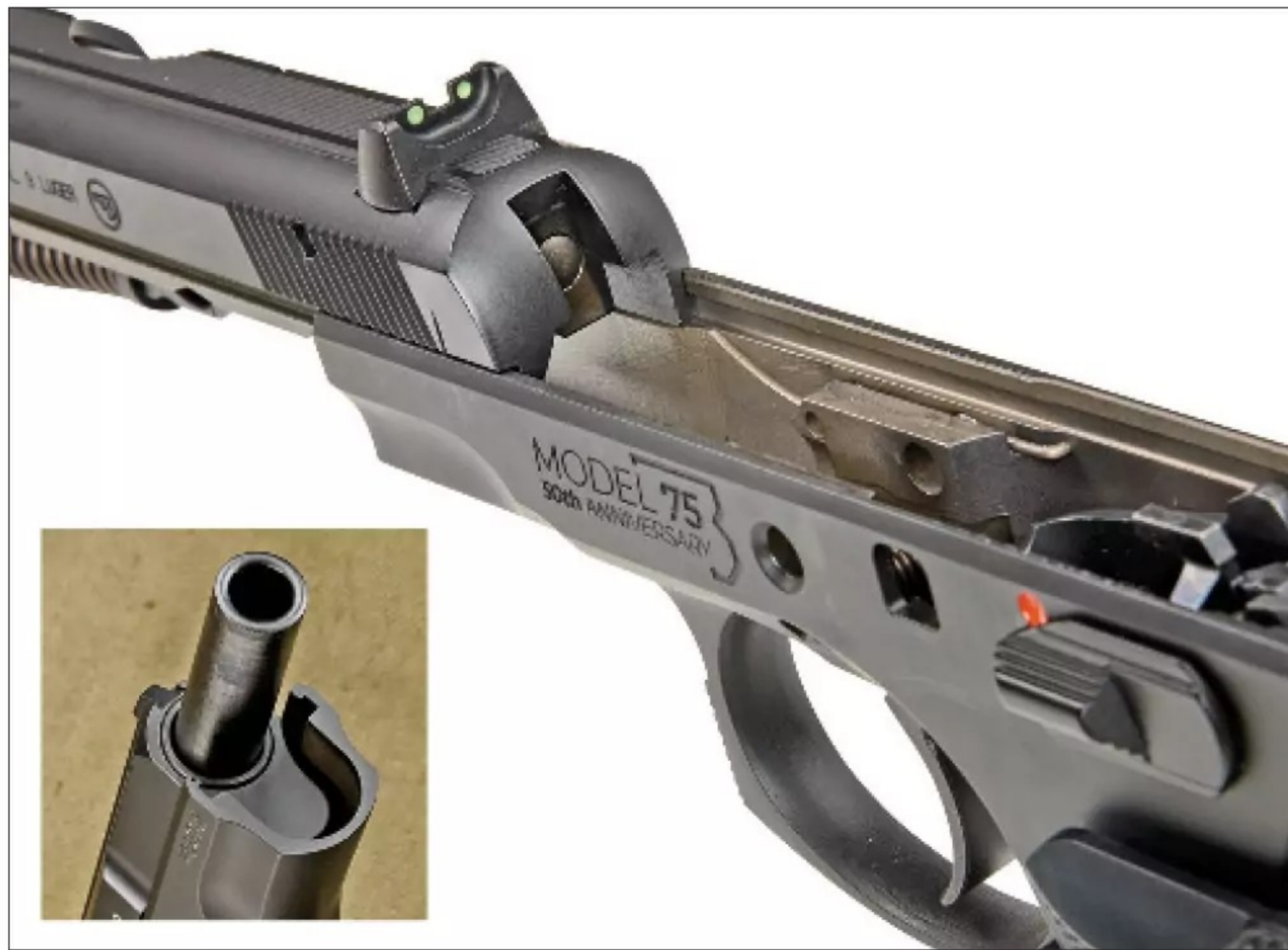
The slide of the CZ 75 rides inside the frame rails. Inset Photo: The recoil spring and guiderod do not protrude from the slide at full recoil, either.
