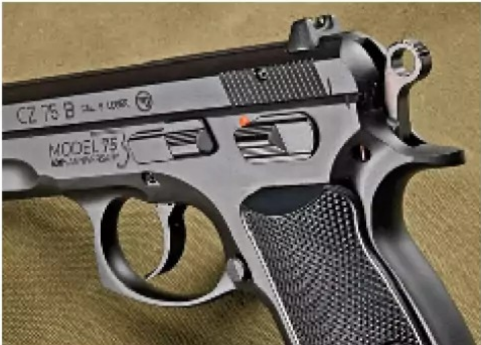
If the hammer must be carefully lowered to the half-cock notch, you can fire the CZ 75 in DA or by cocking the hammer to SA.
