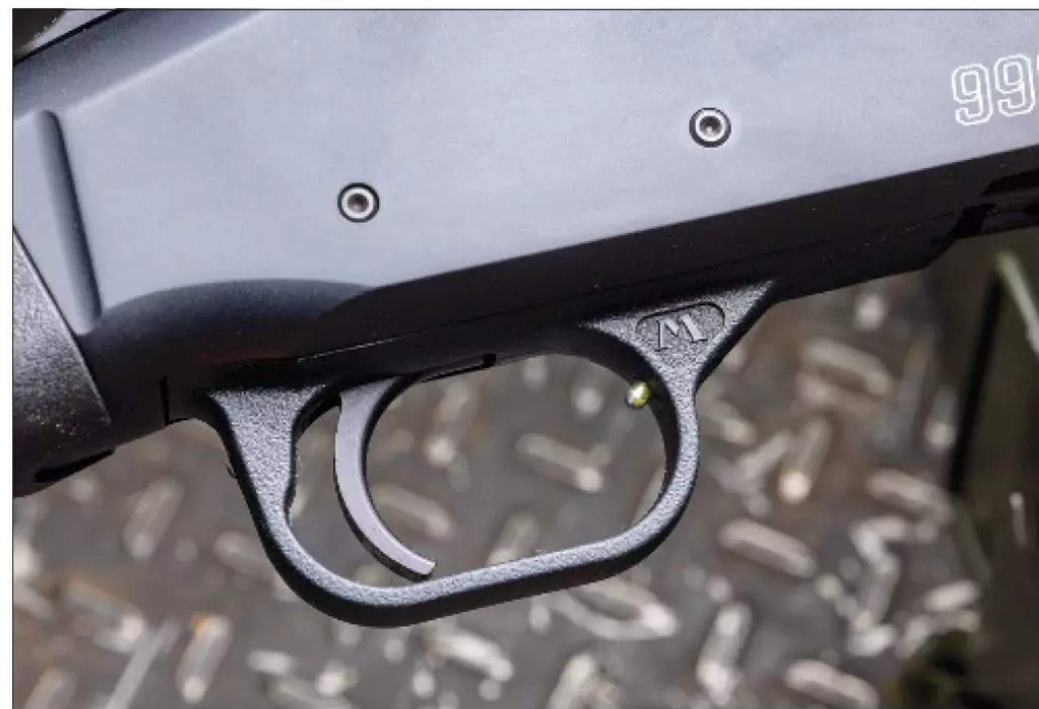
The molded polymer triggerguard is a functional size, and there is a large “M” logo for “Mossberg” toward the front. The steel trigger averaged 4 pounds on the trigger gauge.
