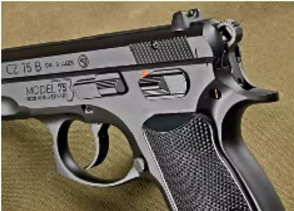
With the hammer at rest, the CZ 75 B can be fired as a double action (DA), using the trigger to cock and fire the pistol.
