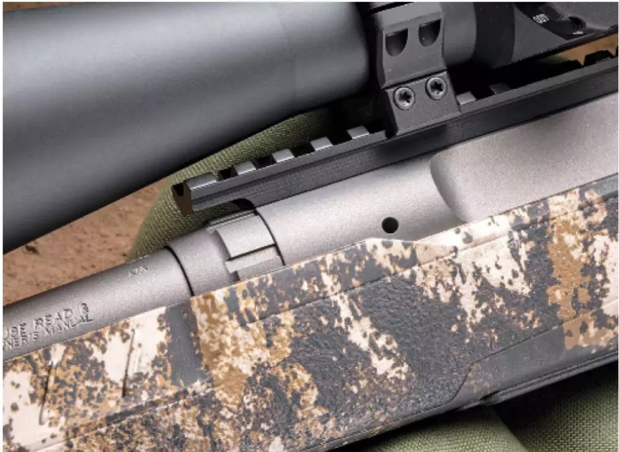
The Axis 2 Pro models maintain Savage’s standard-shank barrel locking system to secure the barrel to the action. The optic rail smartly extends over the lock nut for scope-mounting flexibility.
