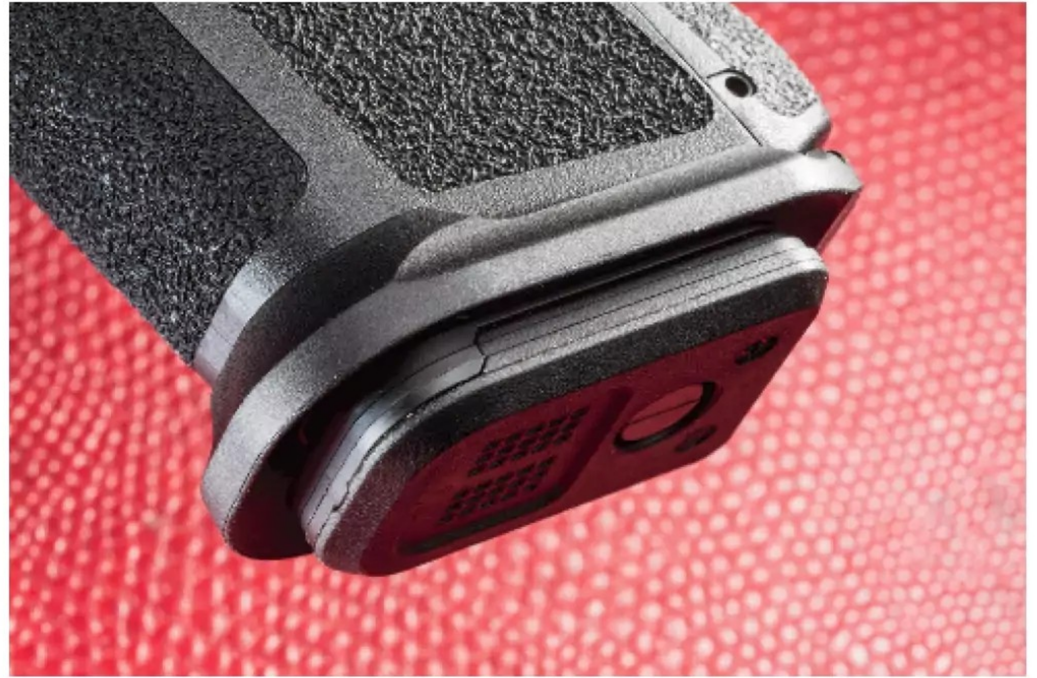
The polymer magazine well is is flared and removable.
