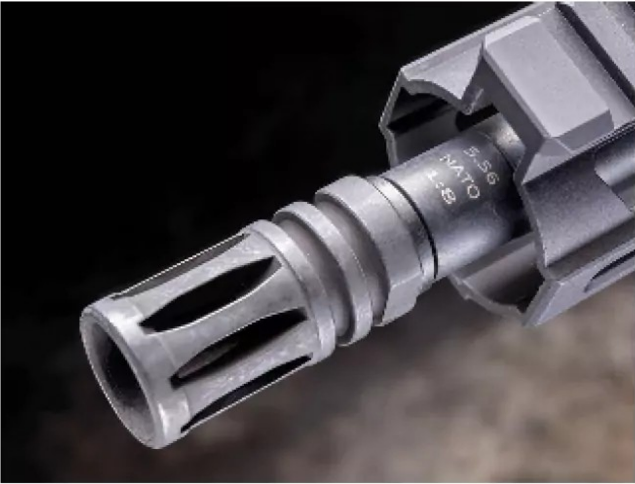
The A2-style birdcage muzzle device is closed at the bottom to function as a compensator. A crush washer is used to clock the ports at the top.
