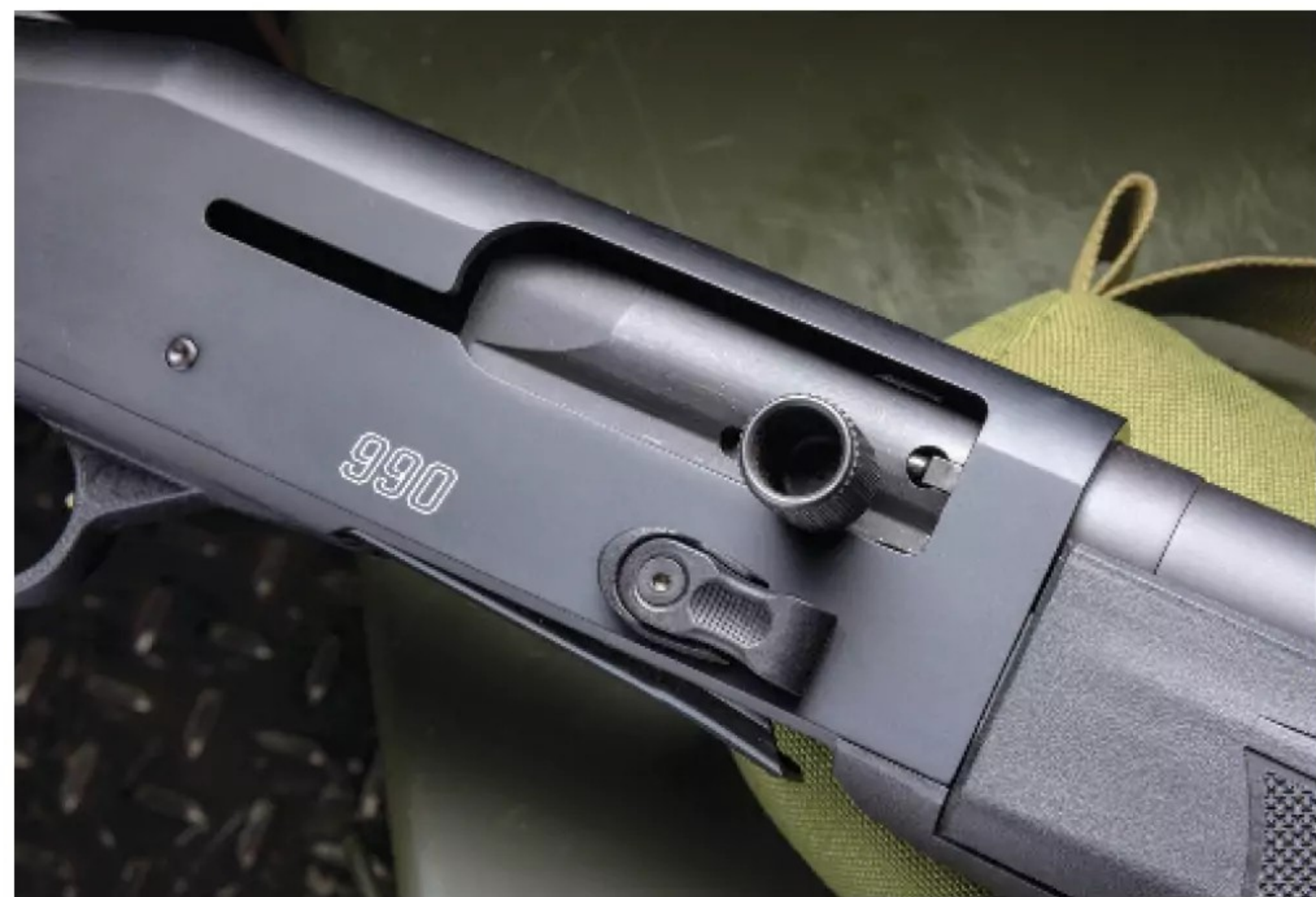
Expected on modern semiautomatic shotguns, the bolt handle and bolt release are enlarged and knurled. The bolt-release button is enlarged and protected by a fence against unintended use.
