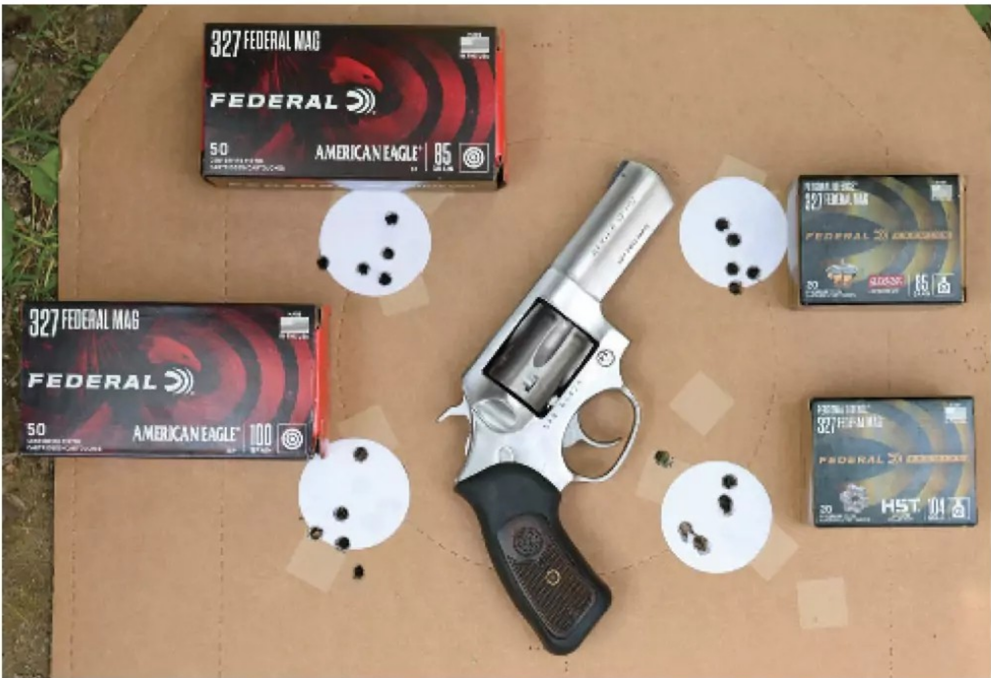
The muzzleblast from shooting the Federal’s modified Ruger SP101 development revolver in .327 Federal was hard work. However, the re-chambered revolver produced excellent groups at 25 yards.
