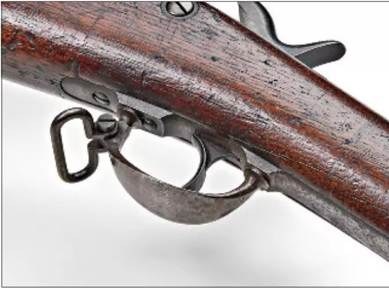
The Trapdoor Springfield retained the triggerguard from the 1863 Springfield muzzleloader. Note the rear sling keeper.
