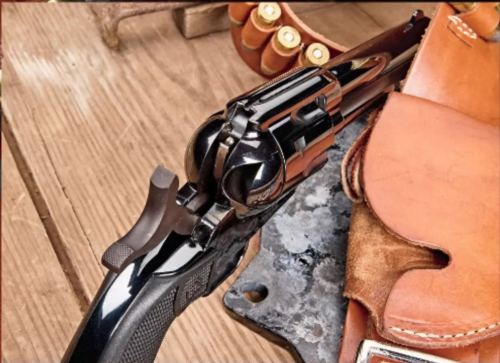
The Deputy incorporates a transfer bar to deliver the blow of the hammer to the firing pin. This means it does not have to be loaded with the hammer resting on an empty chamber, as does the original SAA.
