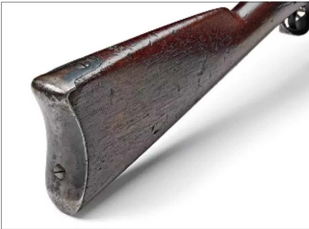
The Trapdoor Springfield also retained the curved steel buttplate from the 1863 Springfield.
