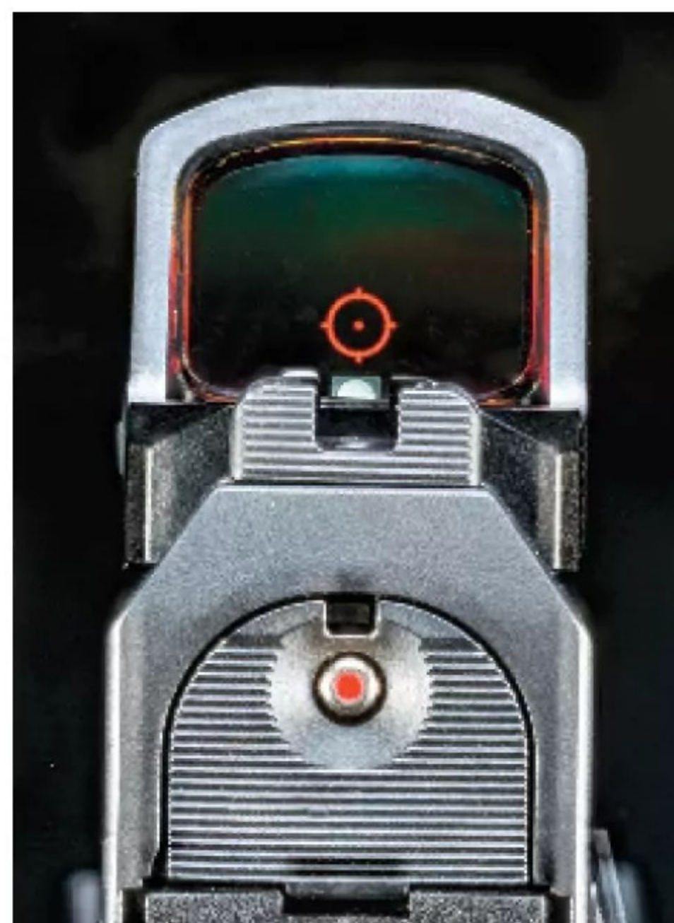
The optic cut is low to support alignment of the front and rear sights through many notched optic windows.
