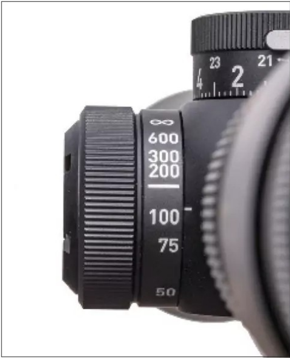
The left knob adjusts parallax. Markings range 50 to 600 yards, to infinity and beyond.
