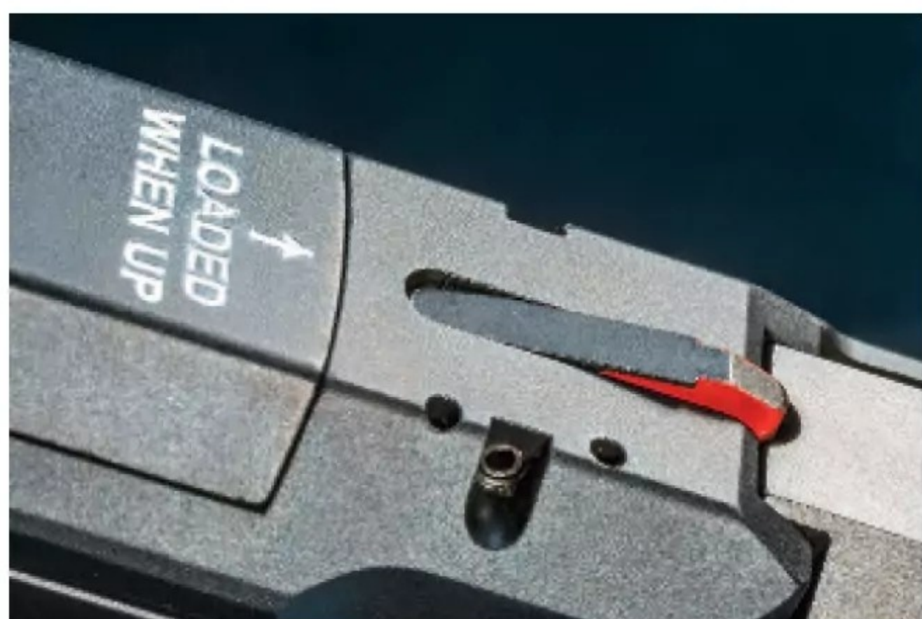
Engraved and prominent lettering along with a red-sided chamber indicator are requirements for CA-compliant pistols.
