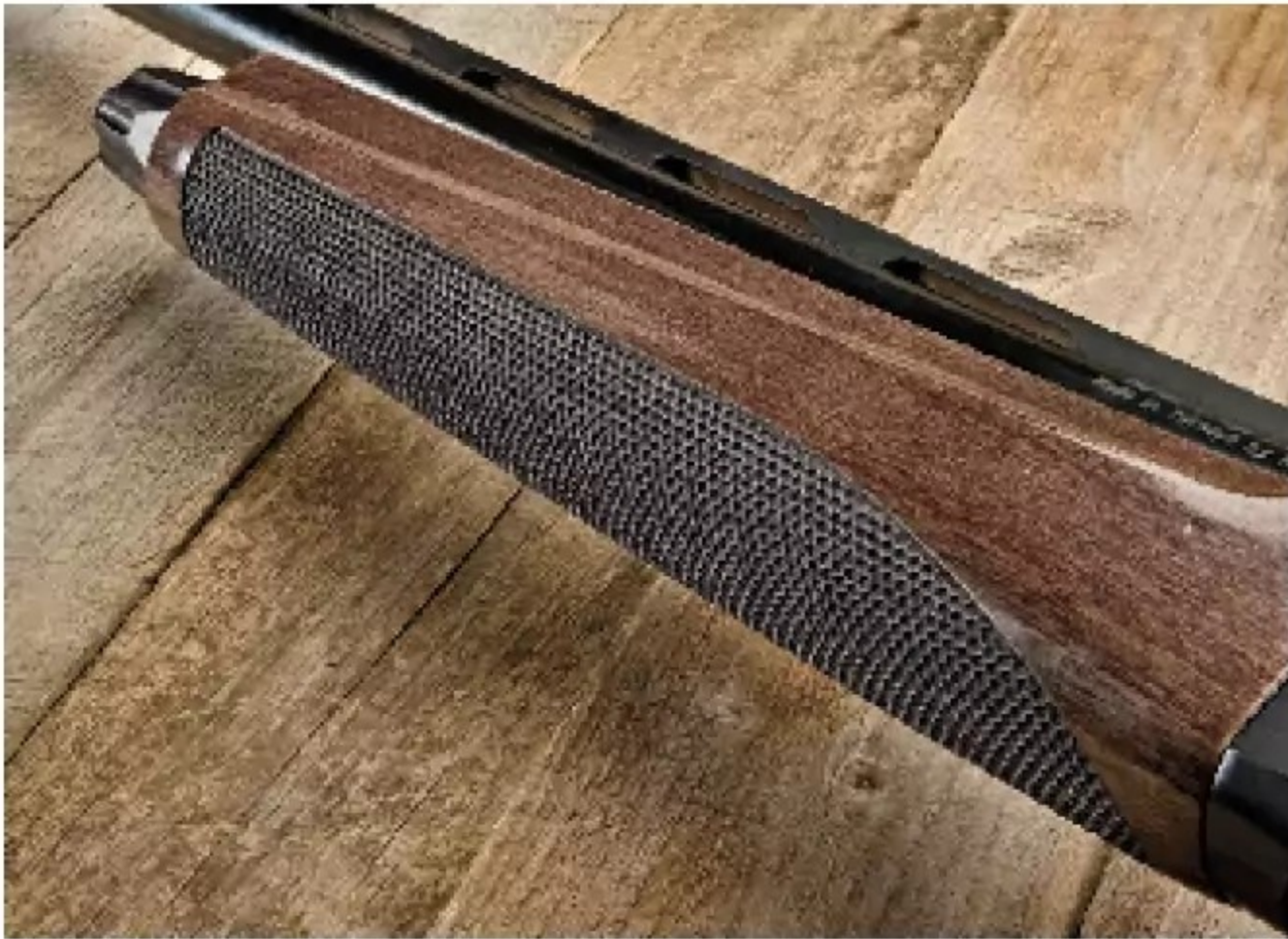
The texture on the grip and forend is a tactile, laser-engraved honeycomb pattern. It may not be as distinguished as hand-checkering, but it is a cost-conscious manufacturing method that enables effective control of the gun.
