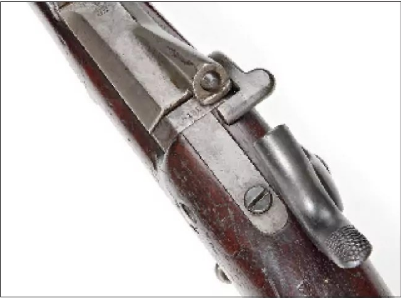
When released, a cocked hammer strikes the firing pin. The lever is lifted and the breech cover swung forward for loading.
