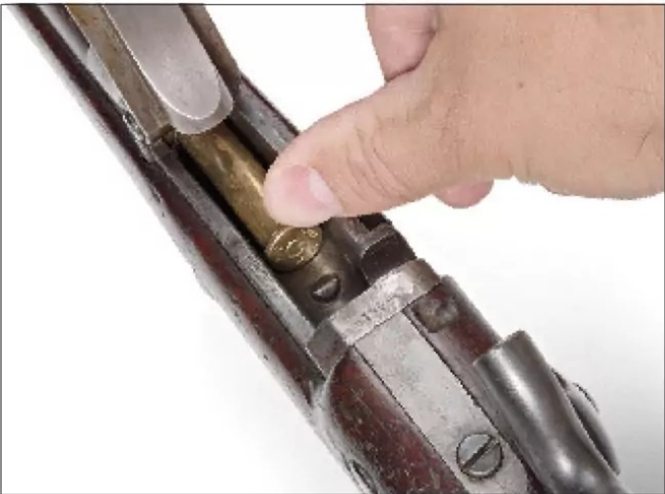
With the breech cover in the forward position, the action can be easily loaded with a self-contained cartridge.
