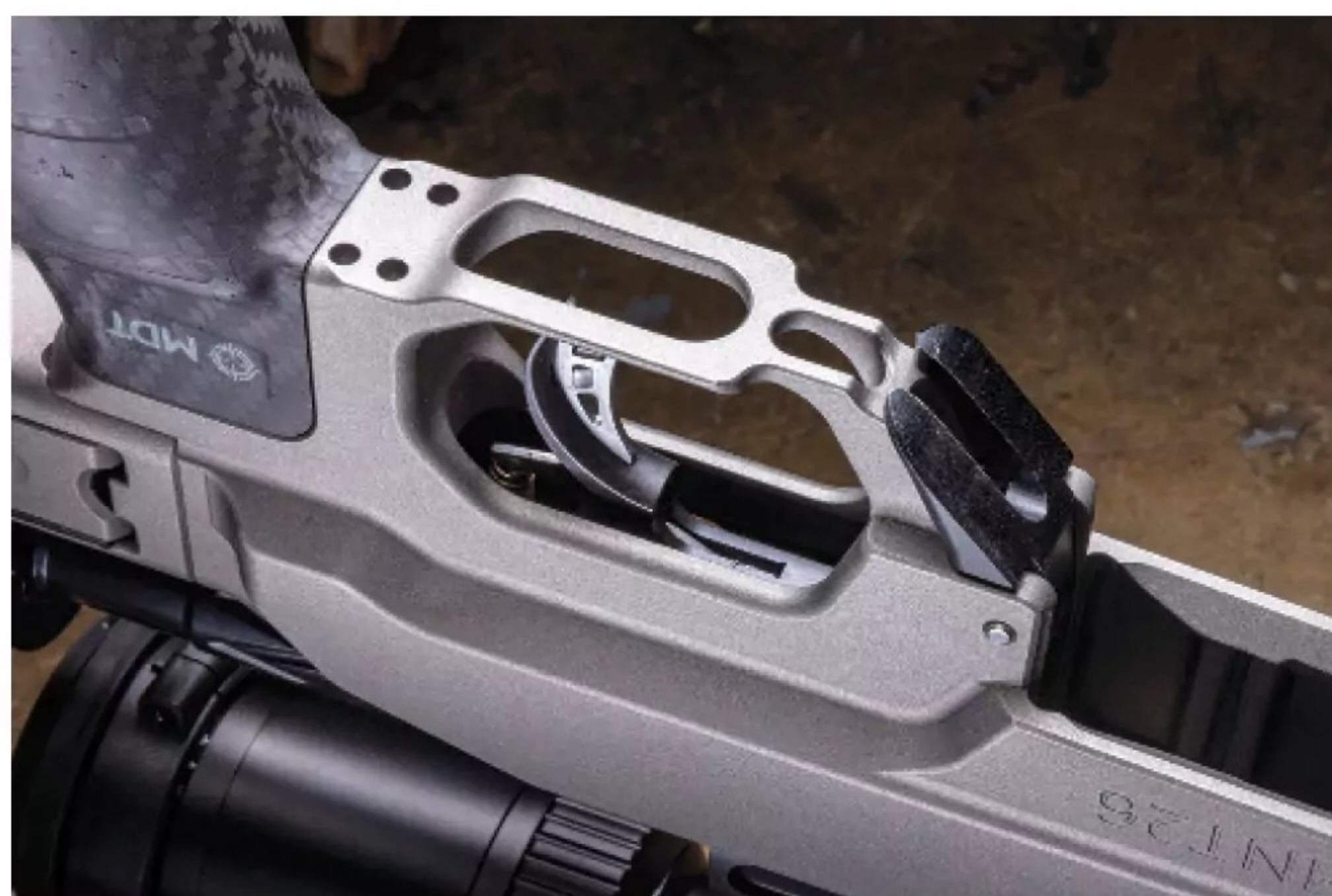
The mag release is a bilateral lever that's positioned forward of the trigger guard. The trigger guard is skeletonized for tool access.
