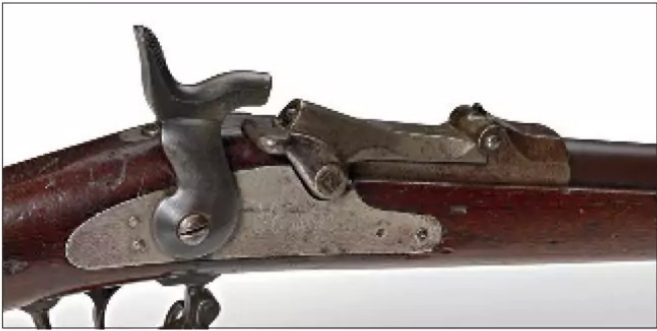
When released, a cocked hammer strikes the firing pin. The lever is lifted and the breech cover swung forward for loading.
