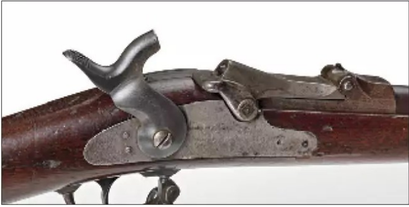
Trapdoor Springfields were equipped with a two-position conventional muzzleloader-type hammer. The hammer was raised to half-cock (above, middle) for a safe and load position. Fully raised, the hammer is in the ready-to-fire position (above, bottom).
