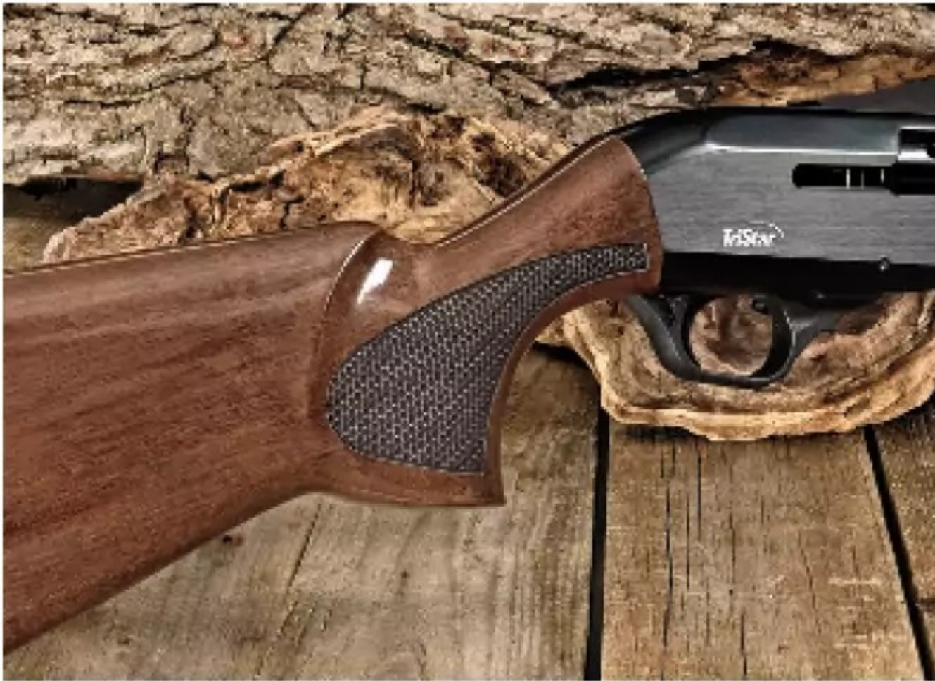
The texture on the grip and forend is a tactile, laser-engraved honeycomb pattern. It may not be as distinguished as hand-checkering, but it is a cost-conscious manufacturing method that enables effective control of the gun.
