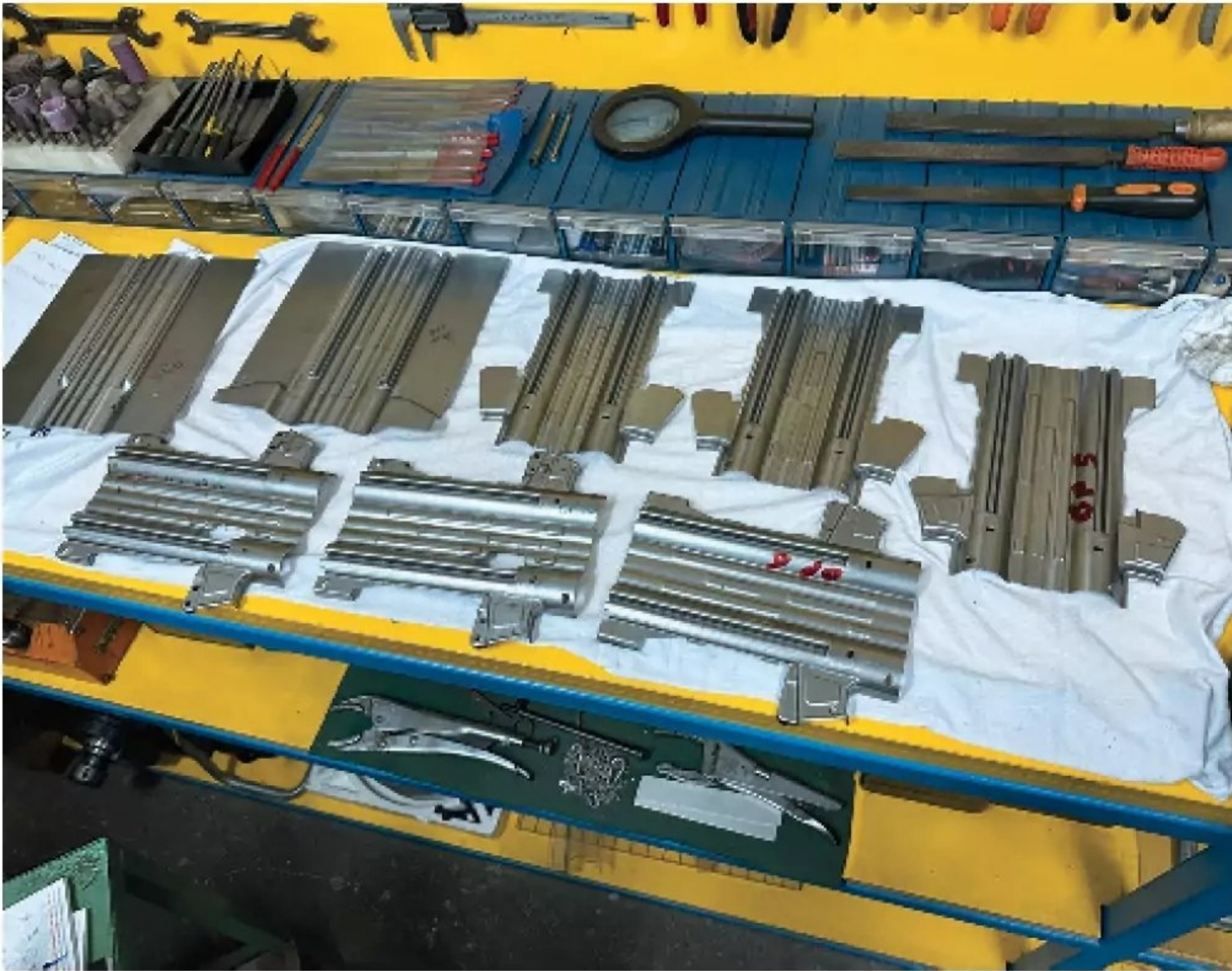
These receivers illustrate the multiple stages of stamping and die-cutting MAC 5-series receivers before they are folded over tooling and fitted with a barrel, sights and subassemblies.
