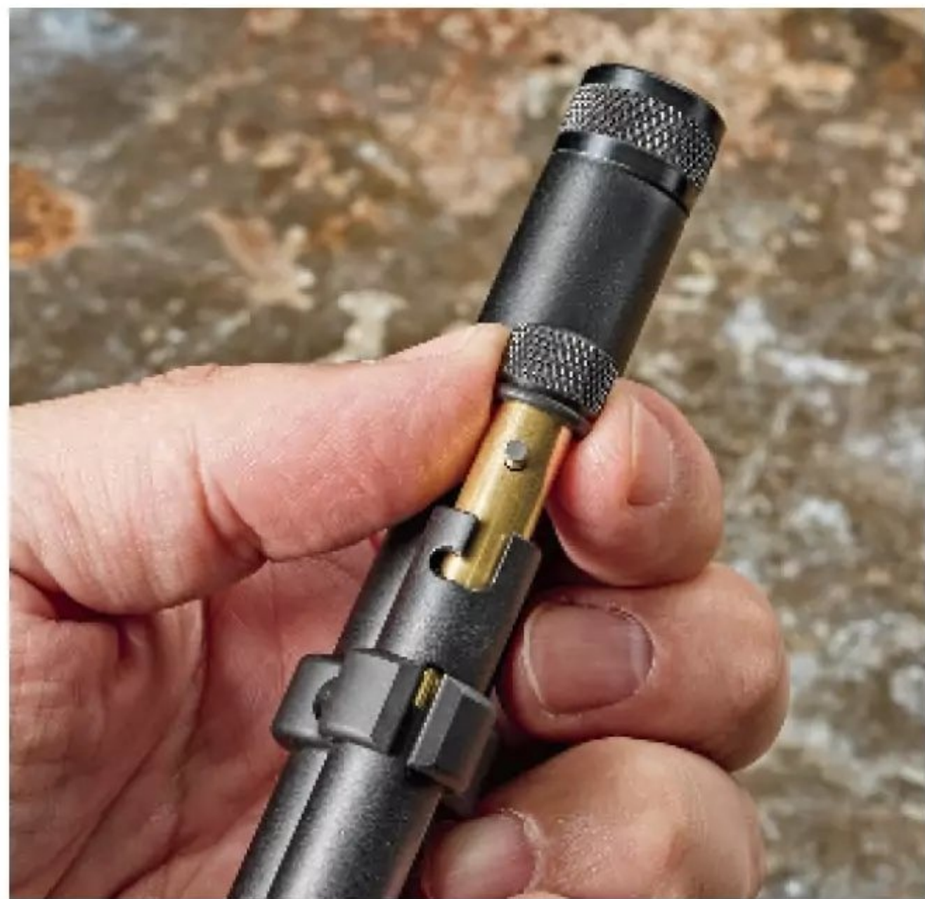
Loading the 12-round tubular magazine is a simple process. Start by twisting and removing the magazine's guiderod.
