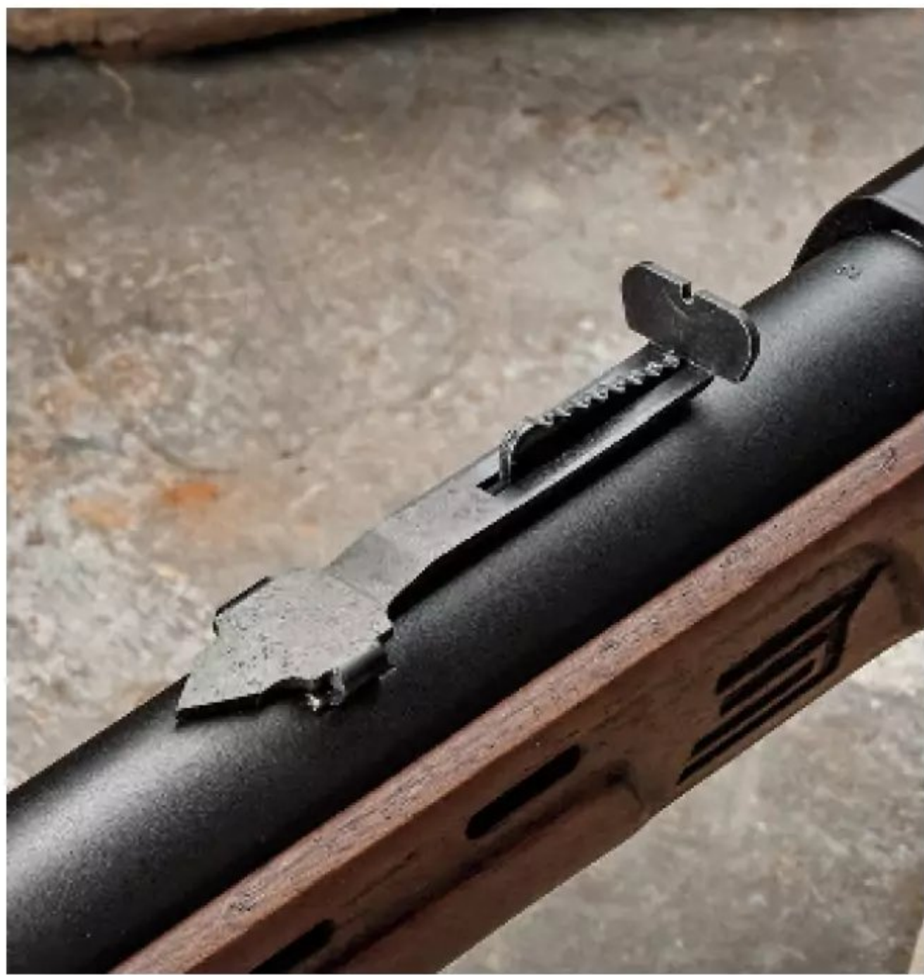
The Savage Revel DLX and Classic models share the same notched rear sight. The rear sight is adjustable for elevation.
