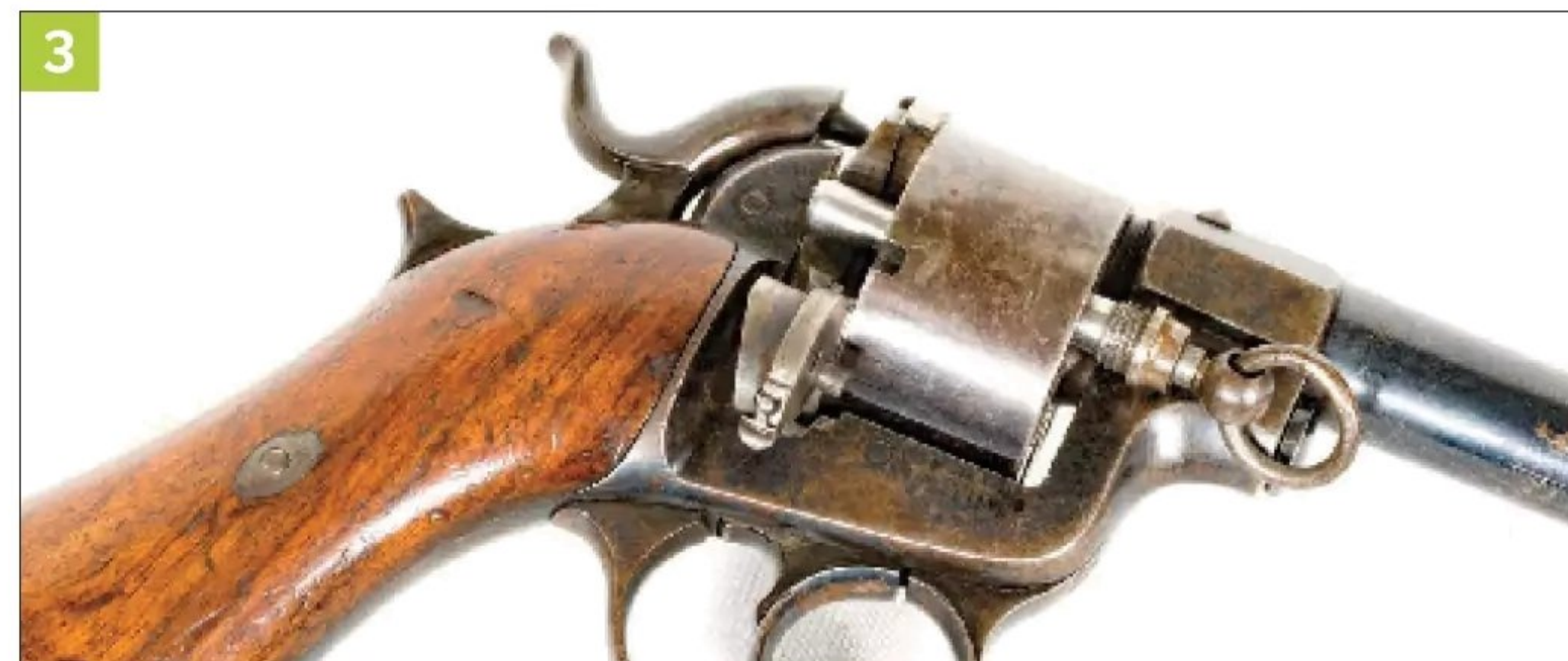
The Raphael employed a separate backplate that unlocked from the cylinder body when the loading gate was opened [1] [2]. Ejection of spent cases was accomplished by a rod with an attached lanyard ring that was unscrewed from the base of the revolver's grip [3].
