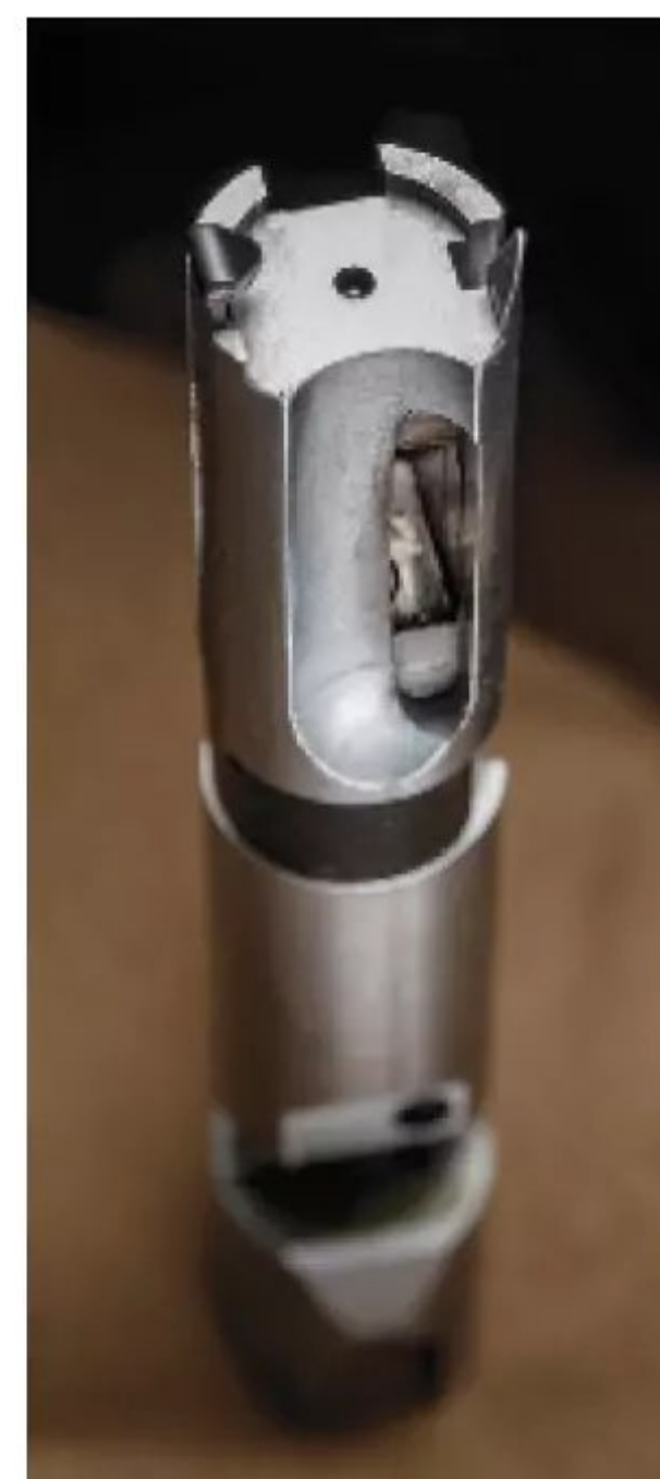
As an added safety measure, the two-piece firing pin only aligns when the lever is in the closed position.
