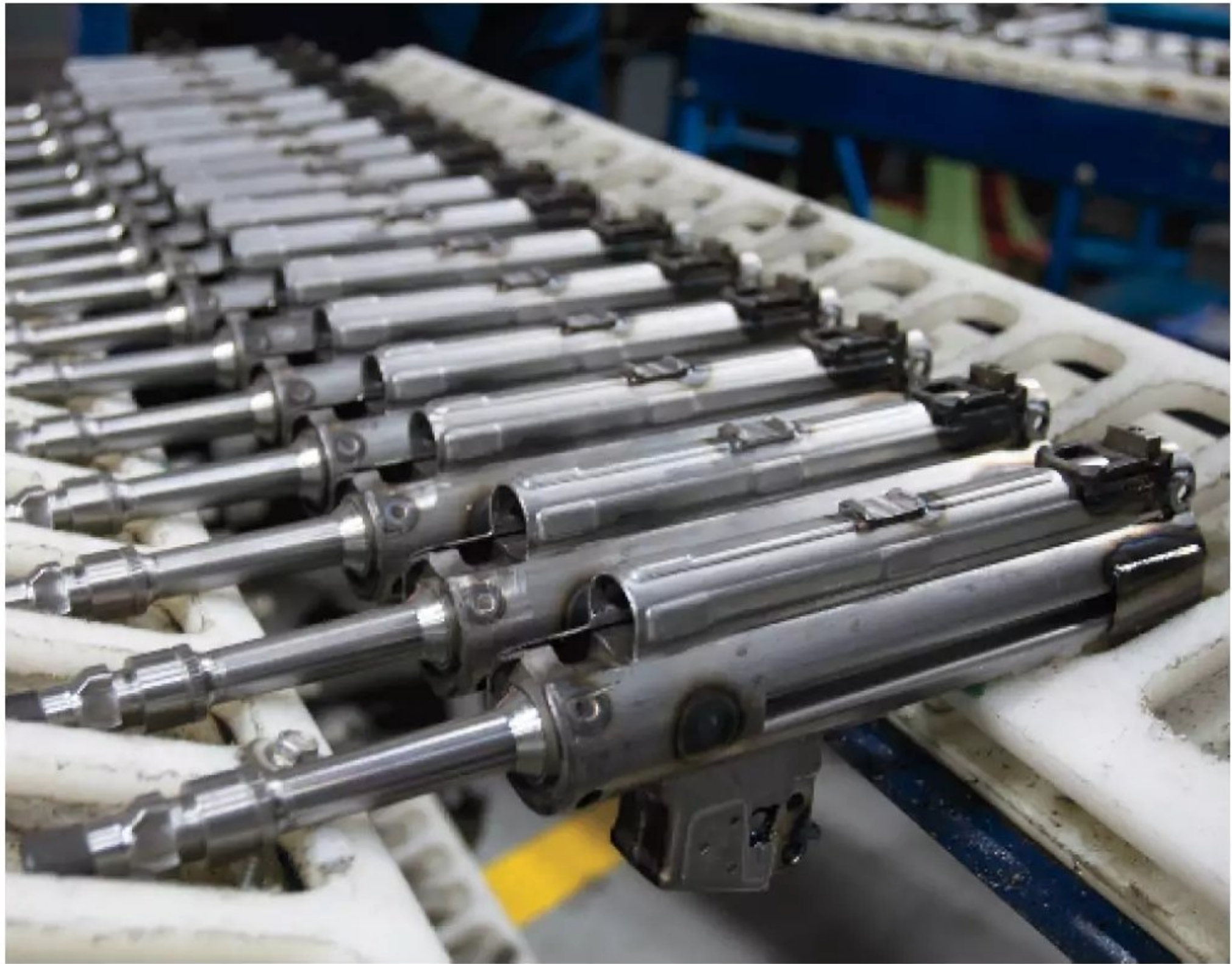
Receivers and barrels are welded with sight bases, magazine well, and a block for reinforcement at the rear. The 5.8-inch barrel indicates these will be MAC 5K models.
