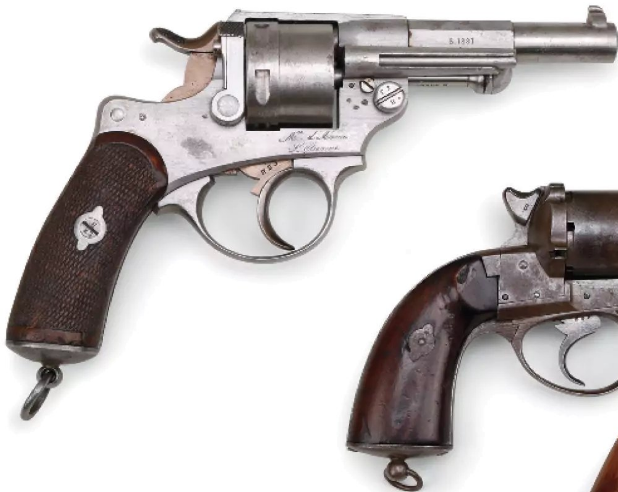
The superb 11mm Model 1873 French Service revolver was rugged, reliable and possessed of an excellent double-action mechanism. These revolvers saw service from the early 1870s through World War II as provisional arms.
