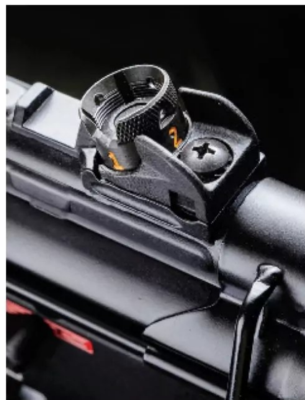
True to the HK original, the Century Arms AP53 features a protected post at the front and a four-position drum at the rear. The rear sight can be zeroed for windage and elevation with a screwdriver.
