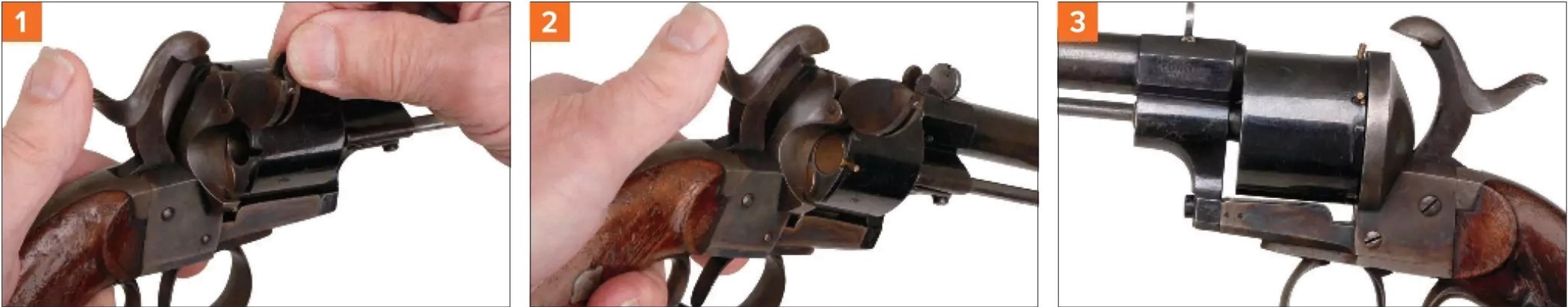
The pinfire was the earliest successful self-contained cartridge system. It continued in use in longarms and handguns for a considerable time. Though many styles abounded, the typical Lefauchaux revolver loaded its rounds through an upswinging loading gate [1] [2]. The most vulnerable aspect of the system was the protruding pins, which could be struck causing an accidental discharge [3].
