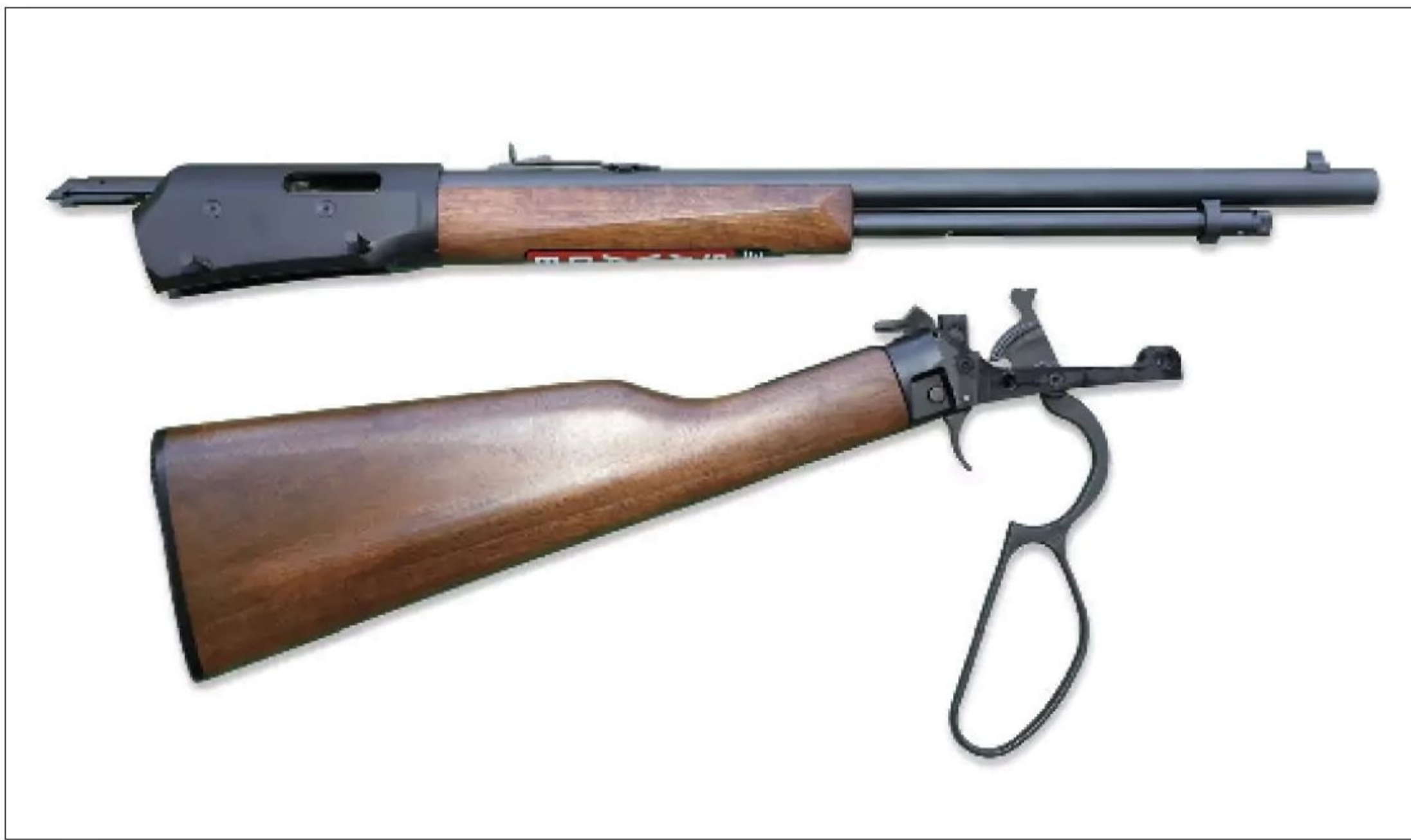
Savage Revel lever-actions are takedown rifles, handy for trail and backpack use. At the bottom of the receiver, above the trigger, the left-to-right captive takedown pins are visible. To disassemble or reassemble, the lever must be down, bolt open and safety engaged.
