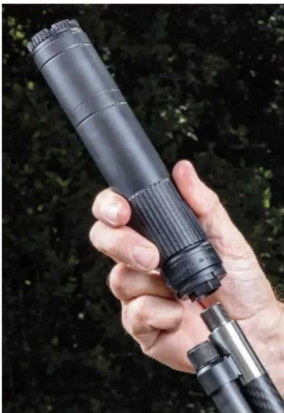
As the model name suggests, the SPD HUSH is ready for use with suppressors. Threads are 5/8x24 for this Henry rifle.
