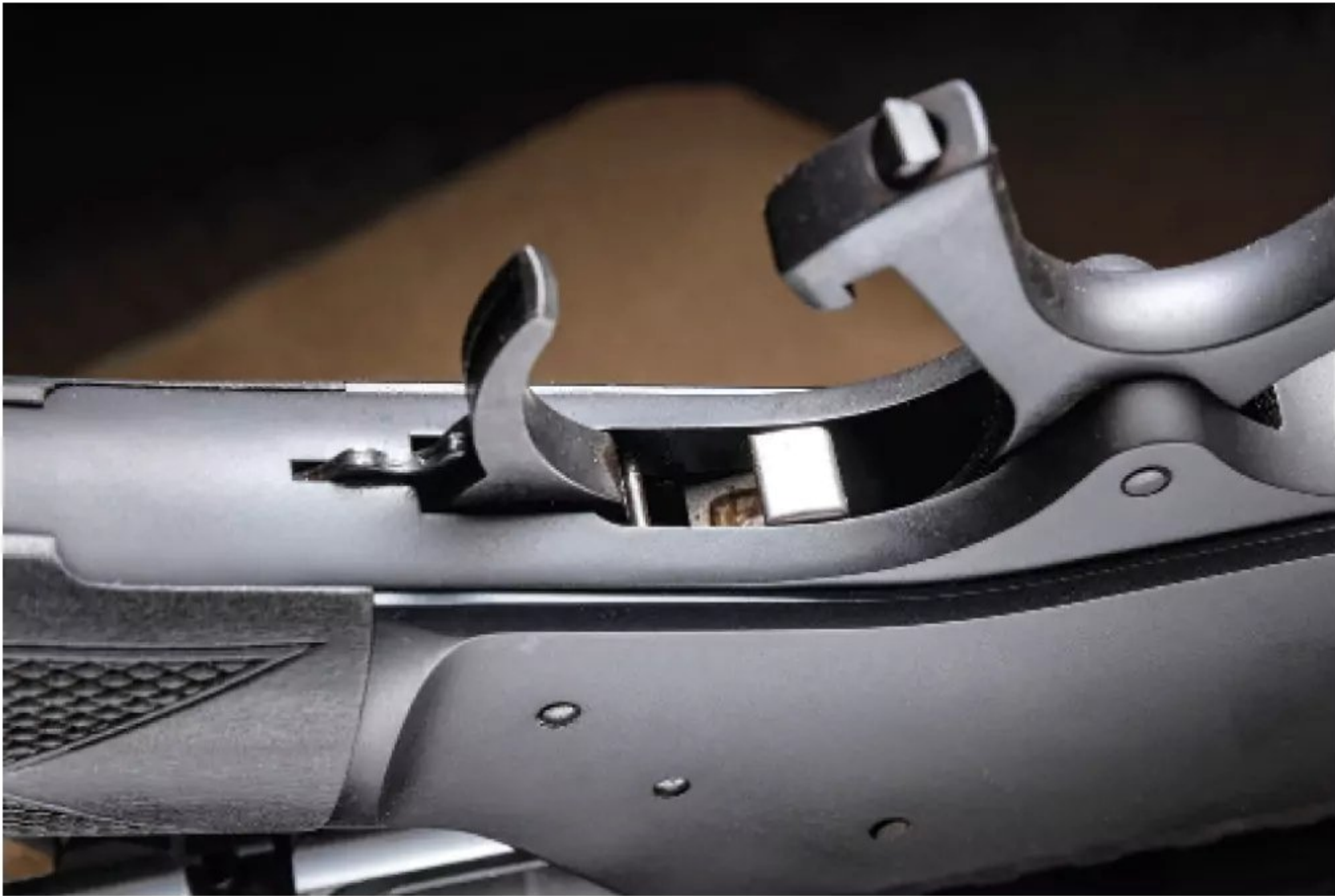
The trigger on the SPD HUSH is on par with most lever-action rifles. G&A's test rifle produced a 6½-pound trigger on a Lyman gauge.
