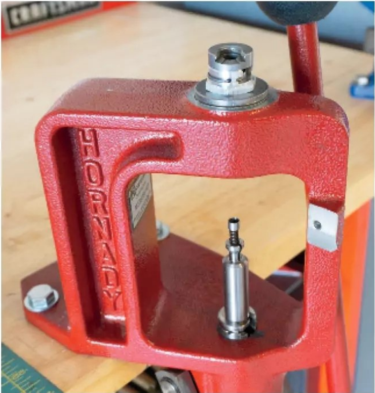
Figure 5: The Lee Ram Prime System can ensure identical seating depth in primers from load to load. $22
