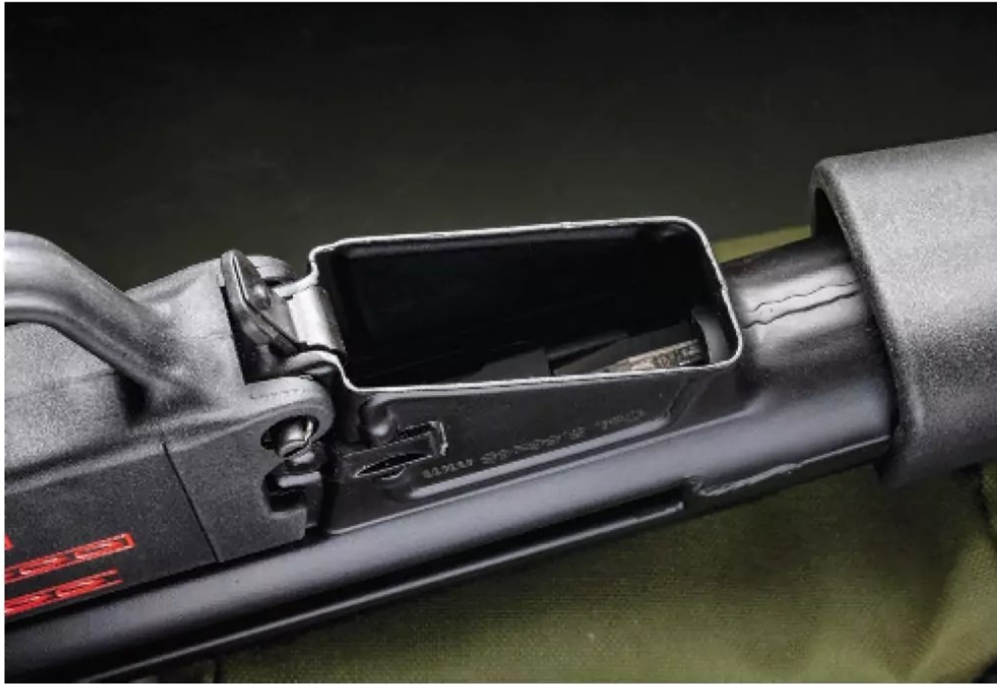
The AP53's magazine well has been enlarged slightly versus the original HK design. This effort improved reliability with different magazines. Magazines insert straight into the magwell for operation.
