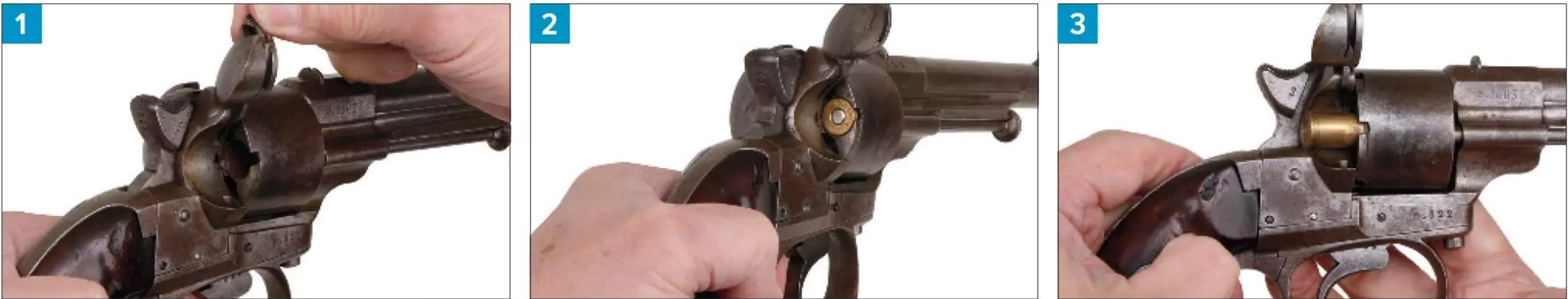
The Model 1858T Naval Revolver loaded and ejected cases in a now-familiar fashion [1] [2]. The pinfire holes were not removed during the centerfire transformation and can still be seen at the rear of the chambers [3].
