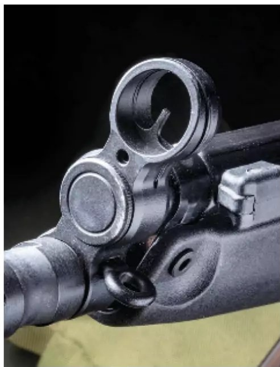
True to the HK original, the Century Arms AP53 features a protected post at the front and a four-position drum at the rear. The rear sight can be zeroed for windage and elevation with a screwdriver.
