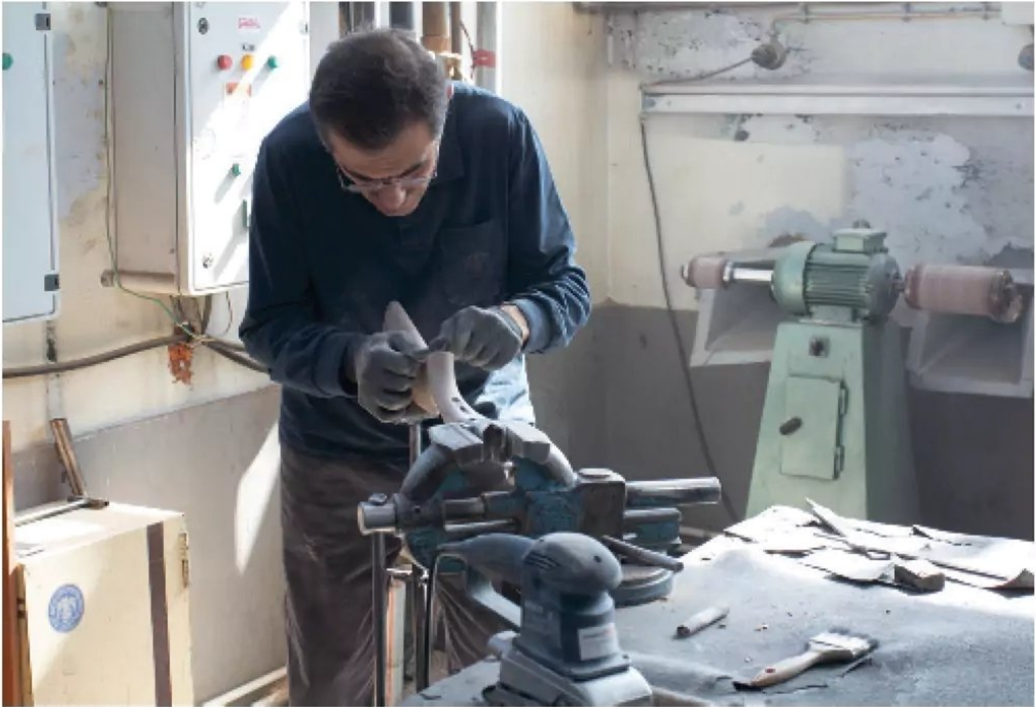
Surrounded by hand tools and working over a vise, a long-time employee at Huğlu sands and blends a wooden stock to a shotgun receiver with careful attention to detail.
