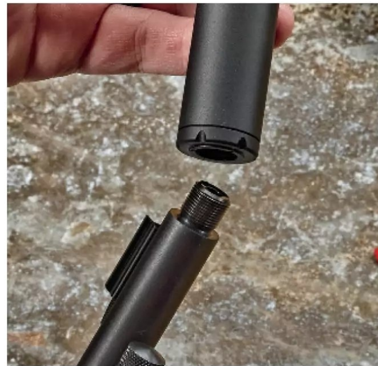
The Savage Revel DLX includes a 1/2-28 threaded barrel for use with rimfire suppressors. With a static bolt, it's quiet to shoot.
