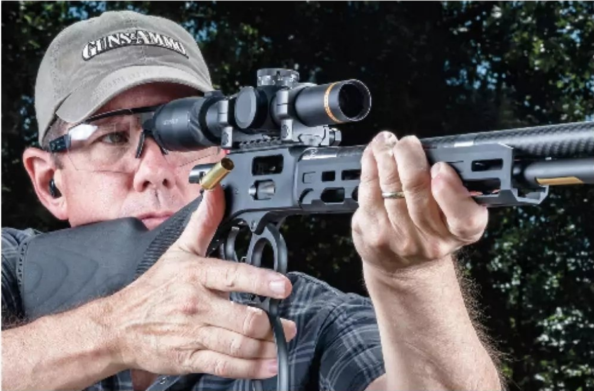
The trigger on the SPD HUSH is on par with most lever-action rifles. G&A's test rifle produced a 6½-pound trigger on a Lyman gauge.
