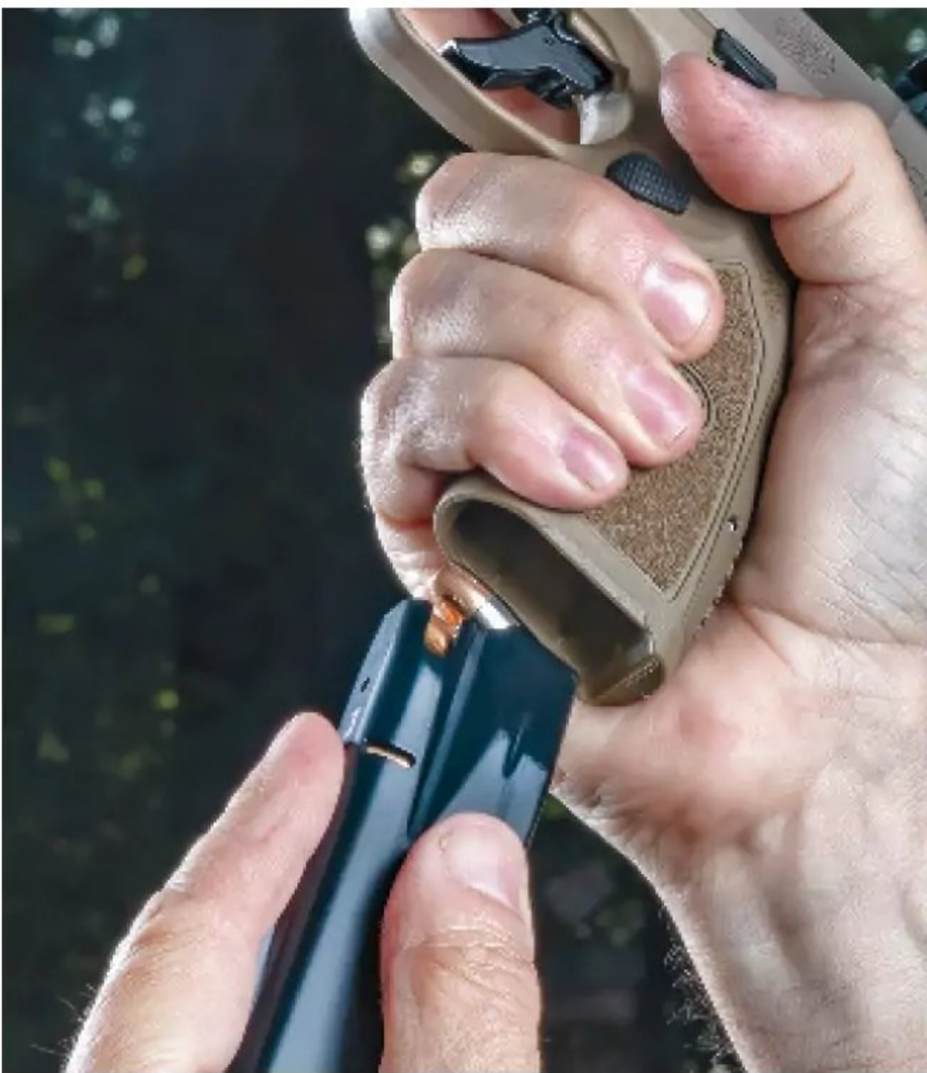
The extended XL grip added four rounds to the Reflex. The extended basepad adds another three for a total of 18 rounds.
