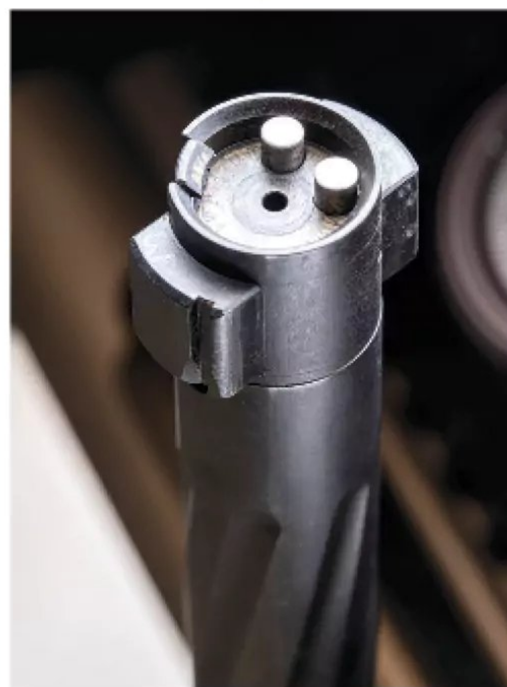
The bolt contains a 32-pound firing pin spring that provides lightning-fast lock time and reliable ignition. The bolt head features a claw extractor and dual ejectors to kick out large magnum cases.
