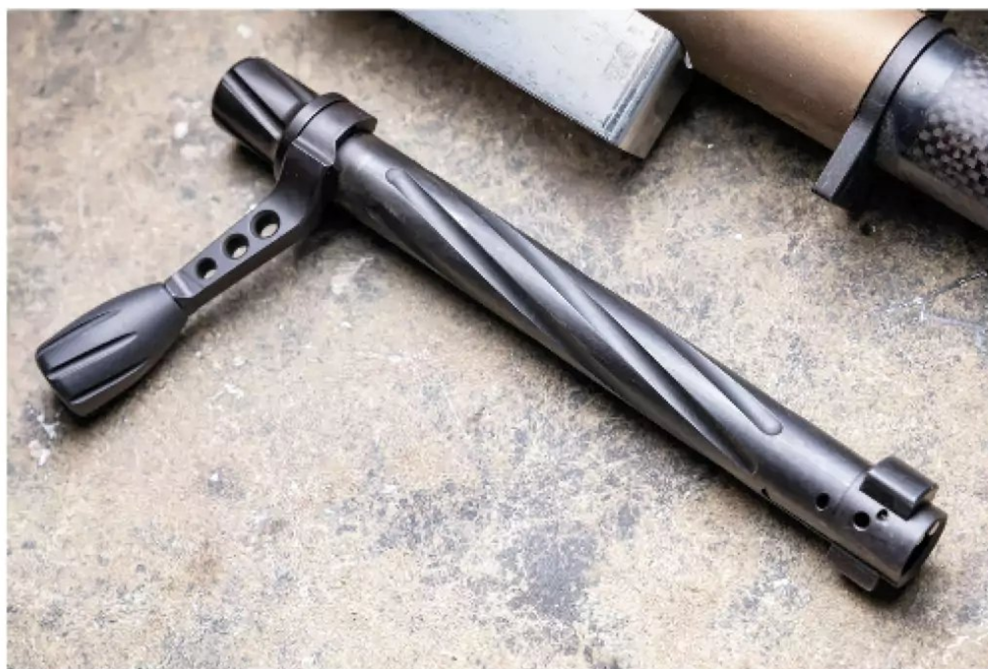
The bolt contains a 32-pound firing pin spring that provides lightning-fast lock time and reliable ignition. The bolt head features a claw extractor and dual ejectors to kick out large magnum cases.
