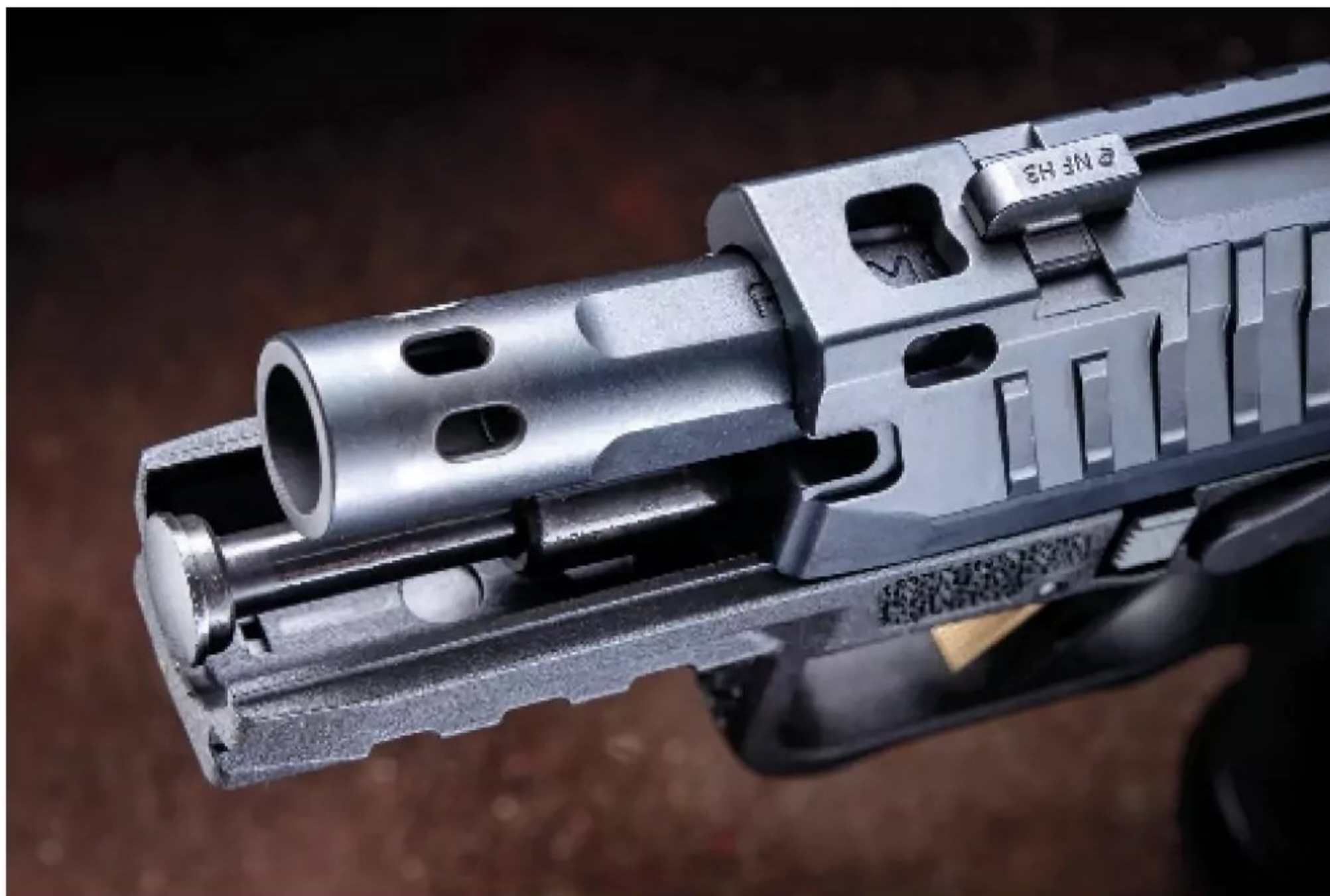
Not simply an aesthetic detail, the barrel features three compensating ports and cutouts in the slide to tame muzzle rise.
