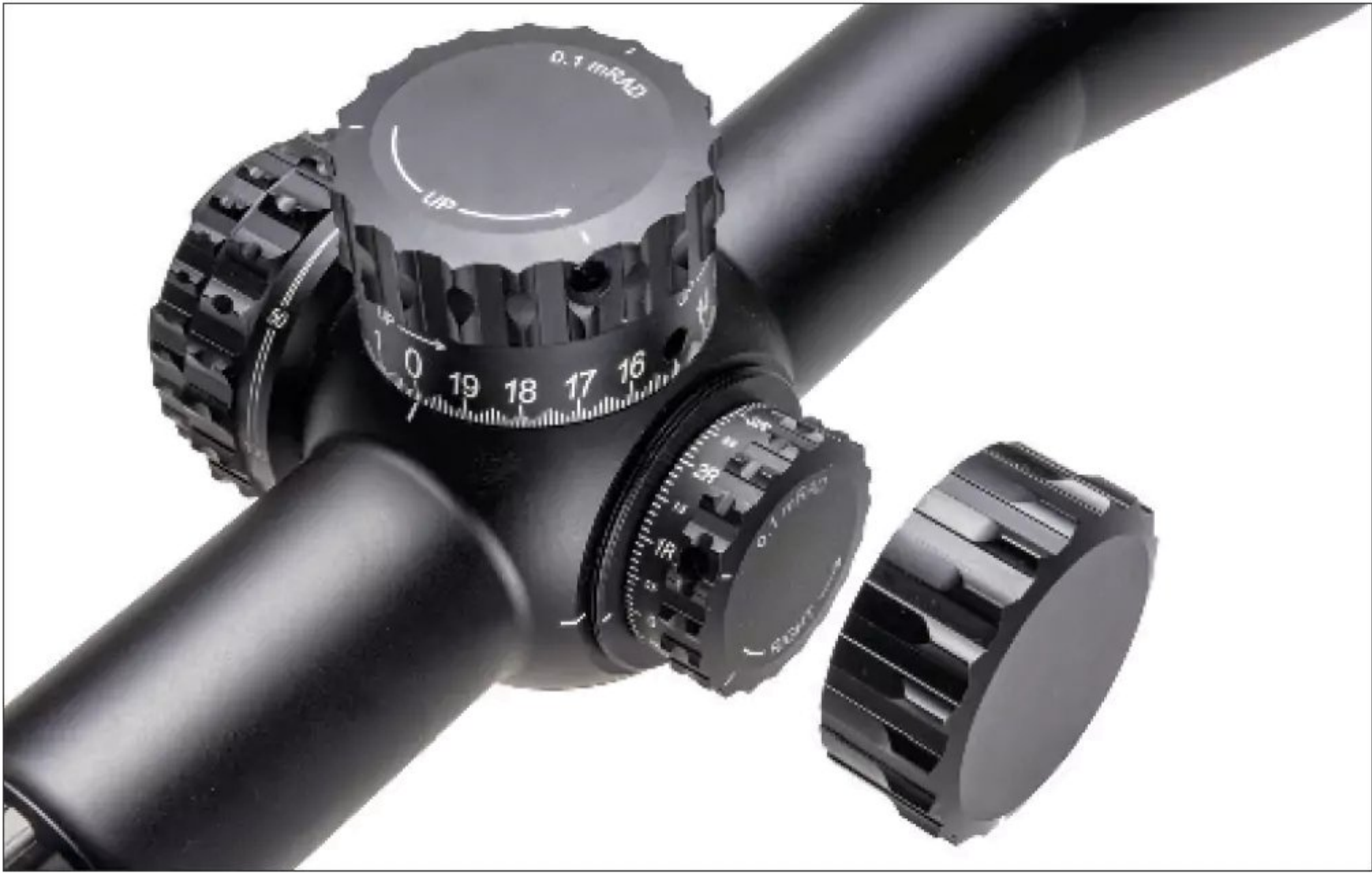
The elevation turret is exposed to quickly adjust for target distance. The windage turret is capped for protection. Both feature .1 MRAD (mil) adjustments per click, laser engraved with directional arrows.
