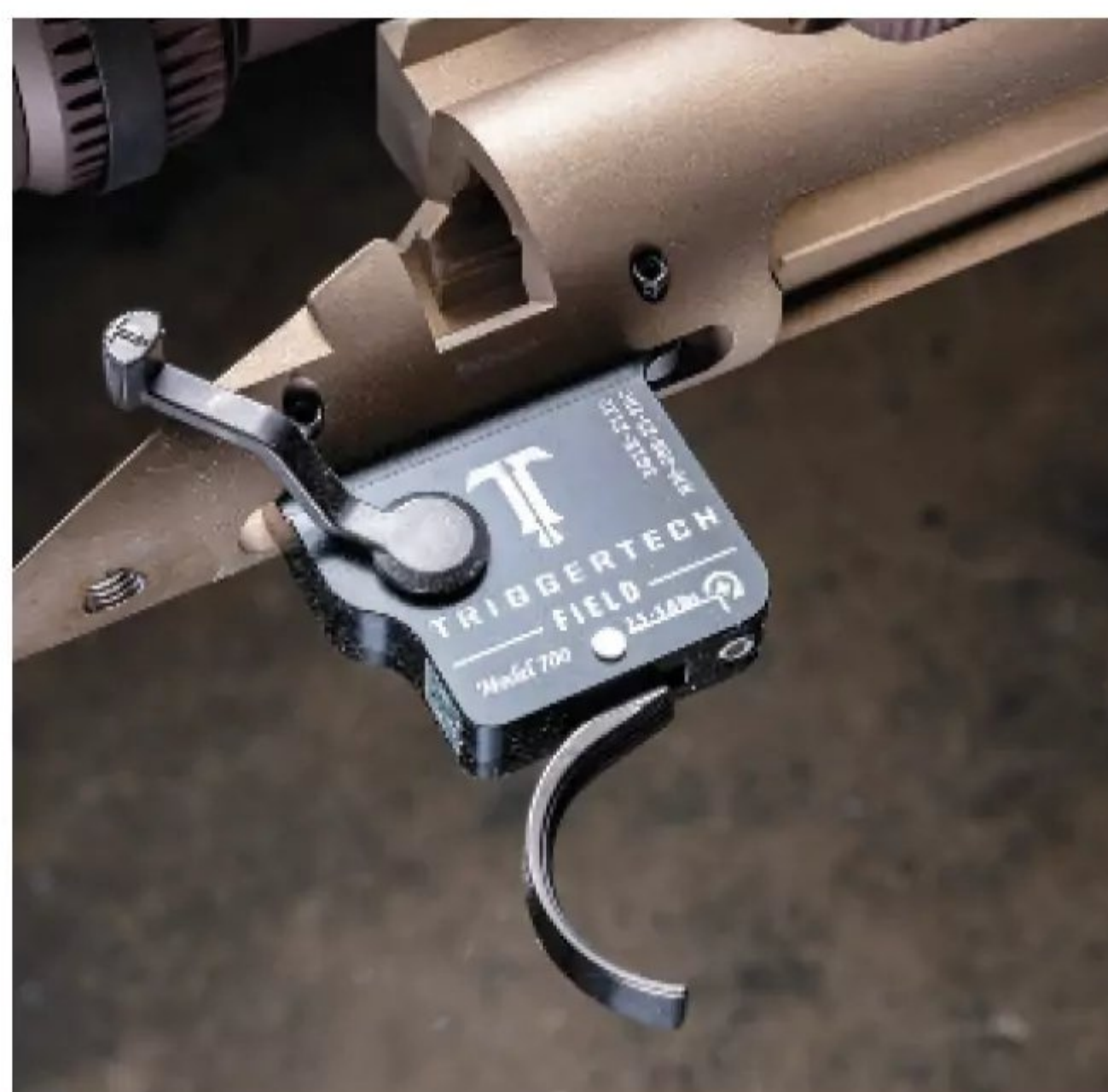
The TriggerTech Field trigger has an adjustment range between 2½ and 5 pounds; thumb safety lever included.
