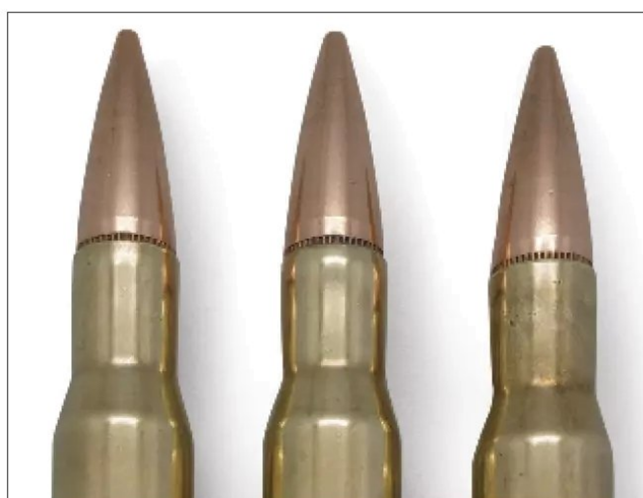
Left to right: A roll crimp compared to an excessive roll crimp with bulged neck, and a taper crimp with a shallow crimp angle at the case mouth.
