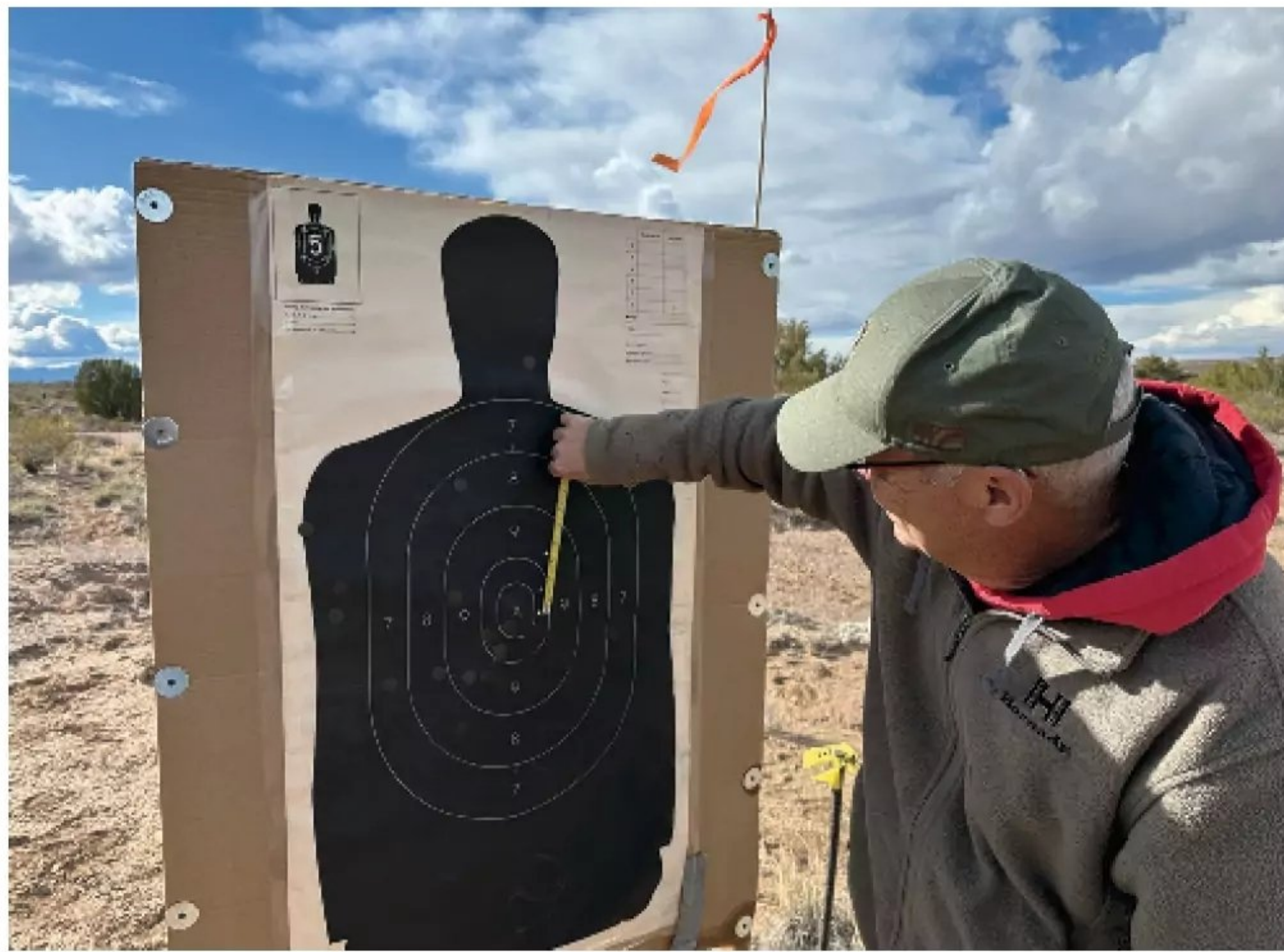
Rifles were compared on a remote New Mexico range using a bullseye for zeroing and 100-yard accuracy testing, followed by three-shot groups on silhouette targets from 200 to 500 yards.
