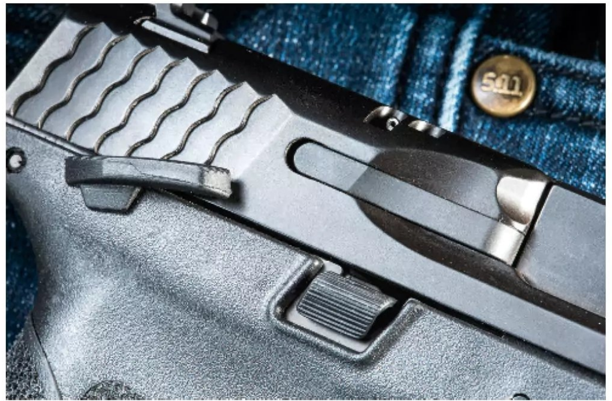
The thumb safety lever and slide release are bilateral controls.
