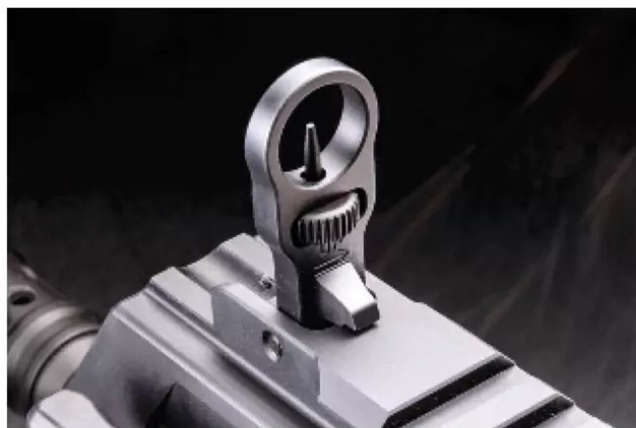
When folded, a fixed, pistol-type dot sight is available. When raised, the needle-post front sight is adjustable for precision.
