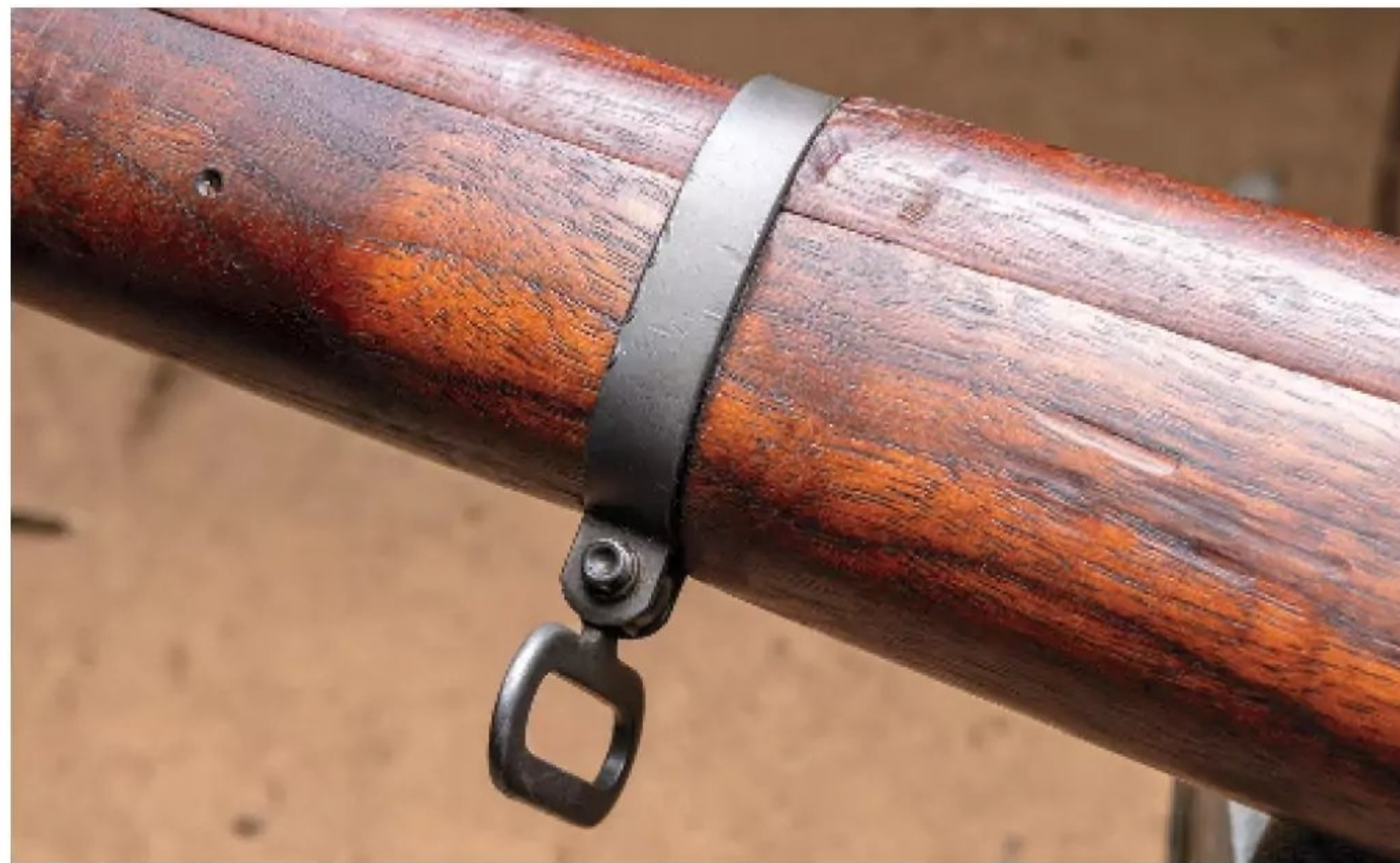
The M1903A4 used the easier-to-produce stamped-steel barrel bands and forend cap of the M1903A3. The M1903A4 did not have sights besides the the Weaver 330-C/M73B1 scope.
