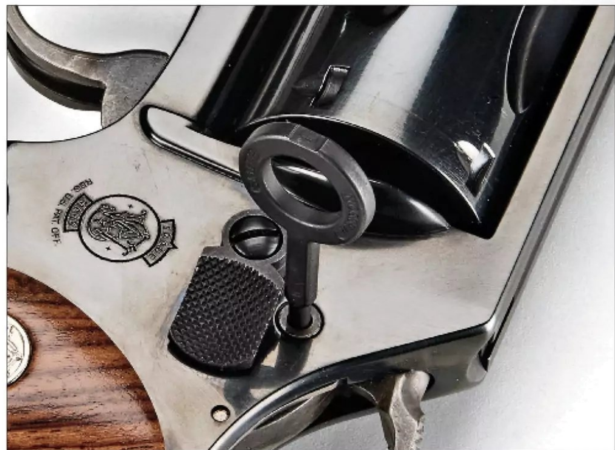
Many revolver enthusiasts objected to locks on both aesthetic and mechanical grounds since their introduction. The lock was often located above the cylinder release latch and required a key.
