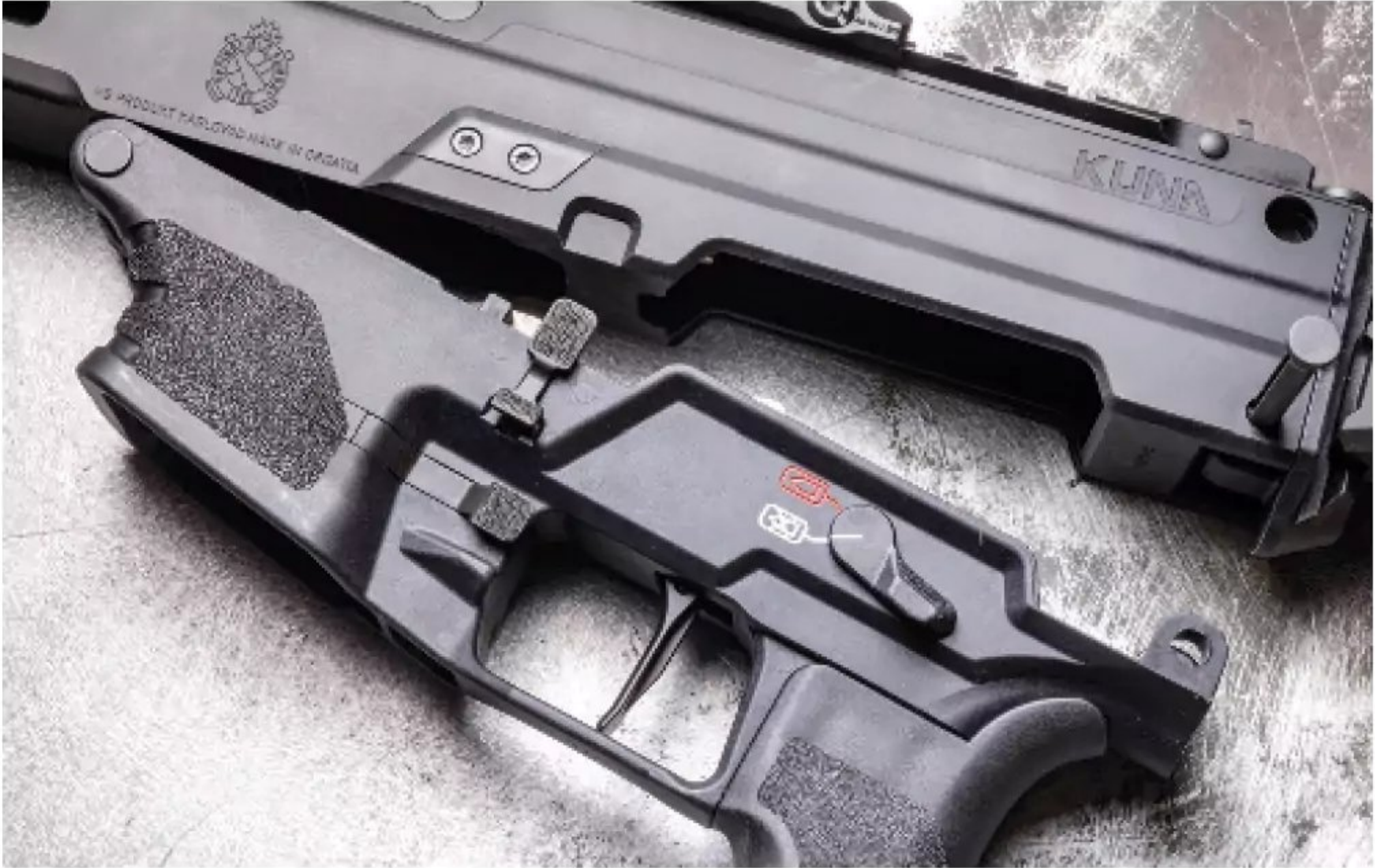
A monolithic aluminum upper receiver is secured to the polymer composite lower by two captured takedown pins. The bolt catch/release, selector and mag release are familiar to AR users.
