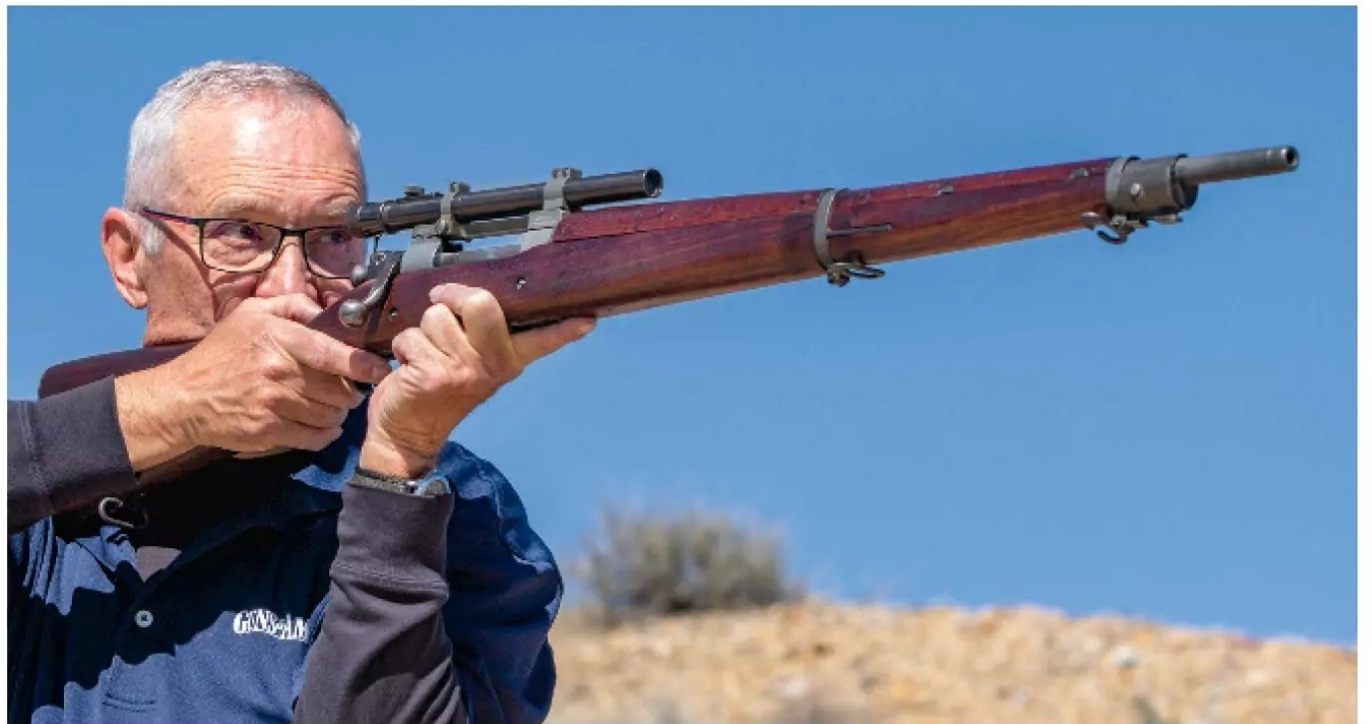
The M1903A4 was an accurate and effective sniper to 400 yards. It was the lightest of the World War II sniper rifles tested. Scope turrets offer quarter-MOA adjustments, too.
