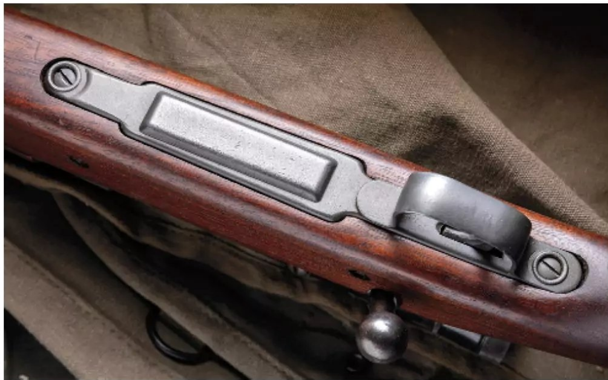
The M1903A4 used the same simplified, stamped floorplate and triggerguard from the M1903A3.
