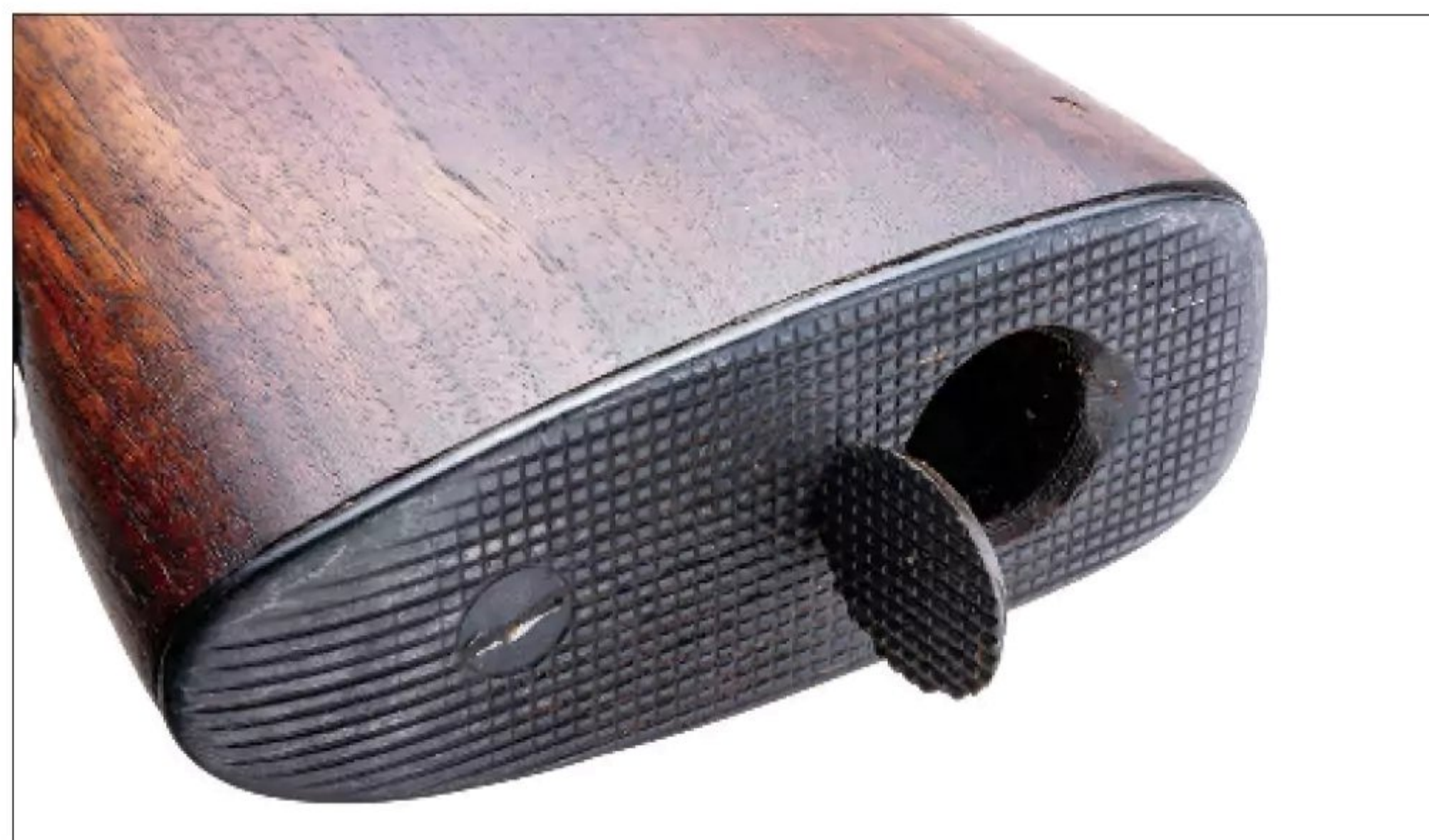
The M1903A4 had the A3 buttplate, which had a trapdoor feature to access a compartment often used to hold a cleaning rod.
