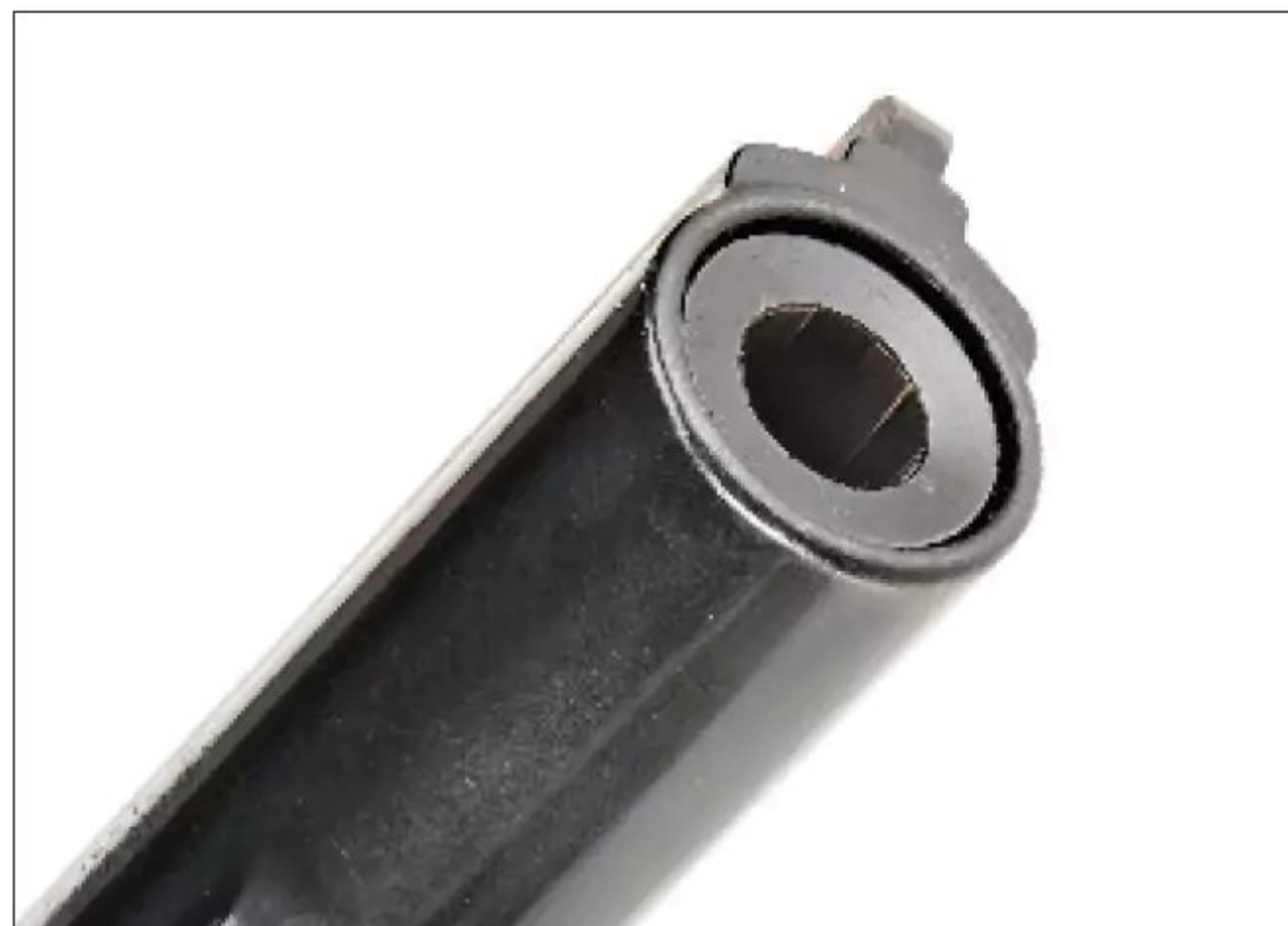
The Model 19 Classic uses Smith & Wesson's modern sleeve-over-barrel approach, which improves its accuracy potential.
