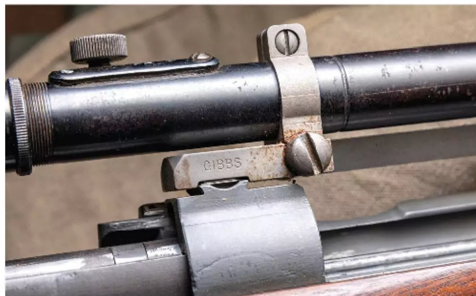
The Weaver Model 330-C scope was selected for the M1903A4, later designated the "M73B1." These had drum-shaped knobs.
