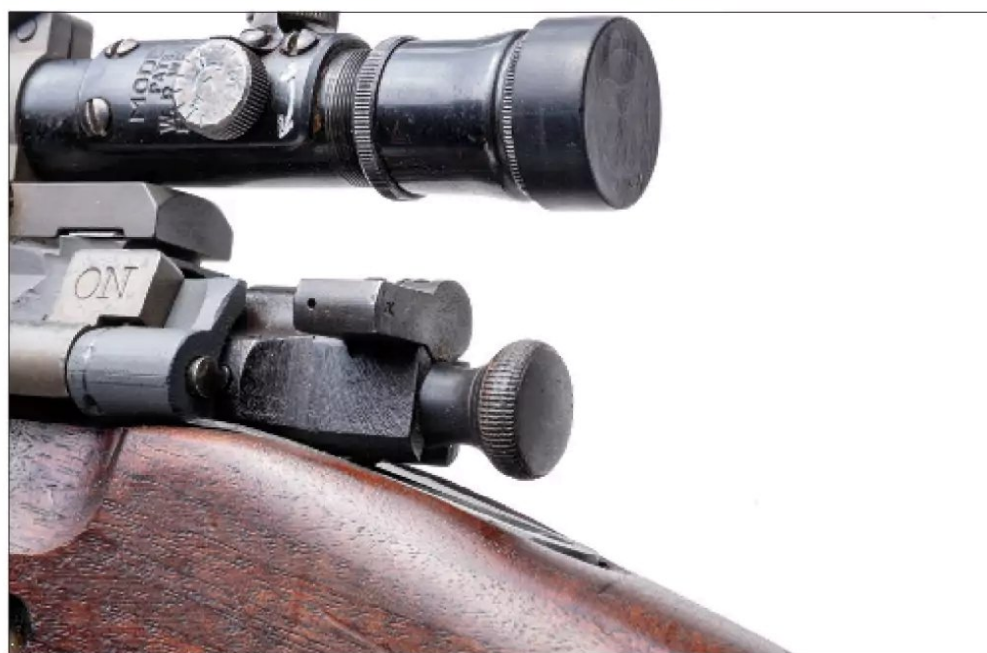
The M1903A4 safety was a copy of the Mauser Model 98 safety with three positions: Fire, a safe position that allows the bolt to open, and safe with the bolt locked closed.
