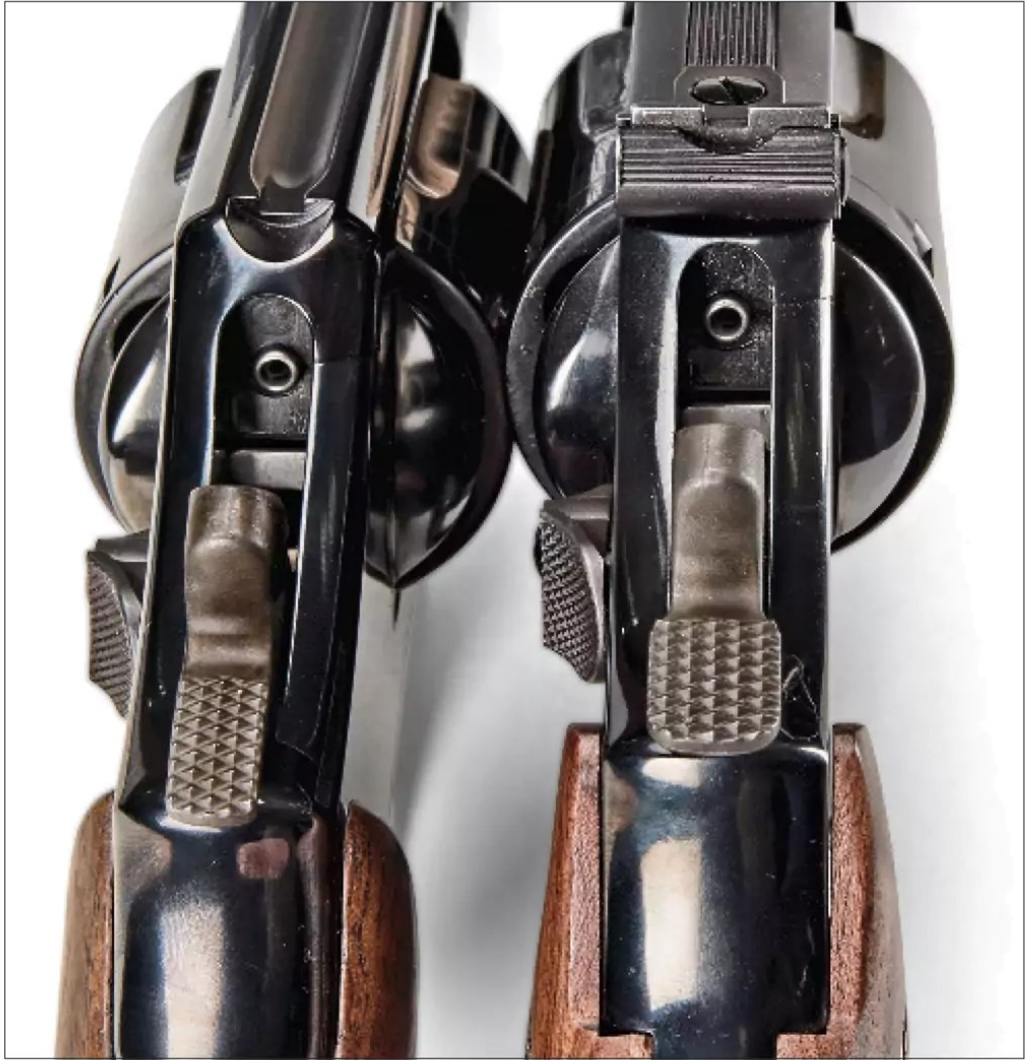
The firing pin in S&W revolvers migrated to the frame in 1997 for more consistent ignition. The Model 10 features a fixed notch in the topstrap while the Model 19 sports an adjustable rear sight.
