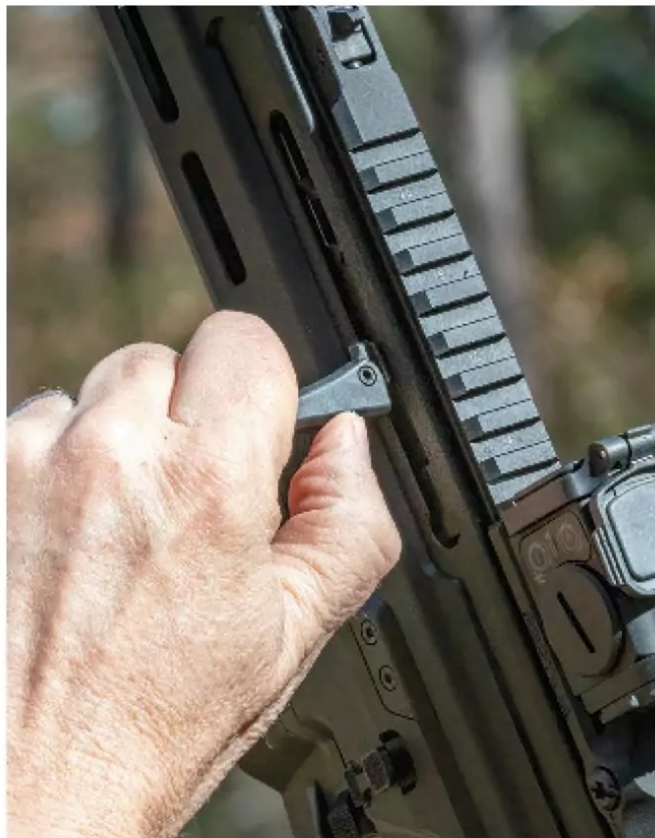
The charging handle is a non-reciprocating design that also folds forward when not in use. The handle can be reversed, also.
