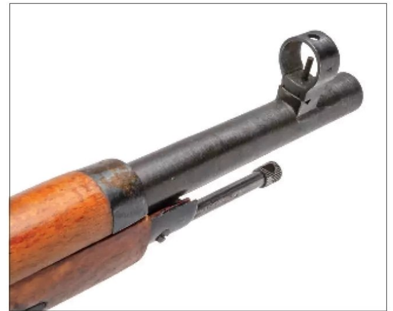
The Type 2 hooded post sight was used on the 91/30 and is unmarked except for an alignment index mark on the front.
