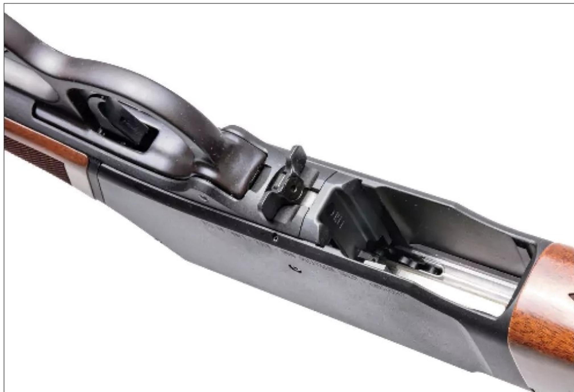
The magazine clears the movement of the lever when racked and displays little movement due to the engineered shape within the magwell. Press the paddle lever behind the magwell to remove.
