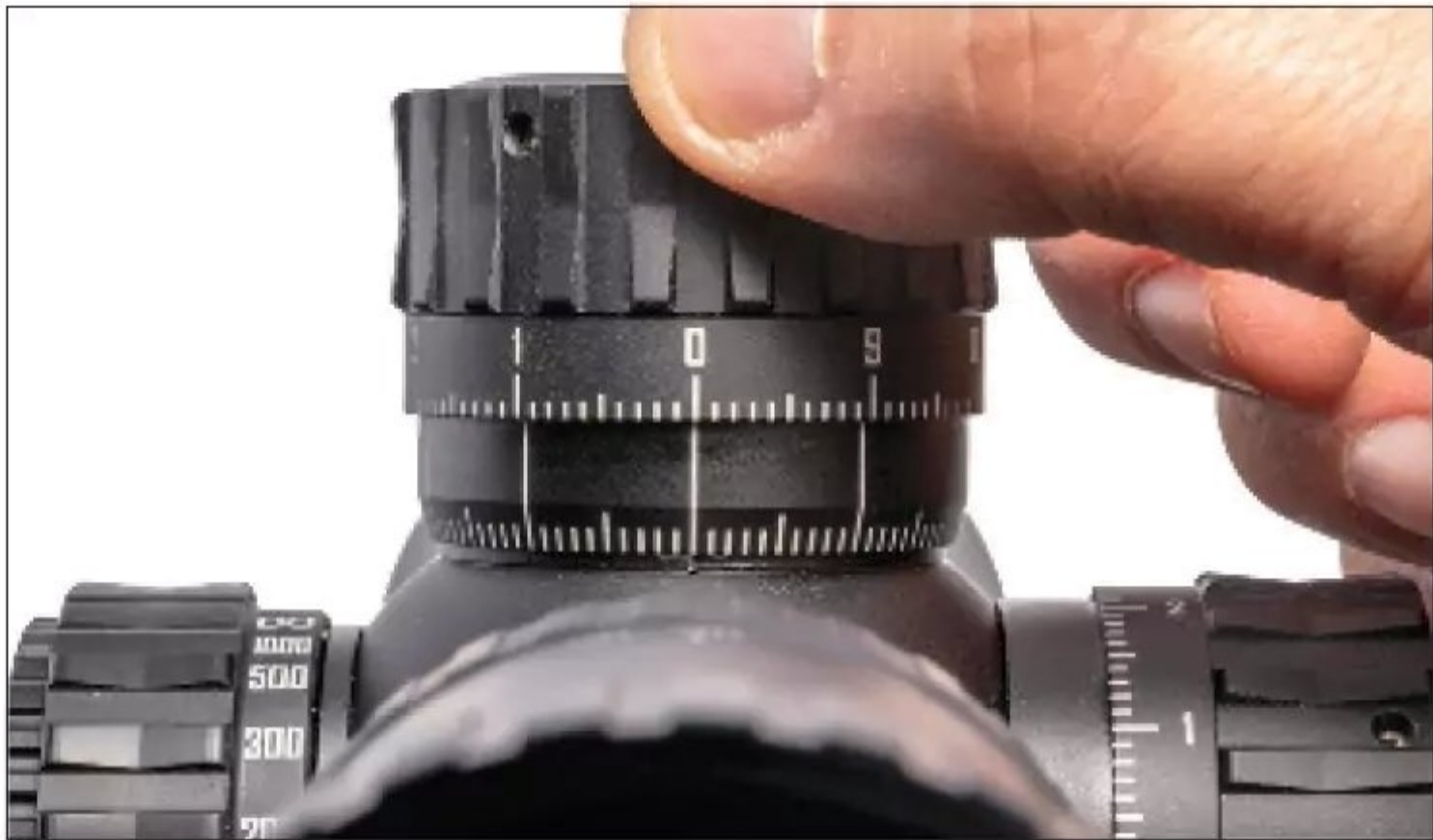
Standard set-screws secure the knurled turret cap. Once zeroed, it can be removed and replaced so that the "0" mark represents the actual zero.
