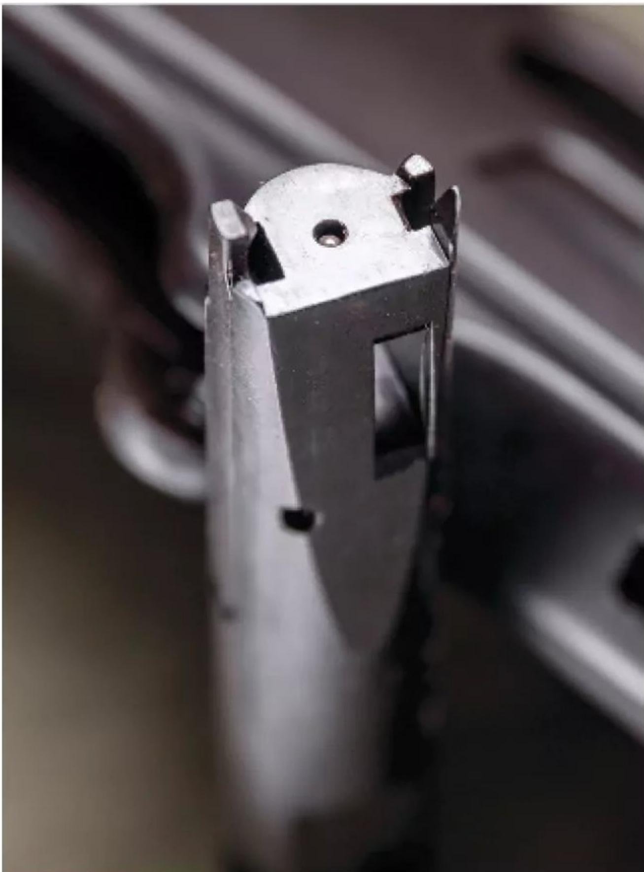
The Model 1854 features a tomb-stone-style bolt face with extended extractor and slot on the opposite side to allow for the ejector. The bottom is ramped for reliable feeding from the lifter.
