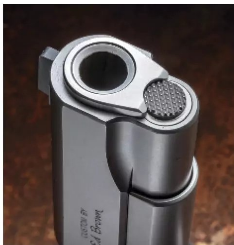
The .45 ACP slide and crowned barrel utilizes a hand-fit bushing, which is secured by the checkered plunger.
