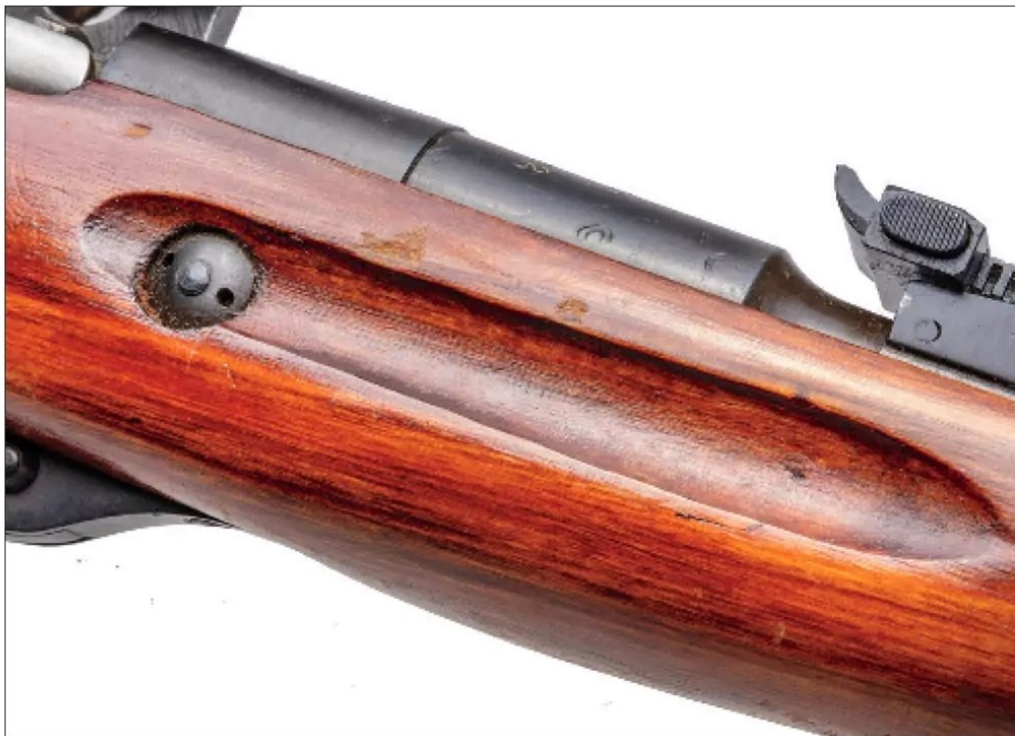
The 91/30 rifle stock was made at the Tula Arsenal. The crossbolt is secured by a nut at the rear of the inletted finger groove.
