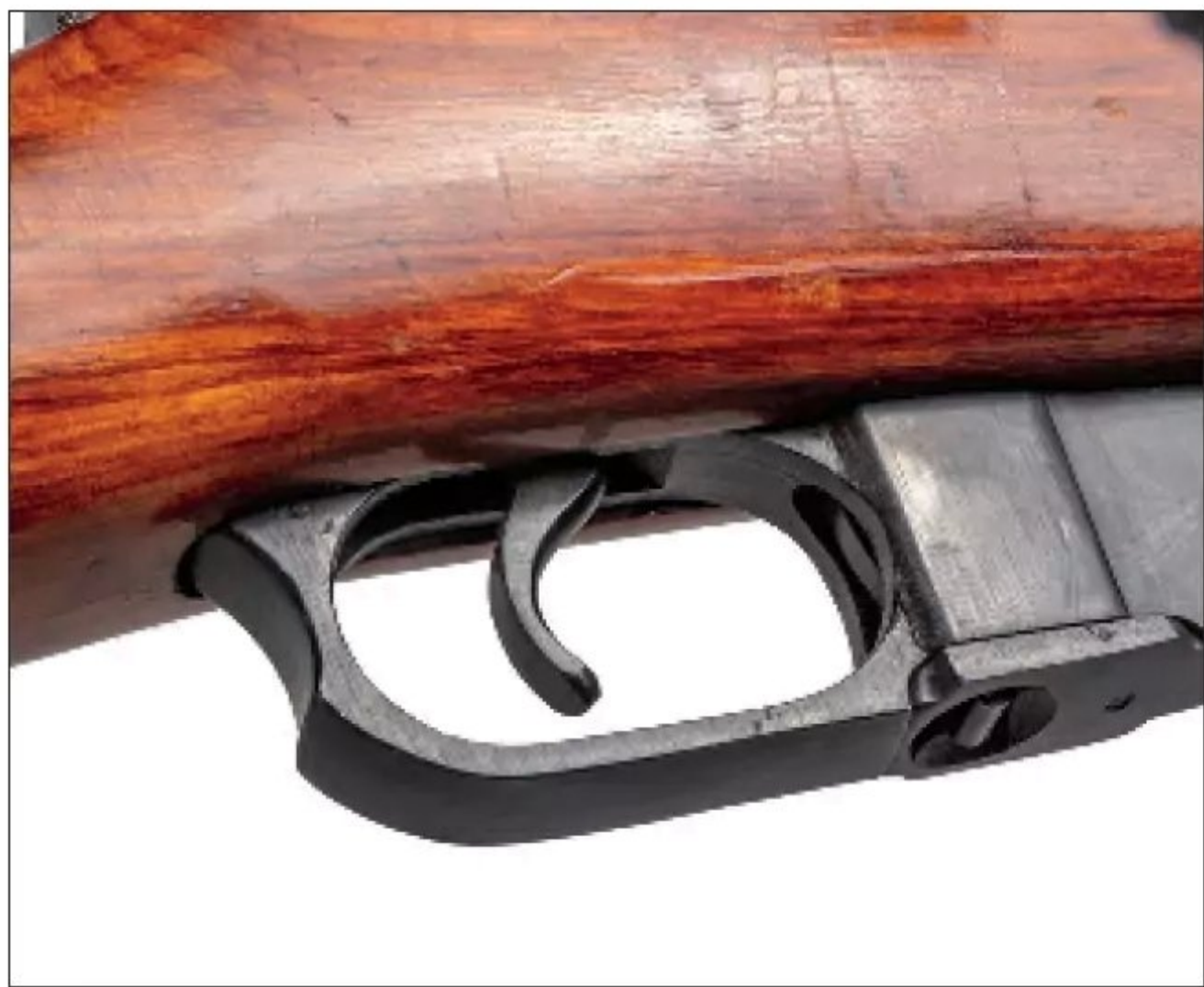
The 91/30 triggerguard features a relief for the middle finger at the rear. The latch to release the floorplate is at the front.
