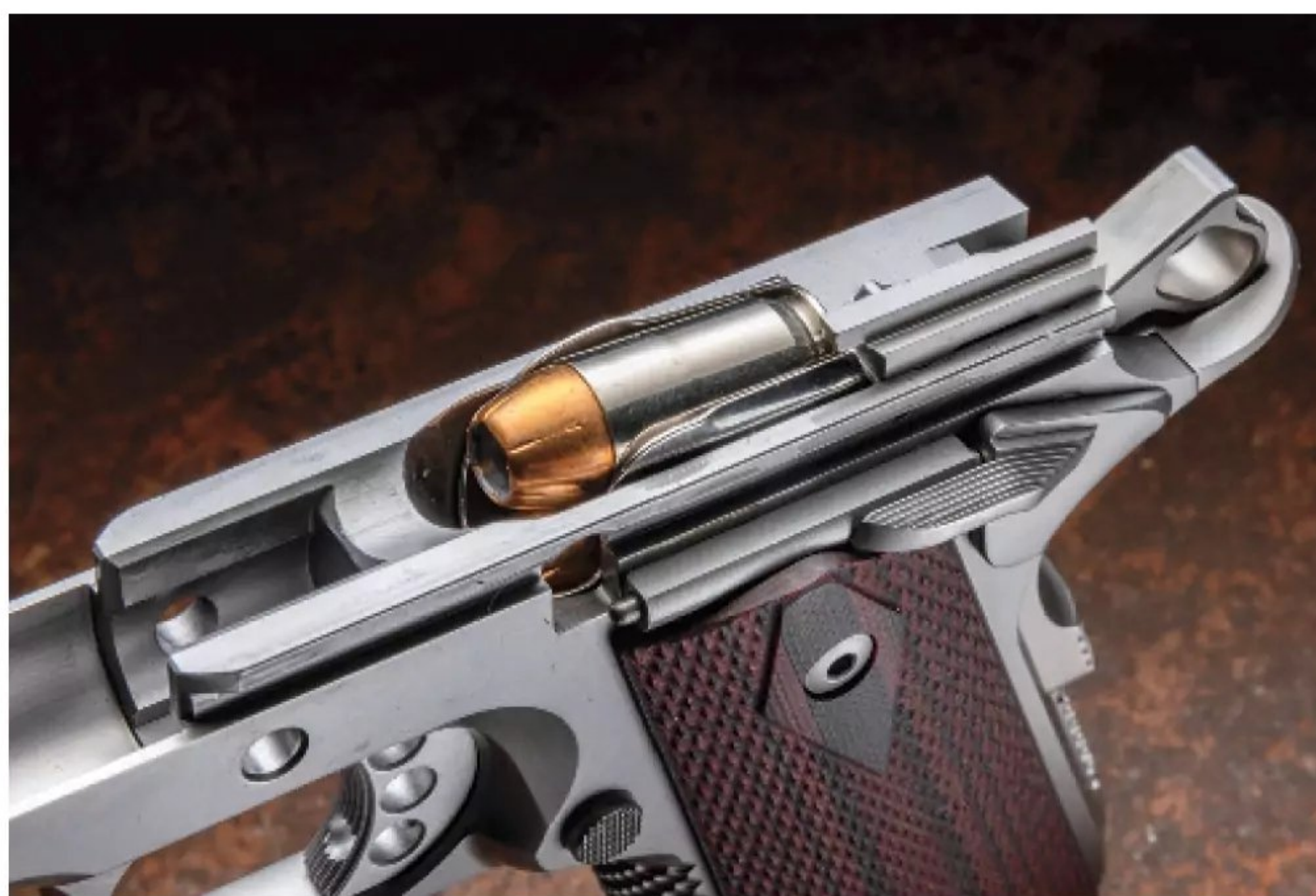
Chambering either .45 ACP (shown) or 9mm, the dual-caliber kit requires the user to change ejectors.
