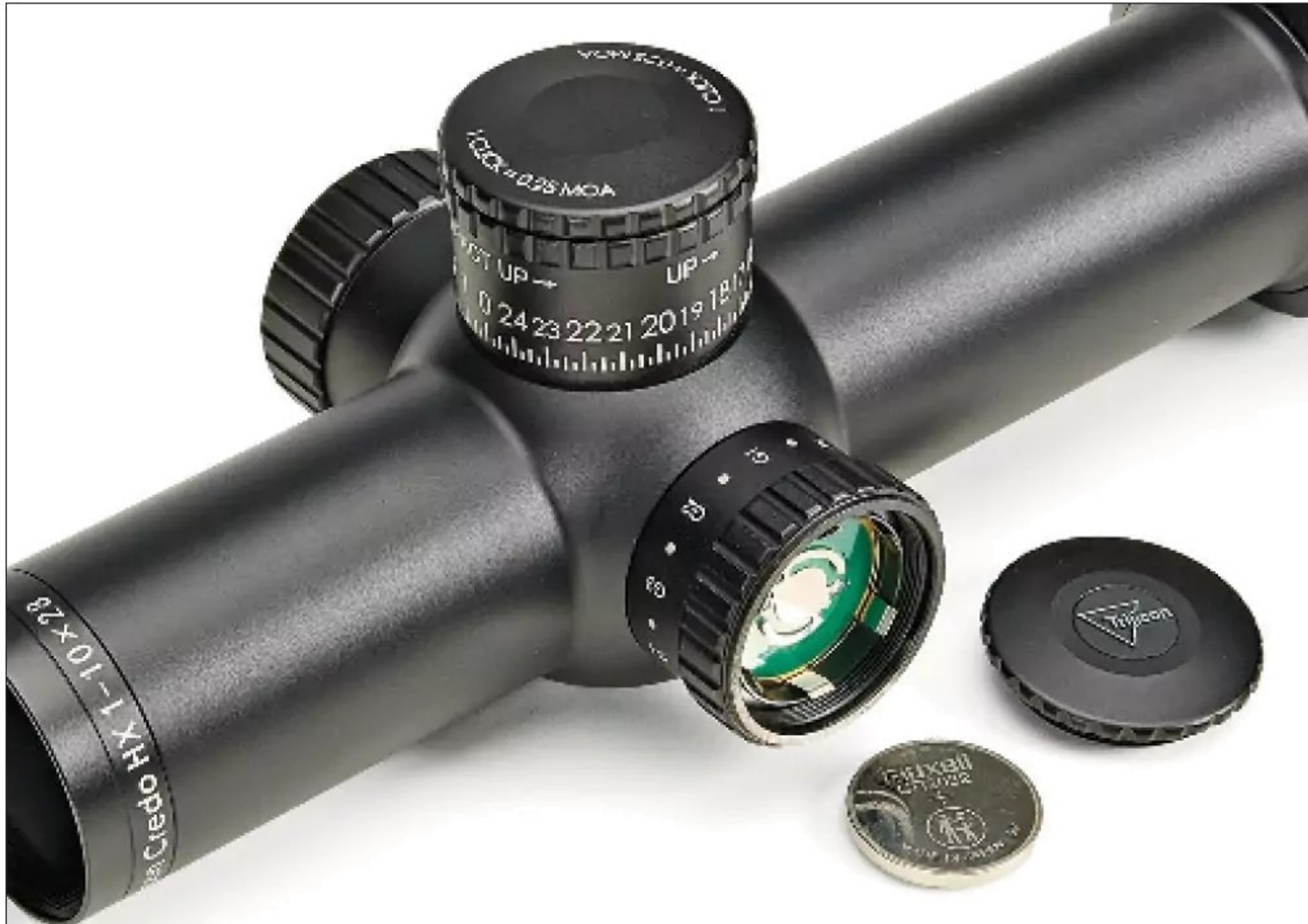
The left-side turret houses the on-off dial, featuring five red intensity levels, five green intensity settings and an off position between each. Illumination is powered by a capped CR2032 battery.
