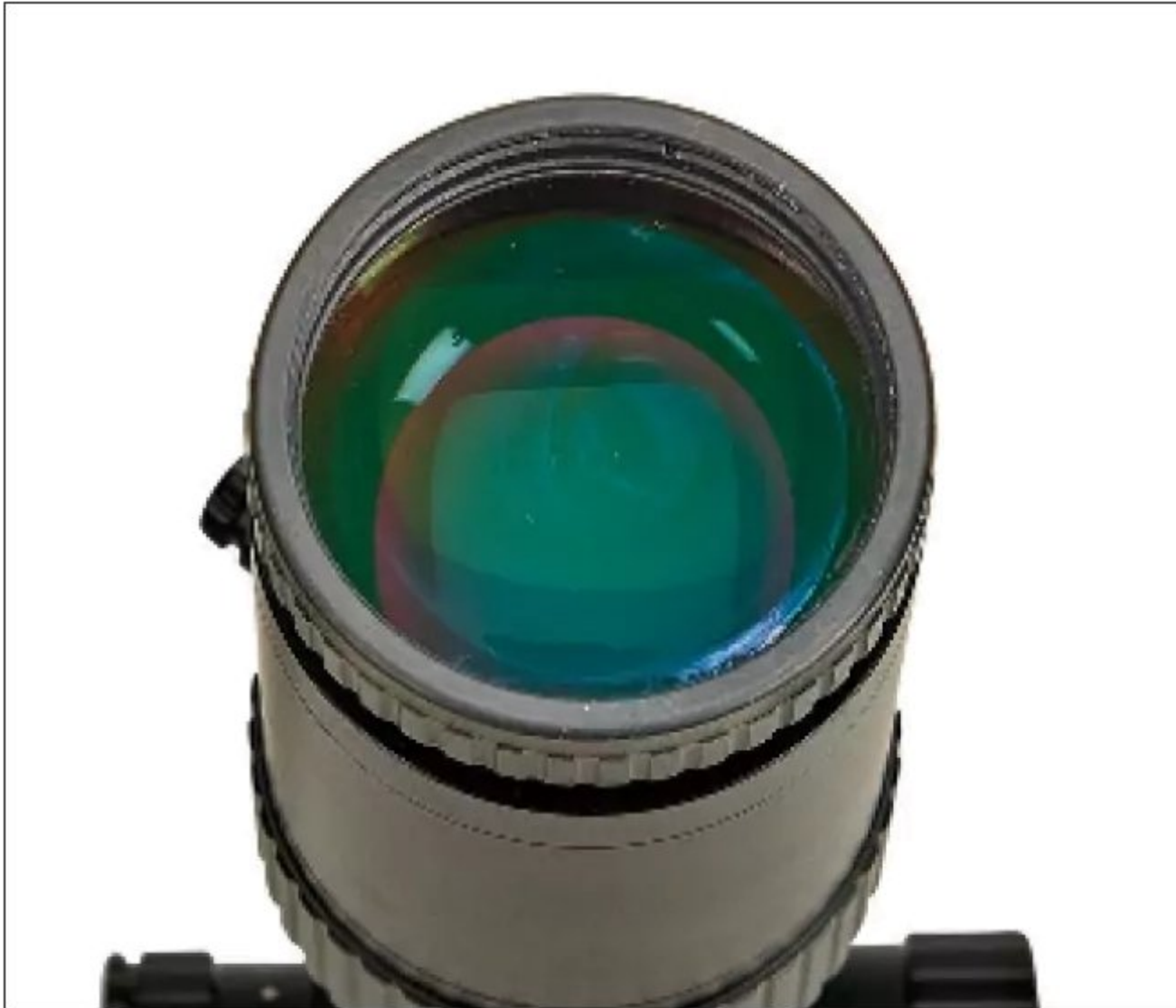
The ocular lens is shrouded by a reticle focus adjustment ring with a rubberized cap. The Credo has a .32- to .11-inch exit pupil with full field of view visible with 3.2 to 3.9 inches of comfortable eye relief.
