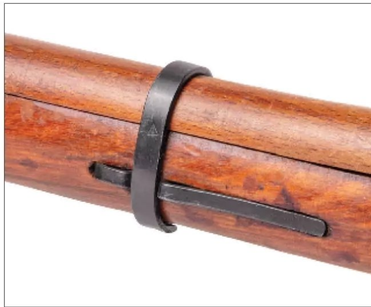
The horizontal bar is a spring pressed into the lower forend of the stock, which applies pressure to the barrel band.
