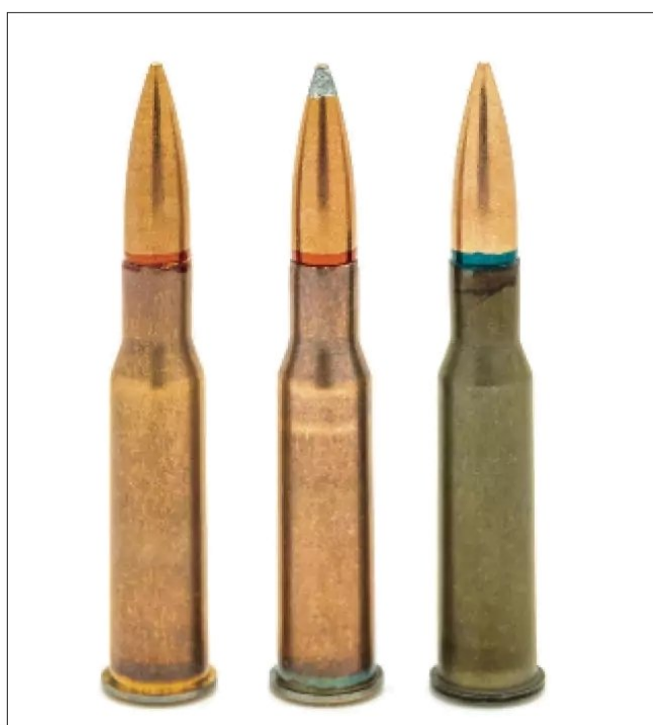
Test ammunition for the Mosin-Nagant 91/30 PU included (above, left to right): 1945 148-gr. light ball; 1971 Bulgarian 147-gr. steel core light ball; and 2020 Red Army Standard 148-gr. light ball.
