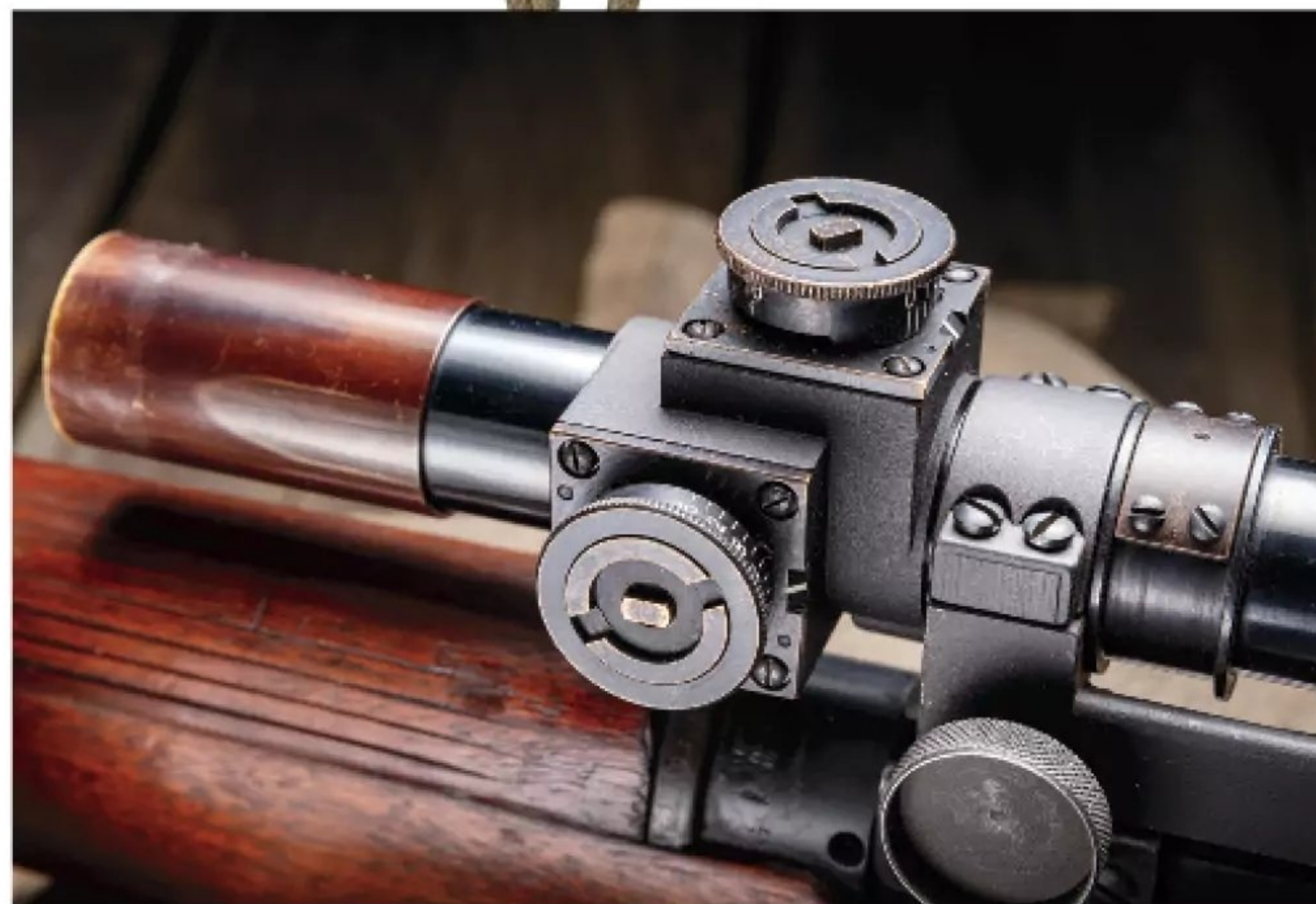
The No. 32 Mk I scope featured 2 MOA windage and elevation adjustment turrets for the .303 Mk VII ball round. Also, the objective and ocular housing featured sliding protective shades.
