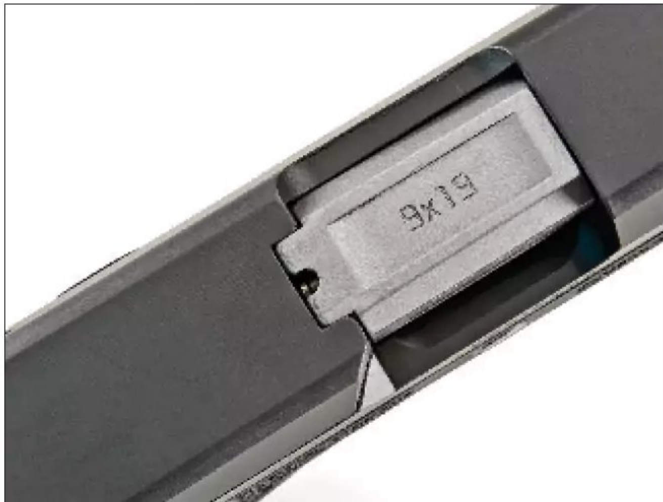
The notch atop the barrel hood at the rear serves as a loaded chamber indicator. Also visible is the cartridge dimensions, 9x19mm. The slide top is flat and smooth.
