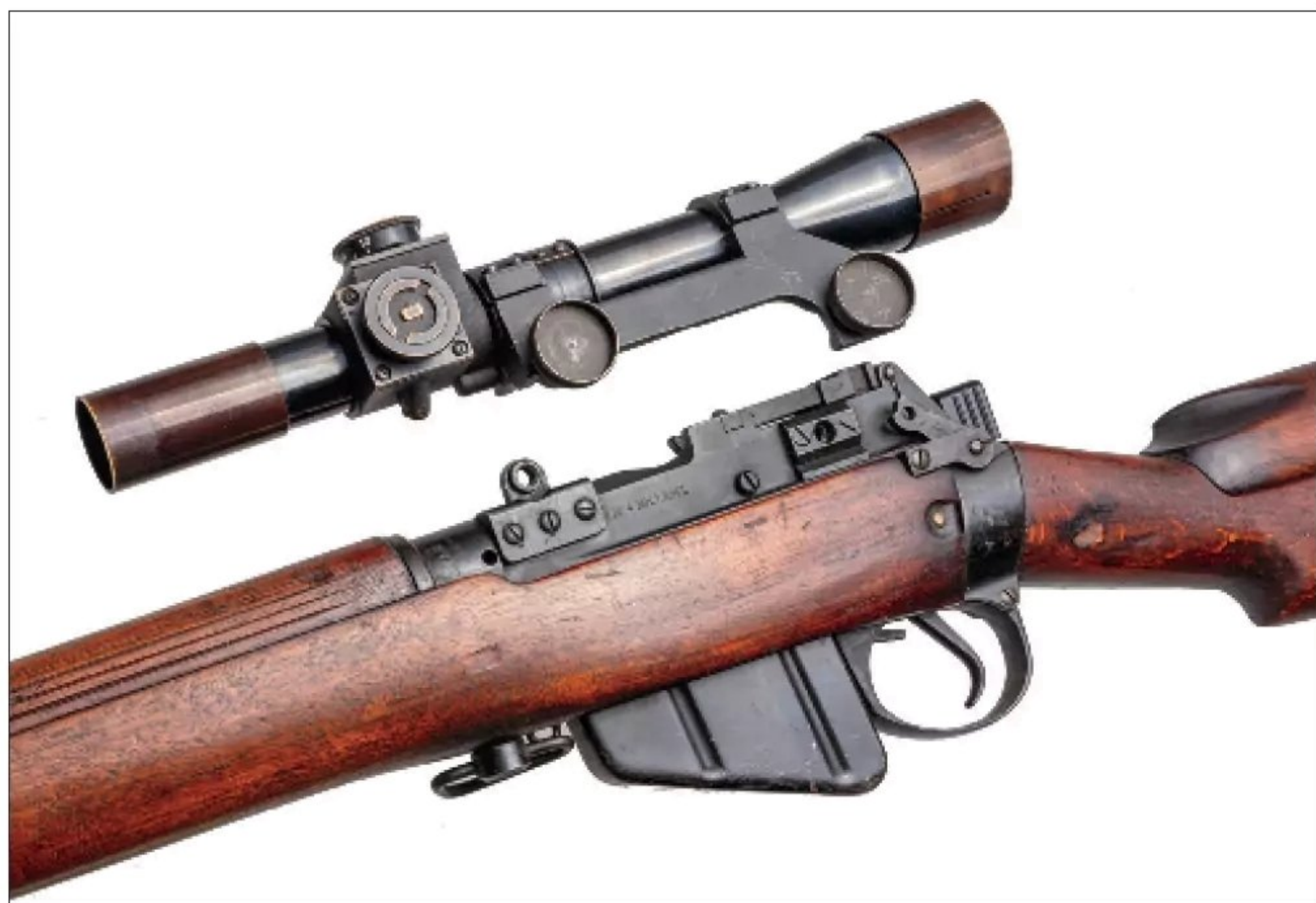
The No. 32 scope and mount could be quickly detached from the No. 4 Mk 1 receiver. It was necessary to remove the scope in order to remove the bolt assembly for maintenance.
