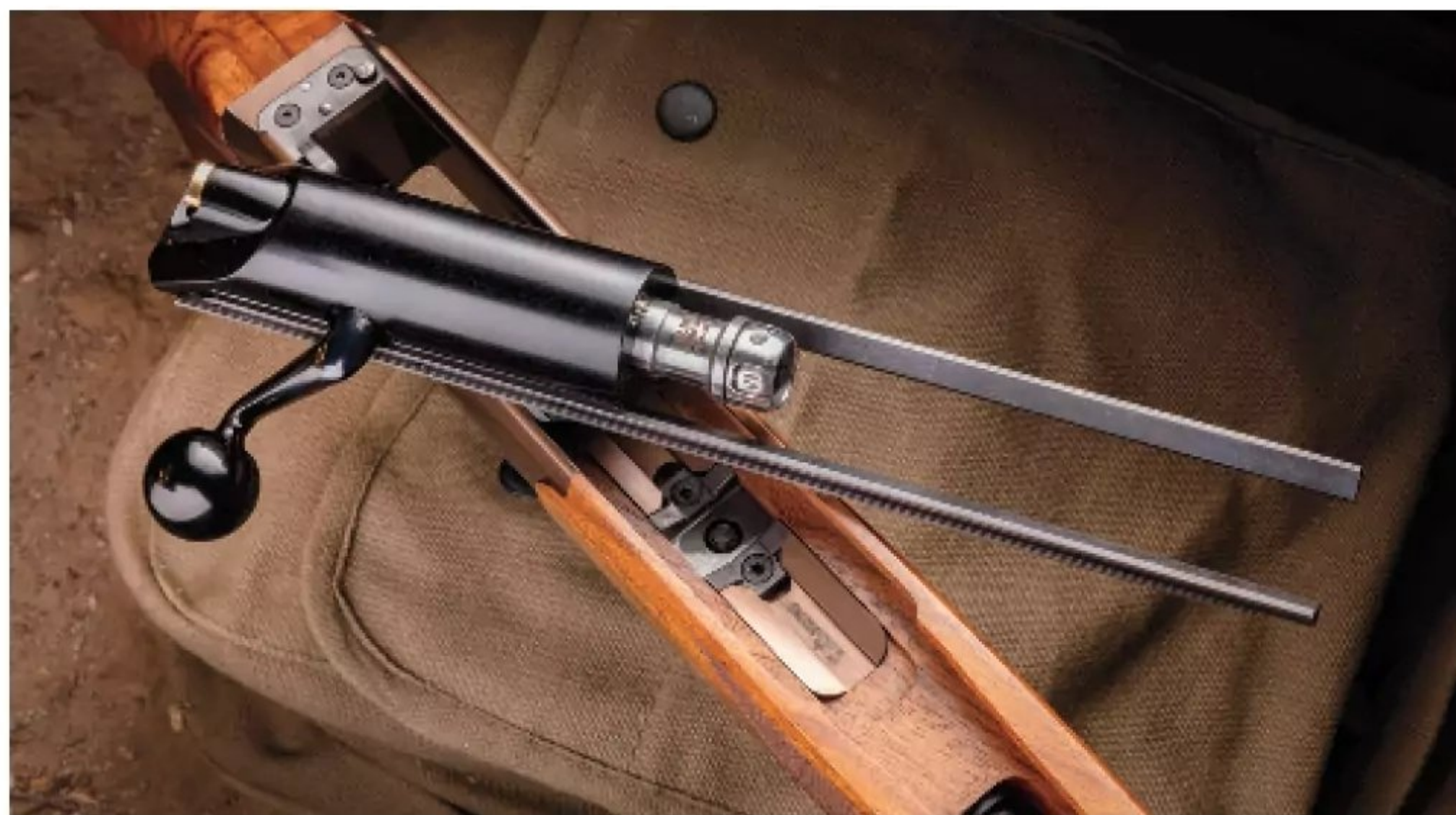
Multiple, concentric lugs surrounding the bolt rate it for high pressure. The ROLS was tested to an impressive 123,000 psi, almost twice the pressure of typical modern cartridges.
