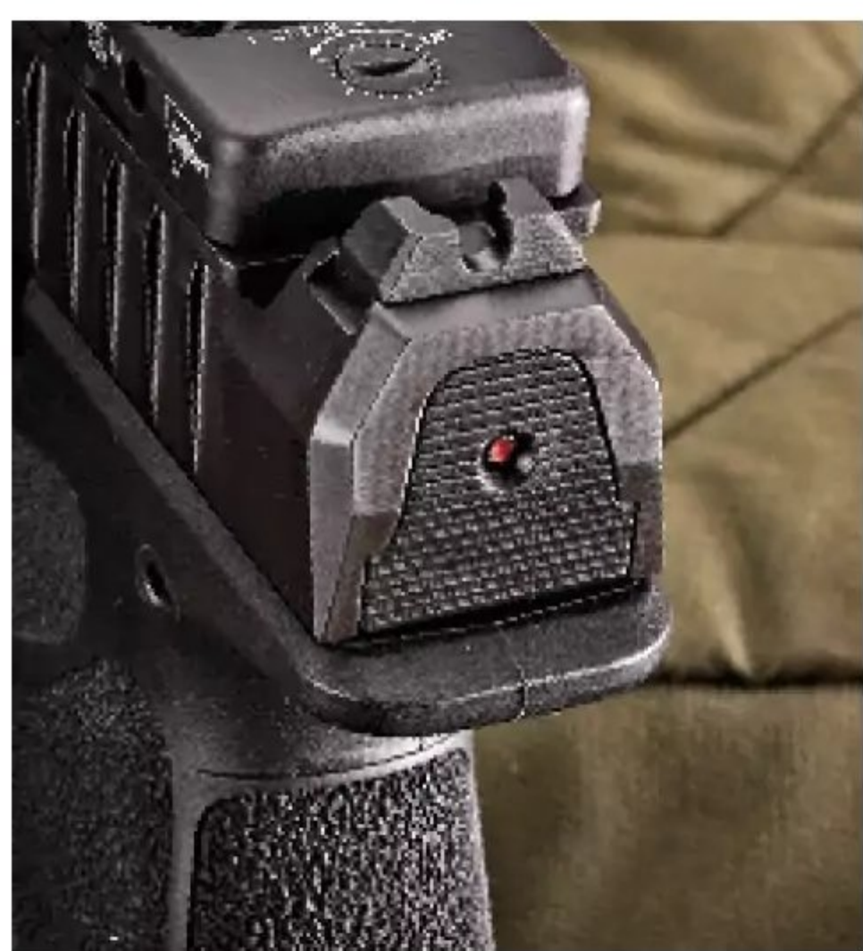
A red dot appears when the striker is cocked. After the pistol is fired, the indicator disappears, providing the user with a status of the pistol's condition.
