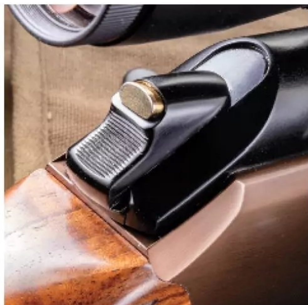
The ROLS Classic safety system does not automatically decock between shots, so it's important to practice using the decocker before heading to the range or field.
