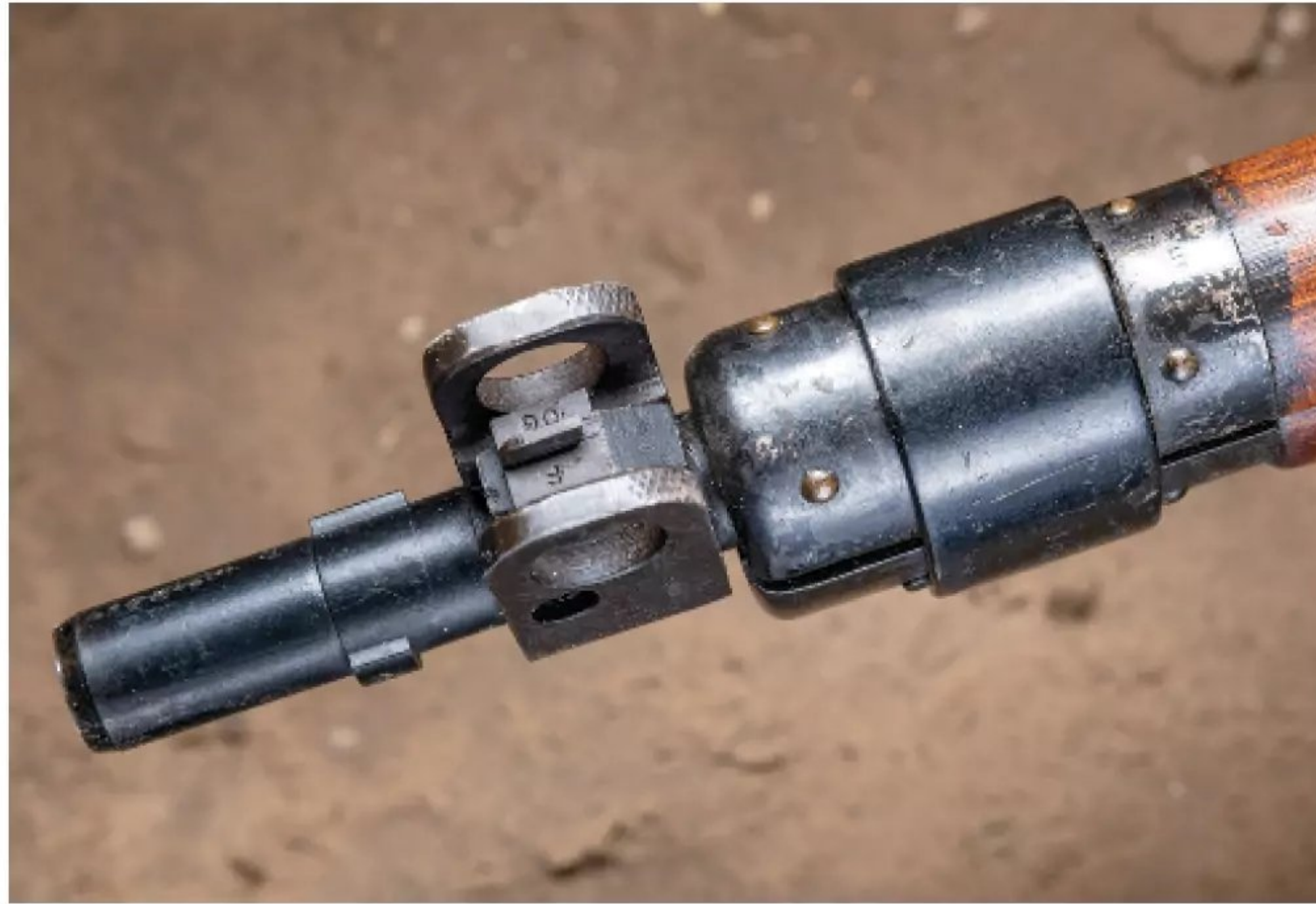
The front sight assembly is protected by the common Second Variation bracket. The sight blade is marked with its height, “.06” and manufacturer “F” for Fazakerley.
