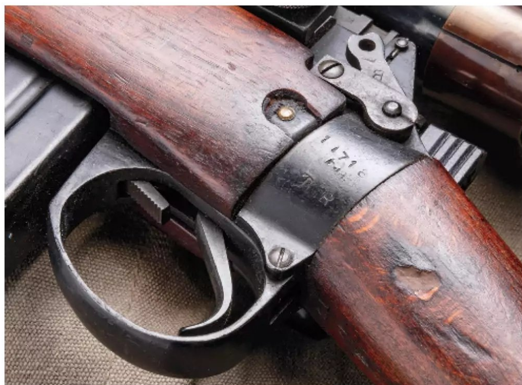
The trigger of the No. 4 Mk 1 (T) was smoothed. Inside the triggerguard is the magazine release lever. The wristband displays serial and "TR" markings, indicating its selection as a sniper rifle.
