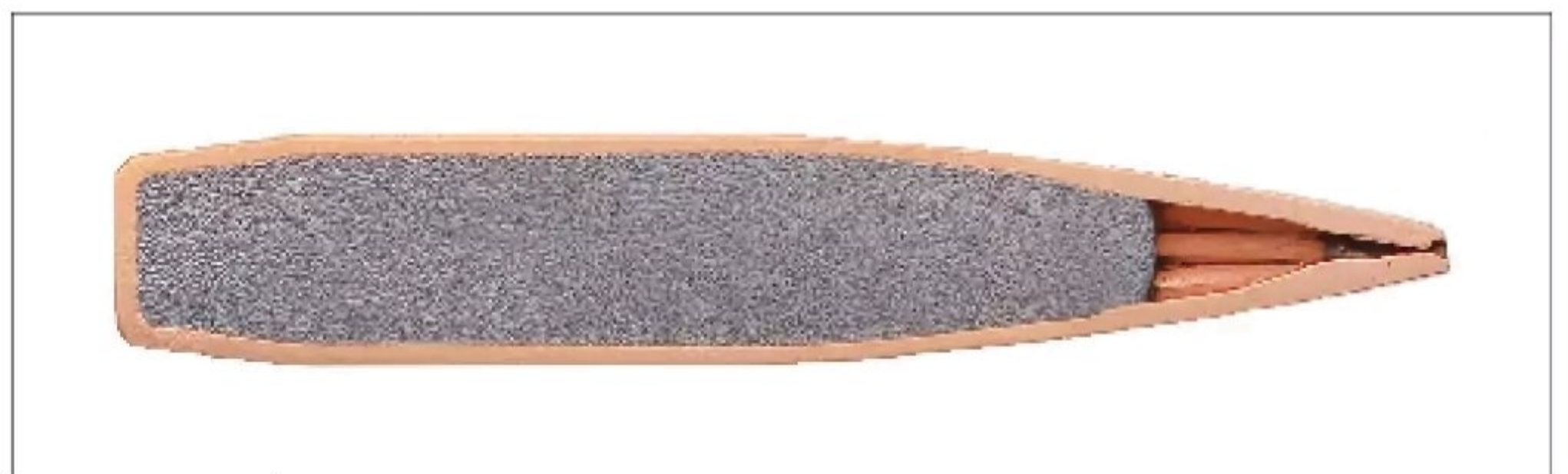
The 195-grain Berger Elite Hunter features a thin copper jacket, and a cavity behind the hollowpoint tip and head of the lead core. MSRP: $81
