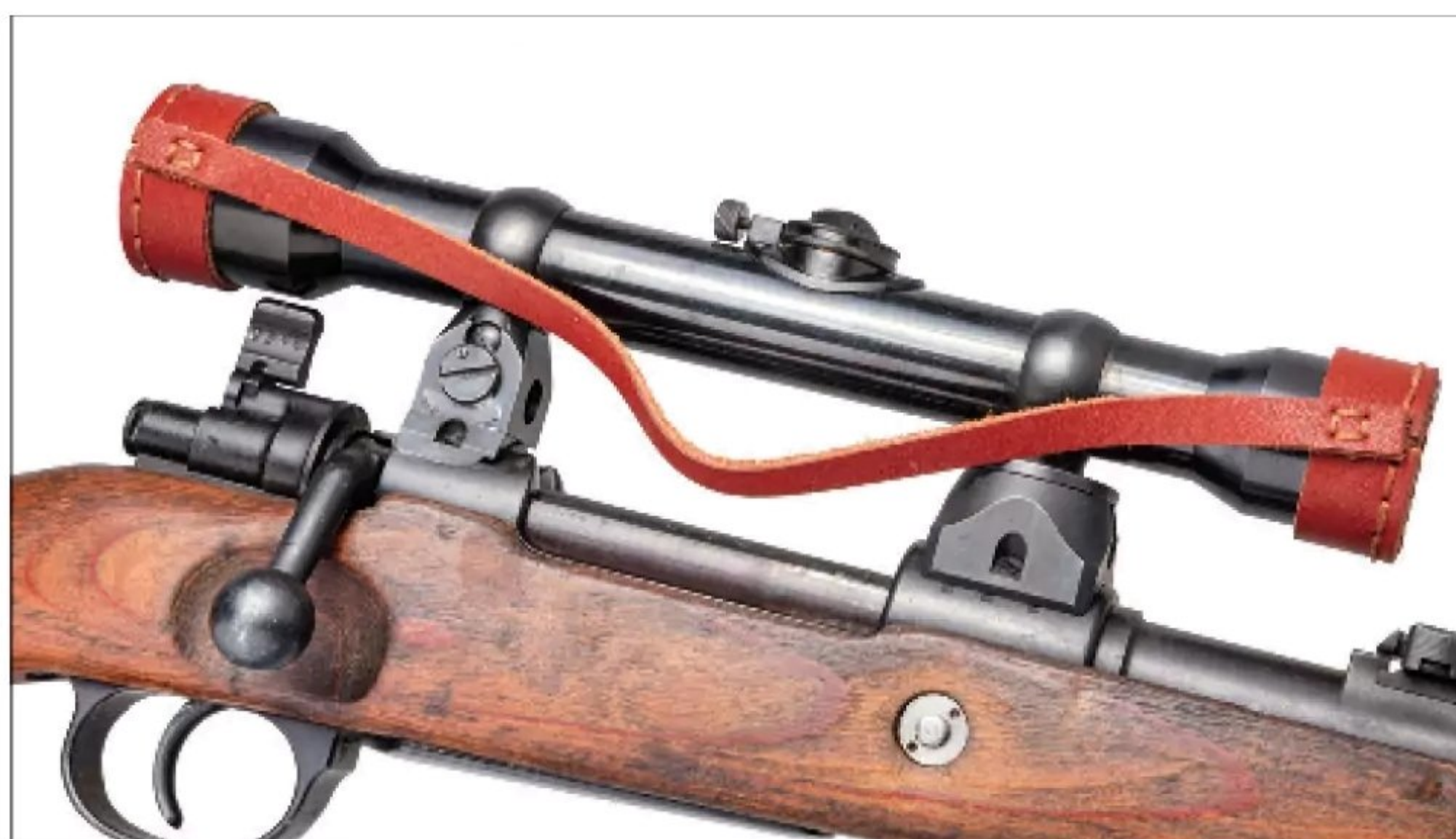
Snipers were issued a metal can to store the Zf.39 for transportation. A leather scope cover protected the lenses in the field.
