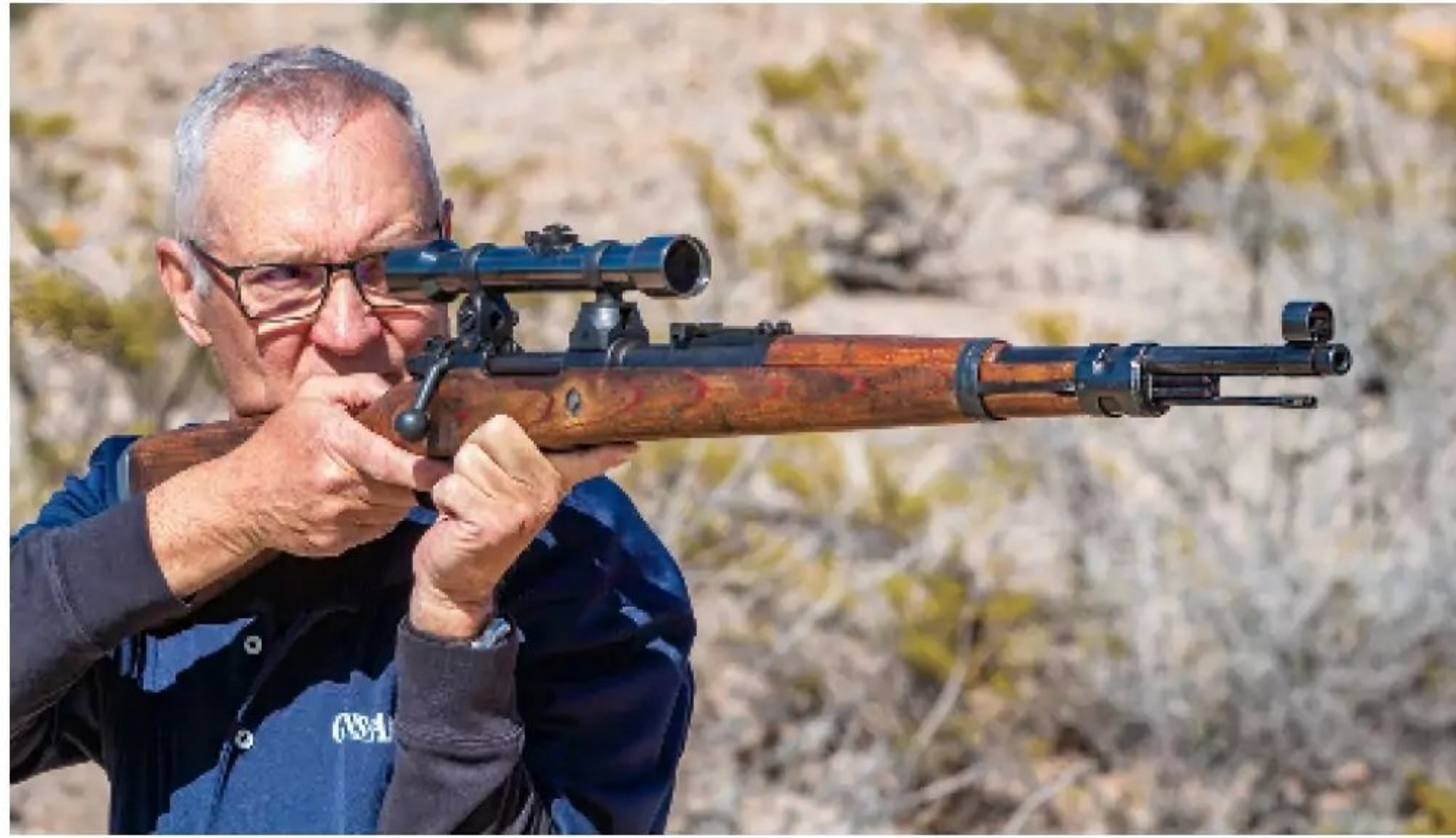
Recoil from the 8x57mm-chambered K98k was significant. Lacking adjustment, the scope required estimated holds for hits.
