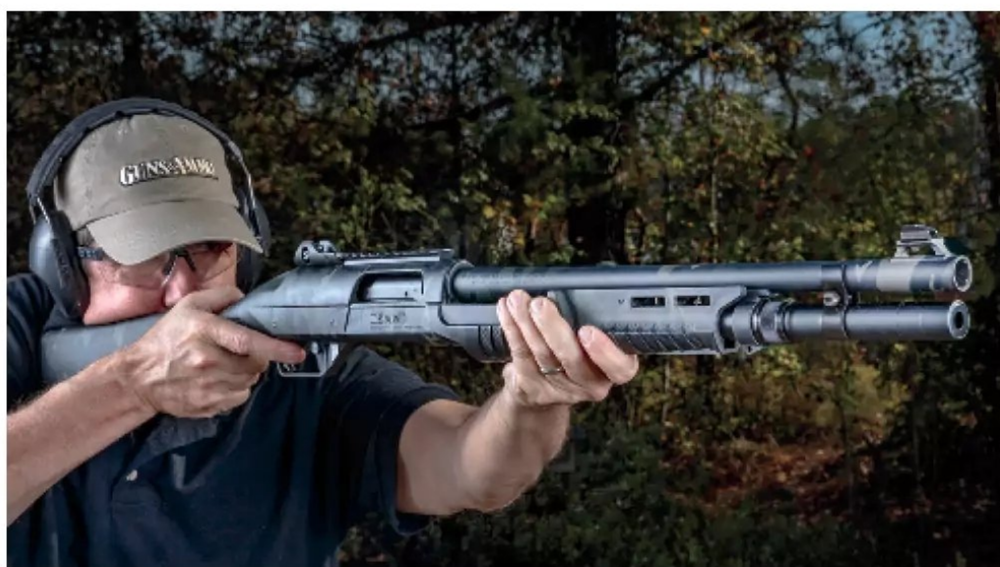
The steel barrel extension and hood were designed to safely contain and guard the polymer receiver from the chamber pressure created as a shell is fired.
