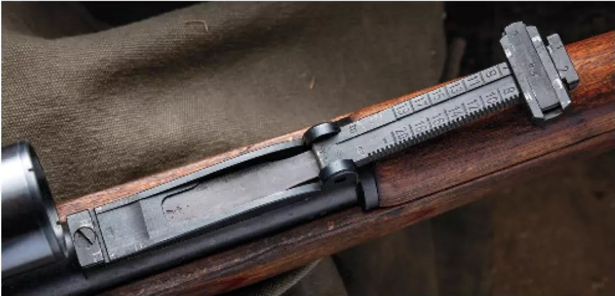
The K98k Zf.39 retained the tangent-curve, 100- to 2,000-meter, adjustable rear leaf sight in case the scope was damaged. The turrets had a tunnel to allow for use of the standard sights.
