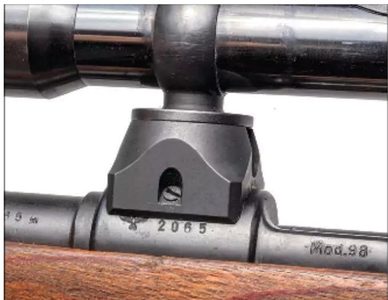
The Zf.39 turret mount was stout, involving both screws and soldering to the receiver. The rear mount (above, center) featured a quick-release lever to either lock the scope in place or remove it. A Carl Zeiss Zielvier 4X was sourced for testing.
