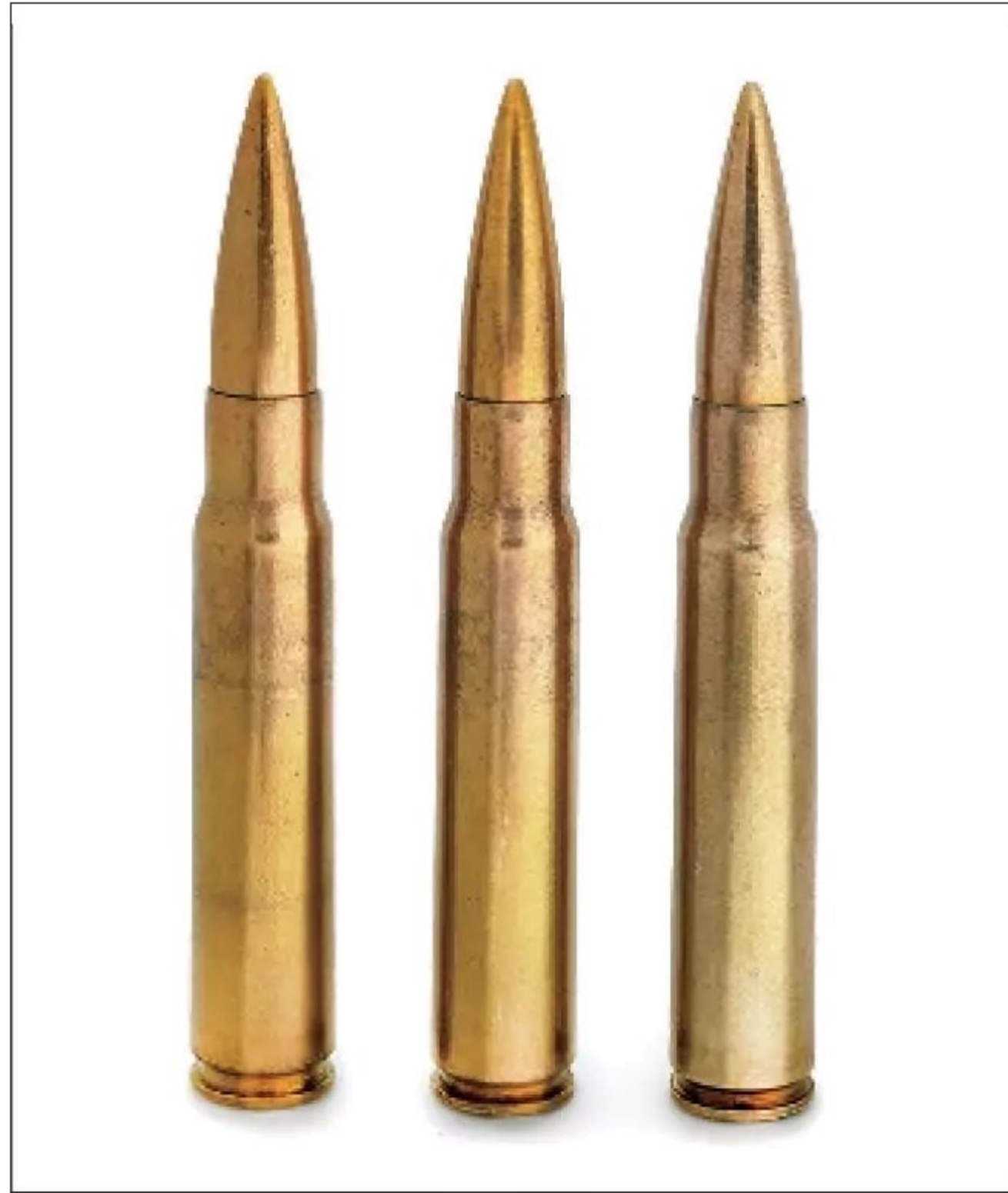
8x57 test ammunition (left-to-right), 1939 SmK; 1938 s.S. Patrone; 1940 s.S. Patrone.
