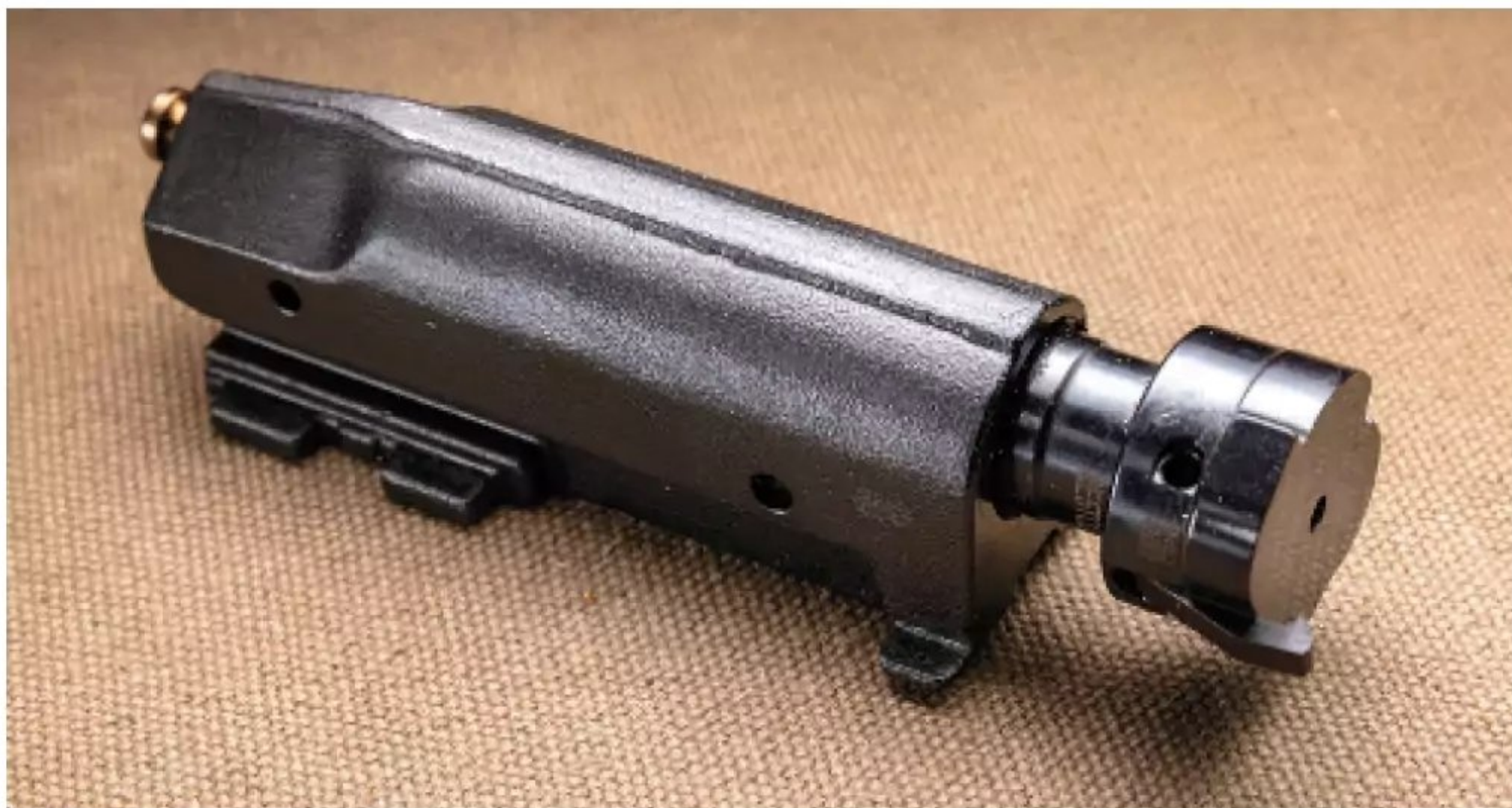
The Nova 3 utilizes a rotating bolt similar to that in the M4 series. Two lugs secure the bolt to the chamber, and the pivoting extractor claw reliably removes shells by the rim.
