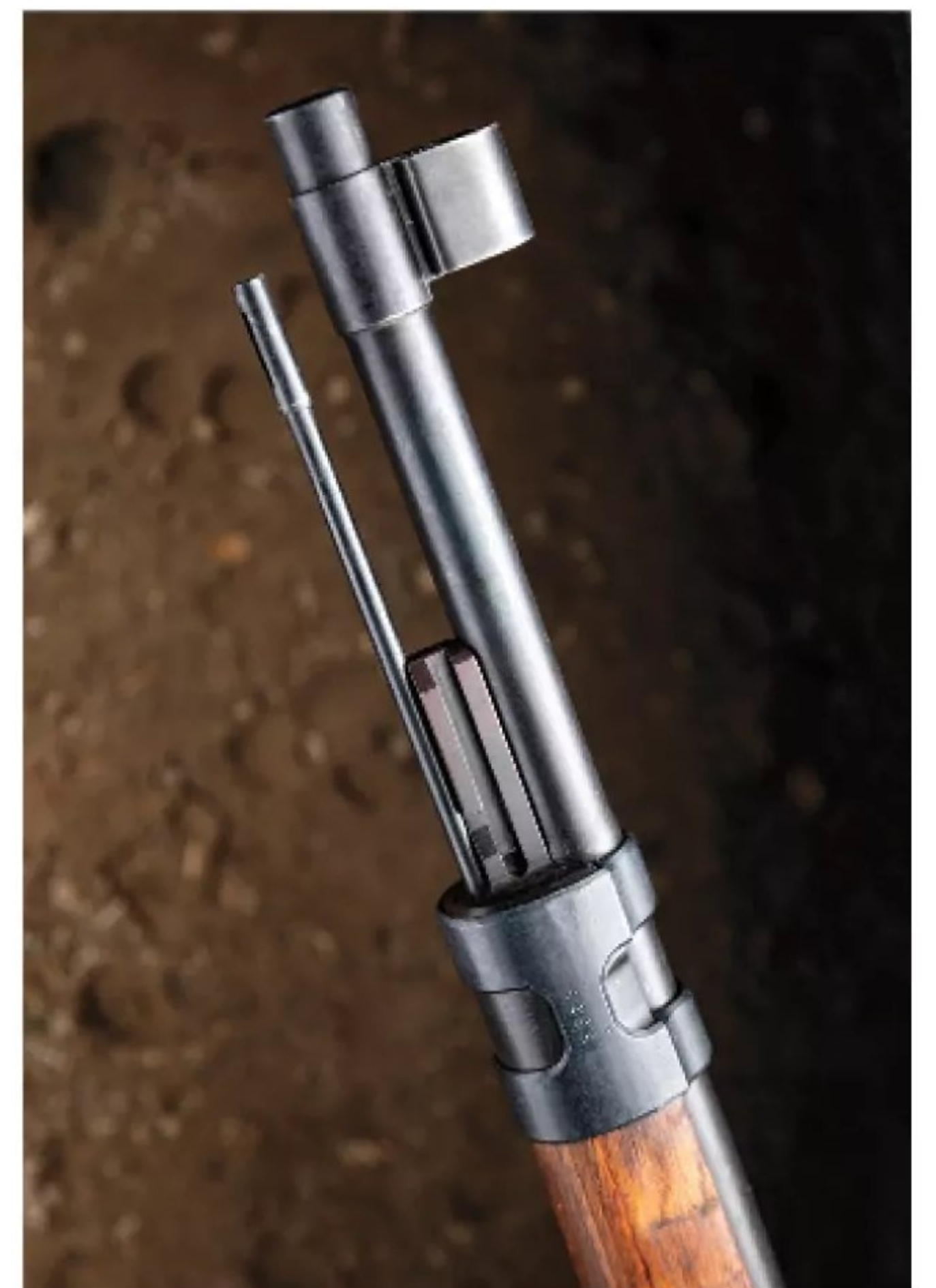
Stamped steel barrel bands and milled H-style barrel bands appeared on K98k Zf.39 sniper rifles.
