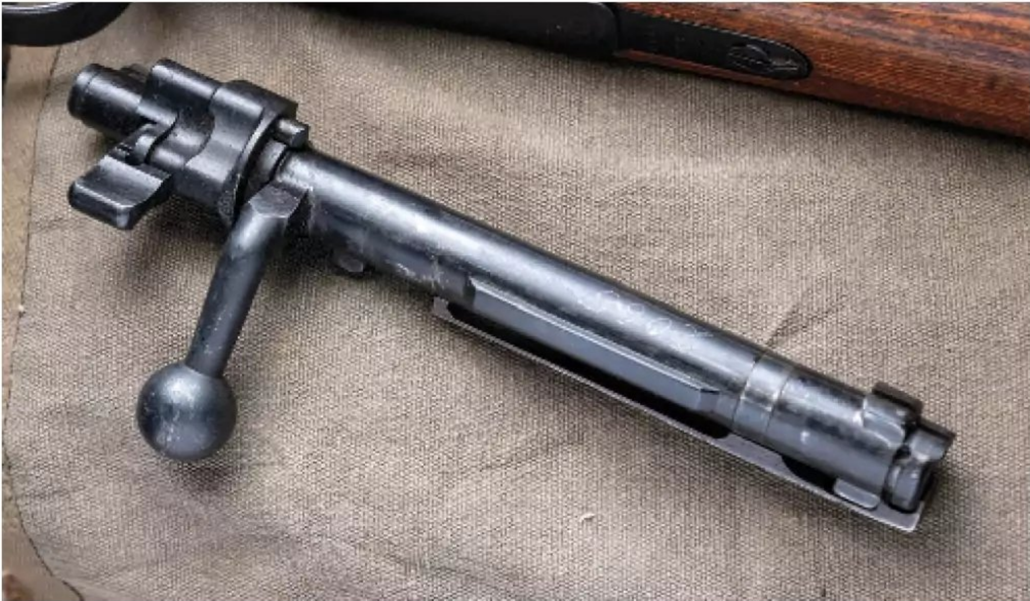
Neither the blued bolt or safety assemblies were altered on the K98k Zf.39. Some late-war rifles had a lower safety to improve its ease of use.
