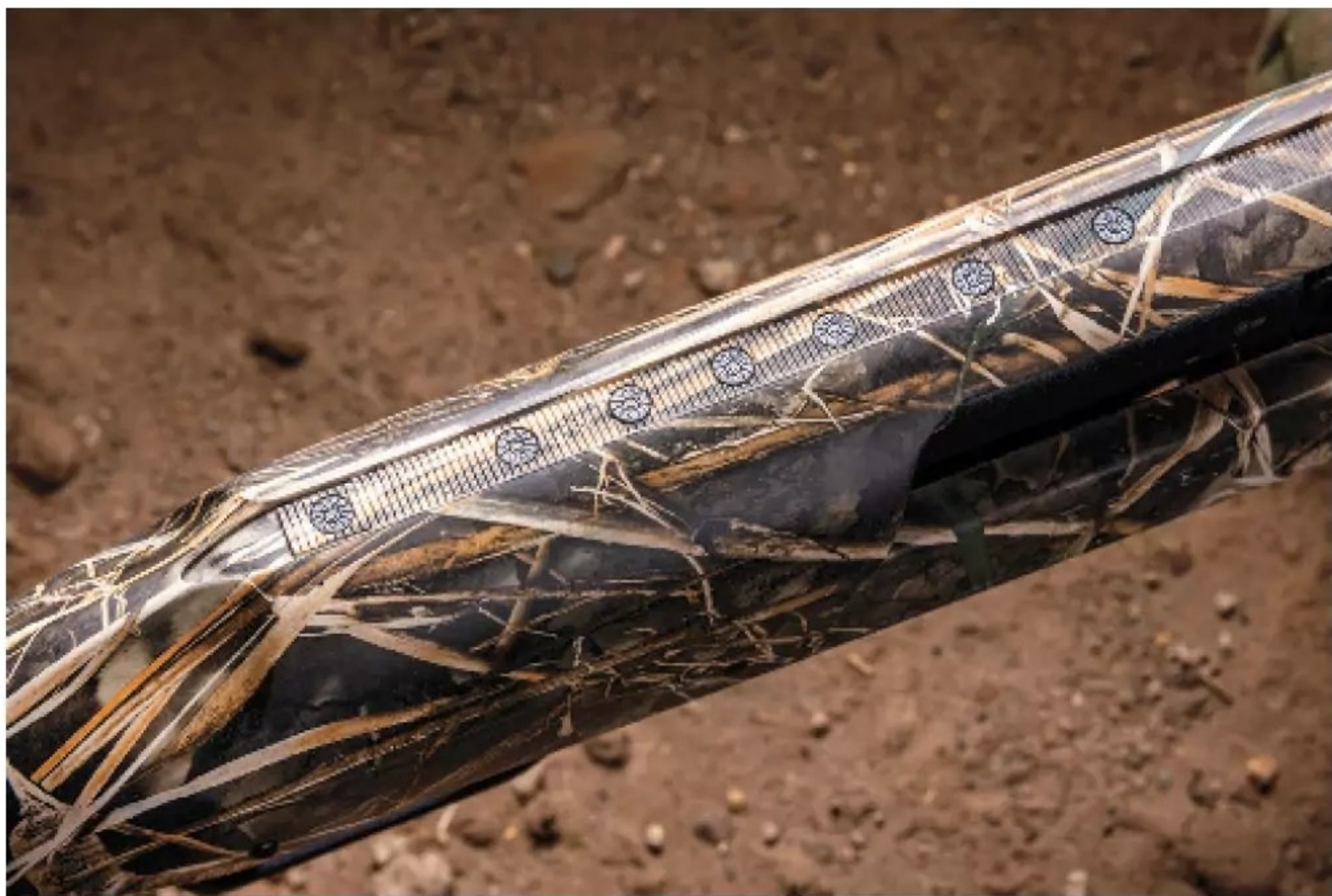
The topstrap of the Nova 3 is reinforced with metal. It is drilled and tapped for mounting an optic rail.
