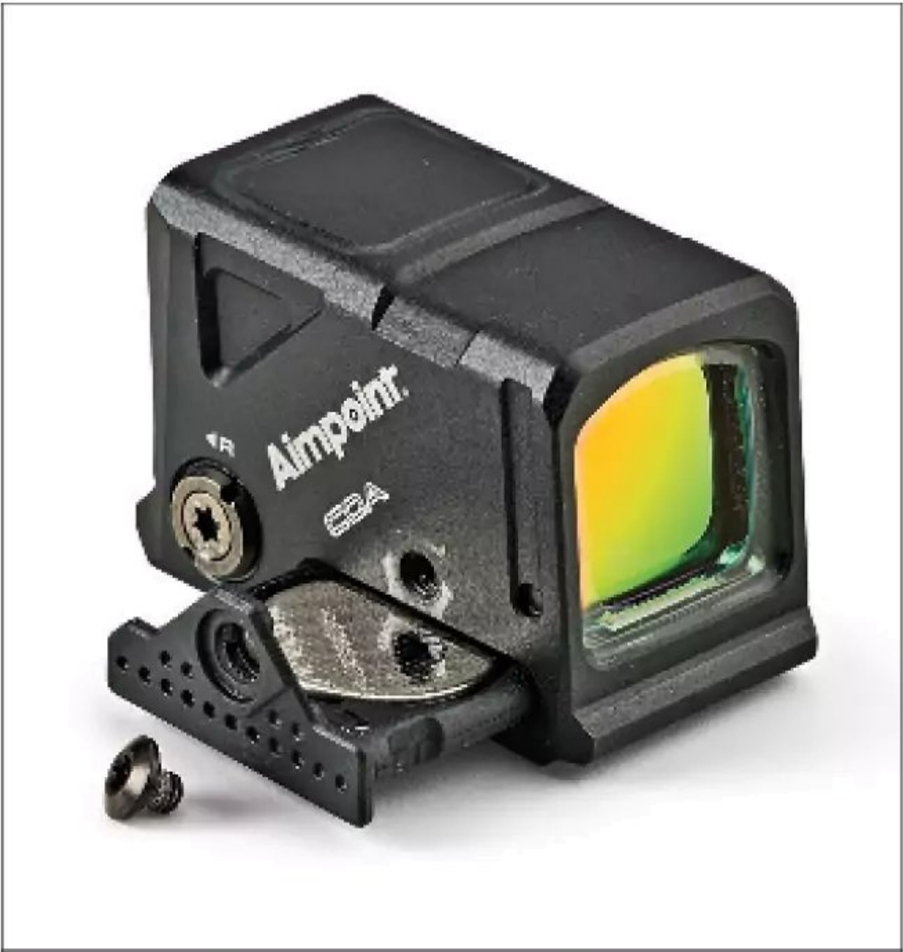
With the T10 screw removed, the user has access to the battery tray. To change the CR2032 battery, the COA does not have to be removed from the slide and re-zeroed.
