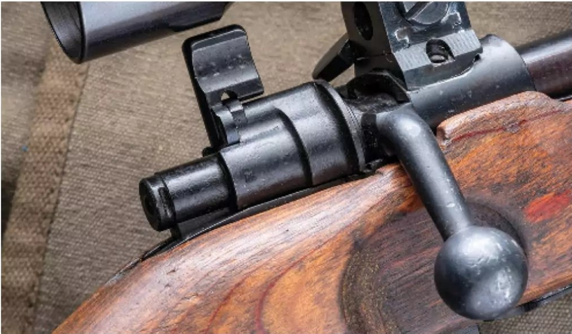
The handle of the Model 98a carbine was turned down, and the stock was relieved for clearance to grasp it. There was minimal risk of interference with the Zf.39 scope when lifting the bolt.
