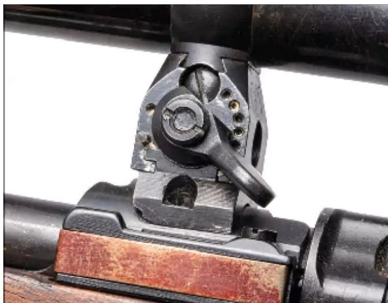
The Zf.39 turret mount was stout, involving both screws and soldering to the receiver. The rear mount (above, center) featured a quick-release lever to either lock the scope in place or remove it. A Carl Zeiss Zielvier 4X was sourced for testing.
