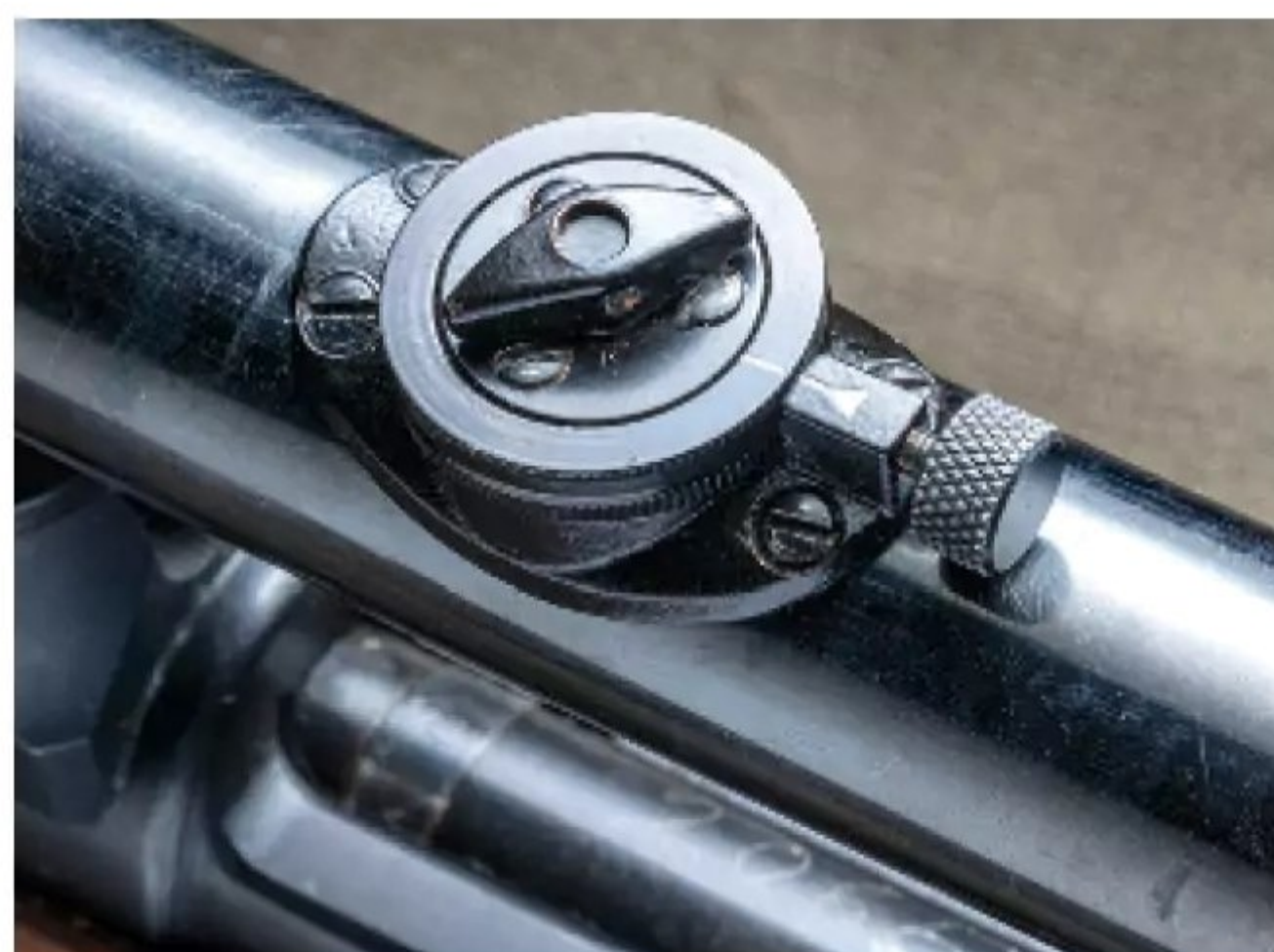
The Zf.39 featured a knurled ring for adjusting elevation with a bar in the middle to adjust focus.
