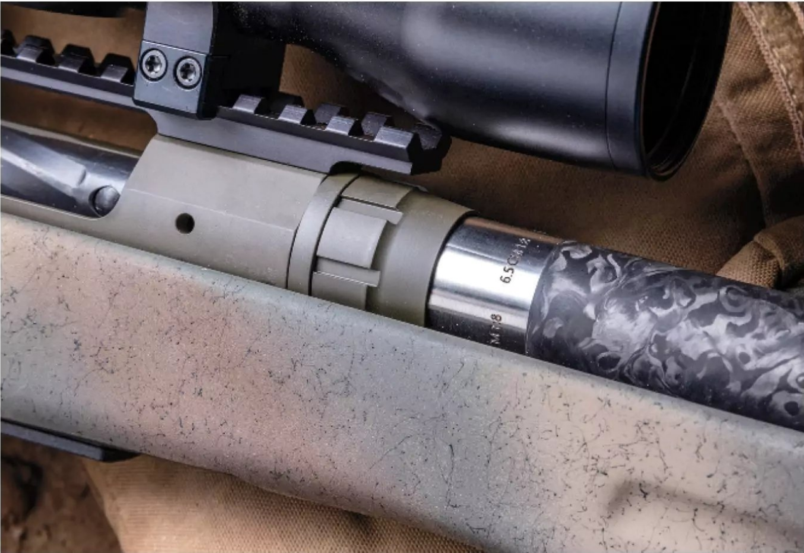
The stainless-steel barrel is marked with its chambering near the action. The barrel is secured to the receiver with Savage's notched barrel nut and lug attachment system.
