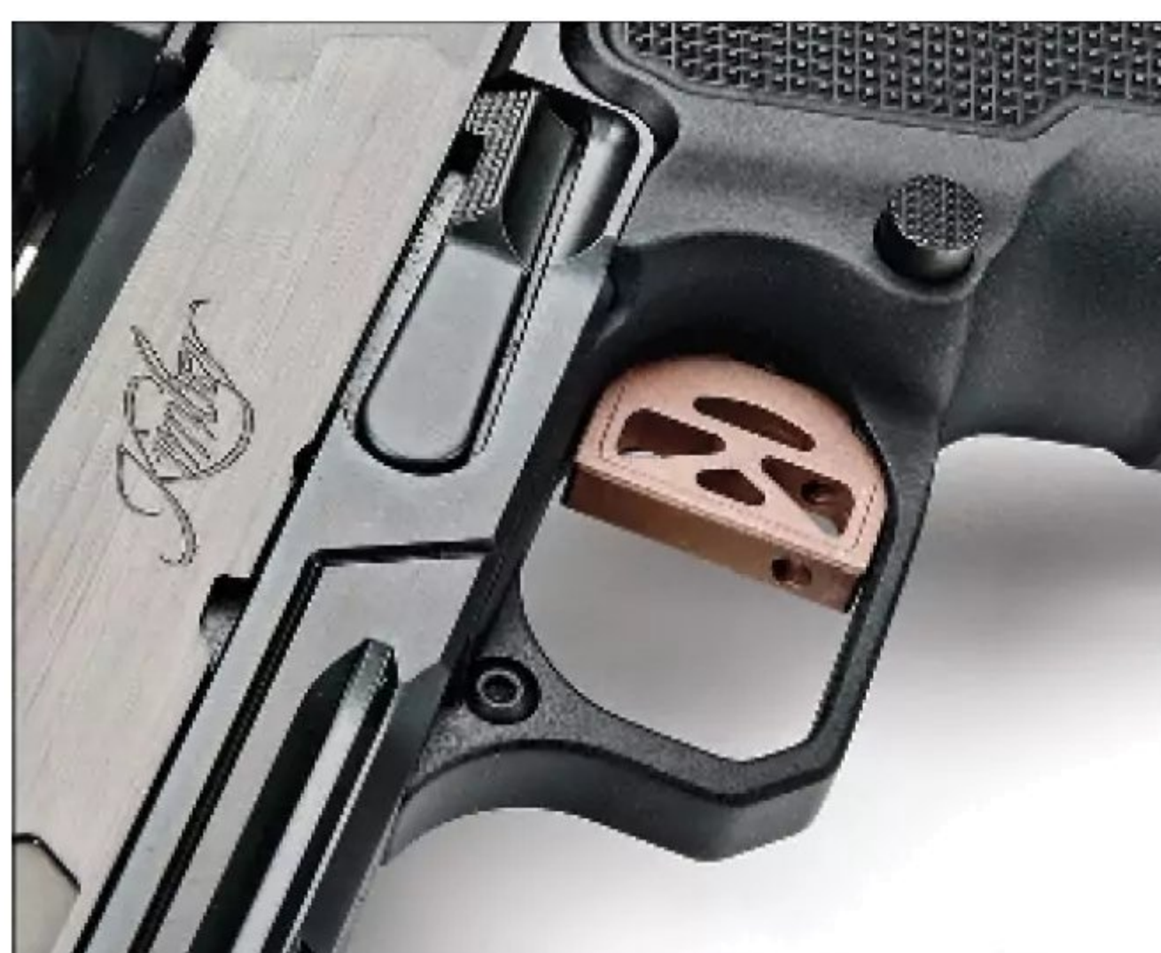
The trigger is a full-length, anodized aluminum unit with an adjustable overtravel screw. G&A's 2K11 tested at 3½ pounds.
