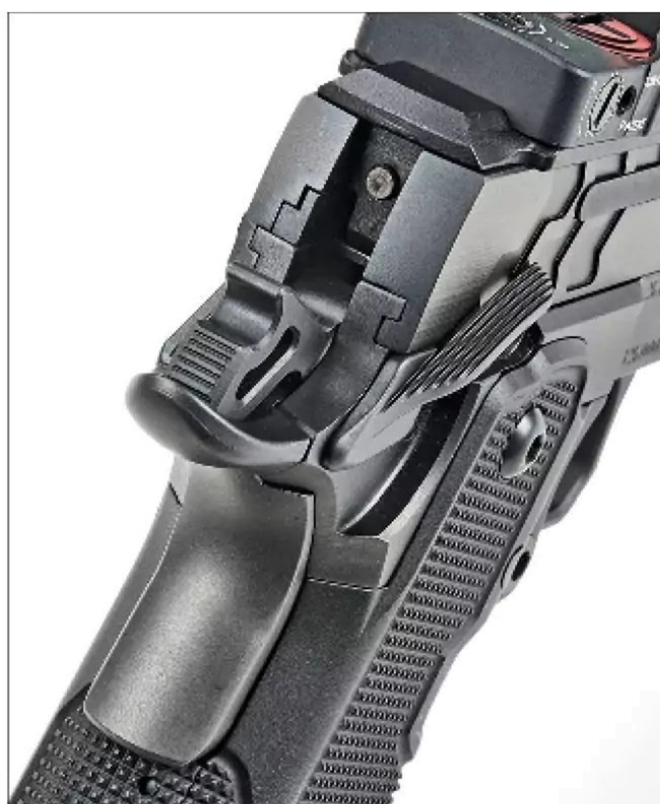
The 2K11 incorporates a serrated, combat-style hammer, smooth beavertail grip safety, and bilateral thumb safety lever.
