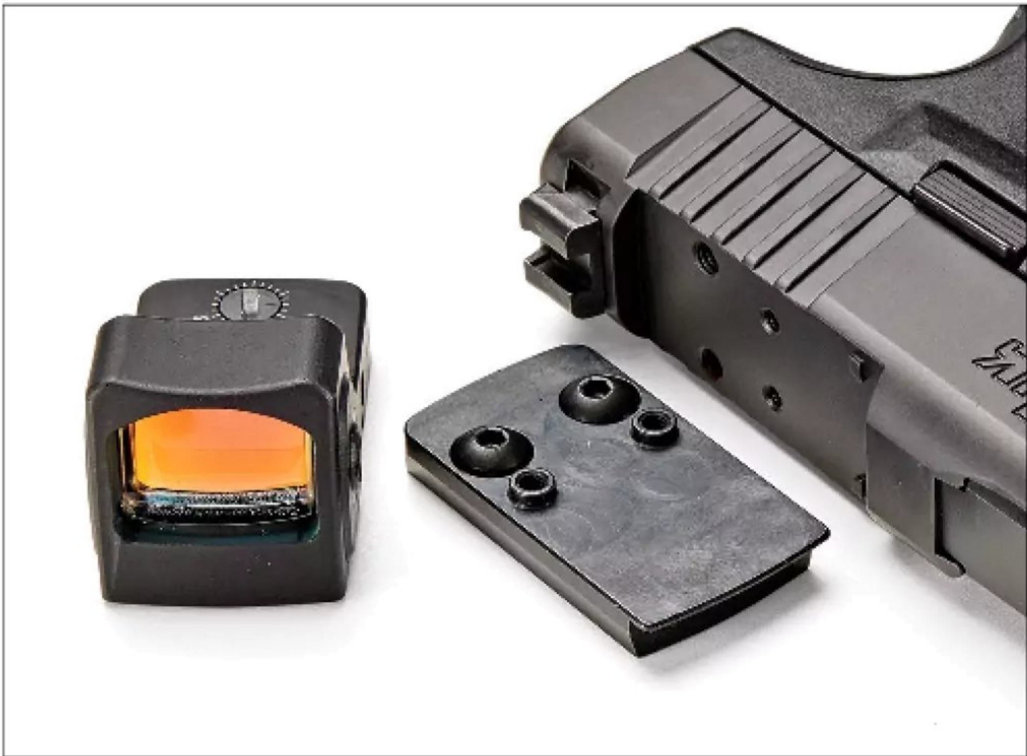
The slide features a deep RMSc-pattern cut to support the co-witness of standard-height sights in the lower third of an optic's window. RMR-pattern optics require an adapter plate.
