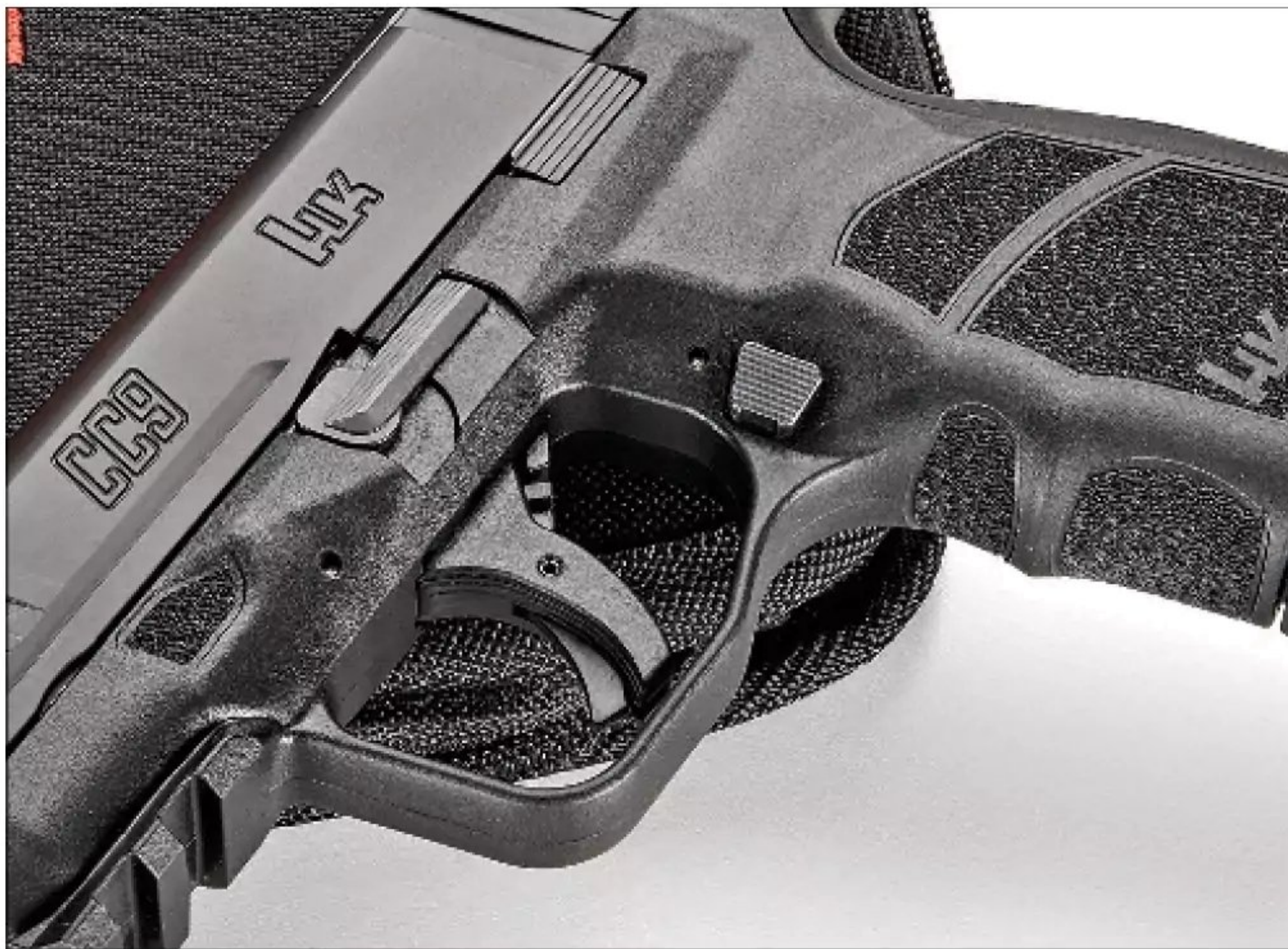
Controls are bilateral except for the takedown lever. With an unloaded CC9 and magazine removed, retract the slide and rotate the lever. A trigger press is unnecessary to disassemble.
