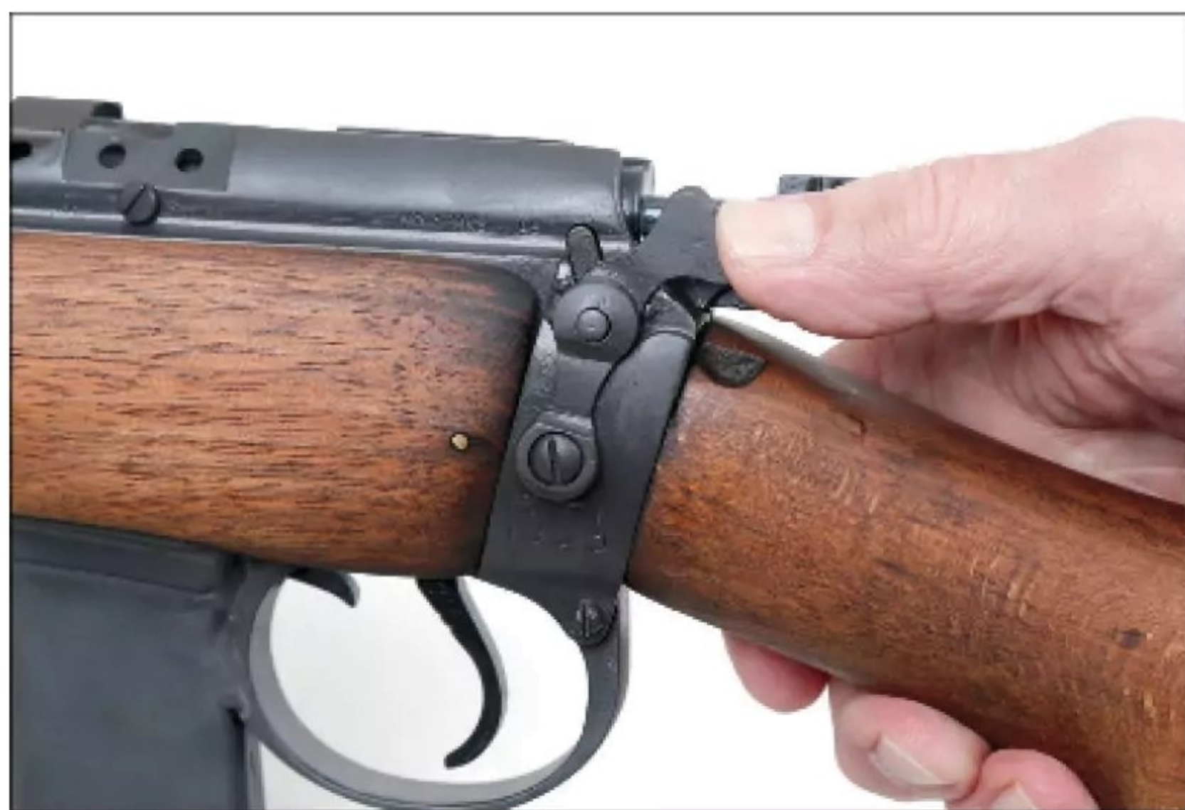
The original thumb-operated SMLE safety is employed in the De Lisle, as is the cocking piece.
