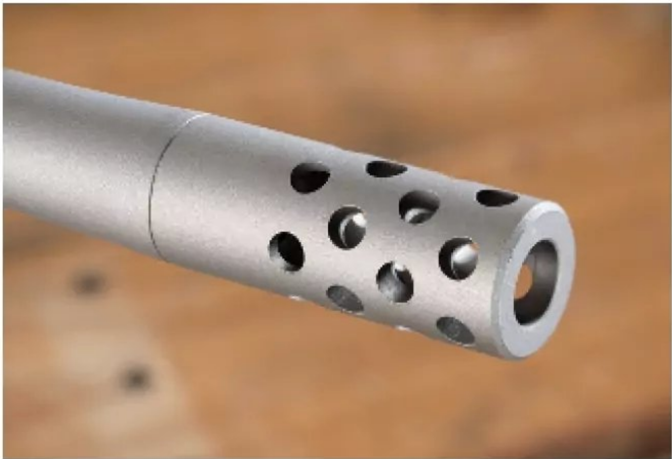
The muzzlebrake is effective at reducing felt recoil, but it does increase adjacent noise. The barrel has metric threads, so an adapter is required to suppress it.
