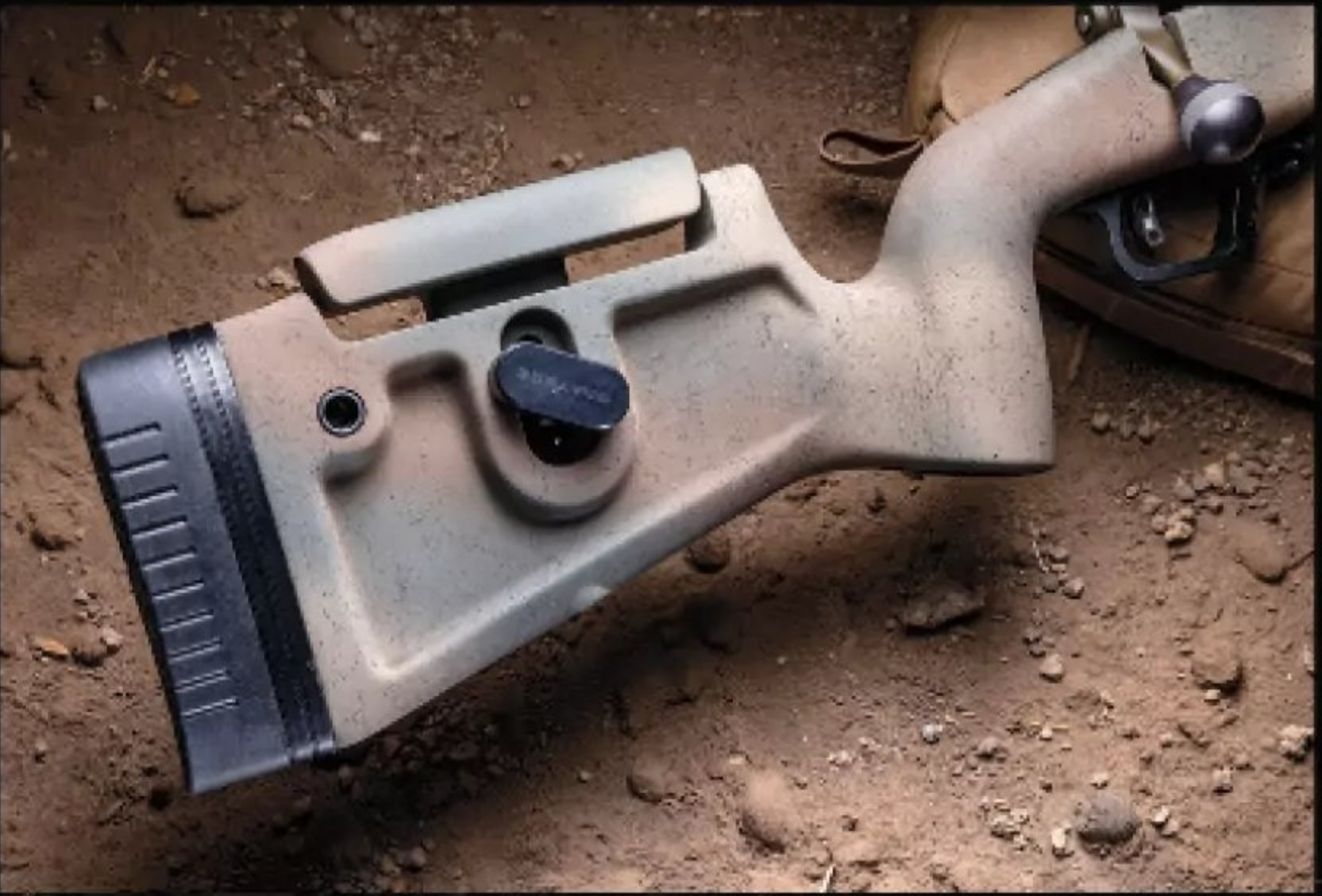
Comb height is adjustable, loosened and secured by twisting the knob on the right side of the stock. Length of pull may also be adjusted using a combination of the provided spacers.
