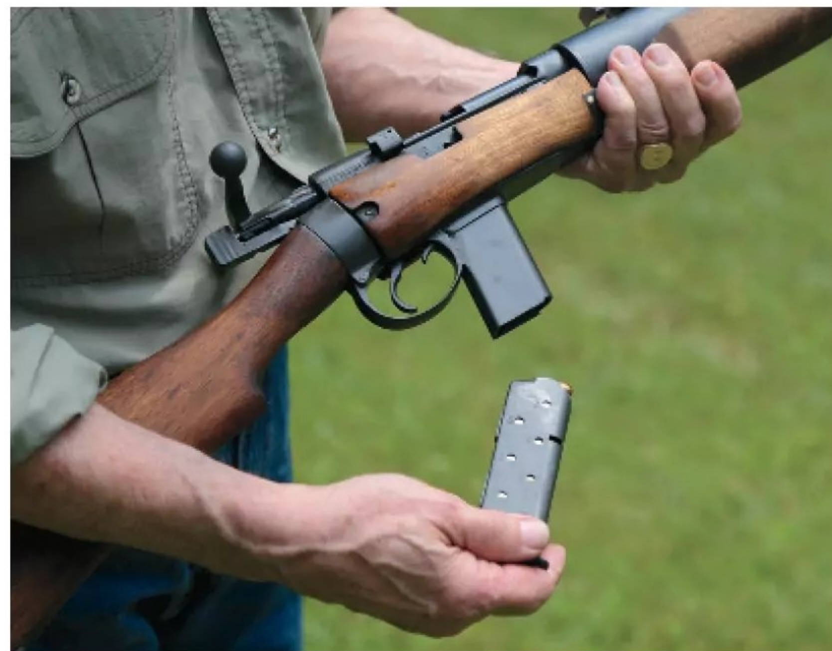
Inserting a modified .45 ACP magazine into the reconfigured SMLE mag well was easy and positive.
