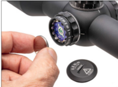
The reticle is powered by a common CR2032 battery. It is accessed by removing the reticle illumination cap.
