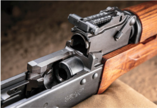
While early AKs were built from milled steel blocks, the AKM switched the platform to stamped and folded steel around a trunnion. The Hellpup is based on the AKM design.
