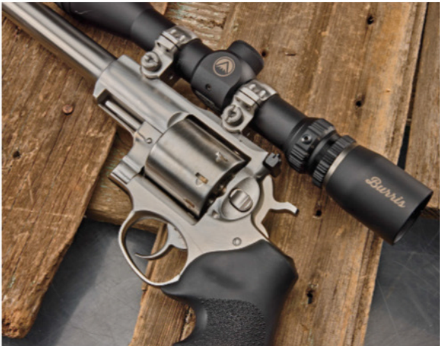
The Super Redhawk was designed to accept handgun scopes featuring extended eye relief. A contemporary red dot on an optic rail would suffice for target shooting and hunting, too.
