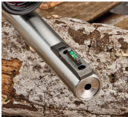
The cold-hammer-forged barrel features a recessed 11-degree target crown to protect the rifling near the muzzle. The twist rate is 1-in-9 inches.
