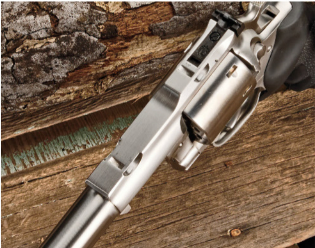
The thick topstrap of the frame supports loads such as the .454 Casull and .480 Ruger in the Super Redhawk. Though a small caliber, the .22 Hornet is a cartridge producing up to 44,000 psi.
