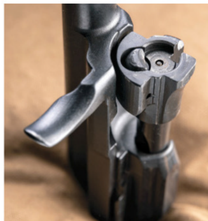
The bolt carrier supports the rotating bolt assembly, which contains the large extractor and firing pin.
