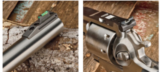
A HiViz fiber-optic front post and adjustable U-notch rear sight are adequate. For precise shooting irons sights are preferred by many versus optics.
