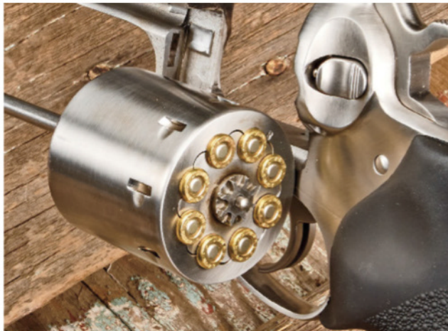
The cylinder and barrel are incredibly stout. The smooth cylinder accommodates eight rounds of .22 Hornet. To swing out the triple-locking cylinder, simply press the cylinder release button.
