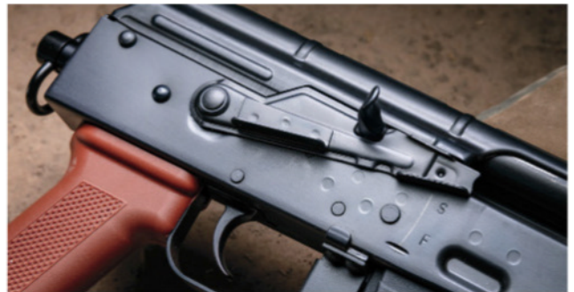
The safety selector can be engaged up to "S", preventing the bolt from cycling (top) or down to "F" for semiautomatic fire (middle). It is also notched to capture the bolt handle (bottom).
