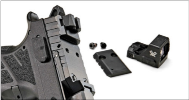
A Shield RMSc and Holosun K footprint was used for the P-09 C Nocturne slide. A Vortex Defender CCW was mounted for testing.
