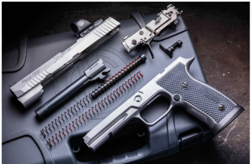
Fieldstripping includes removal of the serialized FCU, which contains the trigger, slide-lock lever and sear assembly. The P320 remains the easiest chassis system to remove from a grip module.
