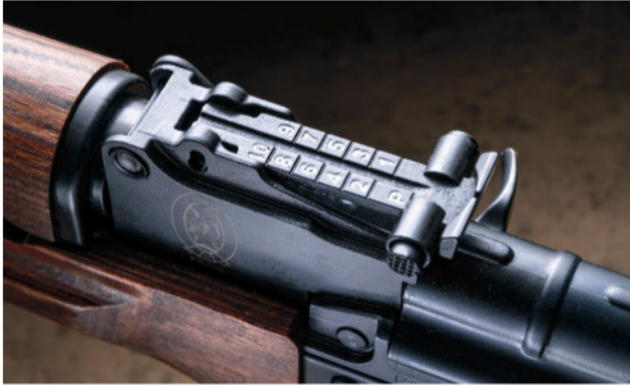
Short AK pistols have the front sight assembly pressed against the gas block. At the rear is a sliding ladder-style sight that can be adjusted from point-blank to an optimistic 1,000 meters.
