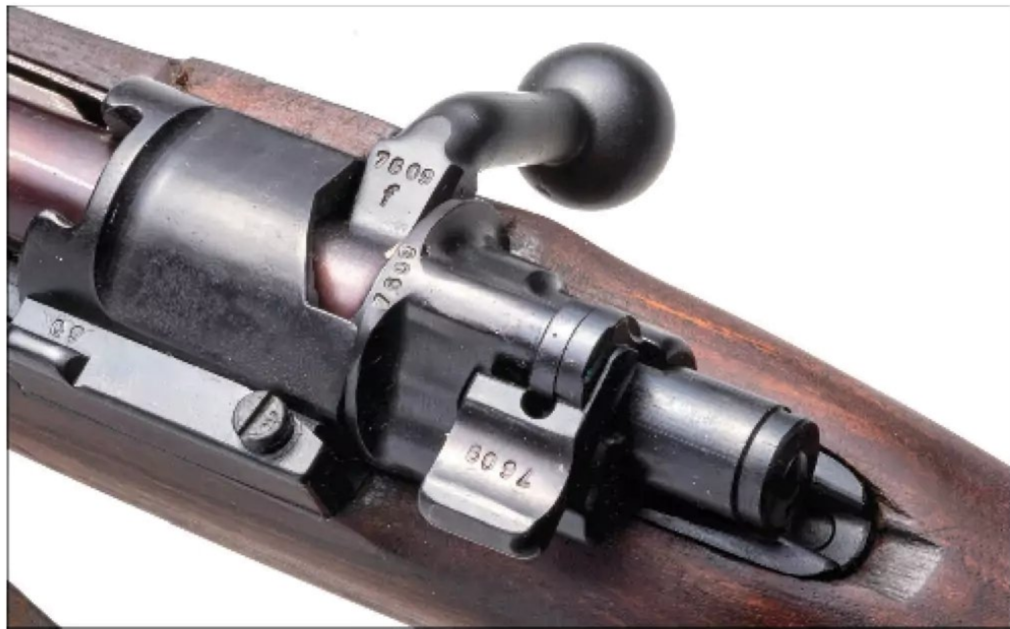
The last two or four digits of the serial number were often stamped on many parts. For collectors, these support originality.
