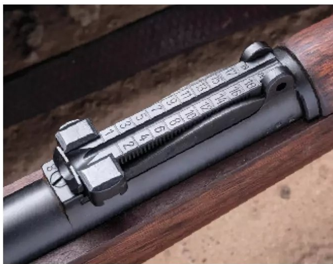
Early Mauser sights were stamped on both sides with range indicators. Later models abandoned this level of detail, eventually giving up on adjustable sights altogether.
