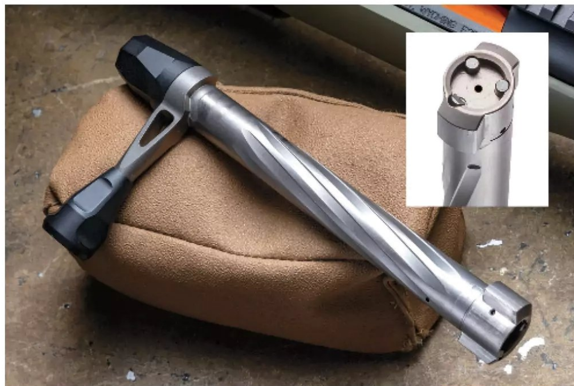
The two-lug bolt features a near 90-degree lift, robust handle, and dual ejectors opposite of a Model 1911-inspired extractor design.
