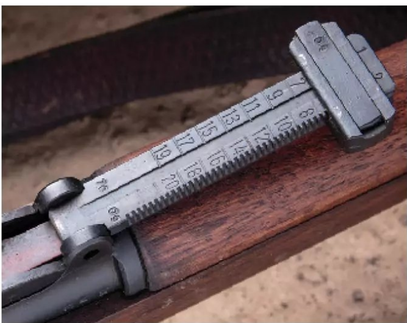
Early Mauser sights were stamped on both sides with range indicators. Later models abandoned this level of detail, eventually giving up on adjustable sights altogether.
