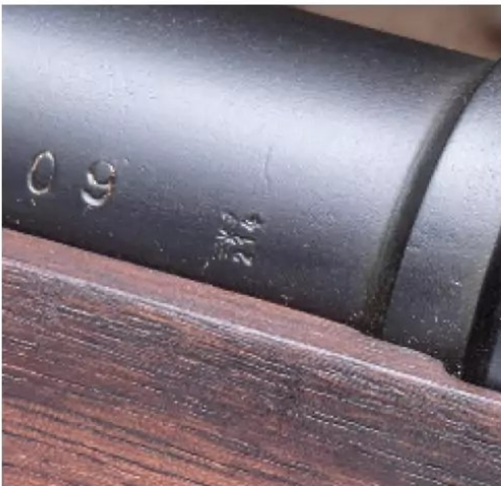
Inspector marks featuring an eagle over a number are often found on individual parts and assemblies.
