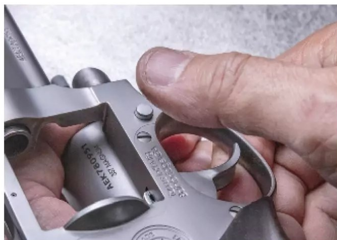
To unload the seven-shot cylinder, press the extended ejector rod to eject the cases. To remove the cylinder from the frame, depress the cylinder-release button on the right side of the frame while pulling the assembly forward and out of the frame; reinstall it in reverse order.
