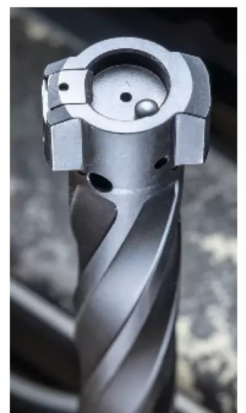
A one-piece bolt offers a comfortable bolt knob turned down for leverage, and to prevent fingers hitting a low-mounted optic. The two-lug bolt head surrounds the large extractor and ejector.
