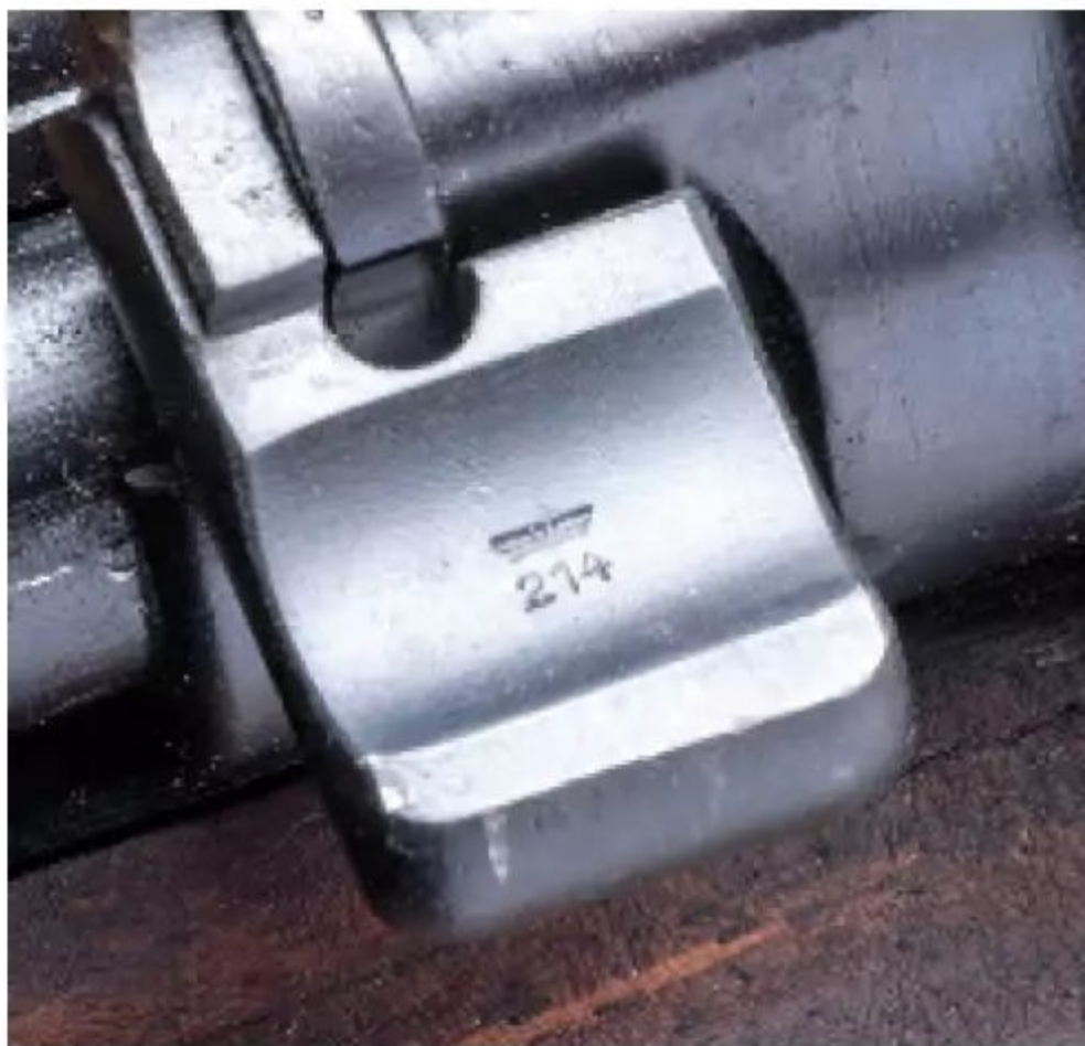
Inspector marks featuring an eagle over a number are often found on individual parts and assemblies.
