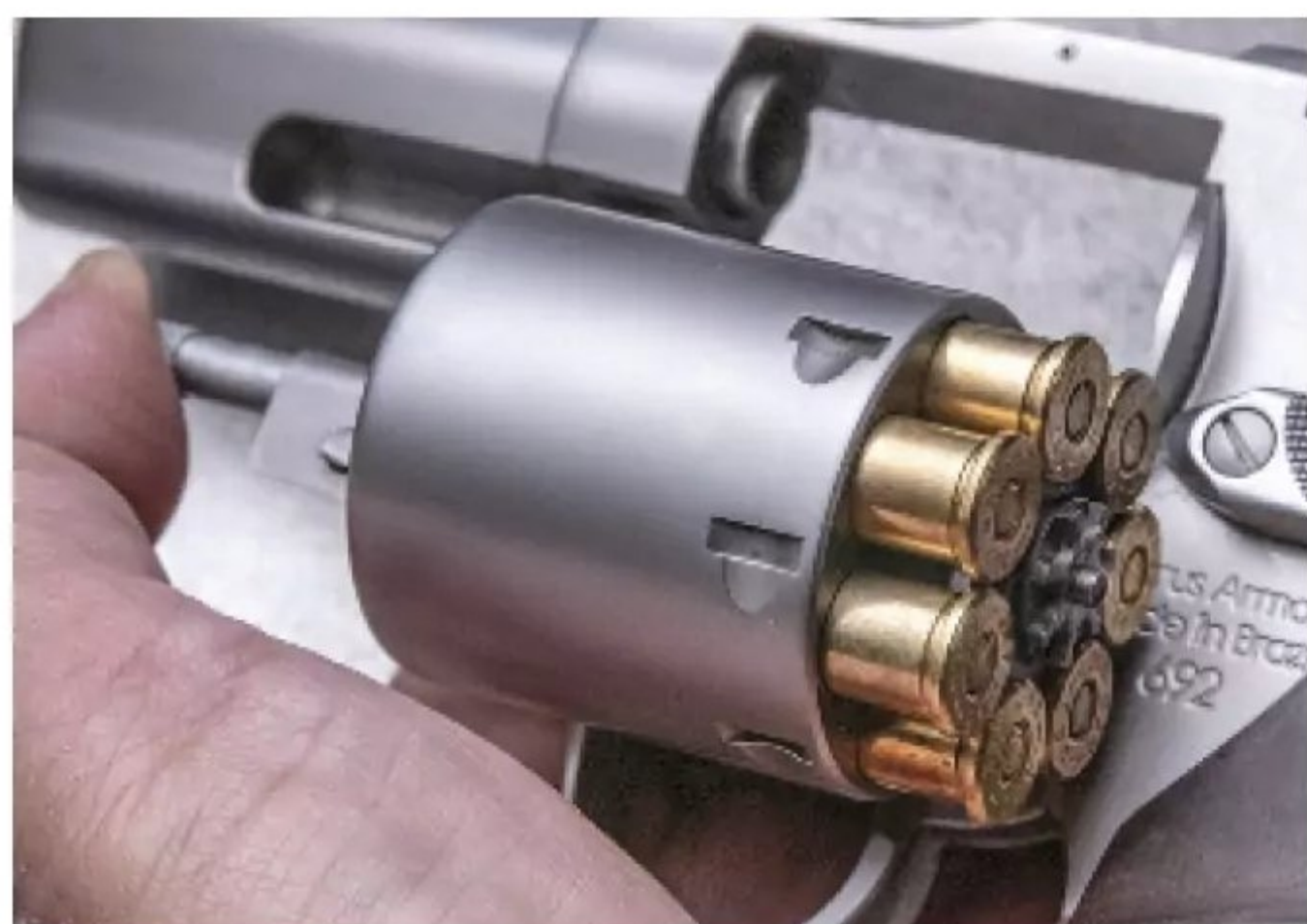
To unload the seven-shot cylinder, press the extended ejector rod to eject the cases. To remove the cylinder from the frame, depress the cylinder-release button on the right side of the frame while pulling the assembly forward and out of the frame; reinstall it in reverse order.
