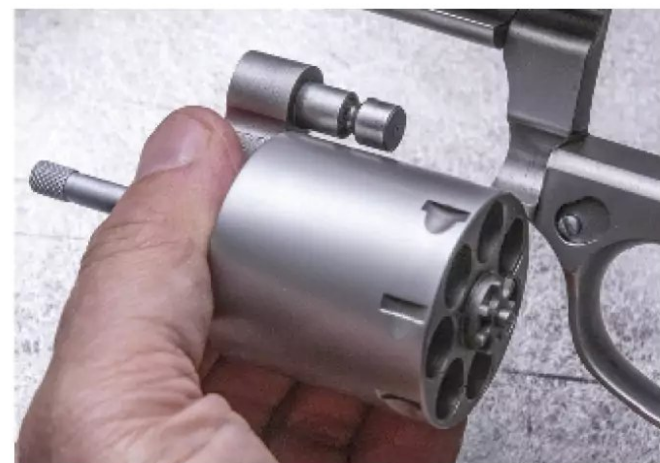
To unload the seven-shot cylinder, press the extended ejector rod to eject the cases. To remove the cylinder from the frame, depress the cylinder-release button on the right side of the frame while pulling the assembly forward and out of the frame; reinstall it in reverse order.
