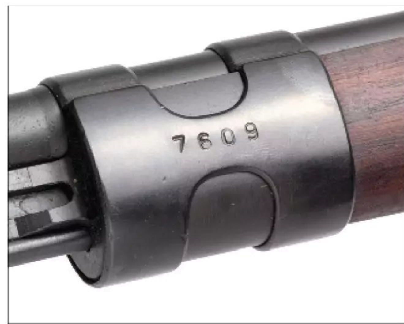
The front barrel band usually had lightening cuts, giving it a distinctive "H" shape.
