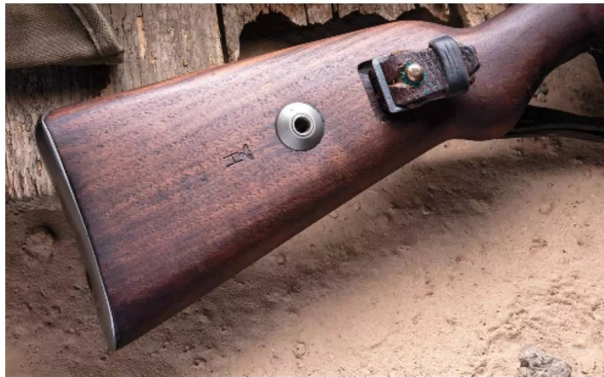
Stocks changed from solid walnut to laminated beech. The round part above the stock inspector cartouche is a bolt takedown disc.
