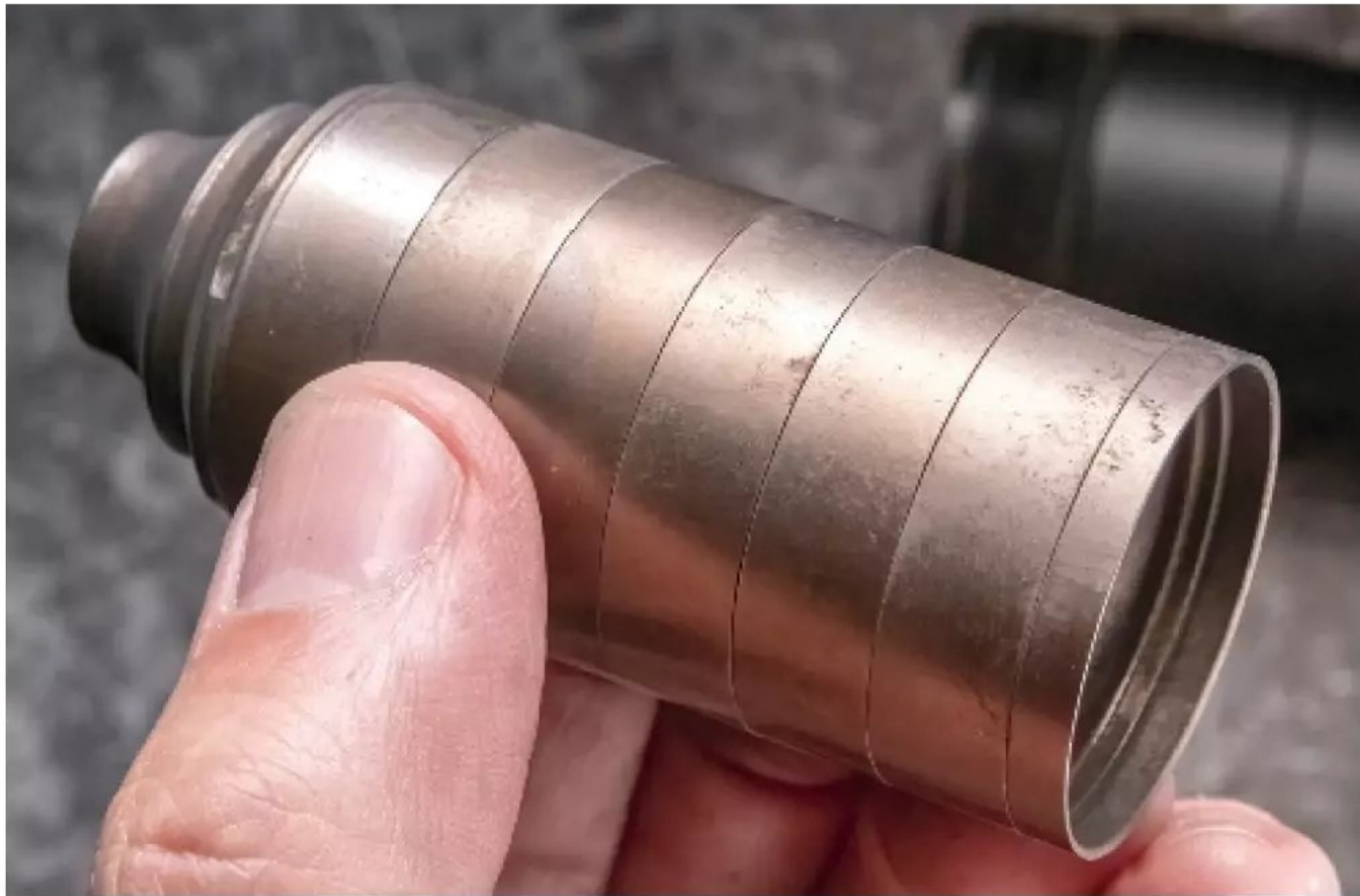
Baffles are made from 17-4 stainless steel and are keyed with indexing tabs to let users align them properly. The baffles also interlock in a way that creates a gas seal, significantly reducing carbon buildup.
