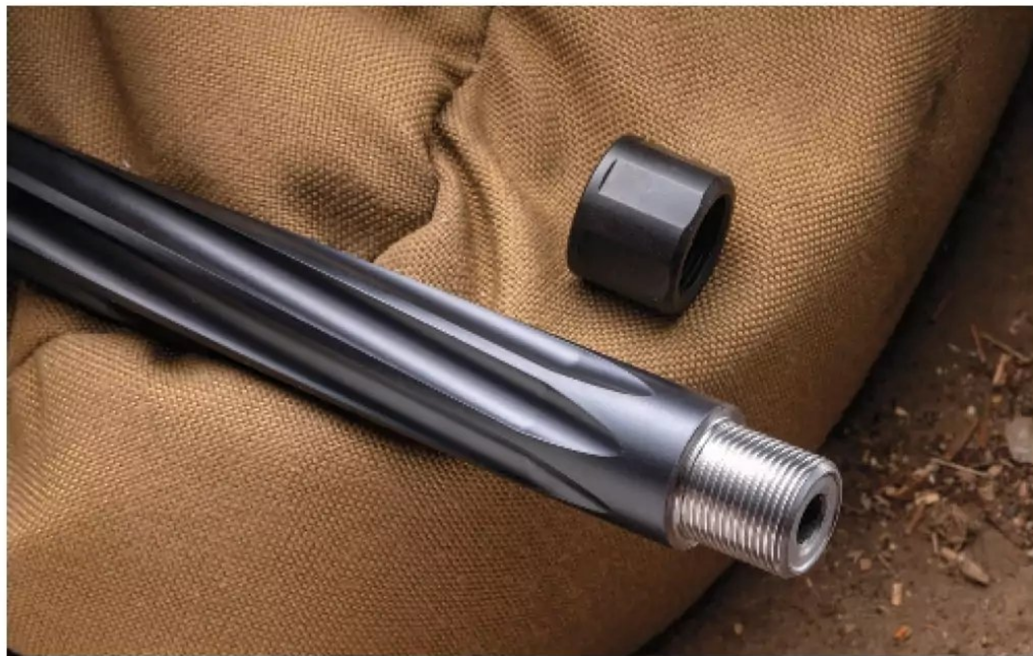
Ballistic Advantage manufactures the lightweight-profile barrel. Spiral fluting reduces weight while enhancing aesthetics. It is threaded 5/8-24 for attaching muzzlebrakes or suppressors.
