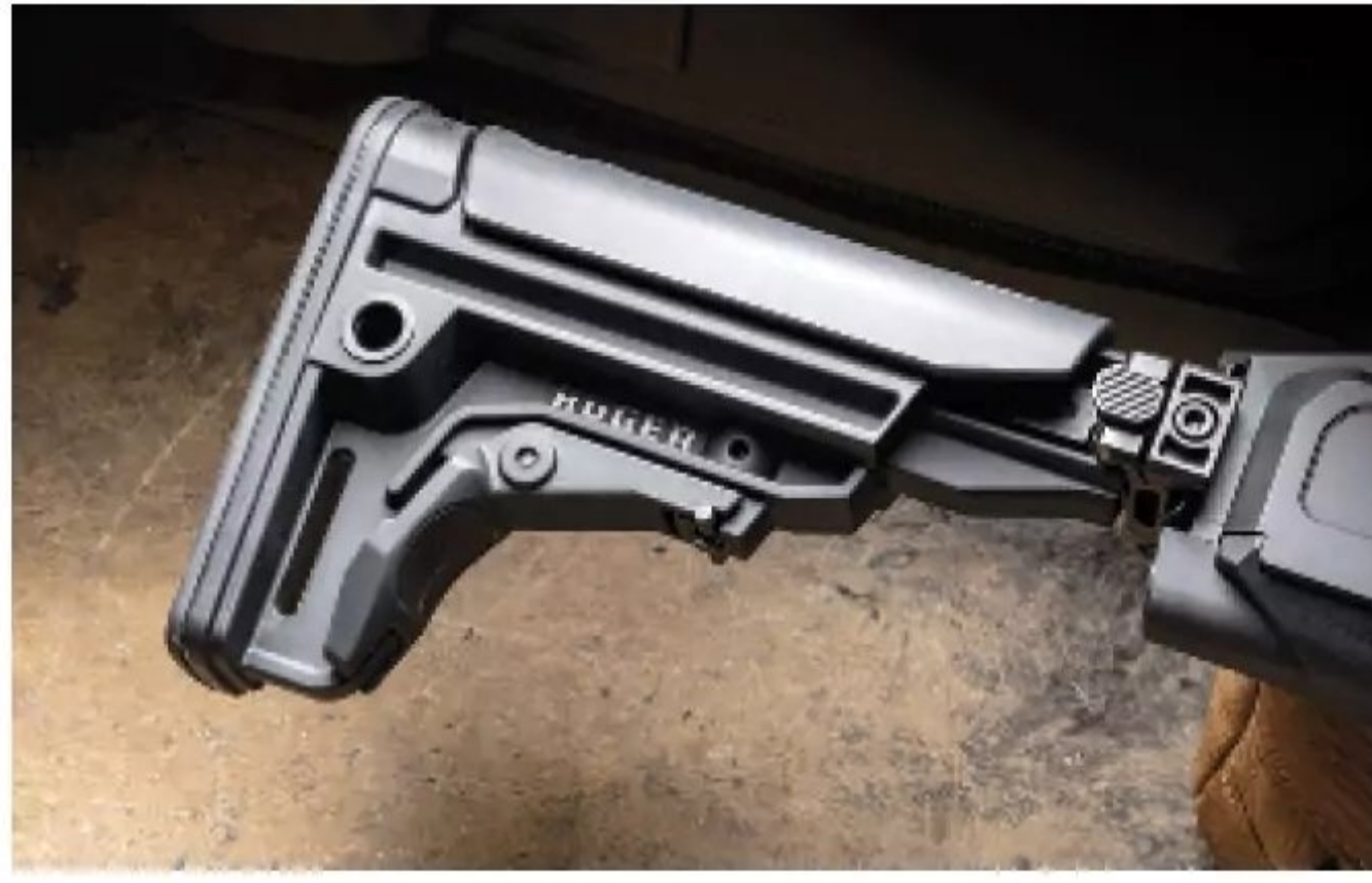
The stock features an adjustable length of pull, from 12 to 14½ inches. The stock also offers a sling-cup socket and a vertical slot to thread the rear attachment point of a sling.
