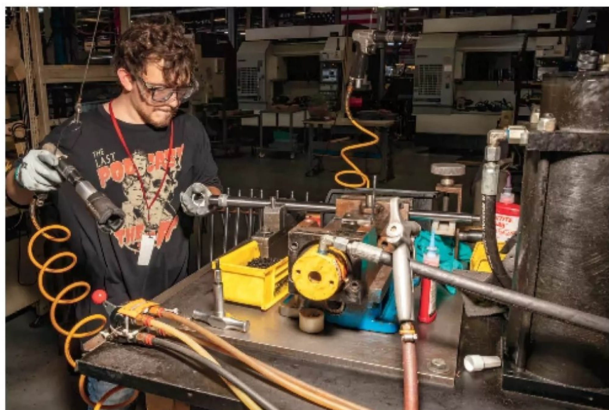
Once threaded, a precision machined barrel nut and lug is installed to each Savage barrel before it is joined with the action.
