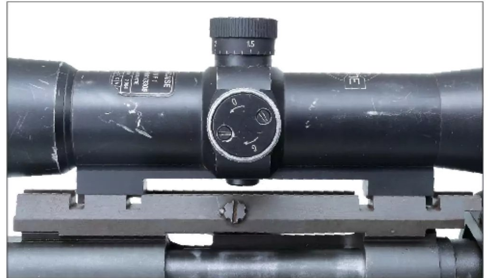
The Scrome J8 8x40mm scope reticle is adjusted using two dials. Initials on the top are B (Bas for "down") and H (Huit for "up") and on the side, D (Droit for "right") and G (Gauche for "left").
