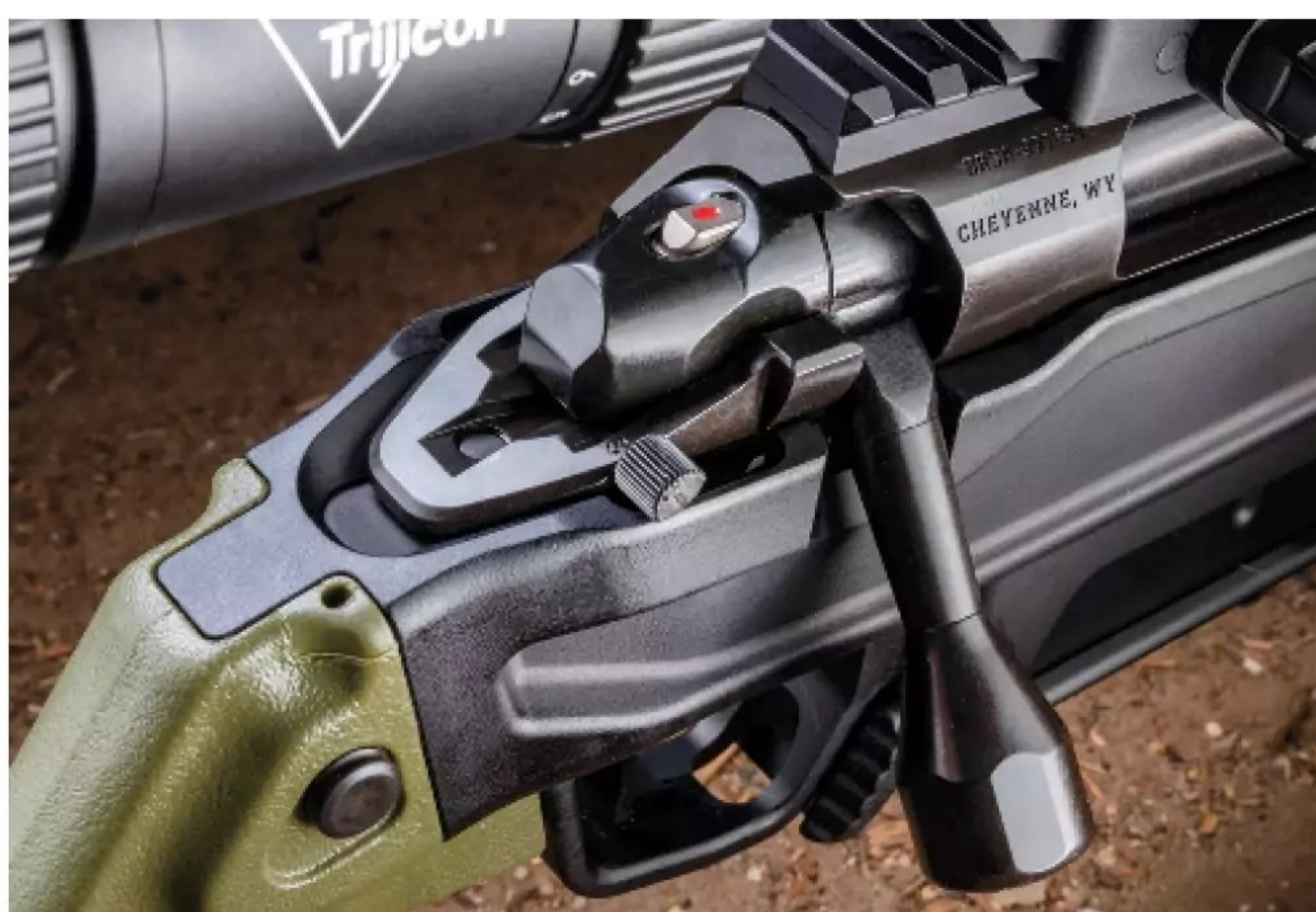
A sear-blocking safety lever is part of the TriggerTech trigger and located just behind the bolt handle. The oversized bolt handle provides excellent leverage, and the short bolt lift was fast.
