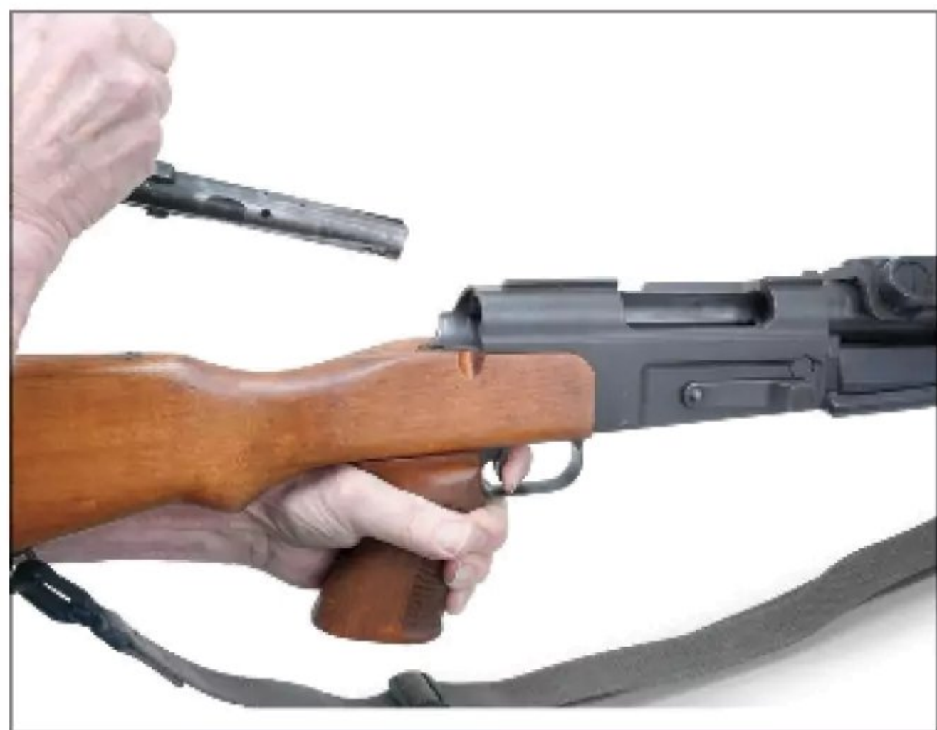
The bolt is easily removed by opening it and moving it to the rear while the trigger is in the rearward position.
