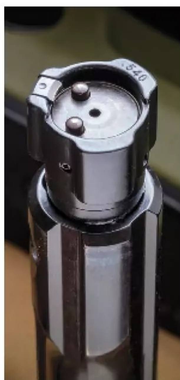
The three-lug bolt head is inter-changeable. Flanking the extractor, dual ejectors ensure cases exit the receiver.
