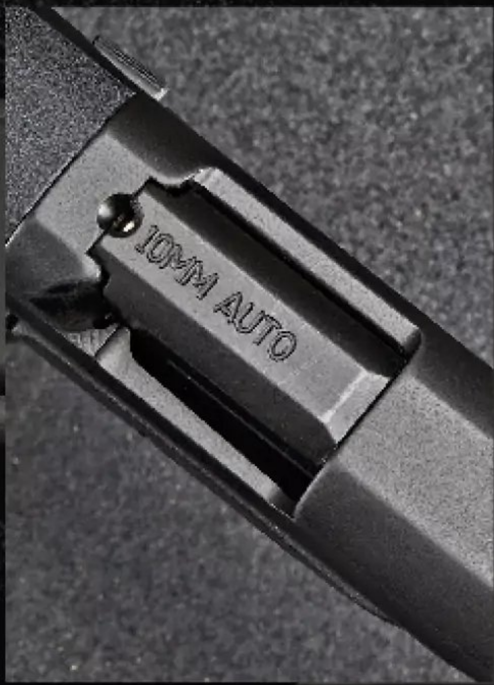
A loaded chamber port appears at the top of the slide and barrel. When a round is loaded, the user is able to see the rim of the cartridge under the barrel hood.
