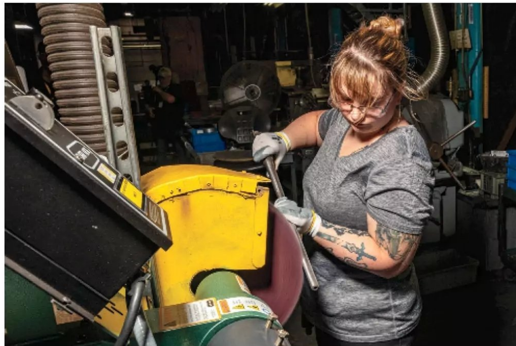
Barrel marks and machining scars are removed by hand using industrial polishing wheels. The resulting finish is flawless.
