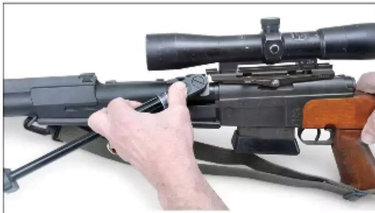
The FRF2 bipod can be lowered into position using buttons on each leg. The legs are extended by spring-mounted detents.
