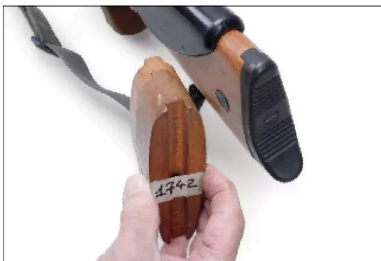
The stock can be extended to suit the marksman by adding a dovetailed wooden insert of the desired length. It is secured by a bolt through the butt.
