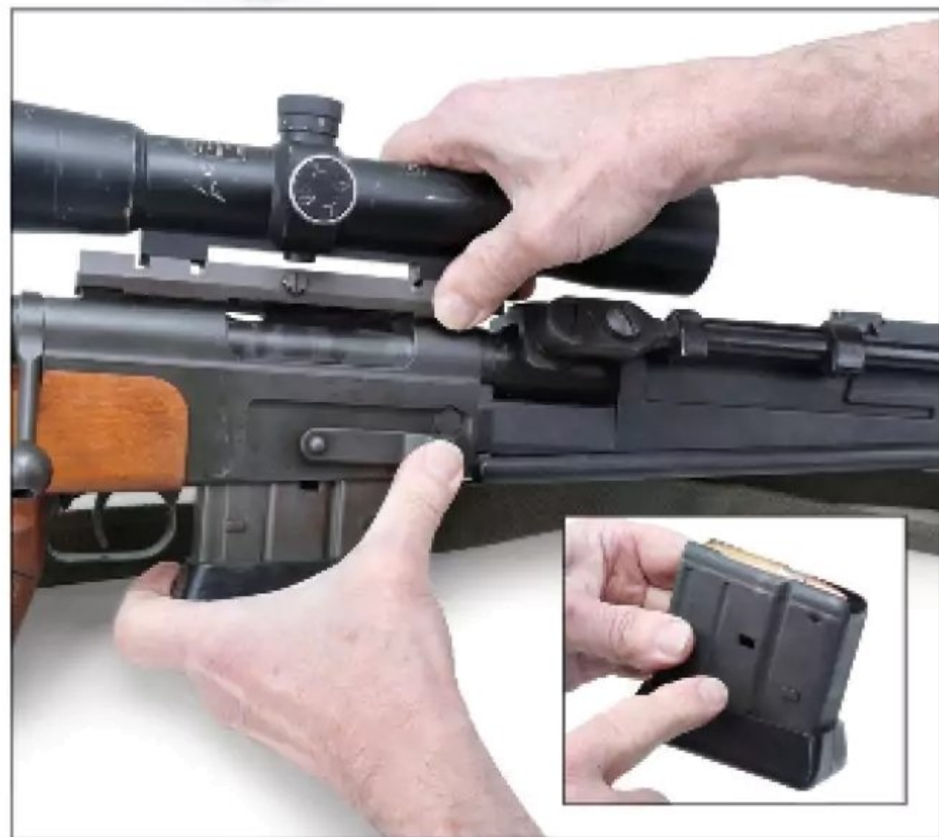
The FRF2 has a 10-round magazine released by a generous lever sited on the lower portion of the side on the action where it is operated by the shooter's thumb. It is secured in position by an internal flange that snaps into a small recess on the magazine body.
