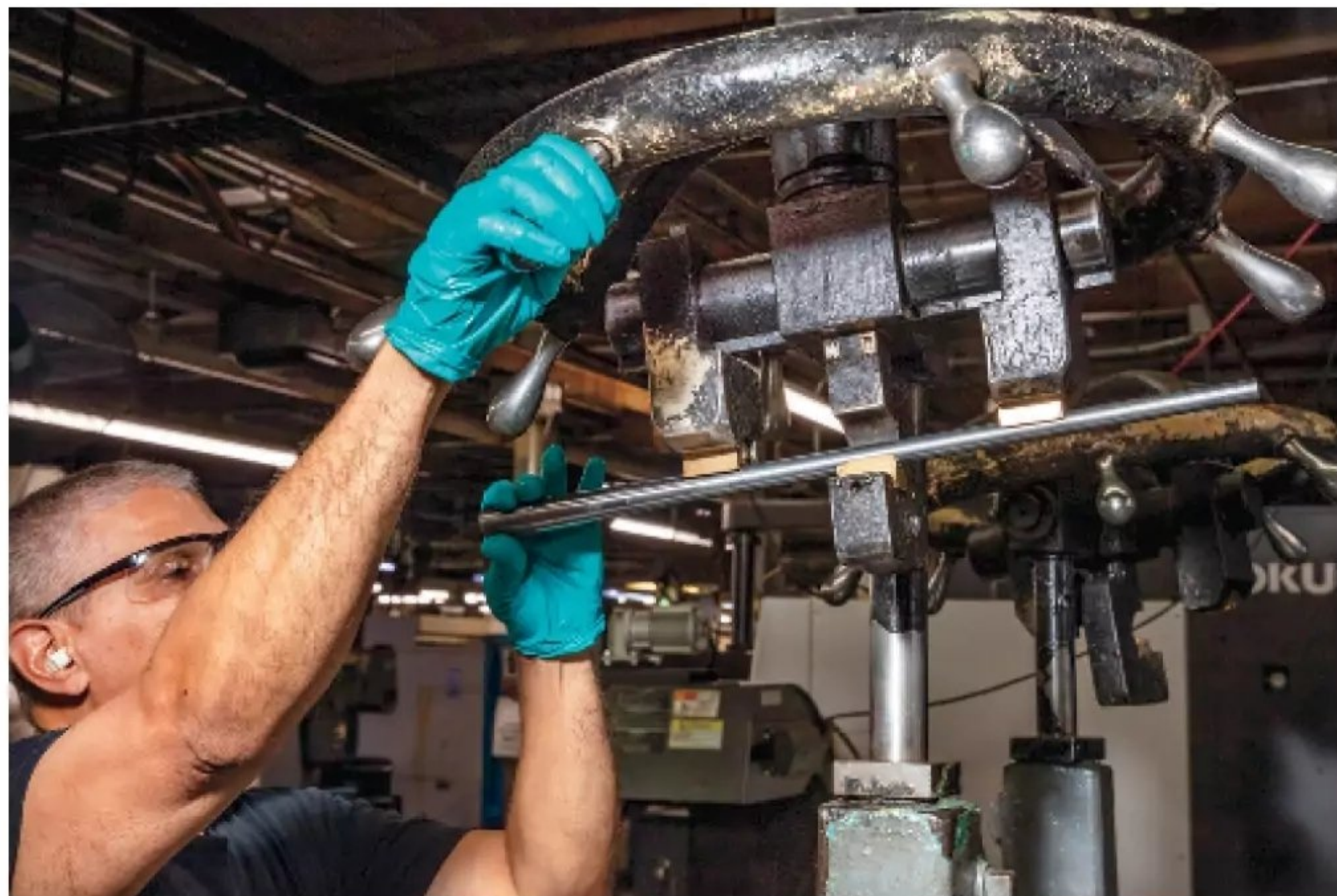
A vintage hydraulic press is used to achieve perfect barrel straightness, a task left to skilled human experience.
