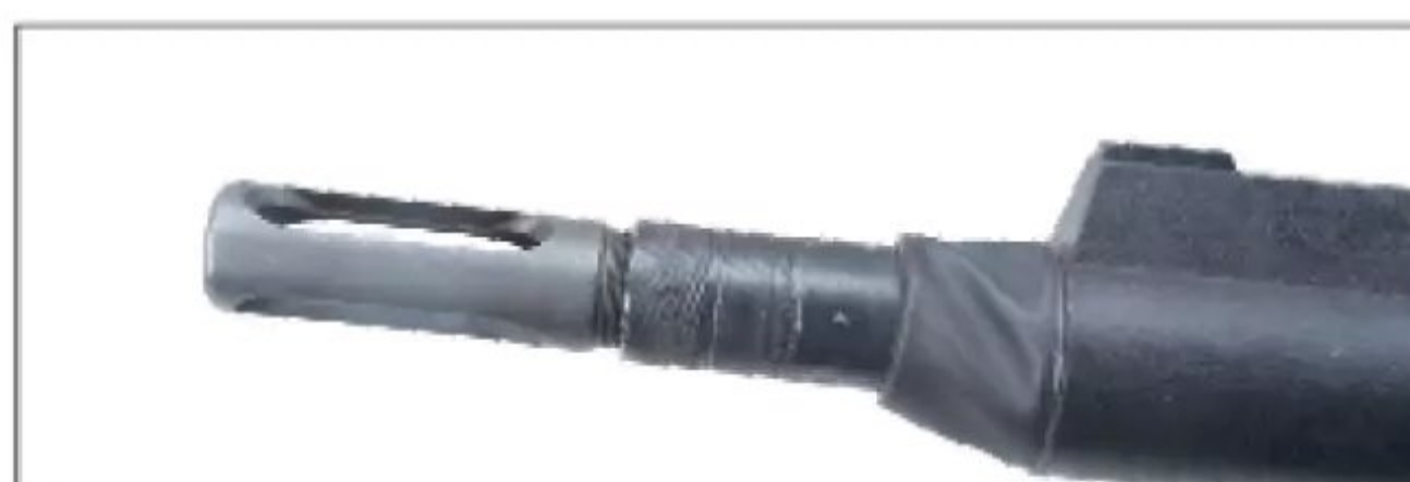
The flash suppressor is adjustable and properly aligned with the barrel's lands/grooves for optimum accuracy and ballistics. A rubber enclosure between the suppressor and handguard is another safeguard against thermal deflection.
