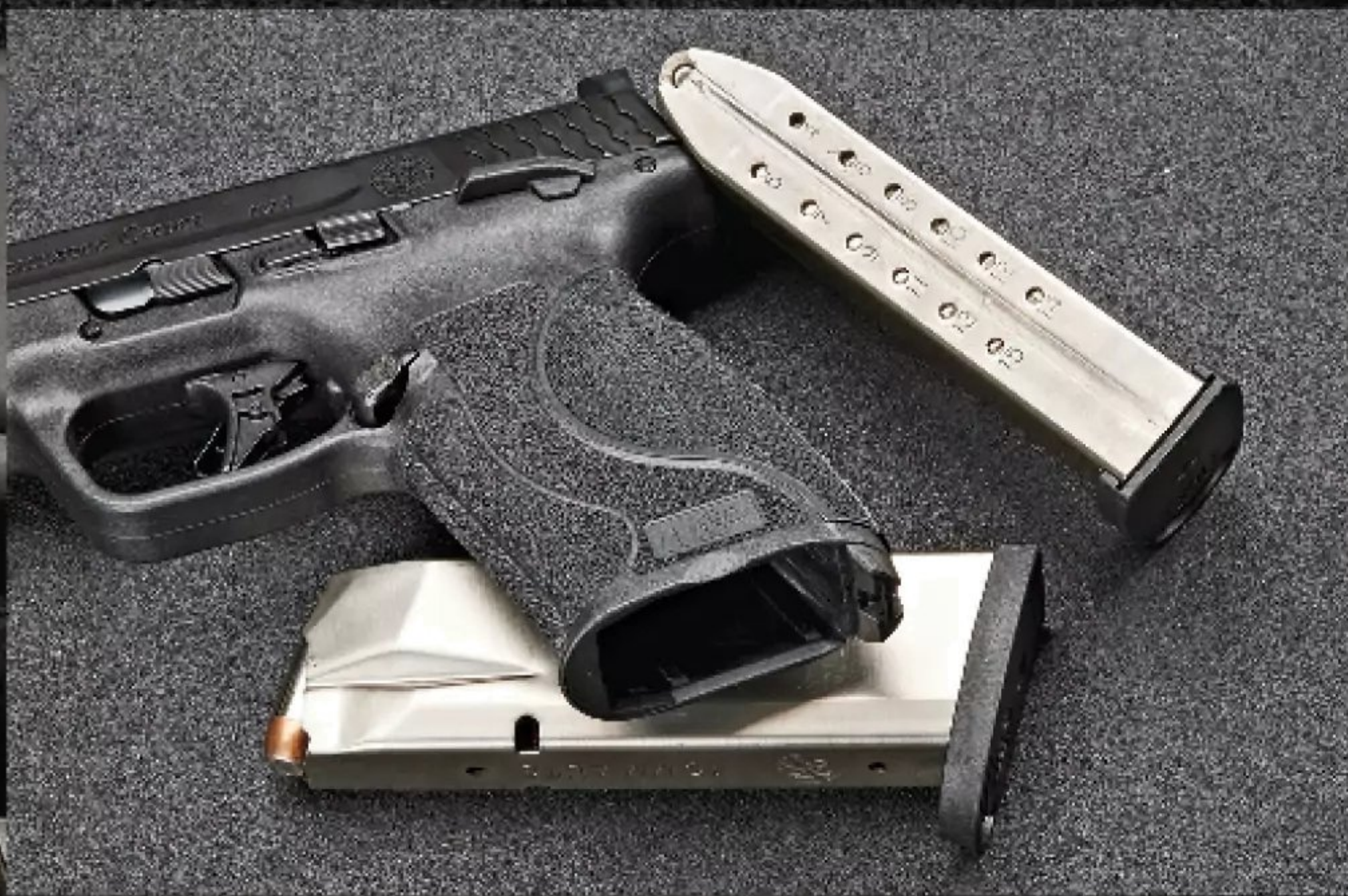
Stainless-steel double-stack magazines accommodate 15 rounds of 10mm. The dimensions required the M&P10 M2.0 frame be made larger. The frame features grip support and large magwell.
