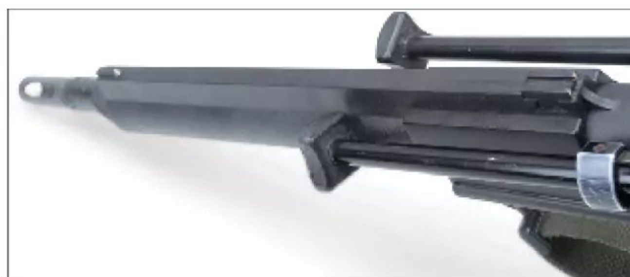
A simple notch-and-blade arrangement is molded into the rifle's polymer handguard so the rifle could be used without a scope.
