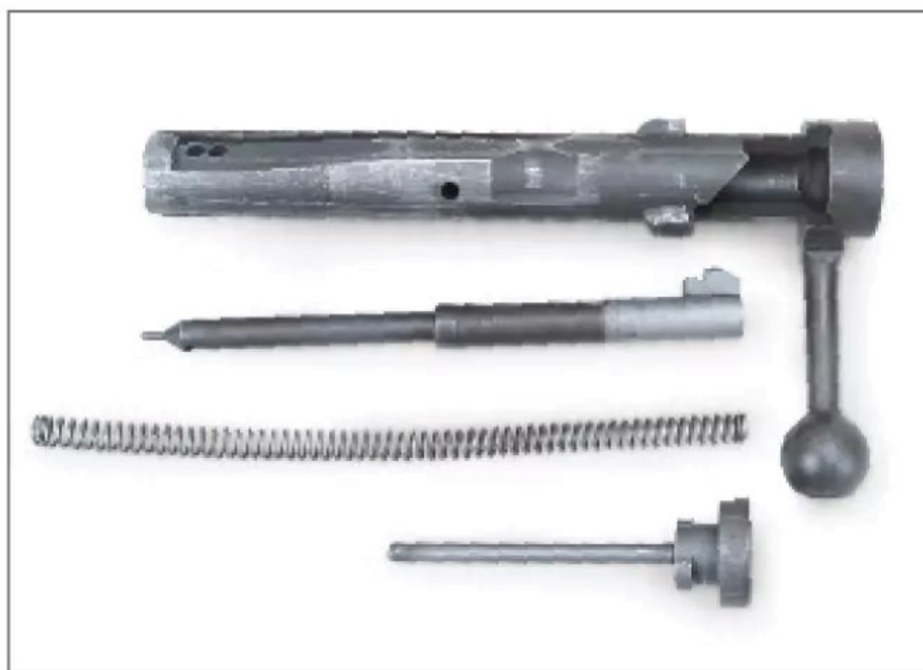
An FRF2 bolt is easily disassembled by simply pushing in on the knob at the rear and rotating it clockwise until it disengages. The spring and striker can then be removed.
