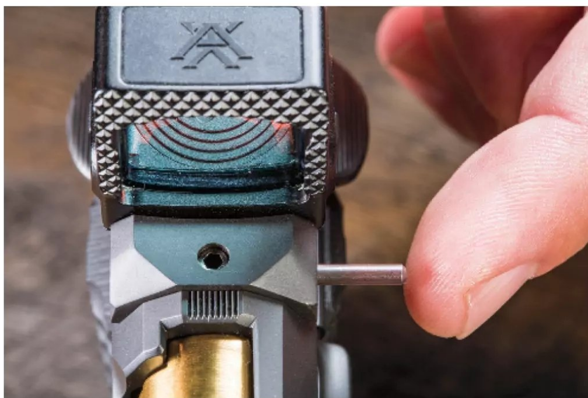
The dovetail-milled slide allows for repeatable zero. The IOS plate is indexed with a retainer pin, which is secured by tightening a set screw.
