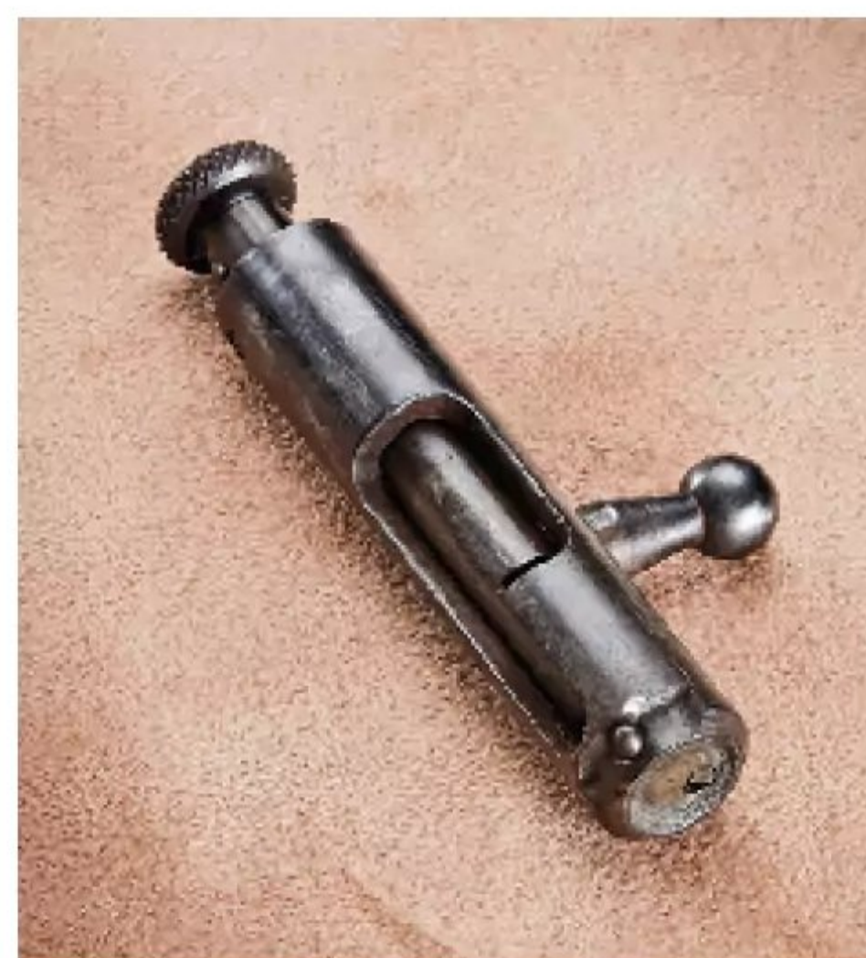
The barreled action was notched to accept a simple bolt. The striker wasn't cocked until the action was closed and the knurled knob was pulled back.
