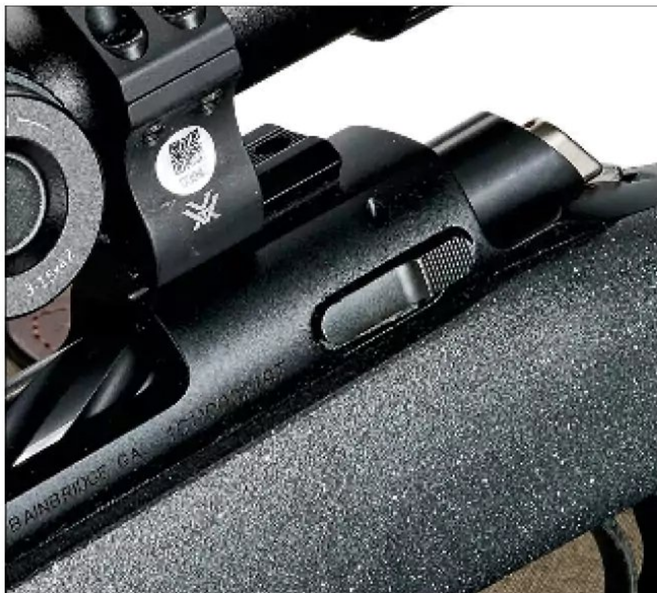
The bolt-release is a lever pinned to the left side of the receiver. With the action open, press it to remove the bolt.
