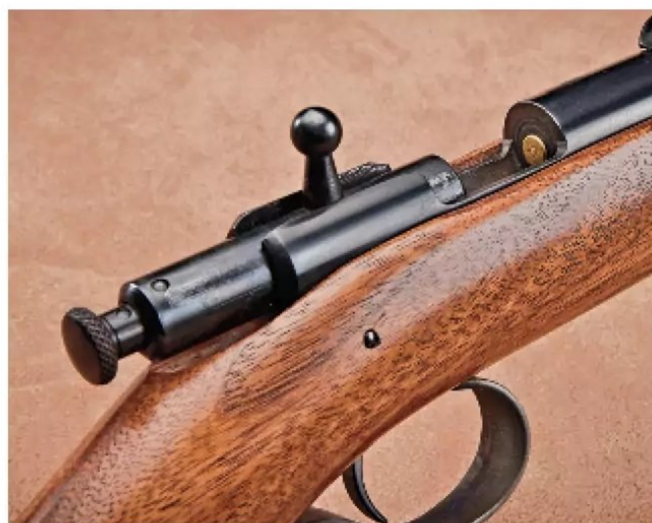
The barreled action was notched to accept a simple bolt. The striker wasn't cocked until the action was closed and the knurled knob was pulled back.
