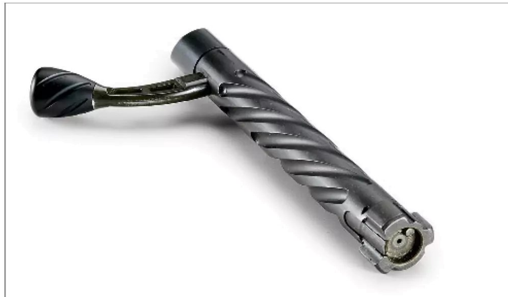
The short-action, .308 case-head bolt features an external extractor, plunger-type ejector, and three locking lugs for a quick-cycling 60-degree bolt lift. Abundant fluting saves weight.
