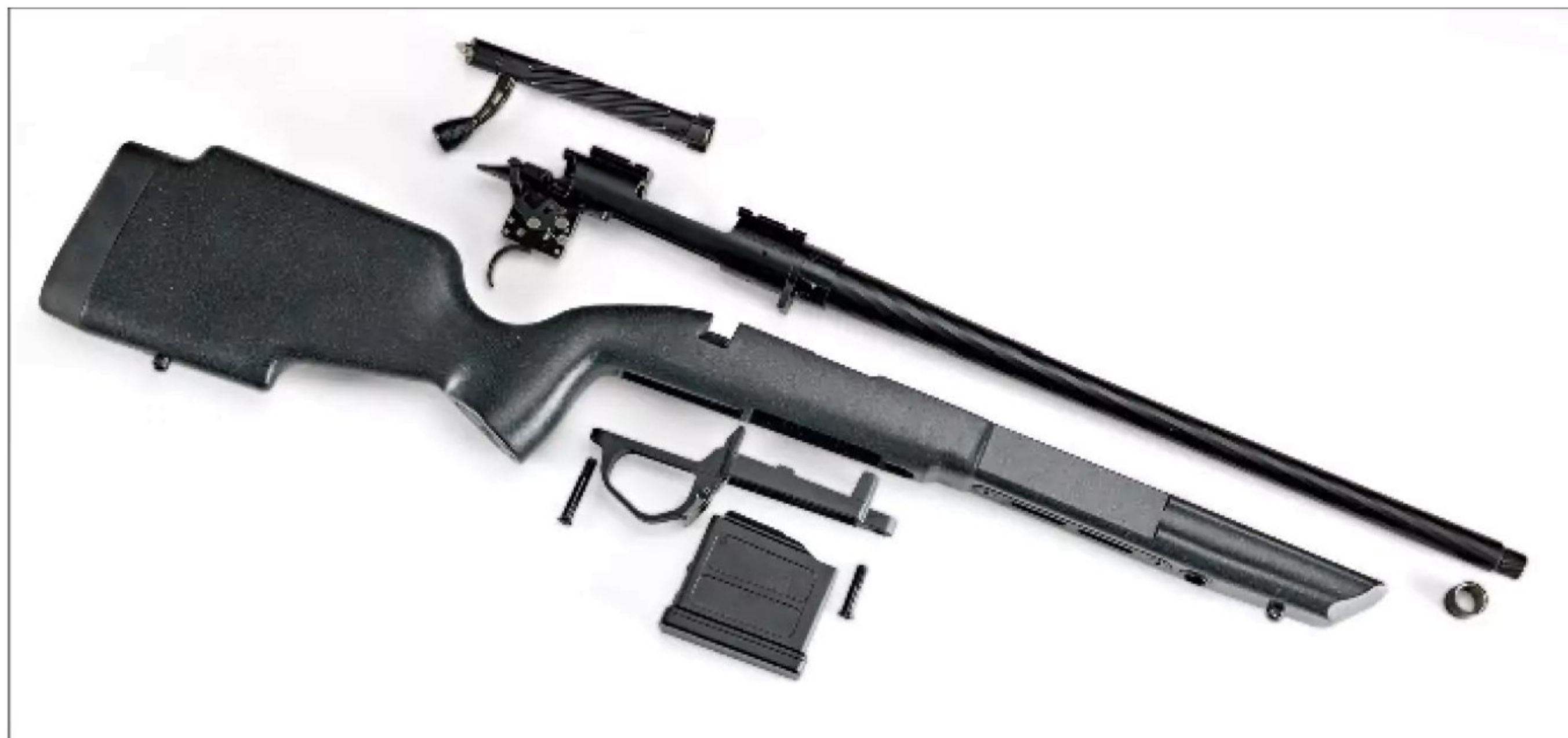
Disassembly of the Expedition is familiar, following the removal of the bolt assembly and two action screws. The bottom metal is actually polymer, a one-piece design containing the triggerguard and mag well. The barrel has a tapered contour and threaded muzzle.
