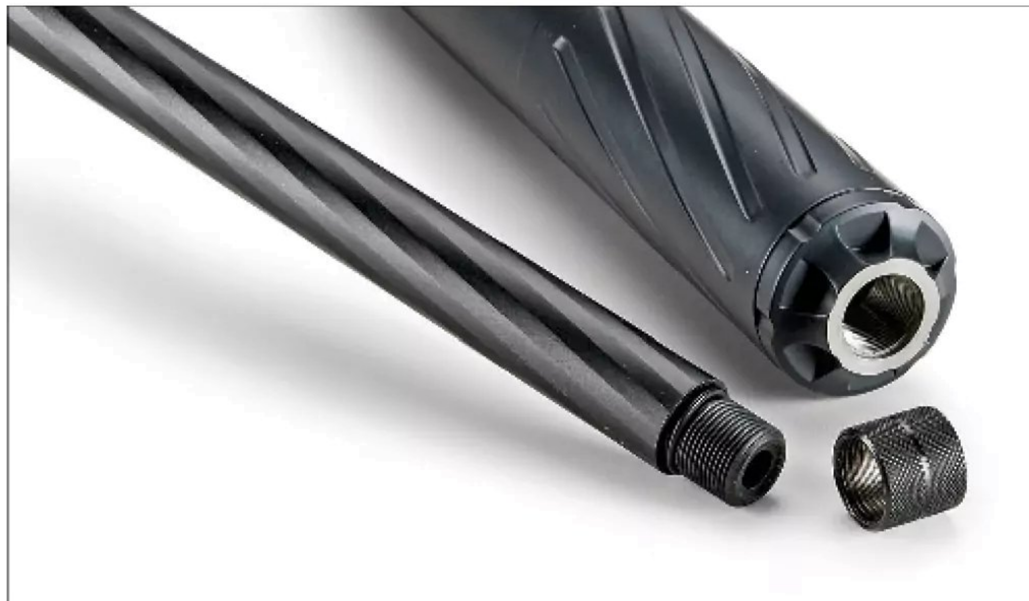
The hammer-forged, stainless-steel barrels are manufactured by Taurus in Brazil. The .308 test rifle featured a 1-in-10-inch twist rate complete with 5/8x24 threads and a knurled thread cap.
