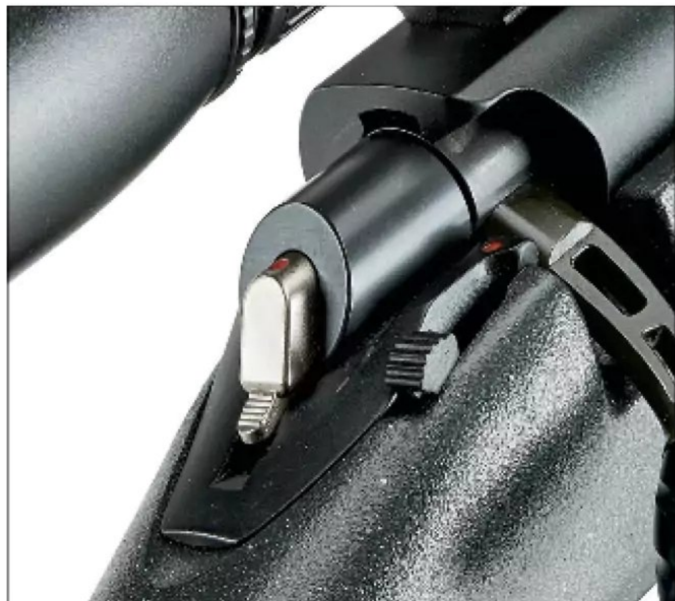
A stainless-steel cocking indicator protrudes from the rear of the bolt when cocked. The safety lever is to the right.
