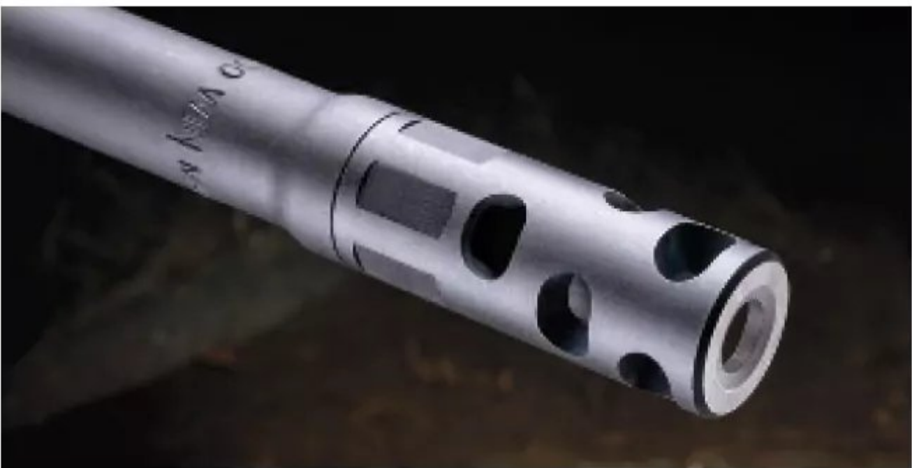
The Cross Magnum includes a radial muzzle-brake with ports that reduce felt recoil and prevent rotating torque from the .300 WM.
