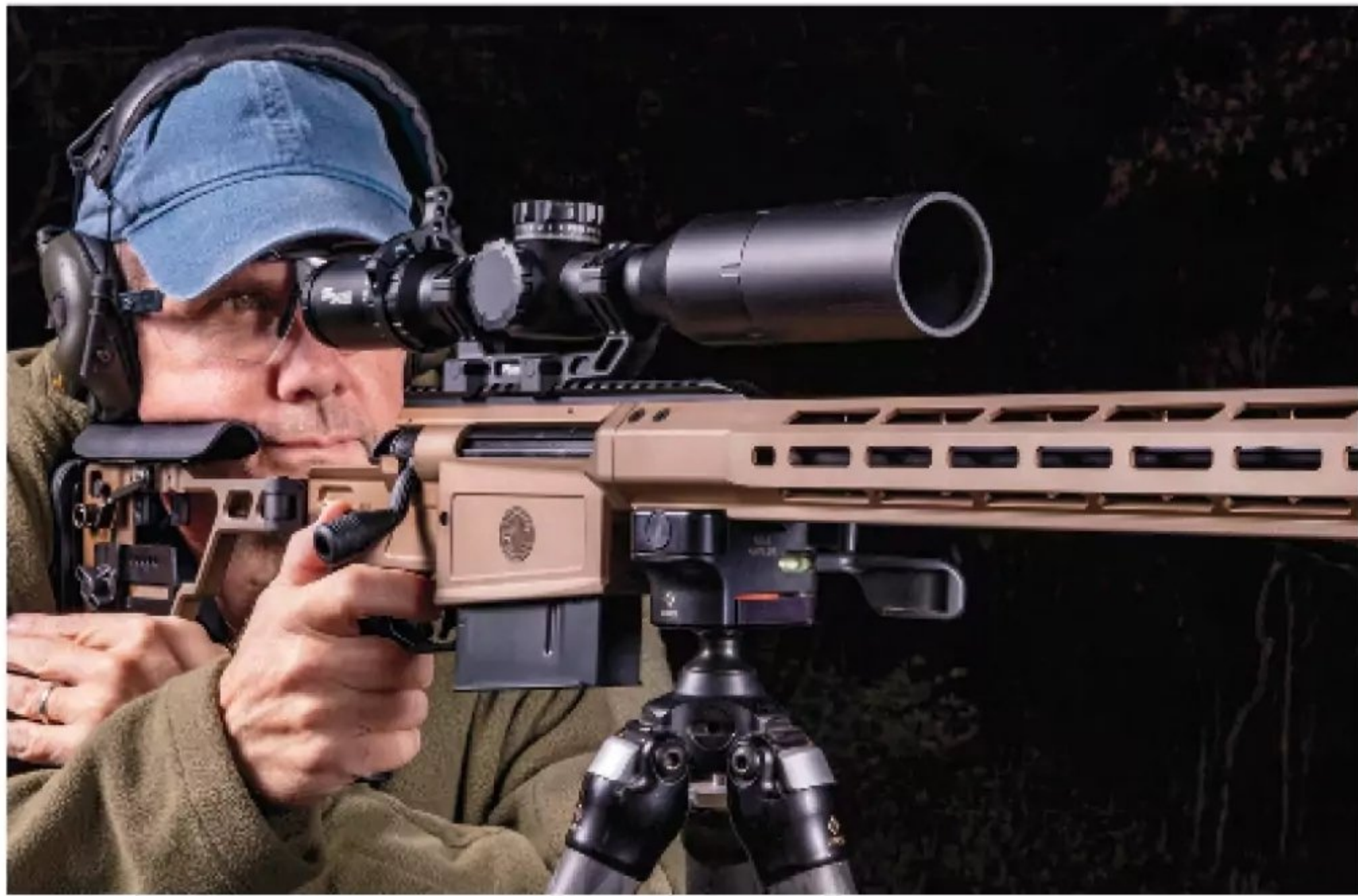
The Cross Magnum's aluminum handguard has M-Lok slots for accessories and an integral ARCA rail along the bottom for easy mounting and repositioning of bipods and tripods.
