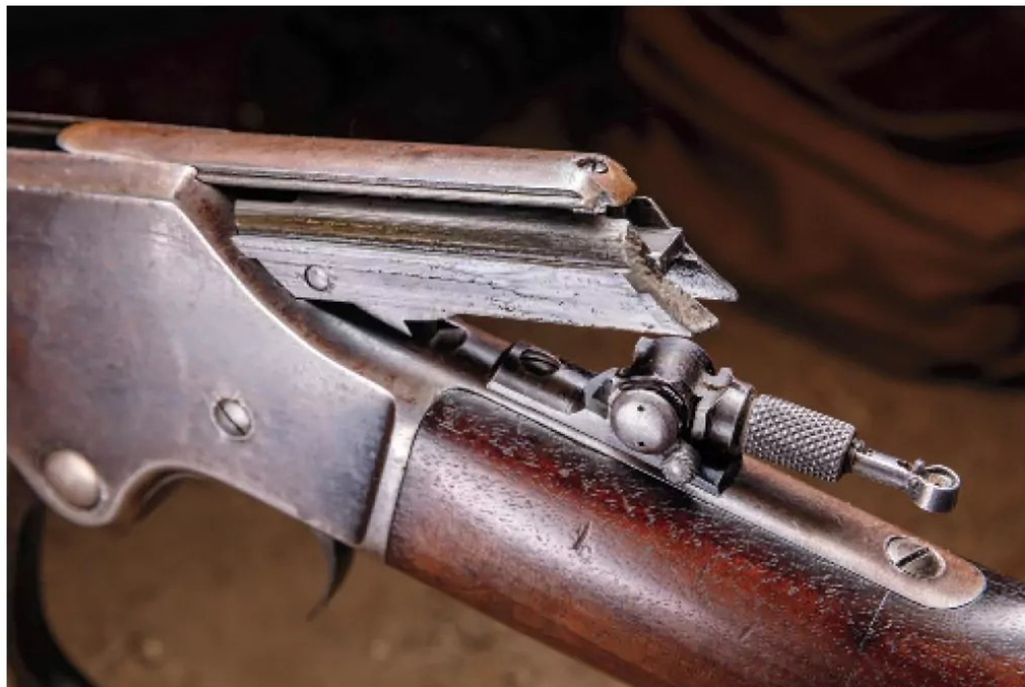
The bolt features an integrated dustcover. One issue with using some tang sights is racking the bolt knocks the sight back.
