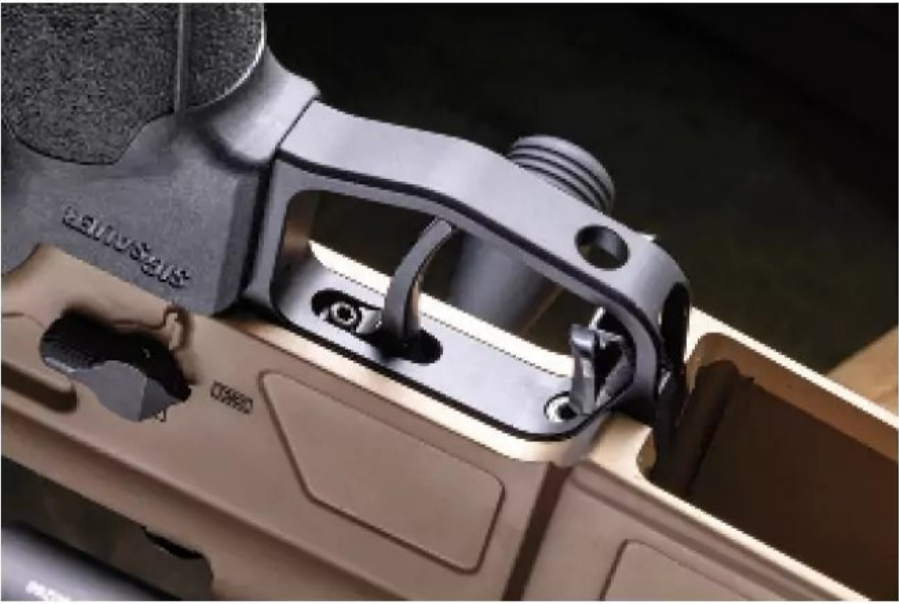
A single T15 screw allows the two-stage trigger to be adjusted for pull weight between 2½ and approximately 4 pounds.
