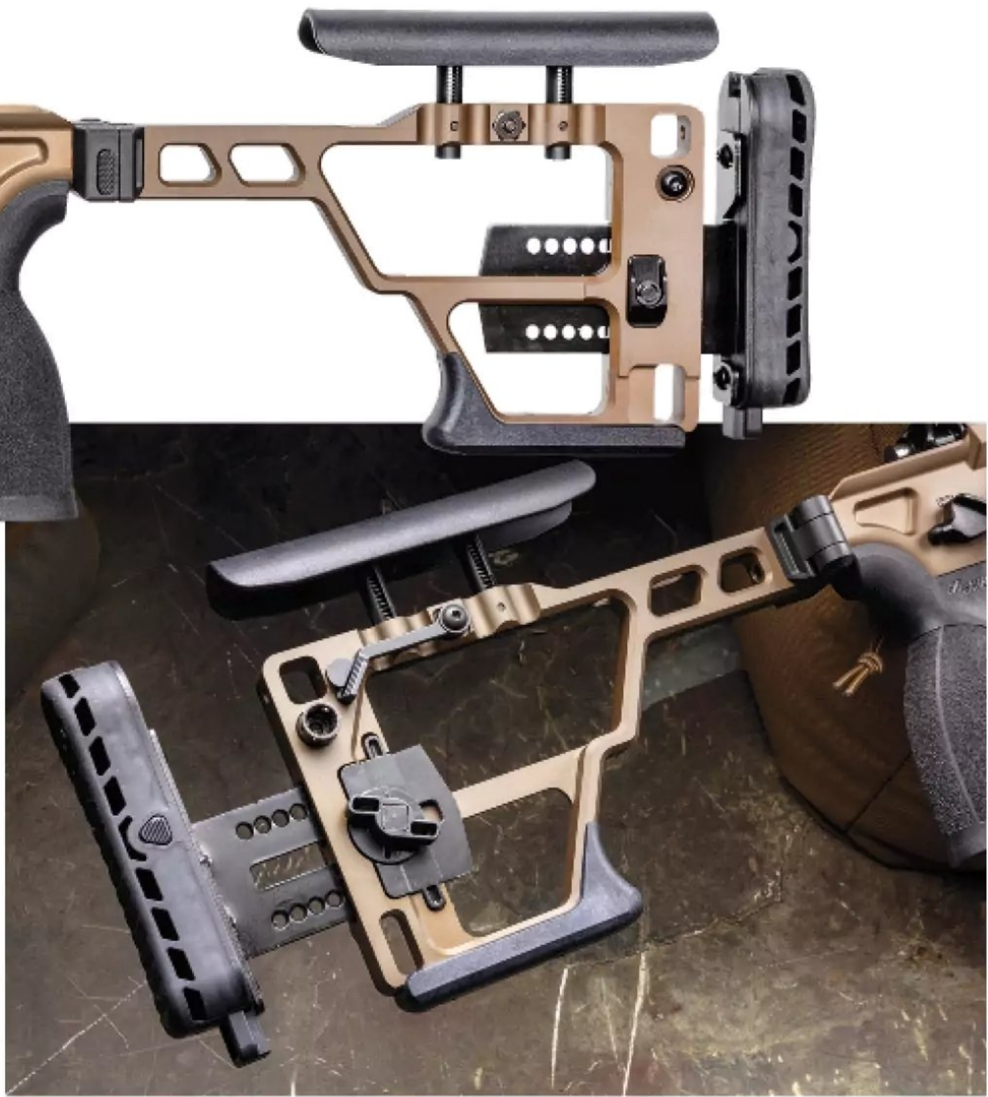
The skeletonized stock has adjustable comb, length of pull, and buttpad height. The stock can also be folded to the right for transport, reducing the gun's length to 36 inches.
