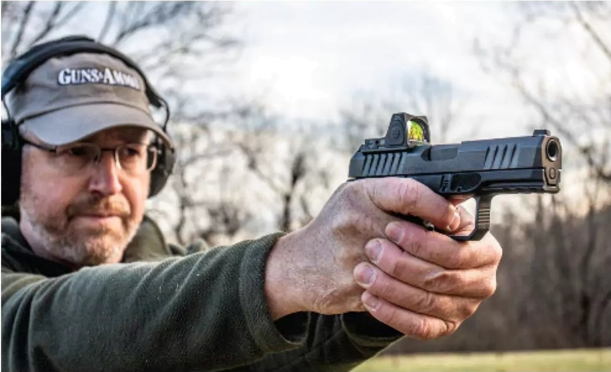
Serrated and textured touchpoints are at the front of the trigger-guard and just in front of the takedown lever. Textured pads on the frame are on both sides, serving as a place to rest your finger while off the trigger or to index your grip with a support thumb.
