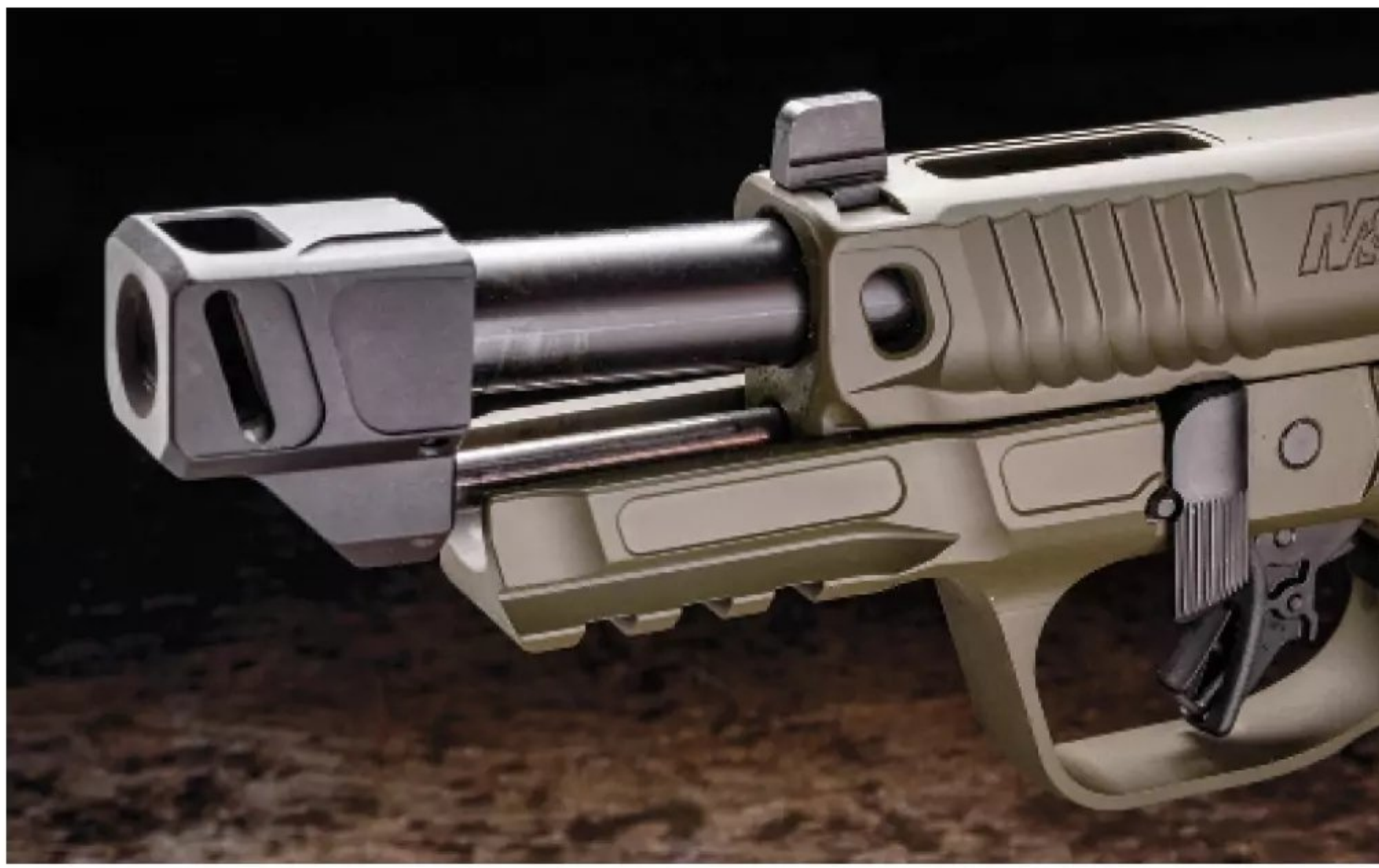
The Faxon compensator diverts gases up like a booster to push the muzzle down during recoil. Lightening cuts in the slide offset the added weight of the comp to ensure reliability.
