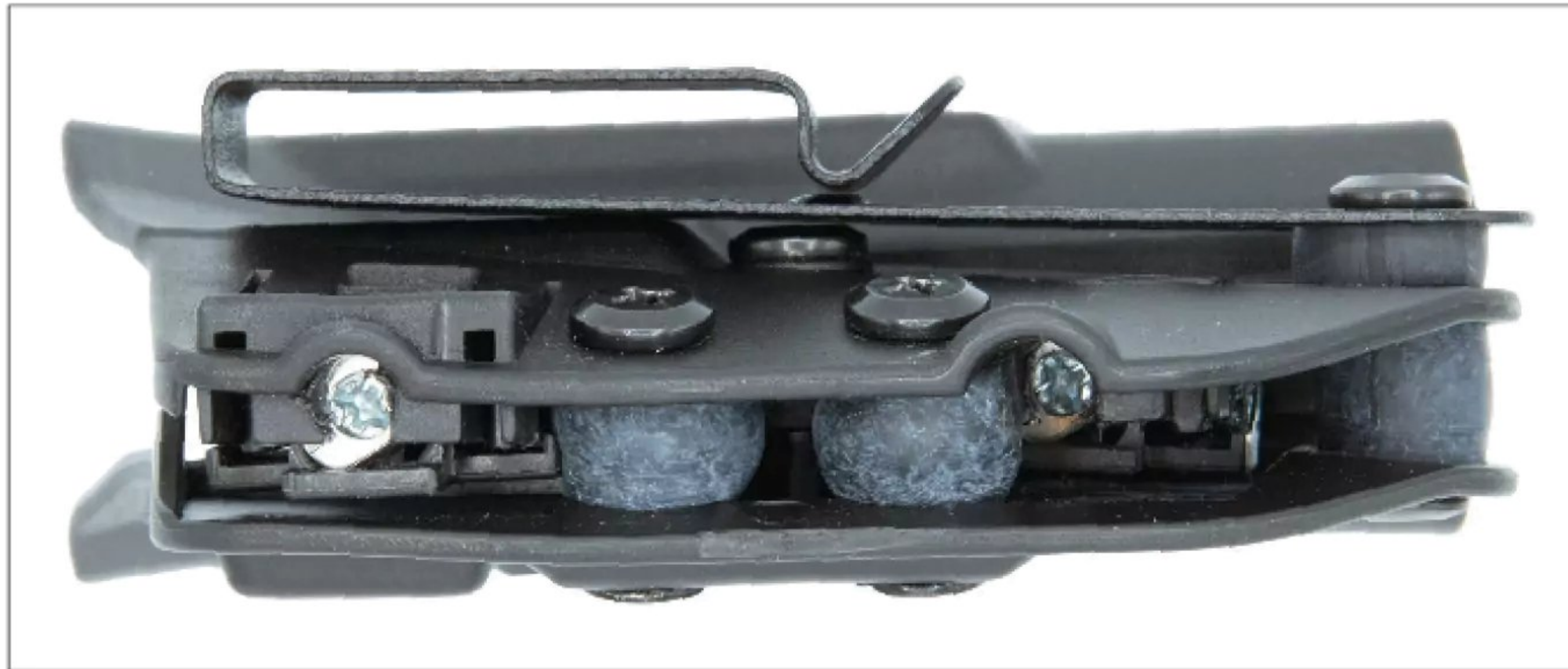
The retention sliders found near the triggerguard expand as the screws are tightened, eventually reaching and maintaining contact with the gun to better hold it in place.
