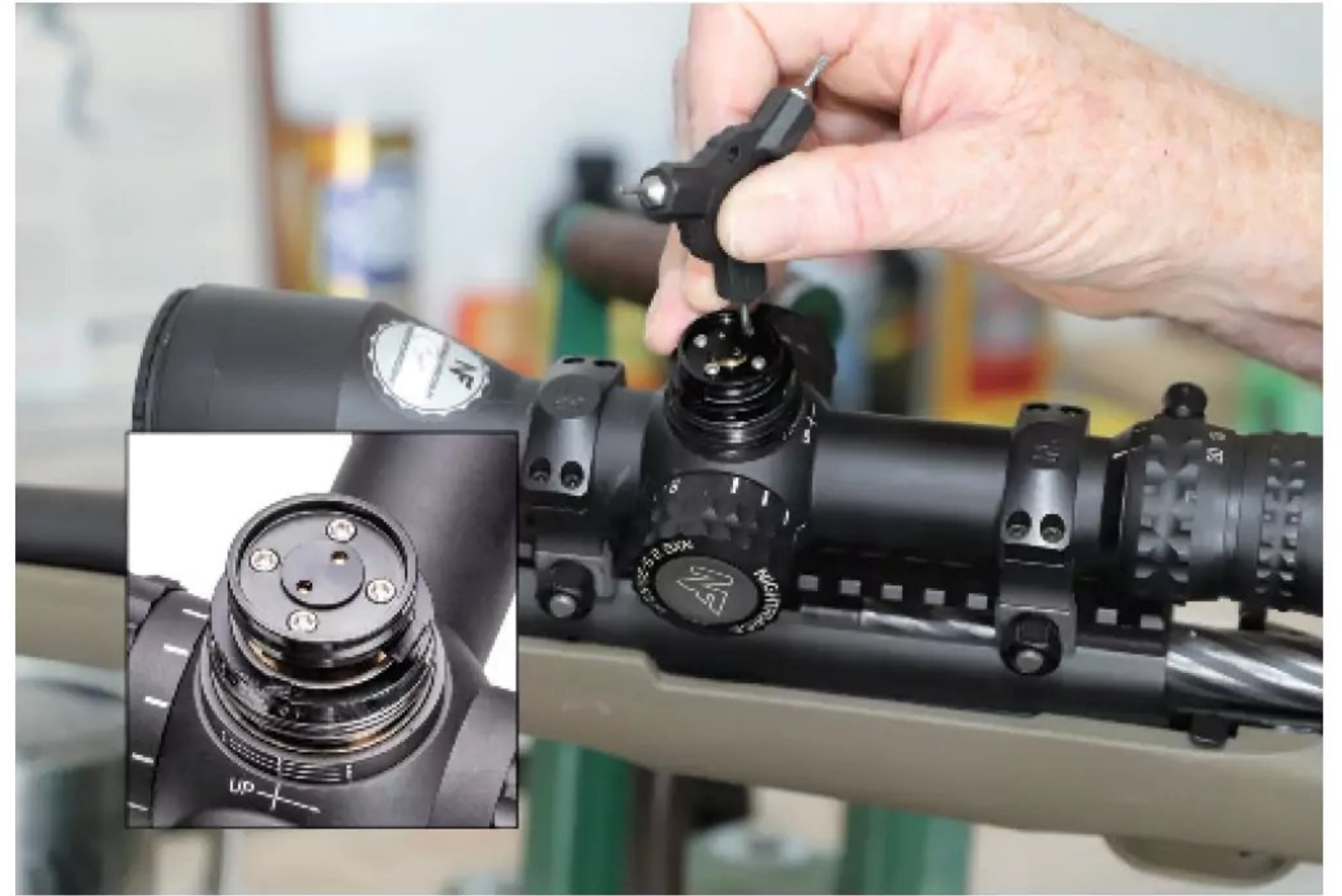
To set the zero stop, remove the elevation cap, loosen the four screws on the upper clutch plate, rotate it clockwise until it stops, then retighten the screws and install the cap.
