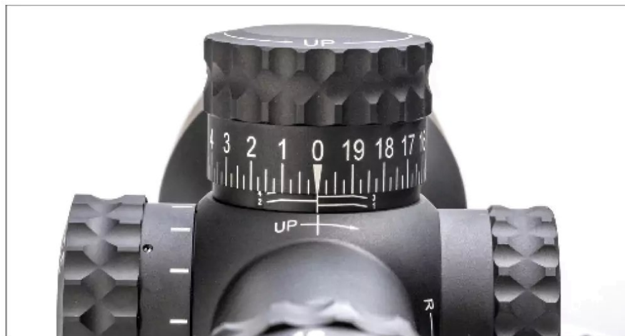
With the zero stop set, the elevation turret only turns counter-clockwise. The horizontal marks at the base of the turret indicate how many revolutions it has been rotated.
