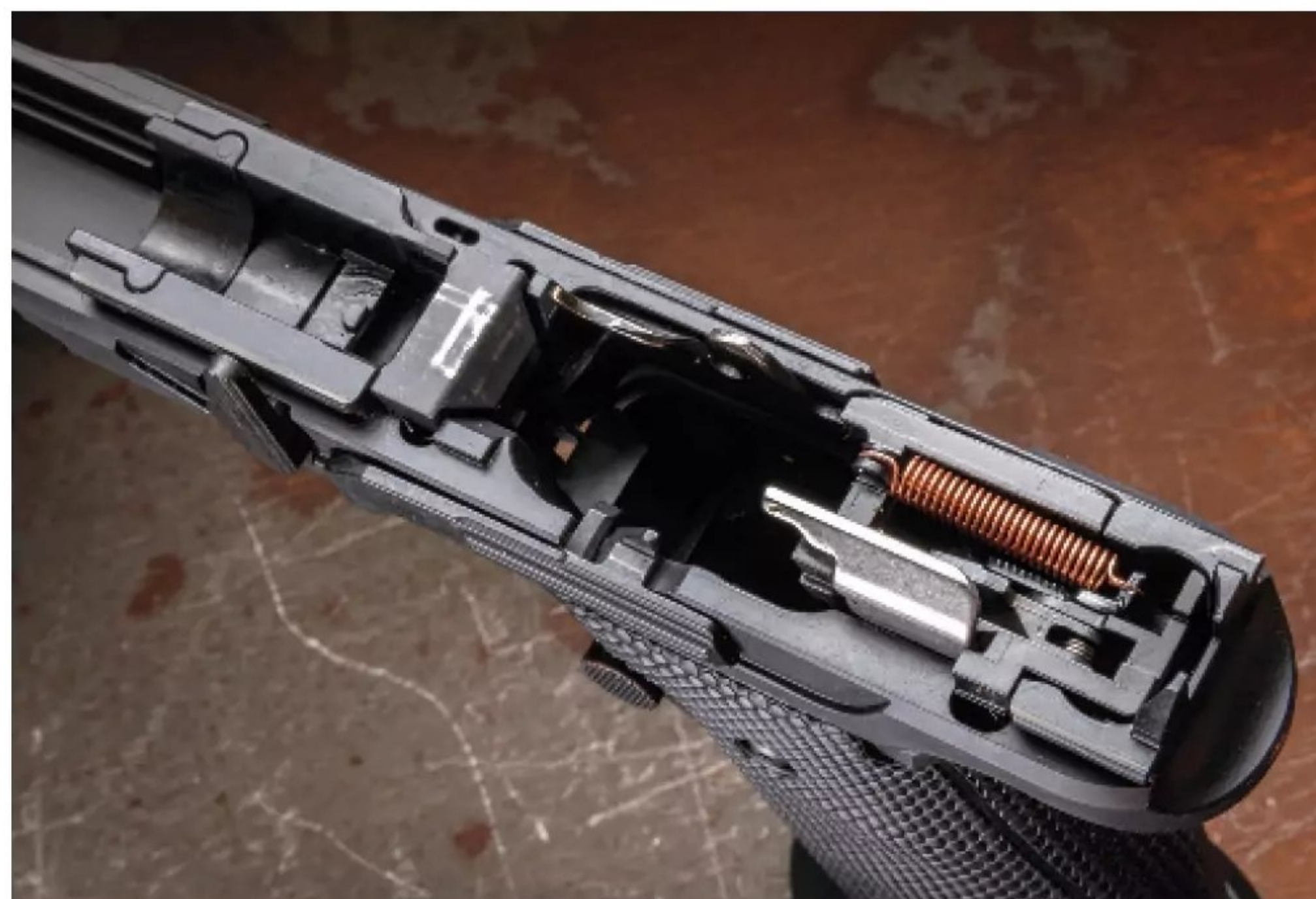
The trigger return spring is similar to the part found in other PDP models, which ensures reliability. Despite the external appearance, the PDP shares several parts with the outgoing PPQ.
