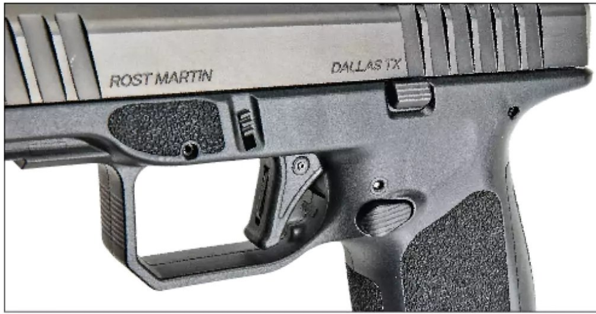
The trigger averaged 5 pounds. It has a wide and flat face, and safety lever. An overtravel stop is molded as part of the frame.
