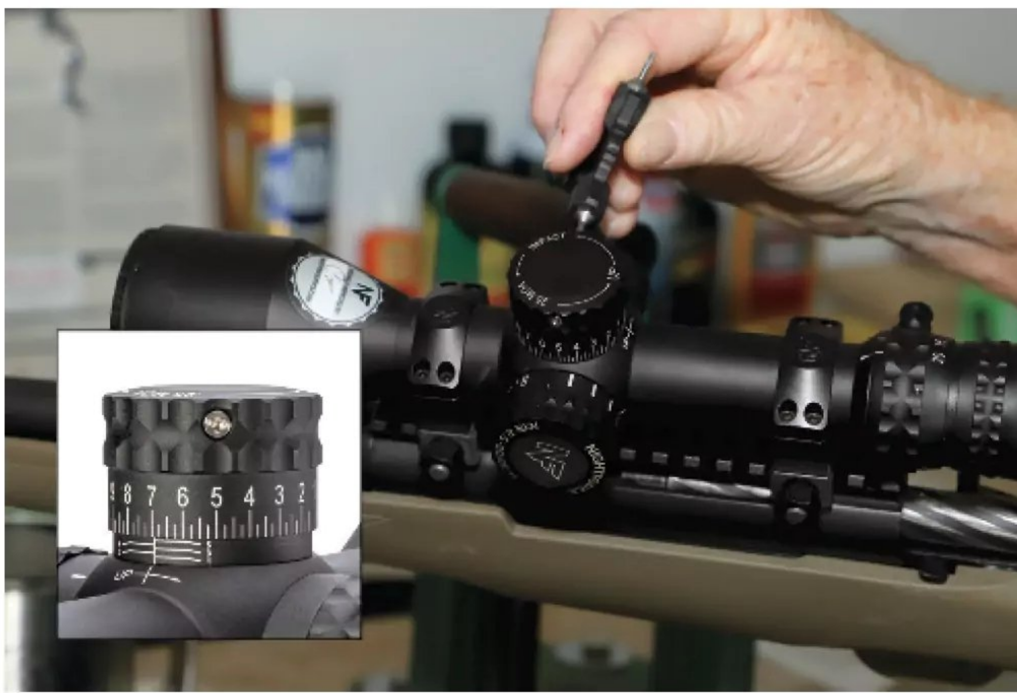
The cap securing the elevation turret cap uses two stainless-steel set screws to guard the zero-stop.
