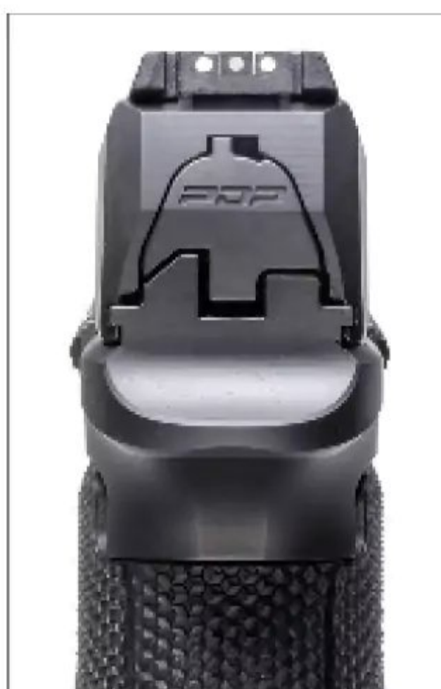
The three-dot polymer sight arrangement is mediocre, and it doesn't co-witness with optics. The rear sight is adjustable, though.
