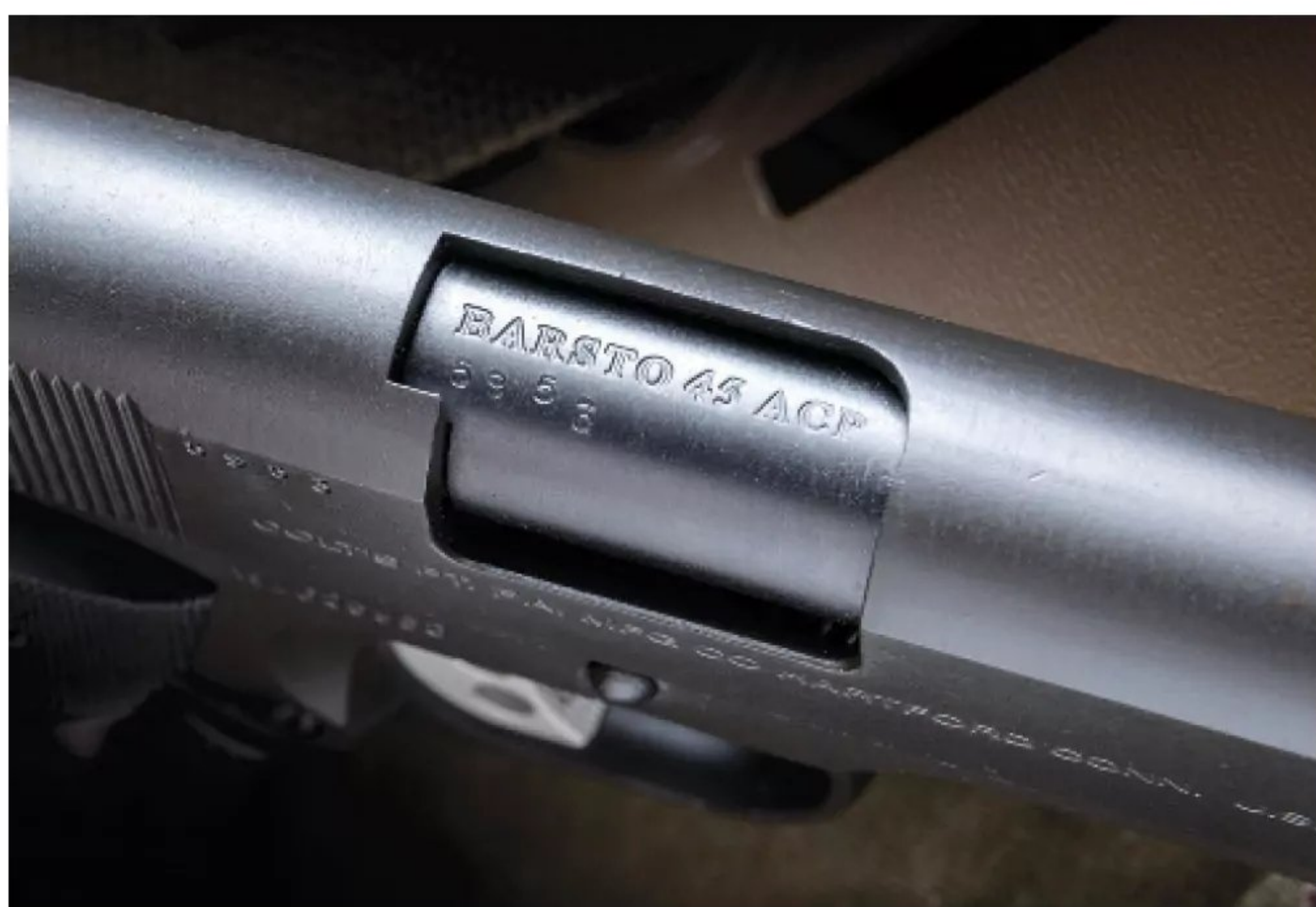
Armorsmiths installed Bar-Sto semi-fit barrels to the GI slide. These barrels were necessary for enhanced accuracy on missions such as in-extremis hostage rescue (IHR).
