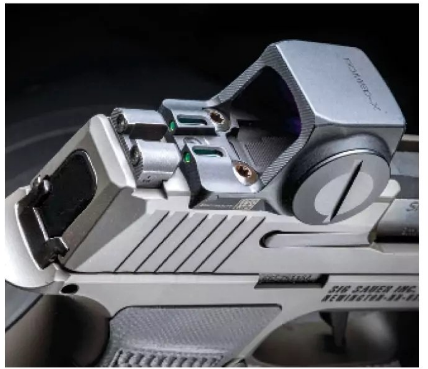
The P365XL-length slide features a pair of compensating ports that reduces muzzle flip. The front X-Ray3 day/night sight is dovetailed just behind the comp. The rear sight co-witnessed in the lower third with the low-mount Romeo-X reflex sight.
