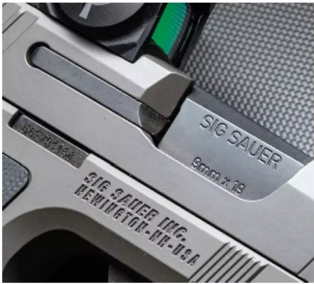
The P365-AXG Legion maintains the design's external extractor and angled bevel to ensure problem-free ejection.
