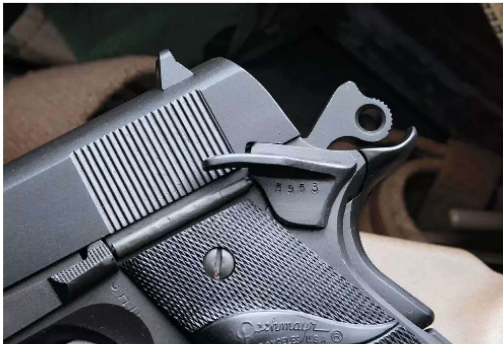
The M45 replaced the GI spur with an aftermarket Commander-type hammer. The armorers also fitted the frames with a Wilson 66 beavertail grip safety.
