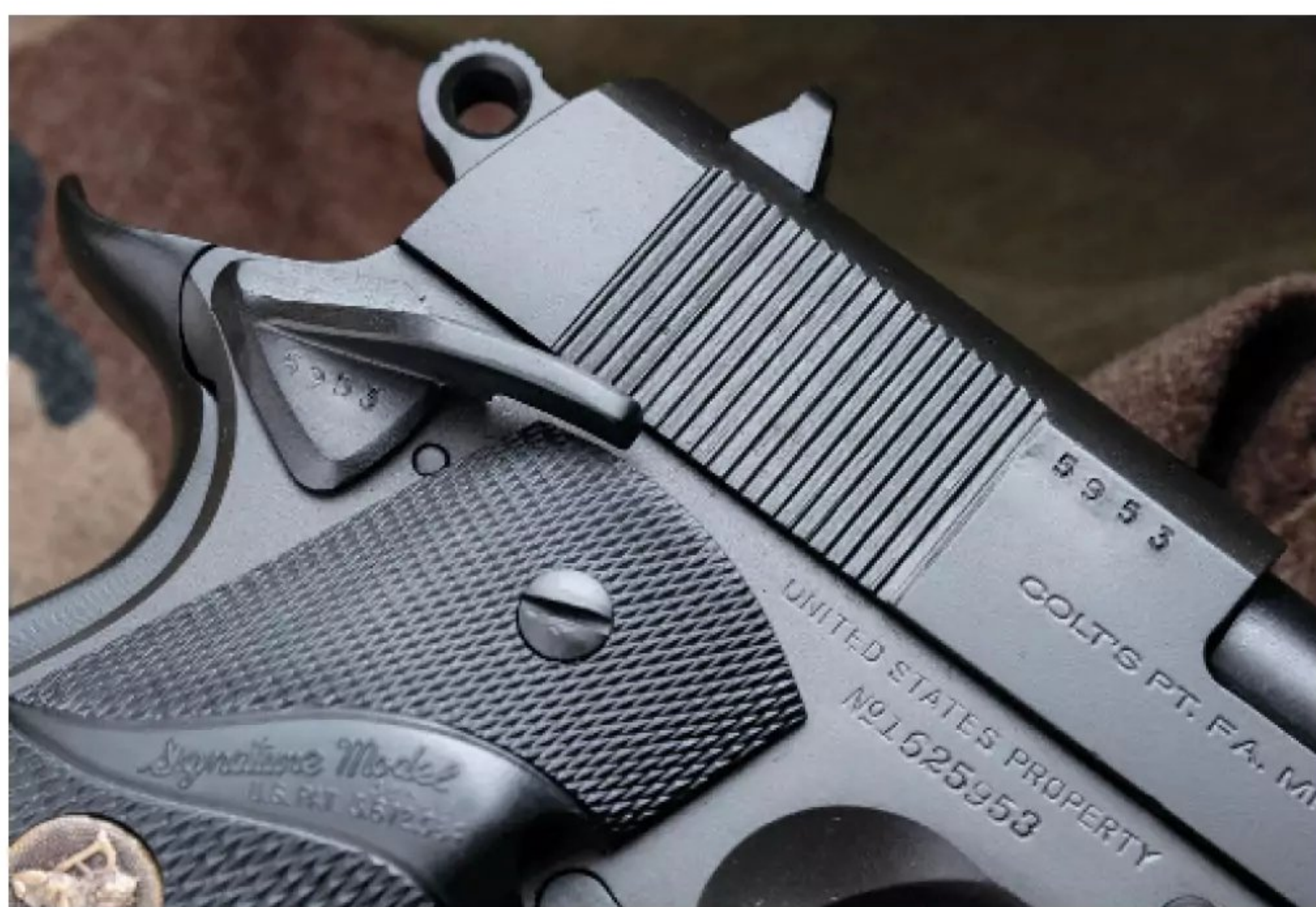
The Kings 201-A thumb safety lever was considered more robust than the competition-style levers on match pistols. All M45s were fitted by armorers with ambidextrous safety levers.
