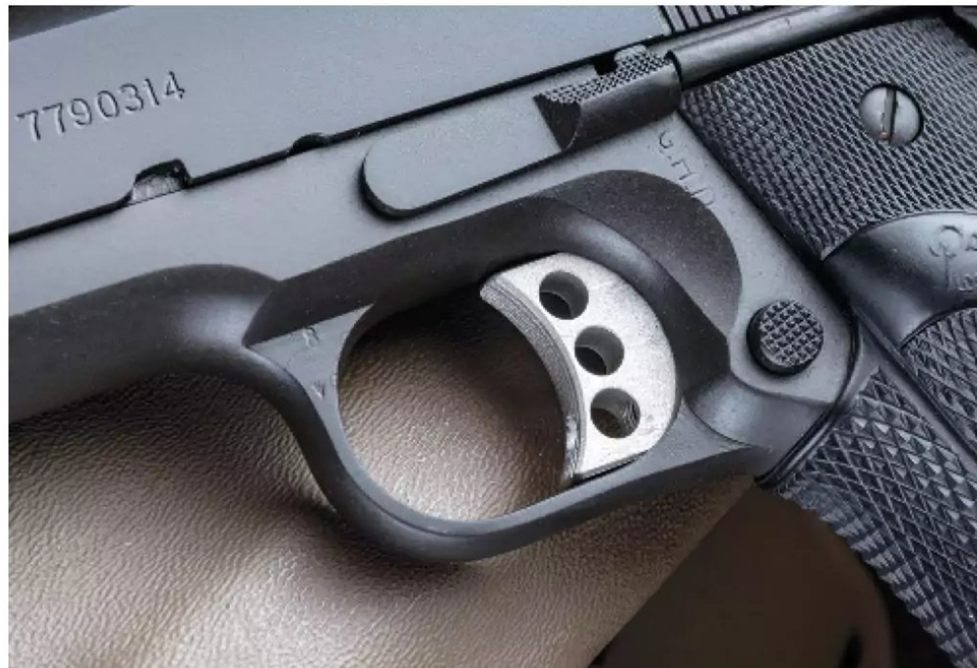
Unique to the M45 is the Videki three-hole speed trigger. Marine armorers removed the overtravel screw and welded the hole. The checkered-type slide-lock lever and mag release button were GI.
