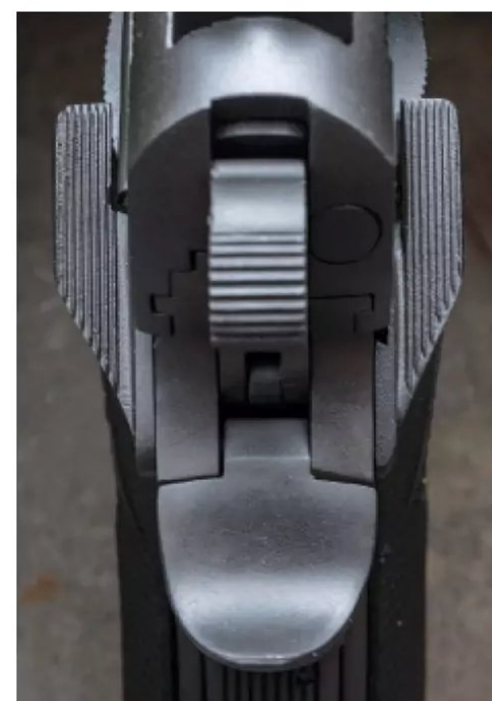
The extended thumb-safety levers assisted operators wearing gloves when shooting.
