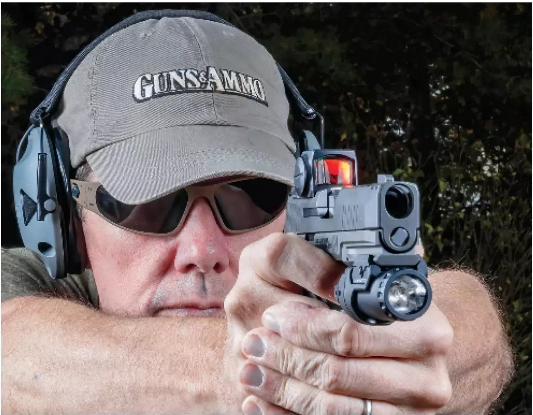
The muzzle of the 3.1-inch barrel is recessed within the slide. Note the angular bevels at the front of the slide and dustcover. These angles aid in reholstering, especially with tight IWB rigs.
