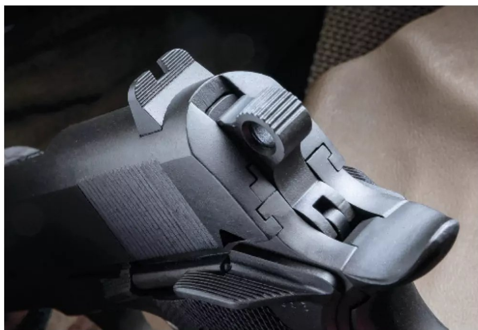
Match armorsmiths custom-made rugged, high-profile serrated sights from barstock and pressed them into the standard dovetail cut.
