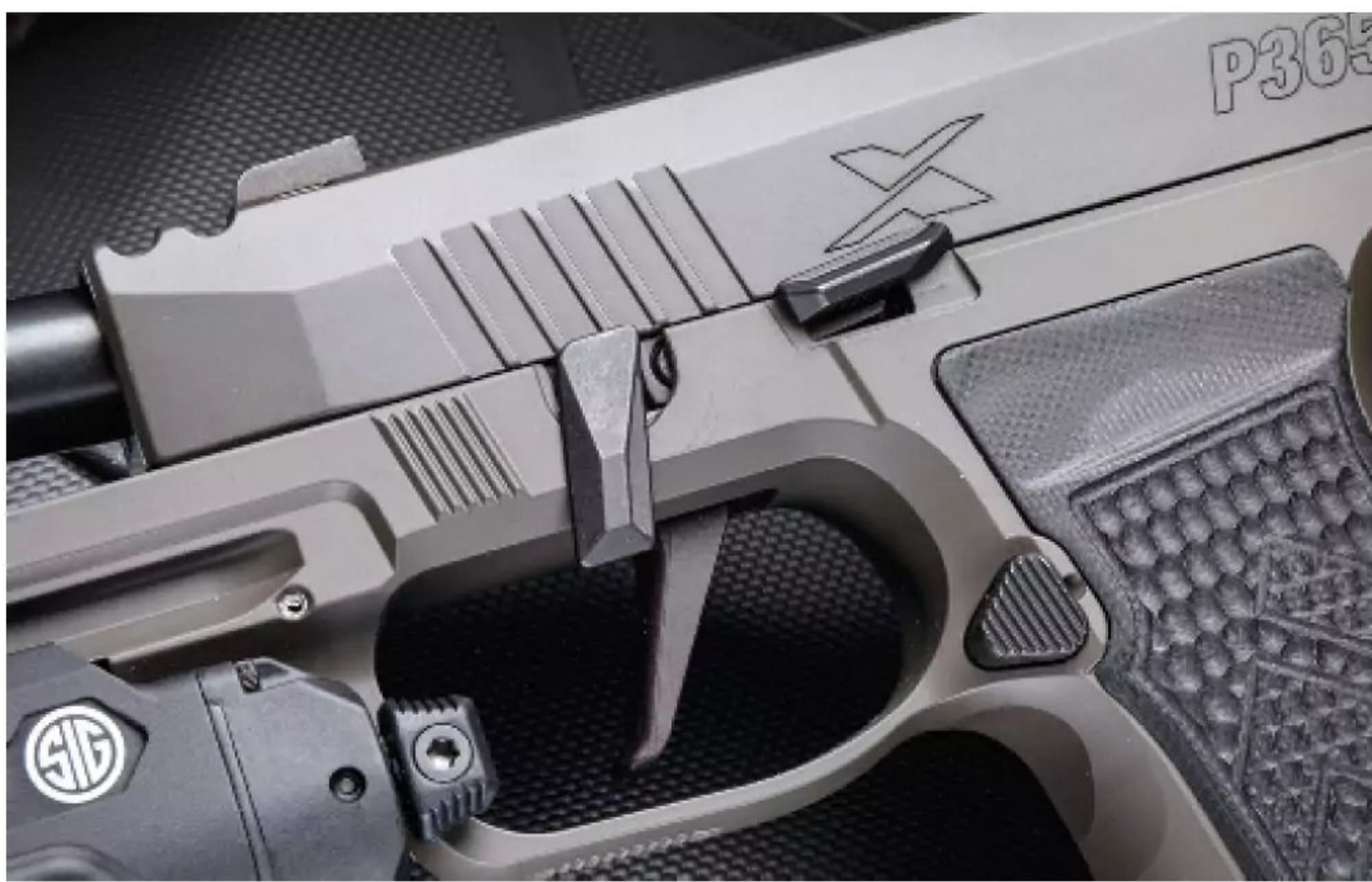
The slide catch is an extended version of the standard P365 unit. To the left is the takedown lever. With the slide locked back, the takedown lever can be rotated 90 degrees down for disassembly.
