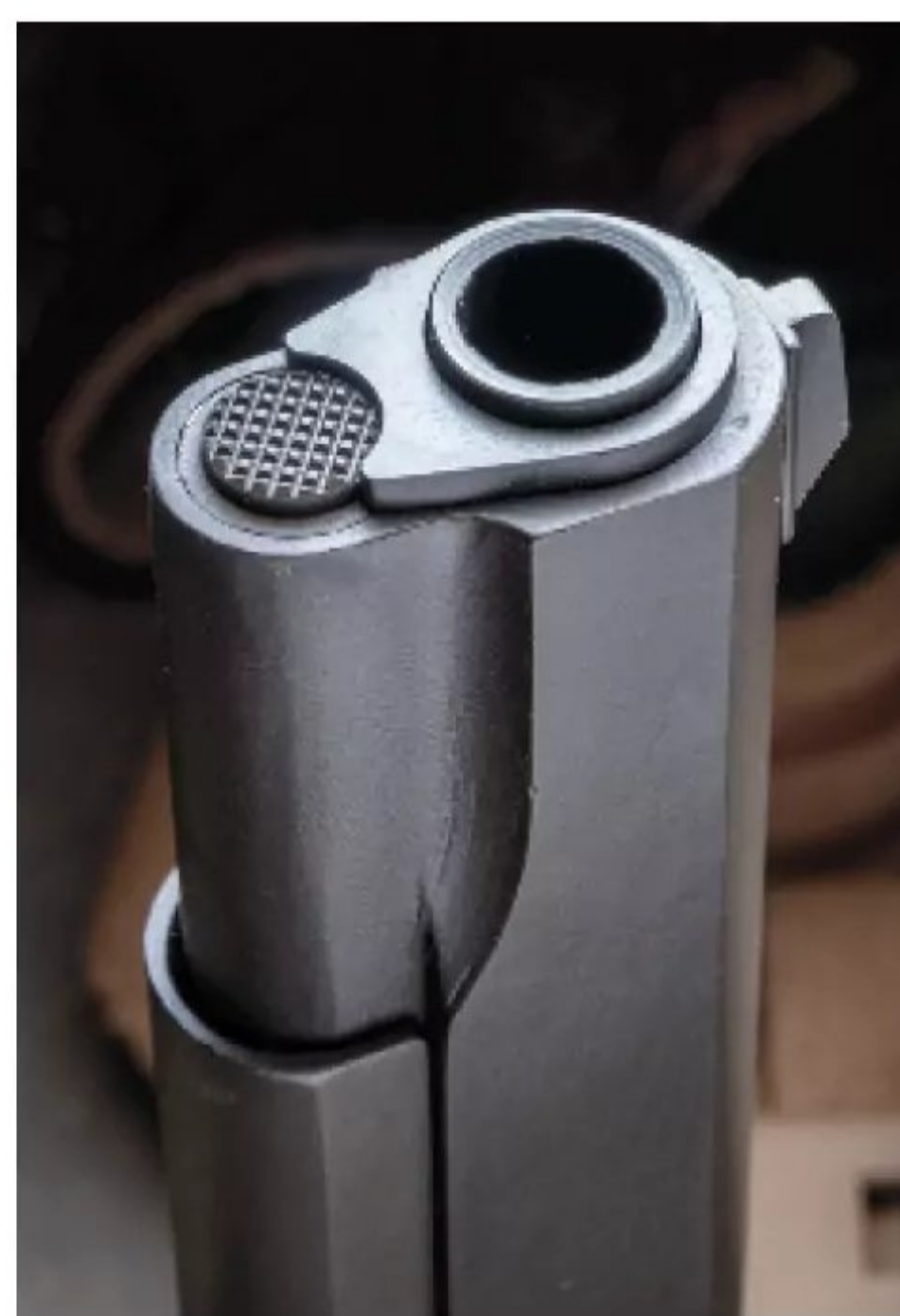
The bushing was included with each Bar-Sto semi-fit barrel. The checkered plunger was GI.
