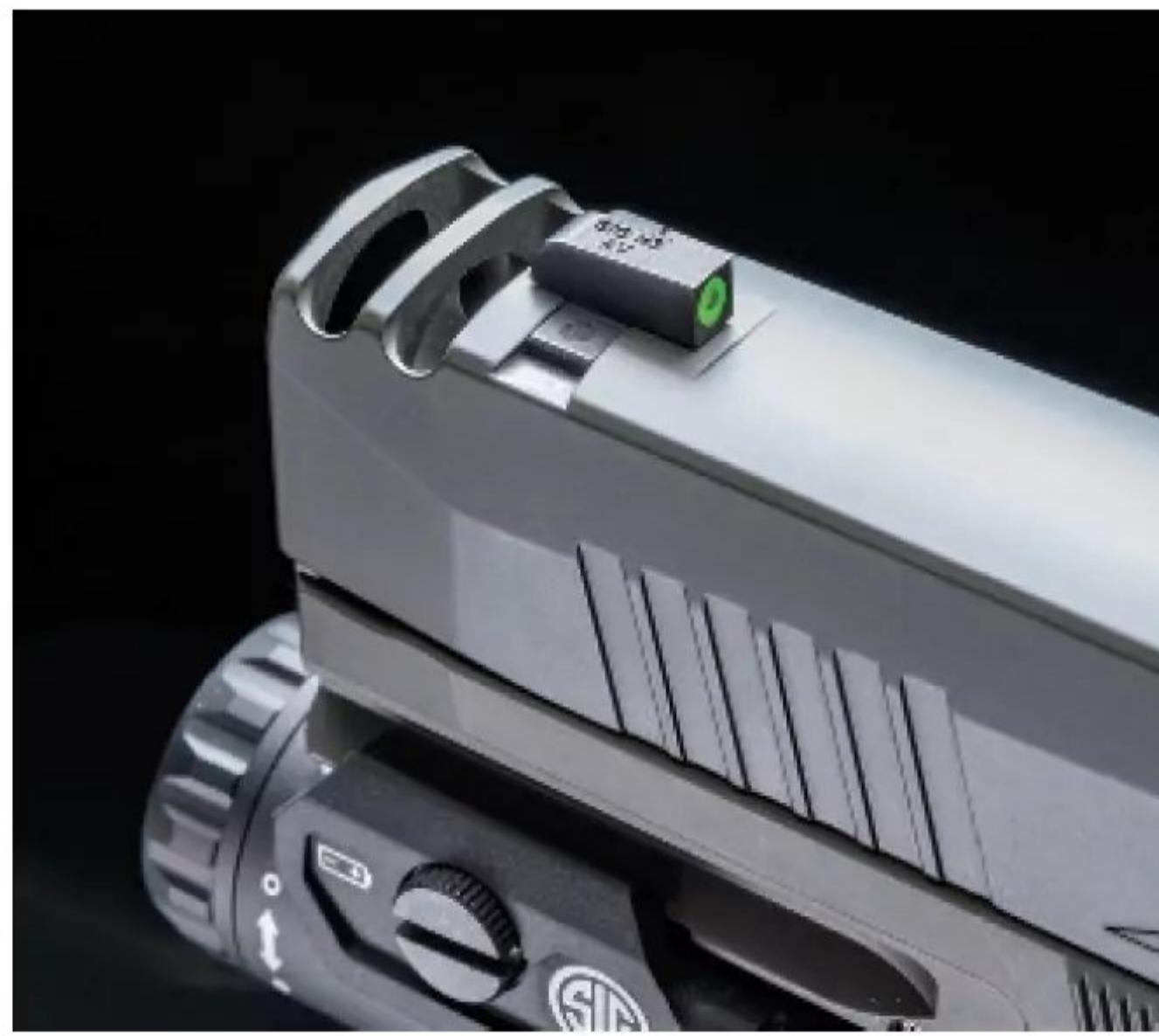
The P365XL-length slide features a pair of compensating ports that reduces muzzle flip. The front X-Ray3 day/night sight is dovetailed just behind the comp. The rear sight co-witnessed in the lower third with the low-mount Romeo-X reflex sight.
