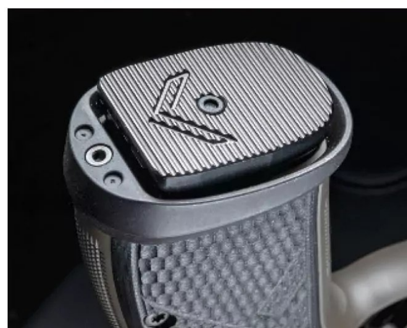
The aluminum magwell supports a positive grip and has a flare underneath to assist smooth reloads. Held on by a screw, it is removable for those wanting a more flush and concealable profile. Magazines carry 17 rounds and have the Legion basepad.
