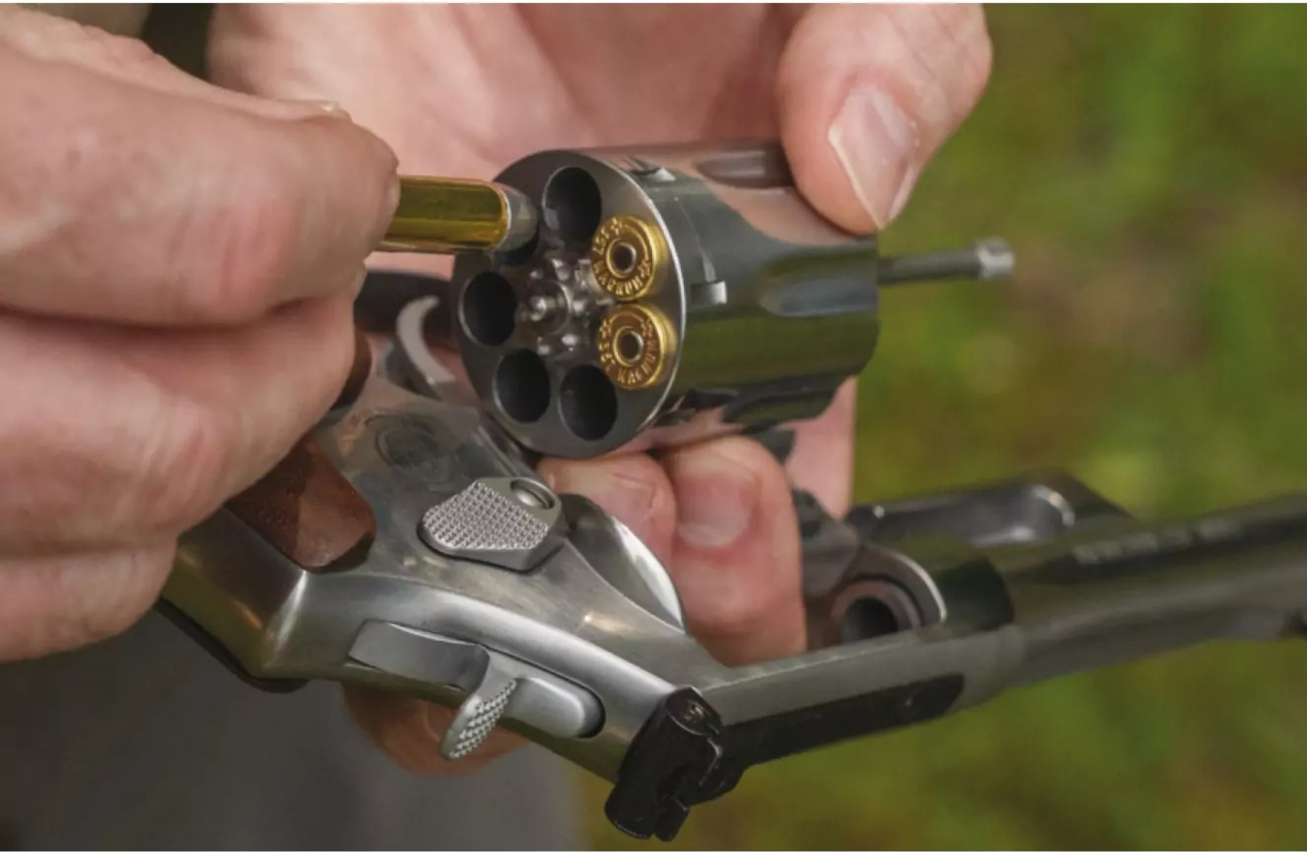
The 686 Plus Mountain Gun from Lipsey's holds seven, as opposed to six, rounds of .38 Special or .357 Magnum ammo.
