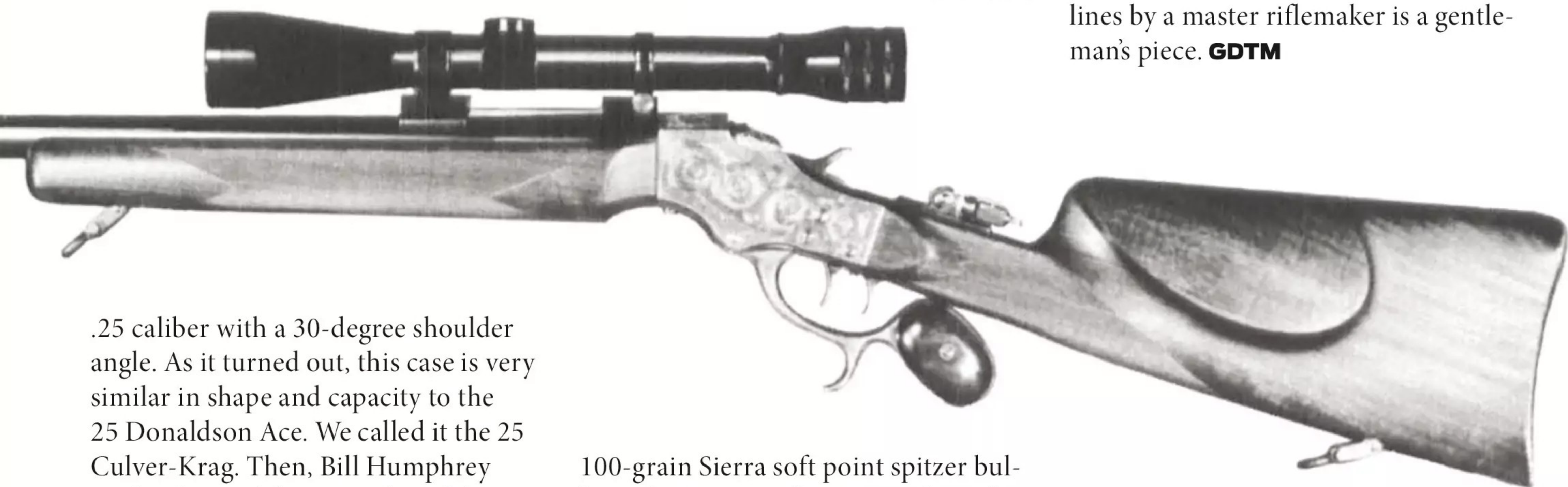
Rifle for the 22-3000 towell R2 cartridge, with Stevens No. 44½ action, owned by James P. Garland. Diller barrel, stock by Humphrey, 6X Bear Cub scope. This rifle has accounted for hundreds of woodchucks and hawks.
