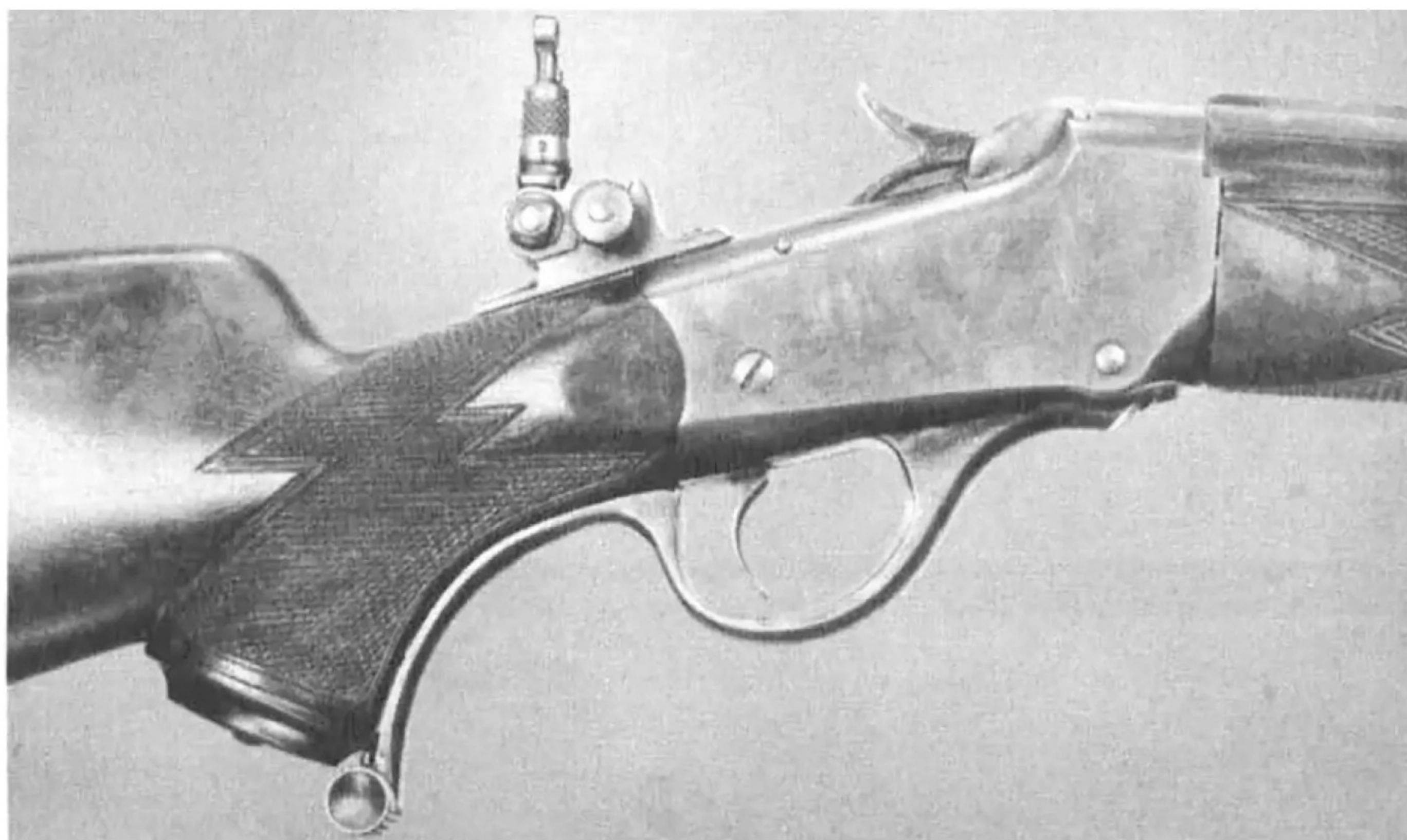
Winchester single-shot rifle for the 25-20 W.C.F. cartridge, with stainless steel barrel. Stock and lock work by Clyde Baker. The first attempt to solve the corrosion problem resulting from chlorate primers.
