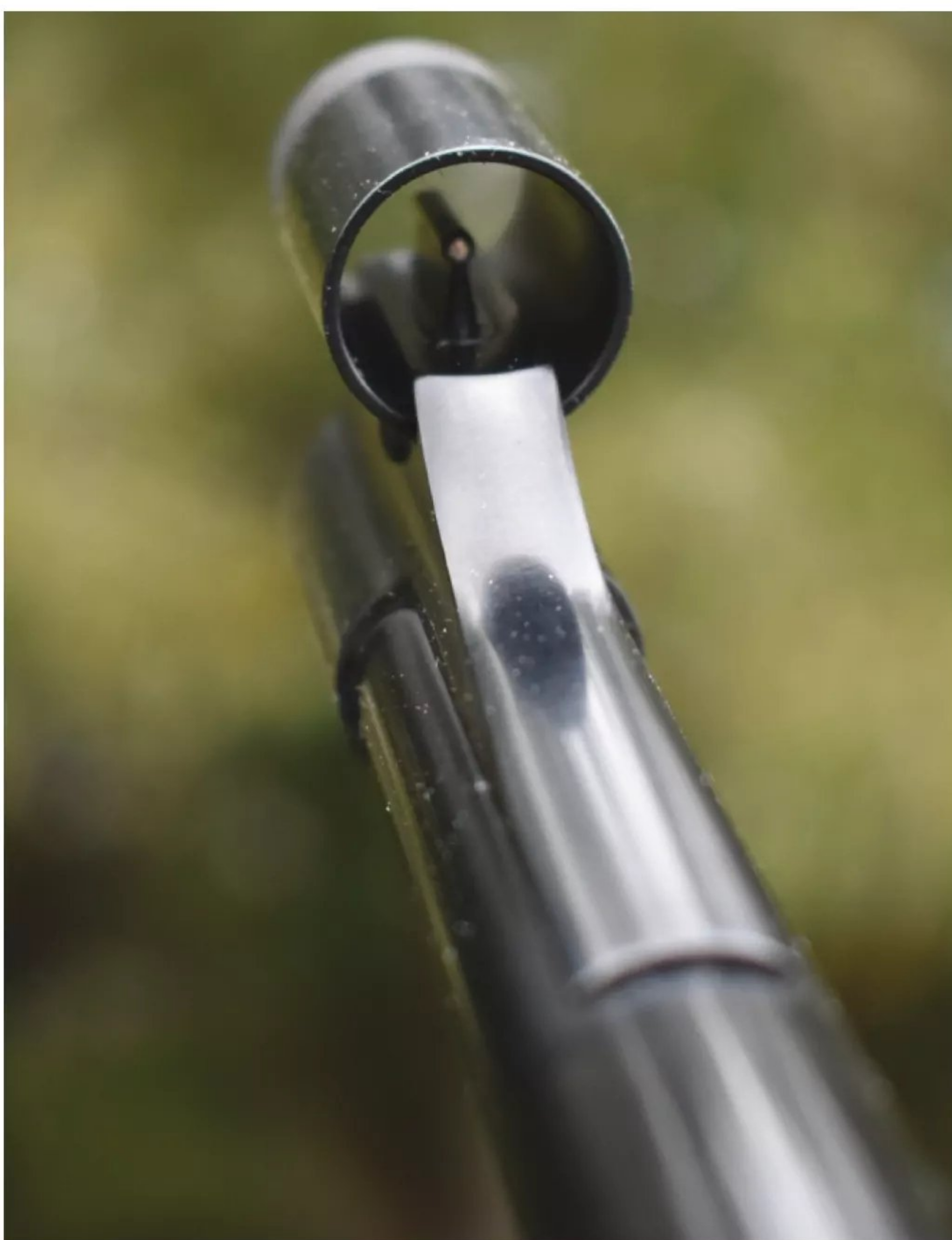
The banded ramp front sight matches up with the express rear sight mounted on a quarter rib.
