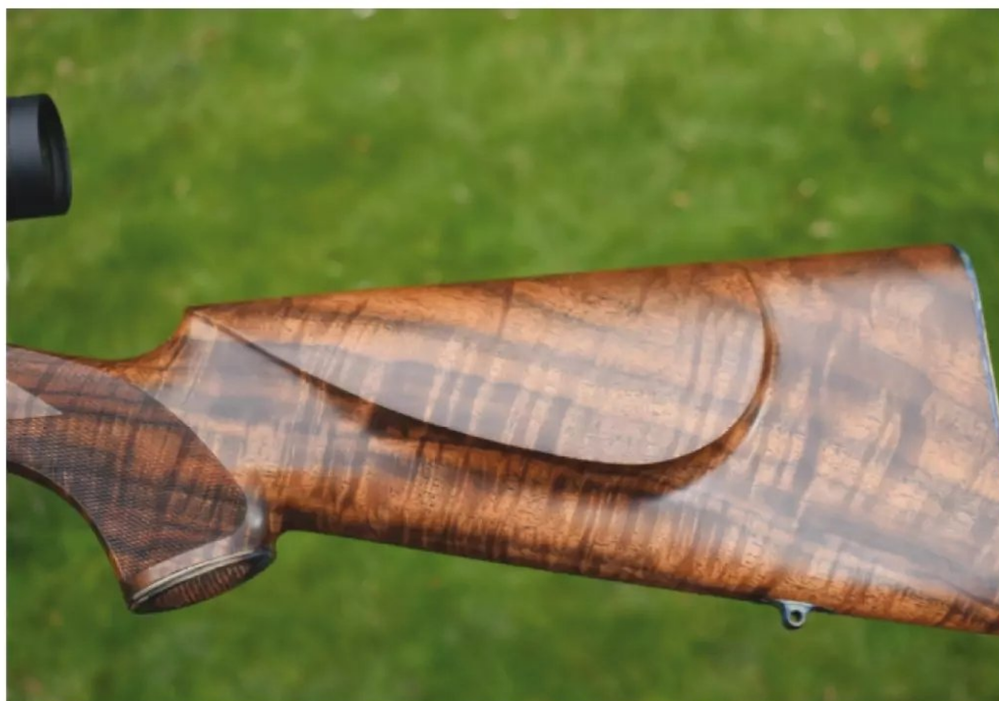
Several of the custom touches include a steel buttplate, skeleton grip cap, Howell swivels, and the cheek-piece and checkering.
