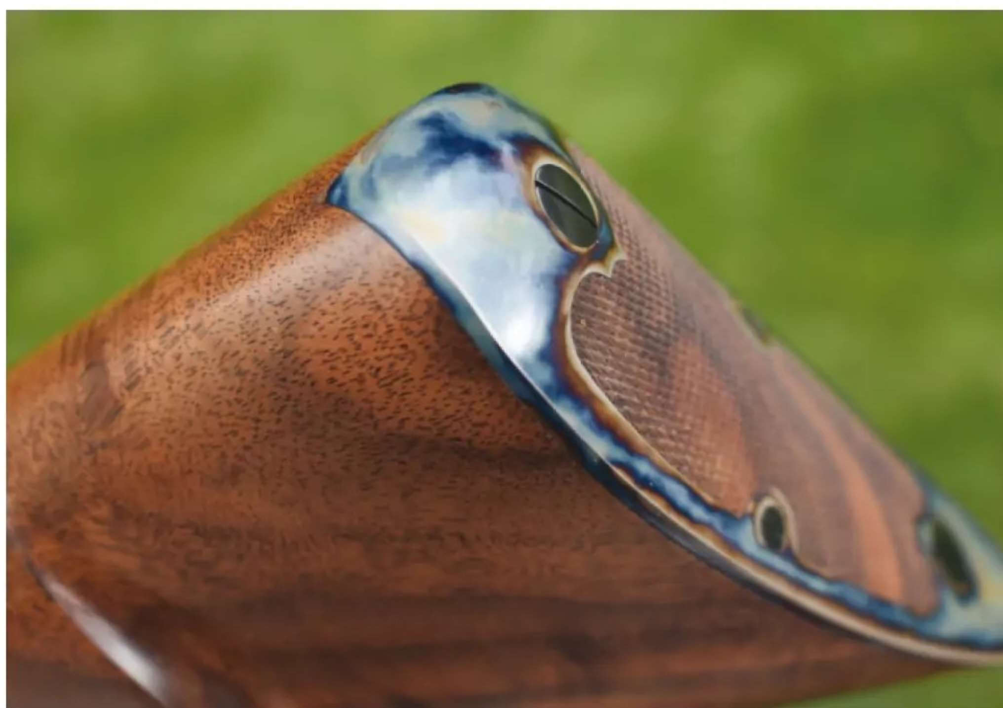
Note the nicely executed skeleton buttplate with a widow's peak. It looks like the wood grew around it.
