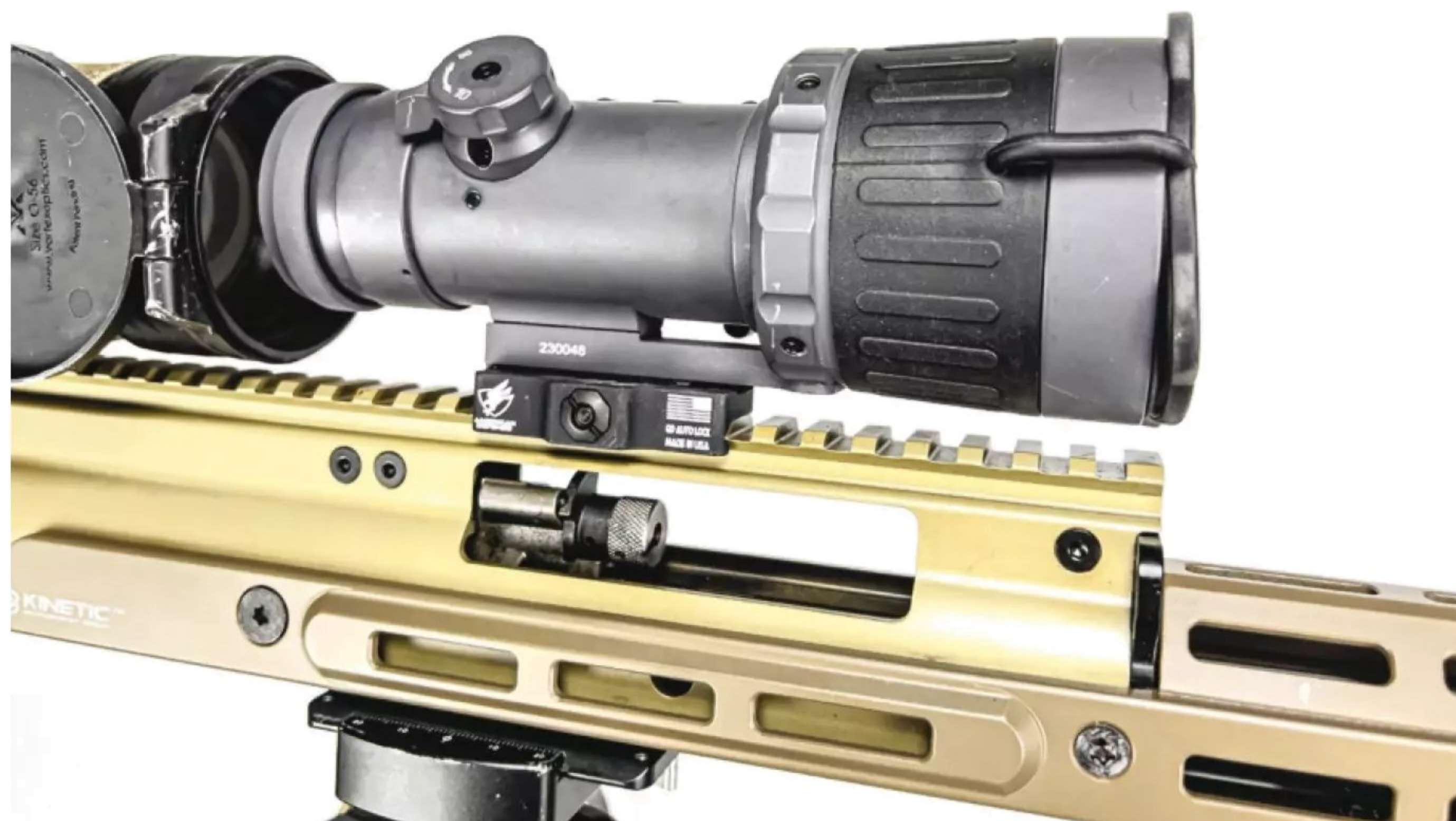
The SCARburator adjustable plug is visible inside the window above the handguard. Rail system by KDG, night vision clip-on by Armasight.
