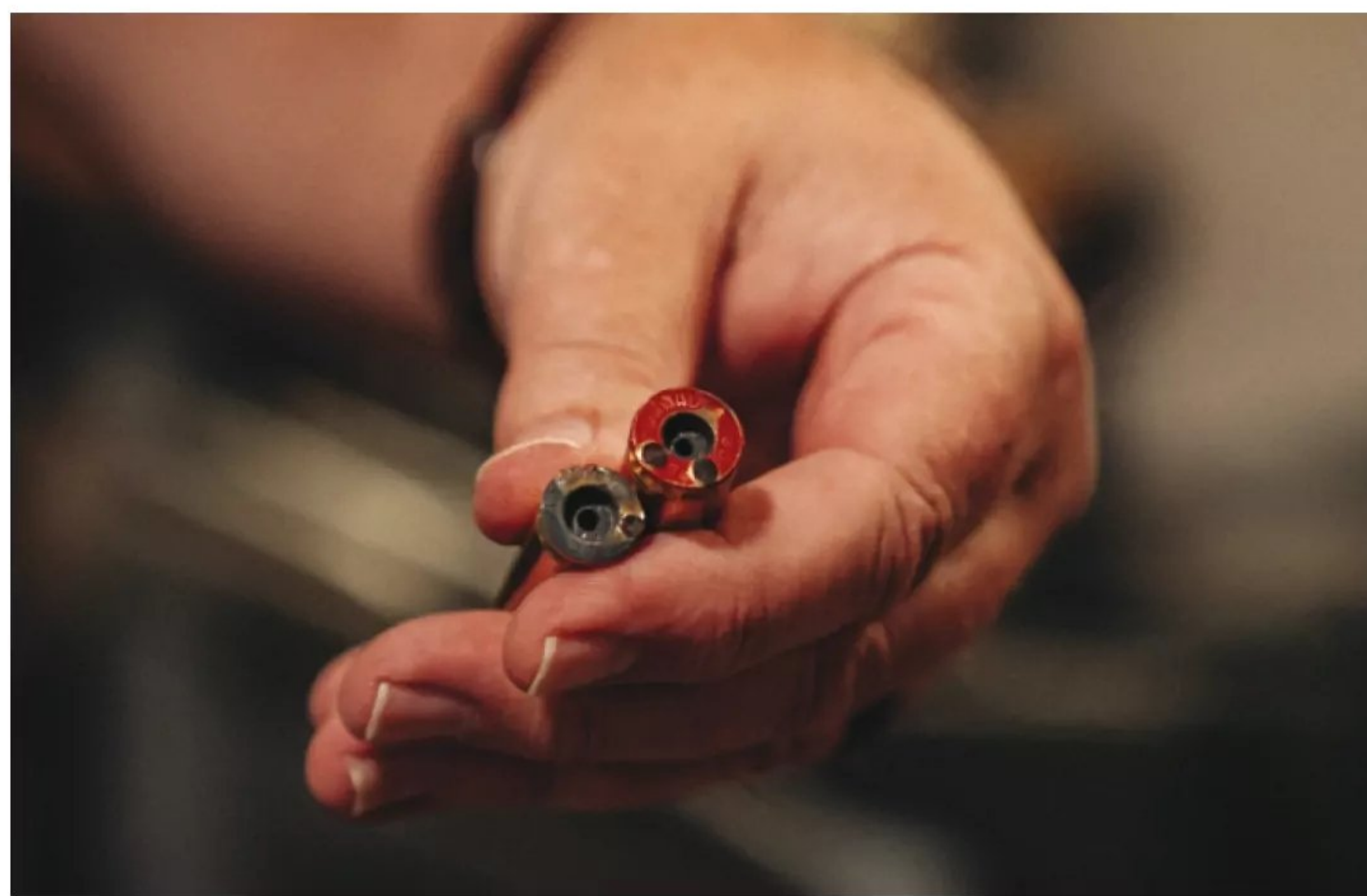
This is something you don't see very often: the case from the proof load that was fired in the Ridgeline FFT test rifle. Proof loads are fired at extremely high pressure to test all new Christensen Arms rifles. (Photo: Christensen Arms)
