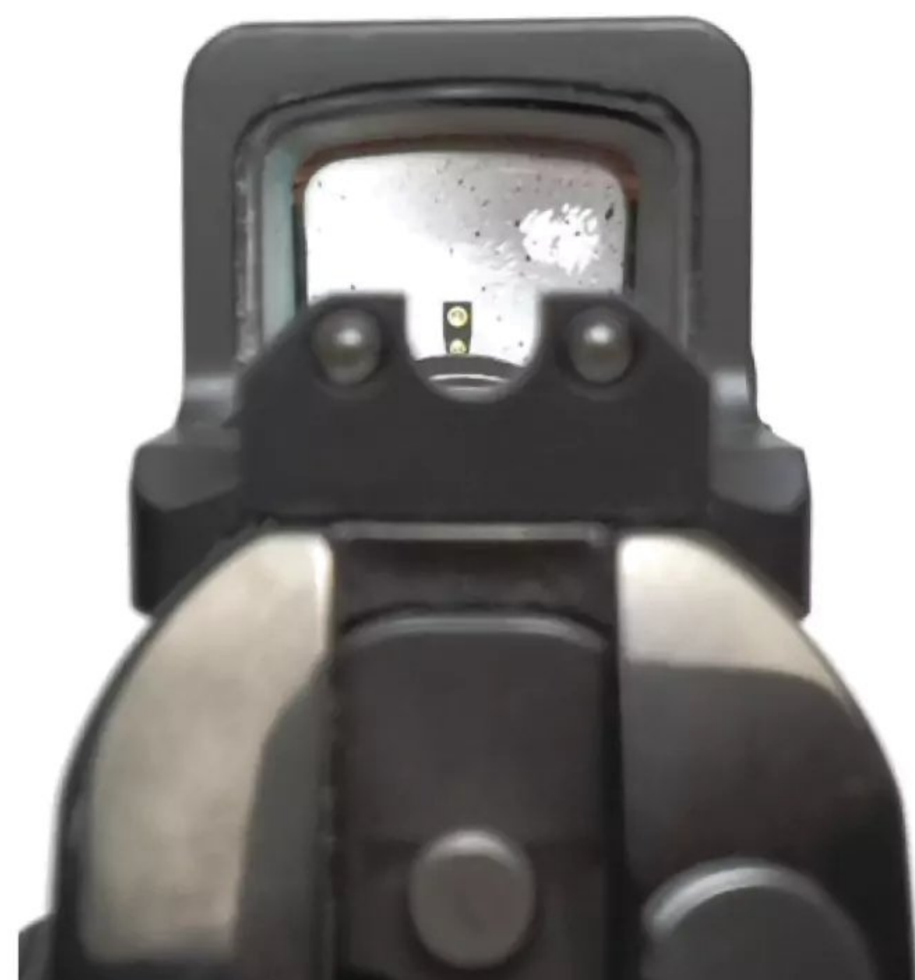
(Right) Co-witnessed irons are an important secondary aiming feature when using electronic sights. Note the dirty lens from being shot suppressed. Something to keep in mind is that dot sights can get filthy in use ... so have good irons.
