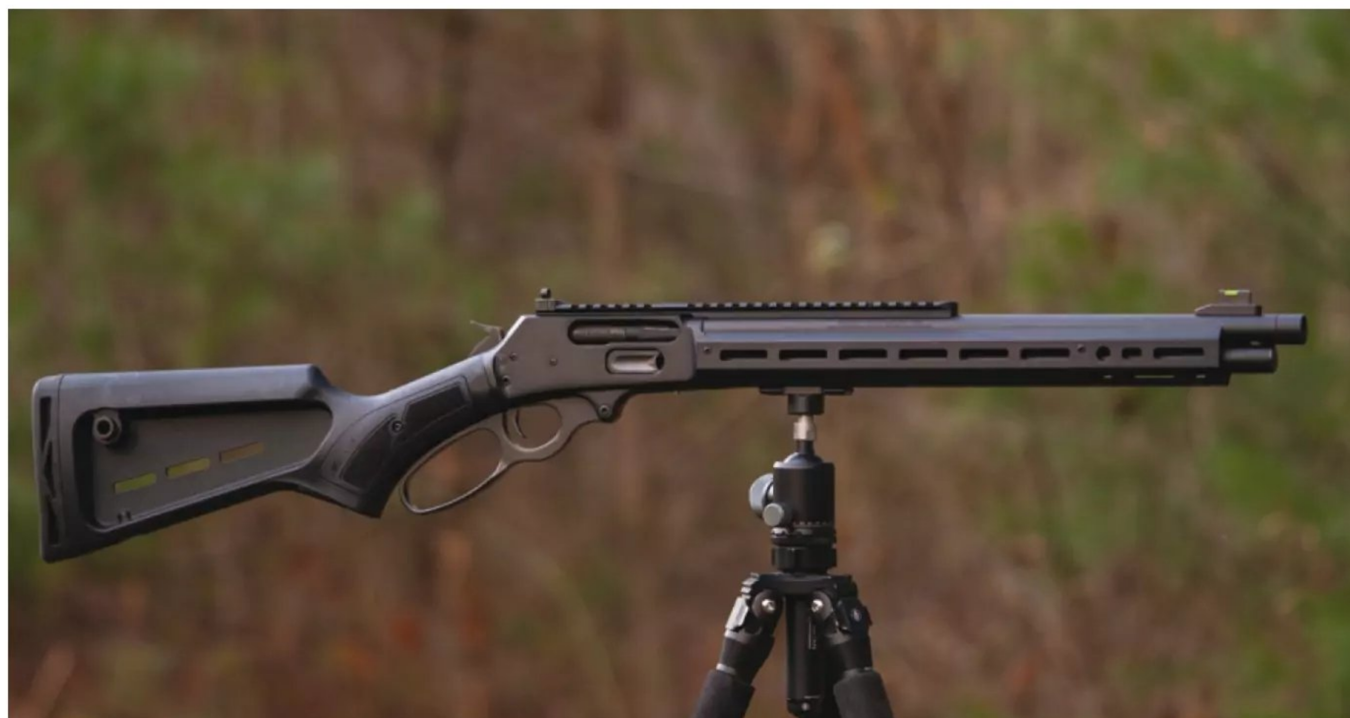
The M-Lok forend of the Marlin 1895 Dark rifle allows for the attachment of various shooting supports. Photo credit: Sebastian "Bat" Mann
