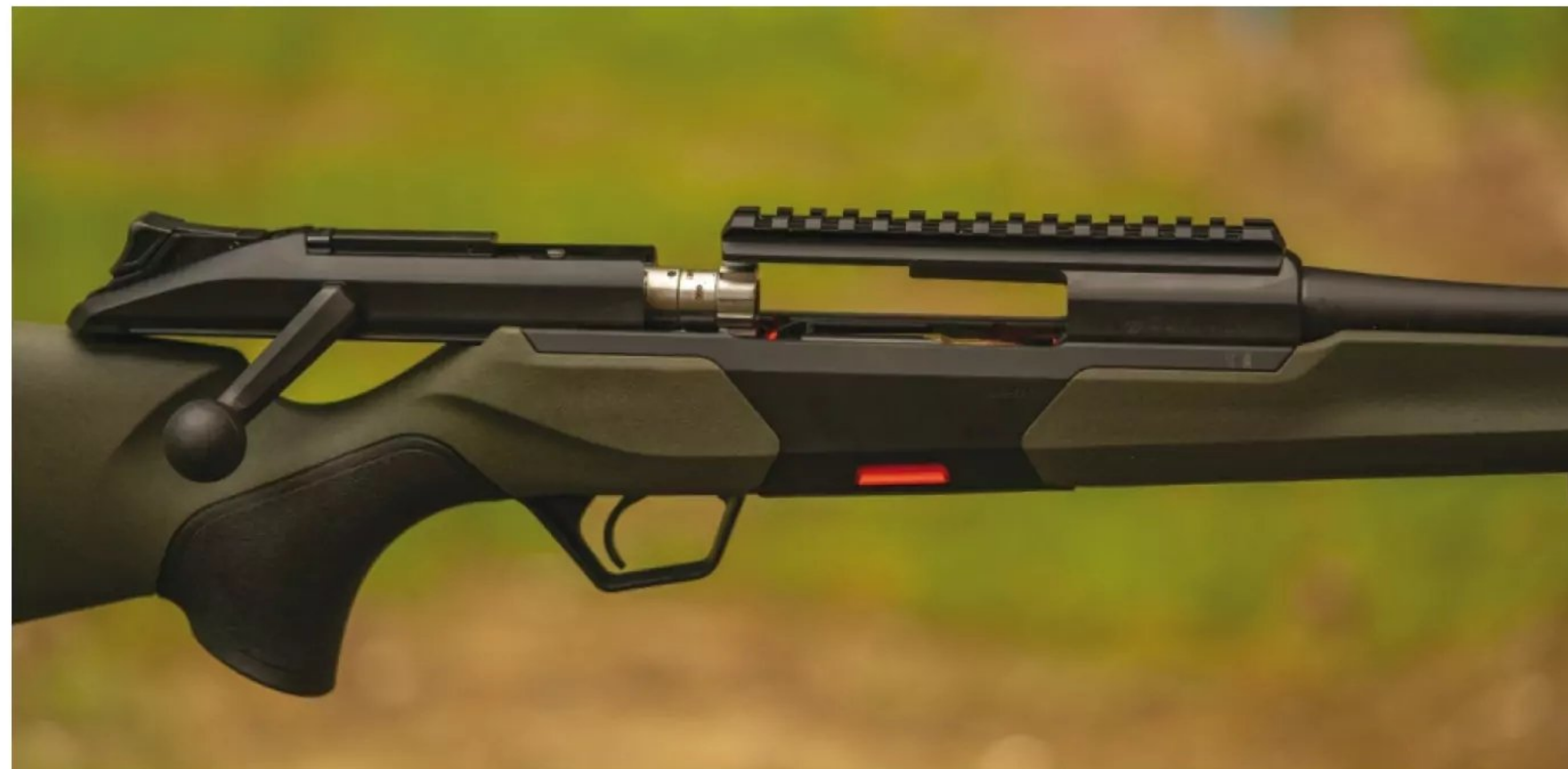
The straight-pull action of the Beretta BRX1 is a bit odd, but it functioned easily and flawlessly, and the rifle shot very well. Photo credit: Sabastian "Bat" Mann
